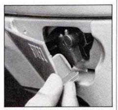
The fuel tap is positioned behind this filmsy plastic door. On a cold day with thickly gloved hands, turning the tap isn't easy.
