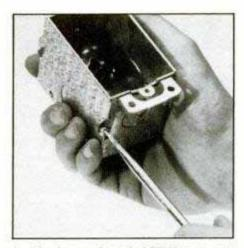
Junction boxes, also called GEM boxes, must enclose and protect all splices, connections, switches, outlets and other in-wall wiring flxtures. Surface wiring boxes are slightly different. This in-wall wiring junction box has removable ends so two or more boxes can be ganged to make one larger box.
