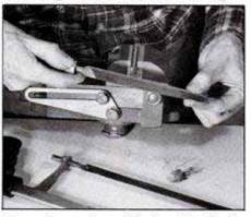
To reduce shop injuries, "pull the teeth" of bars, rods and other metal stock stored for future use. Whenever a piece is sawed from some metal stock, file off the sharp edges and corners on the remaining portion before storing it. Later, you'll be less likely to cut yourself when searching through the assortment of stored items. Work gloves add protection, too.—W.E. Burton
