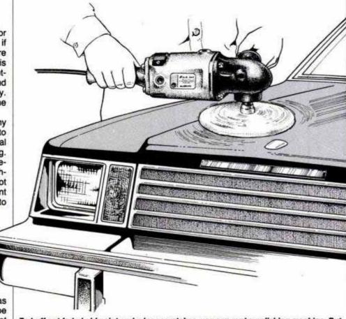
To buff out faded old paint and minor scratches, you can rent a polishing machine. But be extremely careful how you use it—any mistakes can burn right through the paint.
