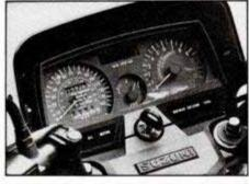
instrument panel is stylish and functional. A digital readout on the panel lets you know which gear the six-speed tranny is in.
