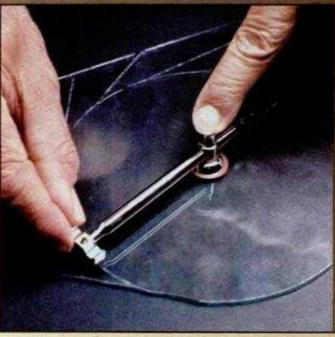
The circle glass cutter cuts up to 10%-in.-dia. disks for picture frames, mirrors, clocks and flashlights. Hold the rubber pivot firmly in the center of the glass and rotate the cutter head in a circle. Next, adjust the cutter head for straight cuts and make tangential cuts from the circle to the edge of the glass. Break off the pieces formed and you have a perfect glass disk. The cutter, which costs \$11.40 postpaid from Brookstone, comes with three spare cutting wheels and a screwdriver.
