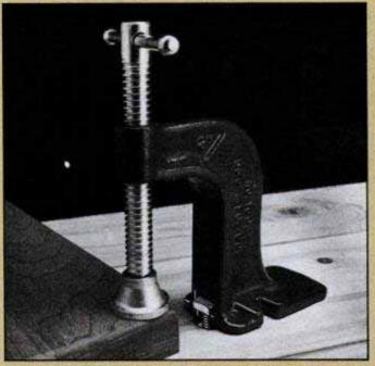
You can install this handy hold-down clamp anywhere on your bench by simply boring and counterboring a hole and installing a hold-down bolt. The clamp sildes onto the bolt head ready to secure work that's up to 3 in. thick. The clamp rotates 360° around the holding bolt to secure work at the right spot or easiest angle for the hobbyist. When it's no longer needed, remove the clamp and let the hold-down bolt drop down out of the way. The hold-down clamp is \$11.95 from Leichtung.
