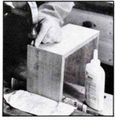
To prevent the glued surfaces from sliding out of position, you should prebore holes before nailing. Take care not to use any nails near the diagonal cutline which divides the box into top and bottom.
