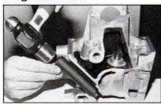
After reaming out damaged sparkplug hole threads, hammer in insert with special tool.
