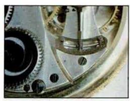
Detailed close-up inside a pocket watch is the type of shot possible with a macro lens. This was taken with a macro adjusted to maximum extension for a 1:1 ratio. Images on film are the same size as the subject.
