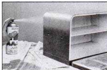
5 A sure way to get a professional-looking surface: First apply quality primer like Plasti-Kote, used here.
