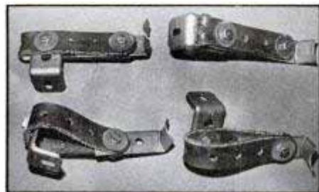
Semi-universal exhaust hanger can be assembled in a number of different ways.
