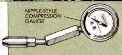
Most basic way of checking cylinder pressure is with a compression gauge, available in two basic types. Gauge attached to the plug port has a hose that screws into plug threads. Gauge at right has rubber nipple that's held against plug hole to get a reading.
