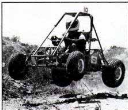
Off-roader powered by 8-hp Briggs & Stratton engine flies during Mini-Baja.
