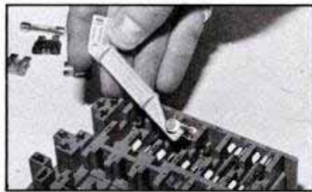
Unhook one end of a cylindrical fuse with the tool. Then pull with your fingers.
