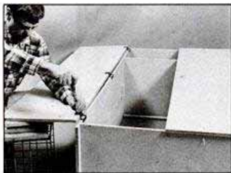
Assembling the particleboard cabinet took about 30 minutes. Note the door support while the hinges are installed.
