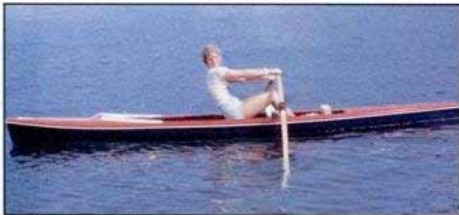
Alden's 16-foot Ocean Shell has a 25-inch beam. Like most recreational shells, it is made of fiberglass.
