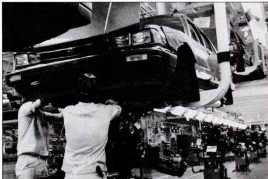
Bodies of Honda Accords meet drive trains on assembly line at Marysville, Ohio, plant.
