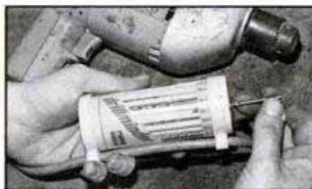
With the dispenser's top arrow at the desired size, the drill bit can slide out.
