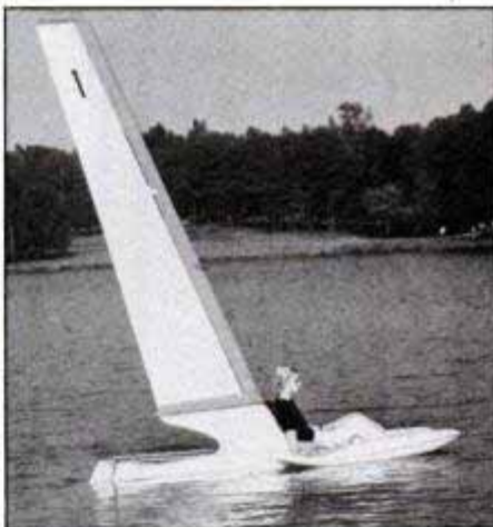
Wingsailer's 27-sq.-ft. wing weighs only 10 pounds. Craft has positive flotation, can be righted quickly in a tip-over.
