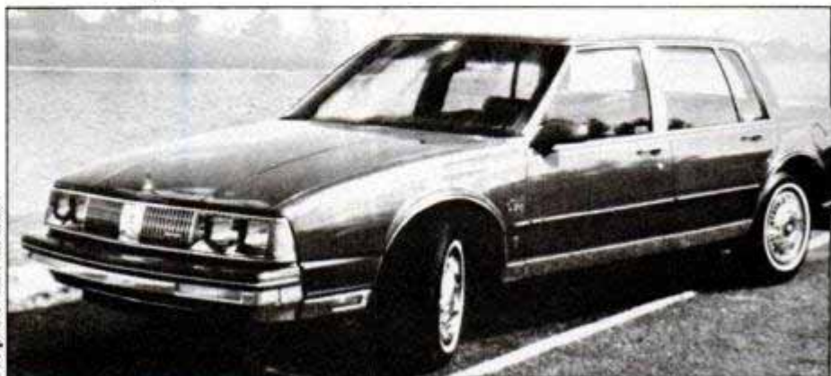
New fwd Olds 98 is 2 feet shorter, 600 pounds lighter than the rear-drive model.
