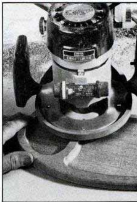
Make the final leveling passes with the router set for extremely shallow cuts.
