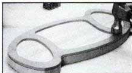
Nail the candy tray's surface carving template to the workpiece's underside.
