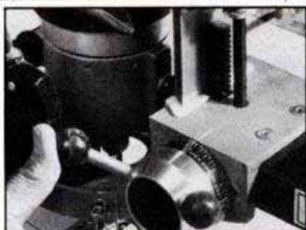
The depth-indicator scale is ruled in \frac{1}{32} -in. increments to give fine adjustments.
