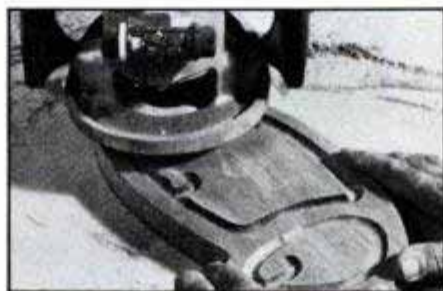
Keep the guide pin against the template cutout's inside edge to groove the perimeters of each candy tray compartment.
