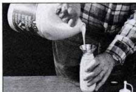
Glue pot was purchased in a housewares store. It's actually a mustard dispenser. Small funnel guides the glue in.
