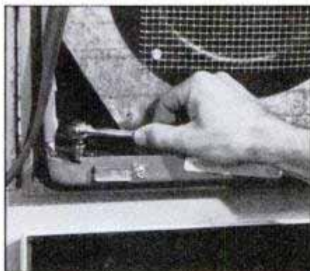
Replace chassis-securing screws that were removed so case could be installed.
