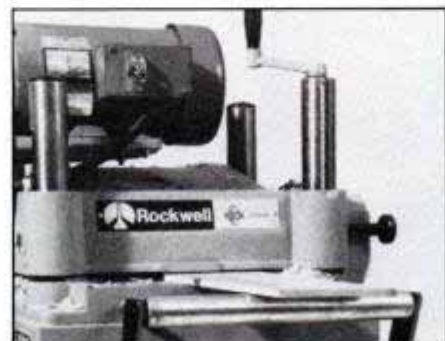
Infeed support is via a single roller held at the same elevation as RC-33's bed.
