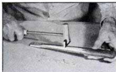
Scraper hammer's beveled file section is used for smoothing rough hardwoods.
