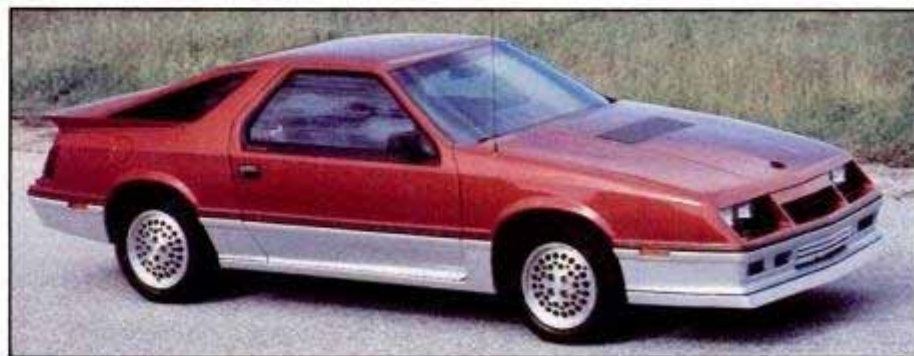
Turbocharged versions have vent in low-pressure area of hood to expel hot gases.
