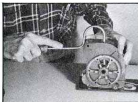
Use the question-mark hammer in spots where other hammers can't fit or reach.
