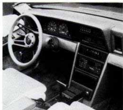
Chrysler has gone the complete electronics route with dashboard and most instruments. Synthesized voice has 15-second delay.
