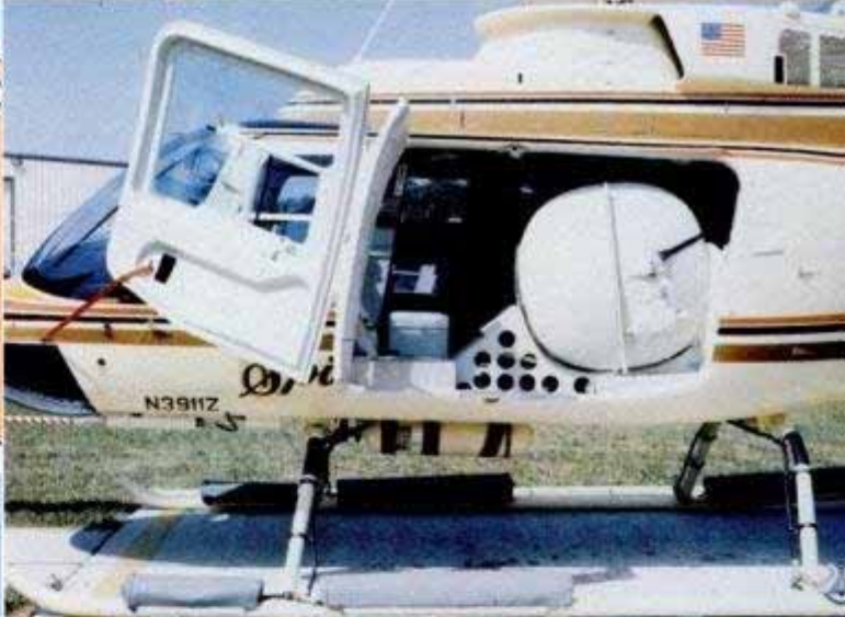
Rear seat of the Bell chopper was removed to make room for an auxiliary fuel tank (above). Some of the advanced electronics gear was also stowed in the rear section.
