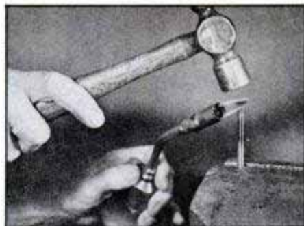
Use torch, ball-peen hammer to form question-mark hammer's striking end.
