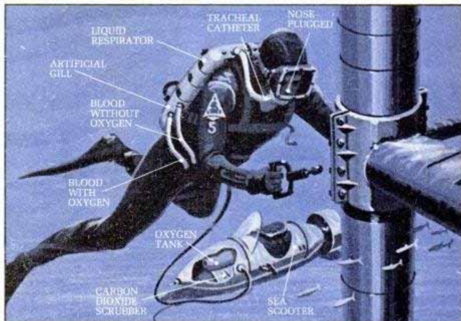
With the artificial gill system, oxygen-rich fluorocarbon is pumped into the lungs by a liquid respirator. Extra oxygen is supplied to the blood through tubes in the diver's groin.
