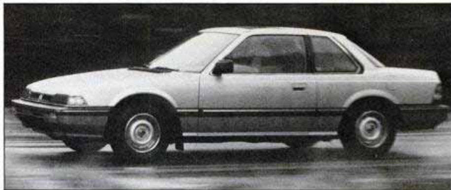
The .36 drag coefficient results in low wind noise and wind resistance at speed.
