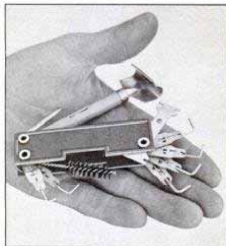
Ignition maintenance tool can even check for electrical leaks in spark system.
