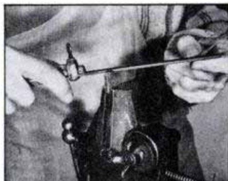
File the beveled edge onto the scraper using a flat file. Be sure to anneal the section of file used as the scraper.
