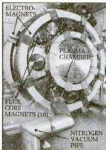
Spheromak, the economy fusion reactor, has smaller magnets, fusion chamber, vacuum system.
