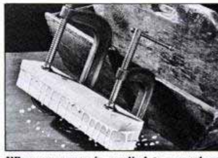
When pressure is applied to overglued pieces, squeeze-out will occur. This has ruined the appearance of many projects.
