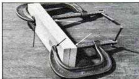
Clamp boards immediately and keep the joint under pressure for at least 24 hours. If workpiece surfaces will show, scraps of wood (pads) should be inserted between the clamp pads and workpiece (arrows).
