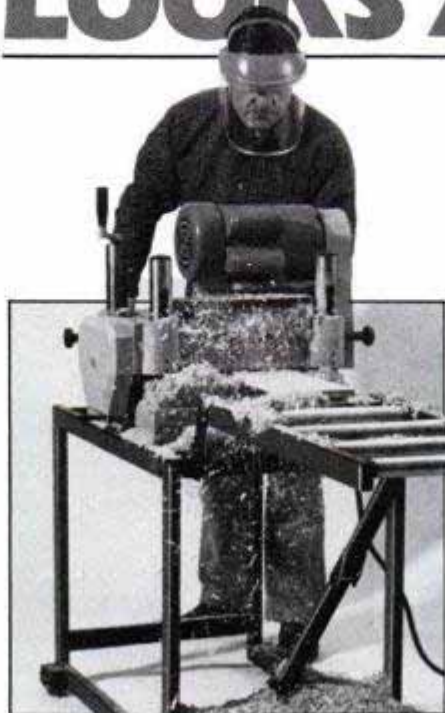
Mobile stand sets planer bed at correct working height, 33 in. from the floor.
