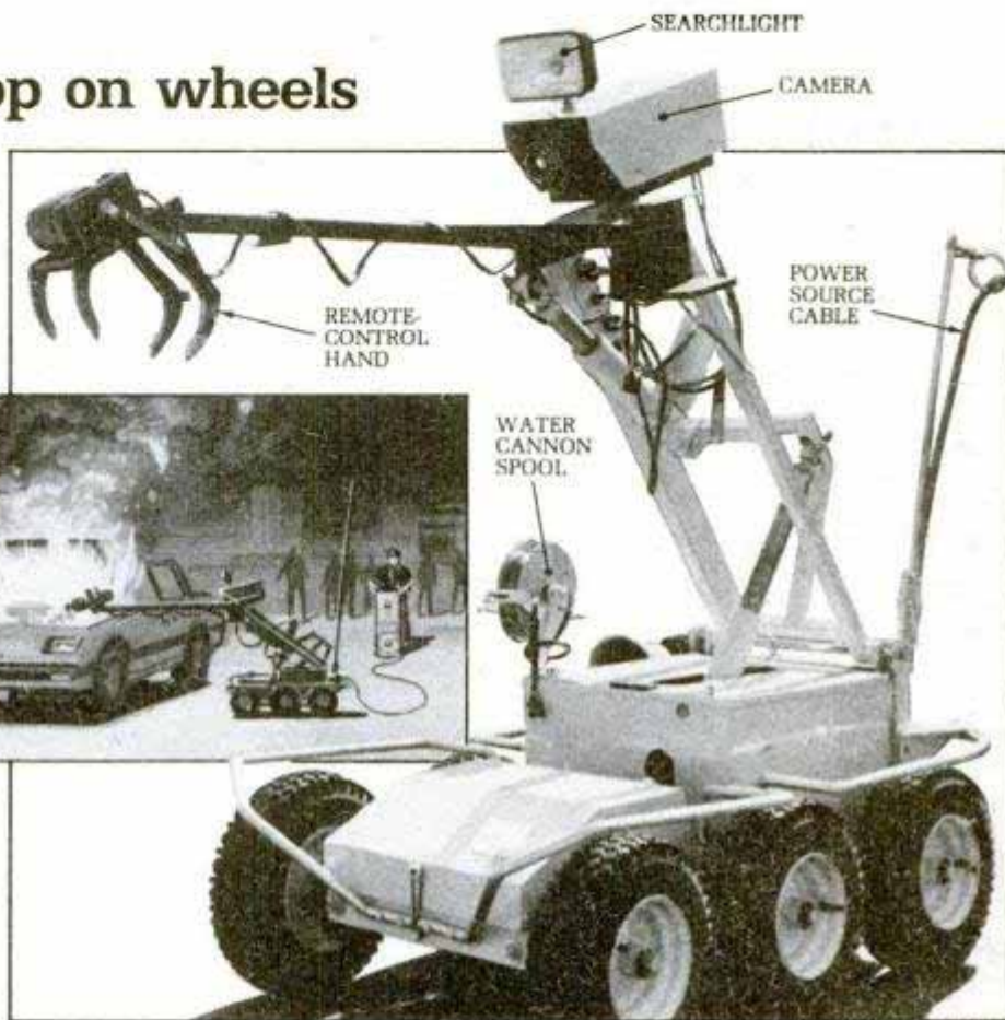
PM photo: Steve Eskow Pedesco Mark-3 unit can pick up bombs with its robot arm or handle a hose to put out auto fires. The $20,000 remote-controlled device has television eyes and a searchlight.
