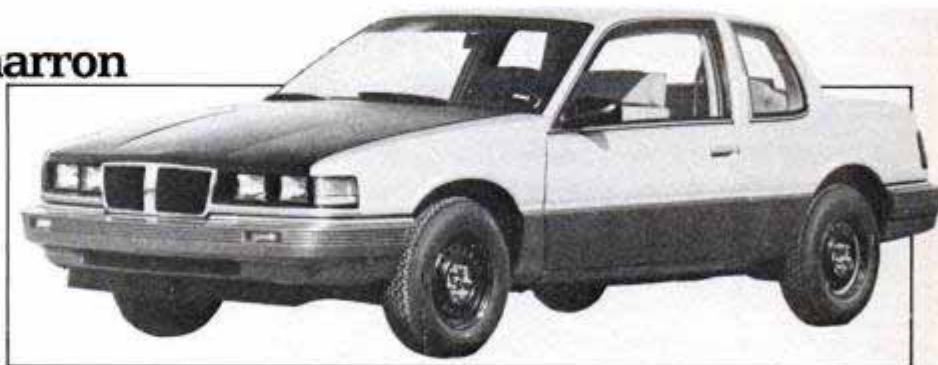
The '85 N-cars will be built on a stretched J-car platform with 103-in. wheelbase.
