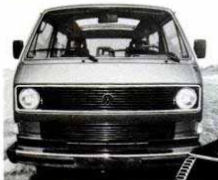
Volkswagen's Vanagon has been updated this year with a water-cooled, flat Four motor. Engine remains in the rear with radiator and plumbing forward (right).
