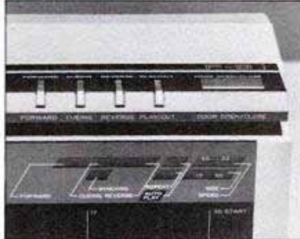
Interior view of Mitsubishi's LT-10V (top) shows linear-tracking stylus nestled in turntable's "jaws." Control panel of Kenwood P-9 (bottom) has touch-sensitive switches for all functions.
