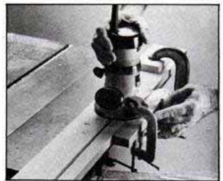
Use a V-groove router bit to bevel paper slot edges. A wood block clamped to base accurately guides the router.
