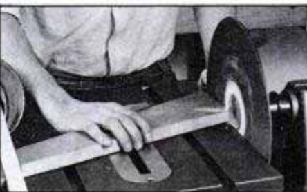
As a disc sander the multi-tool excels. Here, a splayed leg is held against fence and in a jig, while control (arrow) advances the spinning disc. Such capability is handy for production-type work—like sanding four legs to the exact same length.
