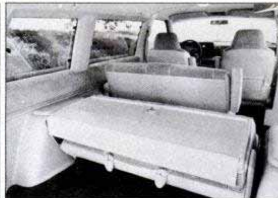
Because of its front-wheel-drive arrangement, Chrysler T-van has a flat cargo floor. The sliding side door makes entry and exit a good deal easier. The van will have a variety of seating arrangements and will be able to carry as many as seven people.
