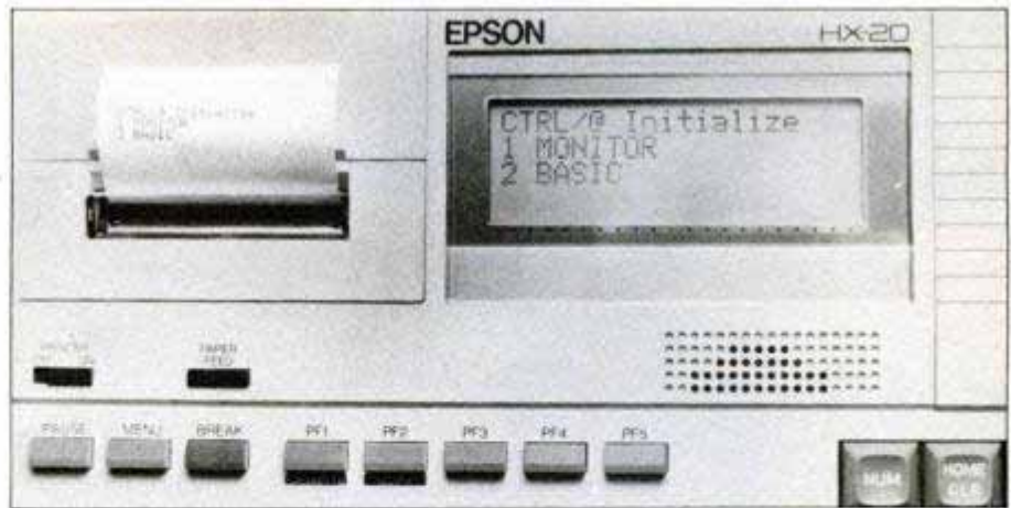
Epson HX-20 is an attaché-case-sized computer with features such as a built-in LOD display, a printer and a row of user-defined function keys, all shown above.
