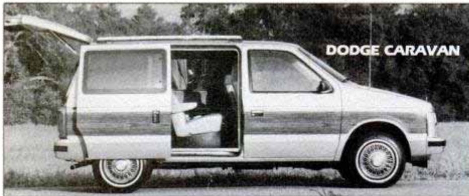
Because of its front-wheel-drive arrangement, Chrysler T-van has a flat cargo floor. The sliding side door makes entry and exit a good deal easier. The van will have a variety of seating arrangements and will be able to carry as many as seven people.
