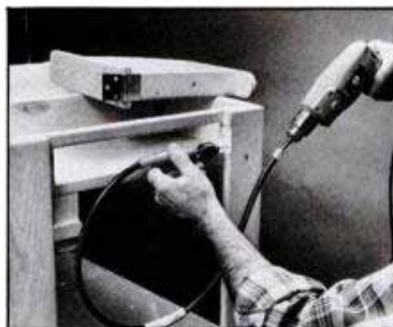
Use a flexible drill-shaft accessory in order to bore pilot holes in tight spots.
