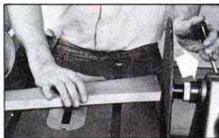
As a disc sander the multi-tool excels. Here, a splayed leg is held against fence and in a jig, while control (arrow) advances the spinning disc. Such capability is handy for production-type work—like sanding four legs to the exact same length.
