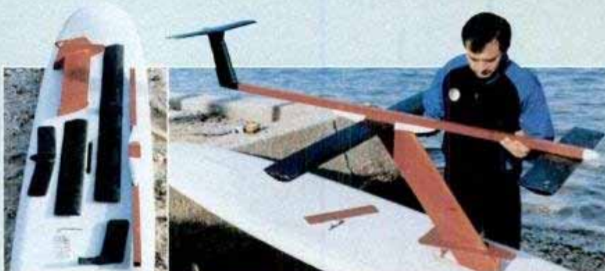
When disassembled (left), Aquafoil is entirely portable and can be transported to the surf on a car roof. Assembly (right) can be completed in three minutes.
