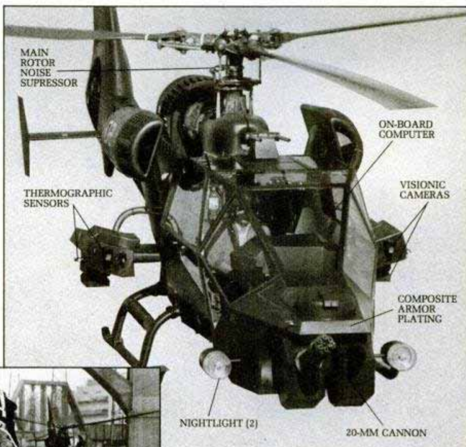
Blue Thunder (above) is a French Aerospatiale Gazelle with composite metal plating, a 20-mm cannon and sensors that see through walls. It was built for a new Columbia film and is seen in low-level flight (left).
