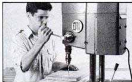
After the table saw, the vertical drill press is the biggest shop need. The first chuck that we tried wobbled.
