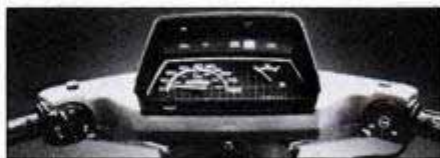
Start button, front brake lever and slick instrumentation are on the handlebars.
