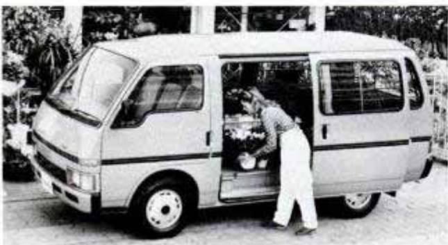
The Isuzu Fargo currently is sold only in Japan and some Asian countries. It is rear-wheel drive and powered by a 2.0-liter diesel or a gasoline engine.
