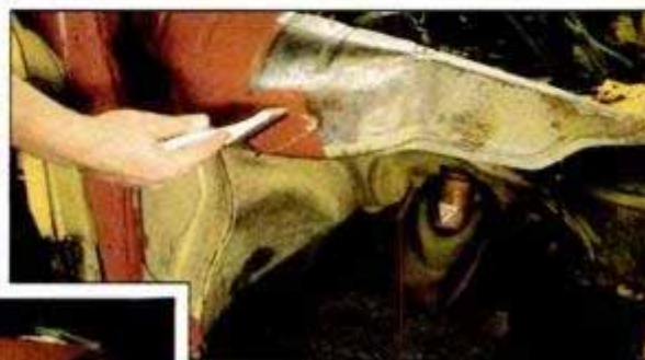
Degrease surface with good solvent (top). Once surface is dry and clean, apply two coats of red metal primer (above). When primer is dry (left), you apply top coat of thick rustproofing material.
