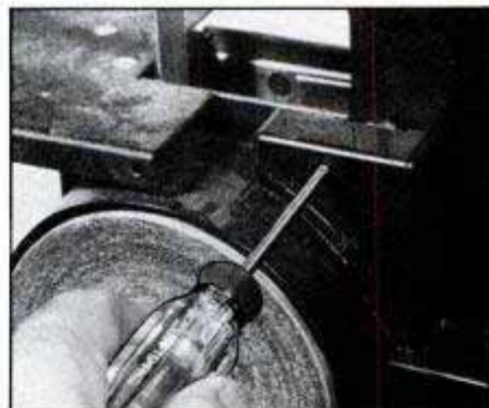
The belt tracking adjustment on the Dremel unit is located within the housing.
