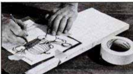
Design is taped to the wood with carbon below, transferred using ballpoint pen.
