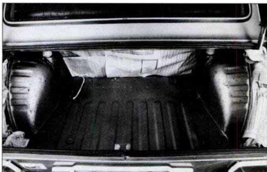
Before you apply paint to the trunk of your car, mask off everything you don't want coated. Make certain that the surface that you are painting is dry and free of oil.
