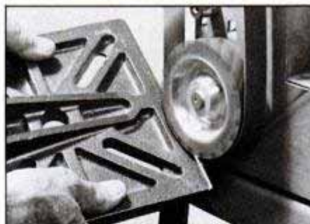
Use the rubber contact wheel with a coarse belt for aggressive, fast stock removal, descaling and deburring.
