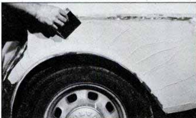
With a picking hammer, gently bang down high spots and remove any slag (above, left). Grind down high spots on weld bead (above) and remove rest of paint from around panel. Mix body filler and apply thin, even layers (left).
