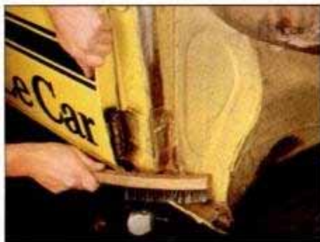
The wire brush will usually be enough to get down to the bare metal. It will reach places the gasket scraper can't get.
