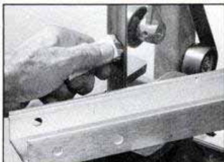
When grinding a nonferrous metal like aluminum, apply a low-melting-point grease to the belt to prevent clogging.
