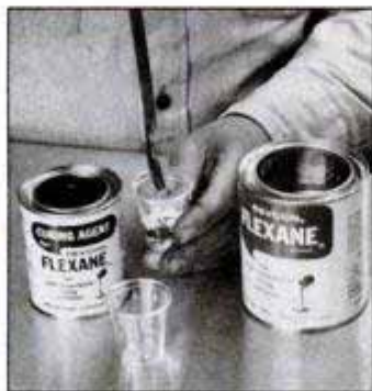
Mix only enough urethane for job at hand. Read instructions carefully so that you mix the proper ratio of catalyst.
