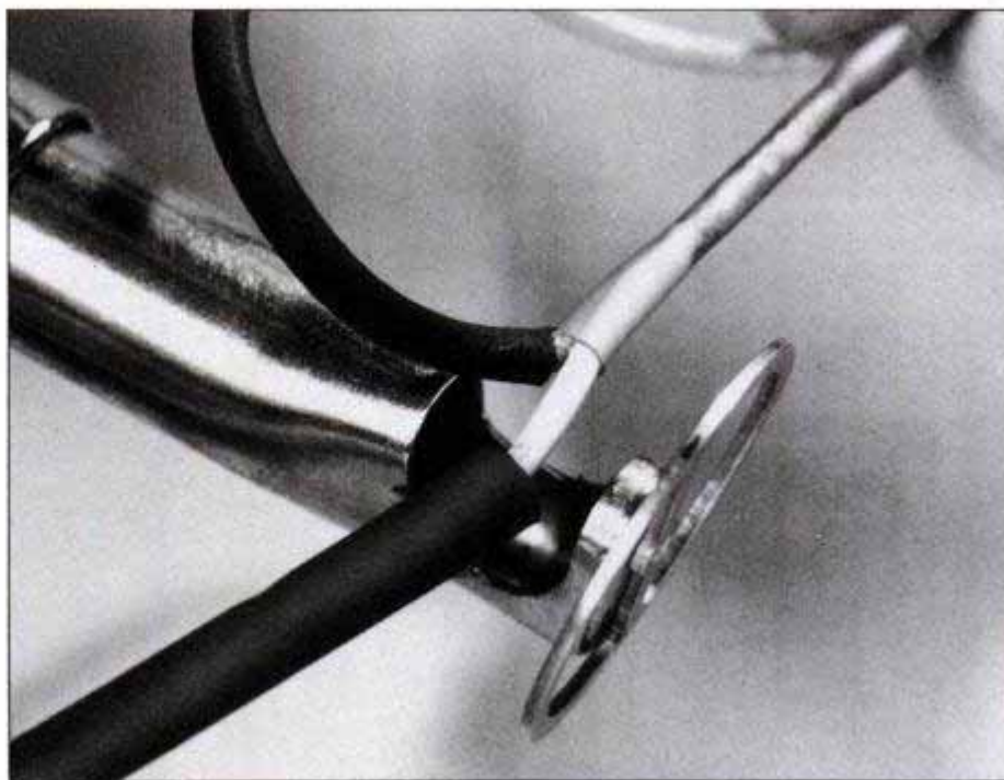
The recommended method for insulating a Y-type connection is to use the heat gun to shrink two legs of the Y, which have been fitted with the appropriately sized tubing.
