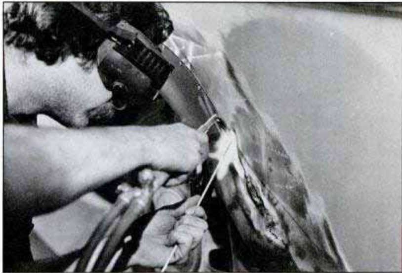
Braze the replacement panel in place with a gas welder and a bronze rod. Don't hold flame on one spot for too long or the metal may become warped.
