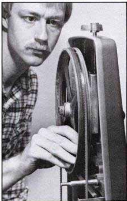
Check blade tracking to be sure it rides at center of both wheels. If not, adjust tilt to get blade running correctly.
