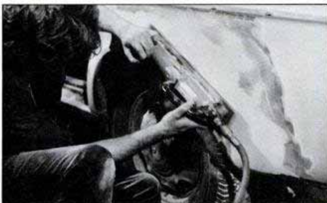
With a power sander or a hand sanding block, sand down the body filler. The edges of the filler should be very, very thin and blend almost inconspicuously with paint at the border.
