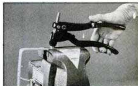
Rivet tool can install a threaded rivet as well as conventional blind rivets.
