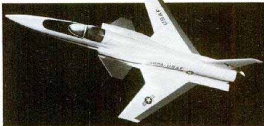
Grumman's X-29 forward-swept-wing jet receives extra lift and fuel efficiency from the craft's odd configuration. A canard stabilizer is mounted forward of the wing.
