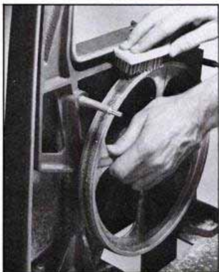
Clean the tires on band saw wheels with a stiff brush. If they're scored, dress surface with coarse sandpaper. If tires are overstretched, replace them.
