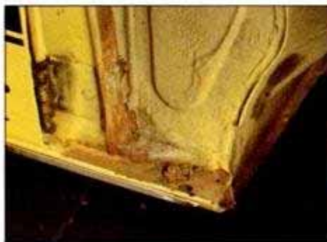
Rust forms where water collects, as here between the fender and body. After three winters, this car was ready for repair.
