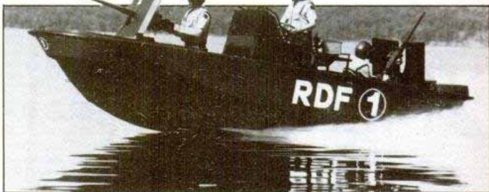
The Raider combines the unsinkable hull of a Whaler with the firepower of 12.7-mm machine guns.
