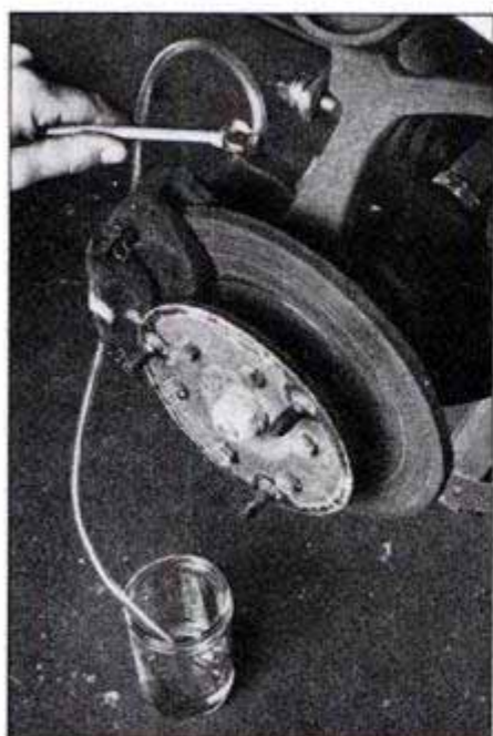
To install silicone fluid, purge the brake system of existing glycol fluid and refill.
