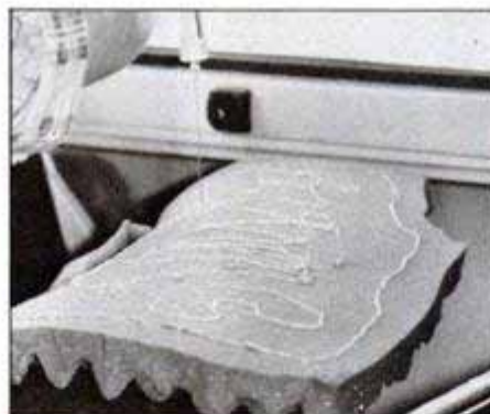
Apply glue to the foam as well as to car's metal surfaces. Let the glue get tacky before installing the foam sheet.
