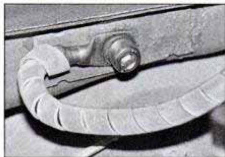
This battery ground cable is protected with spiral wrap, installed with stainless.
