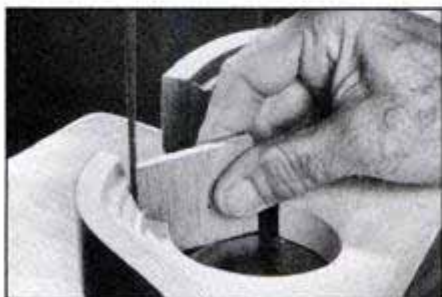
For sanding the most intricate details, guide the narrow belt with a thin wood block. You can make custom-shaped blocks for sanding specific contours.
