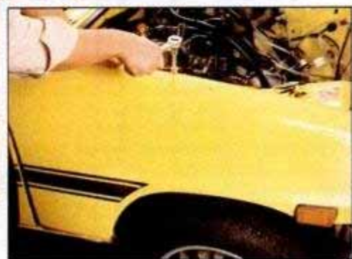
Total rustproofing can be a one-weekend home garage project. Metal primer and a rustproofing compound are all you will need. Removable fenders (right) make it easier.
