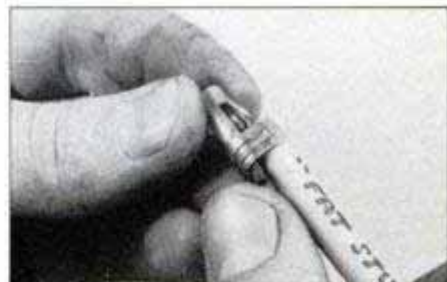
Bend the wire back over the insulation and gently crimp the connector over the wire with a pair of pliers.
