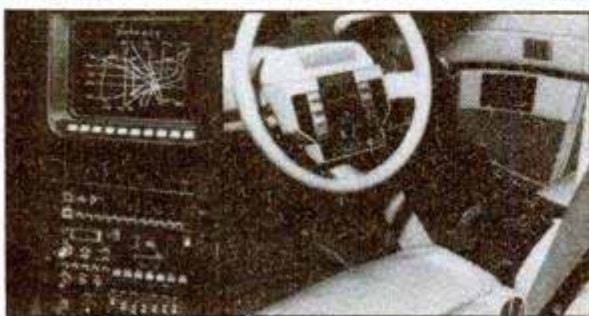
Electronics in Buick Questor include computer screen (left), to pick up satellite maps, and column controls (right).
