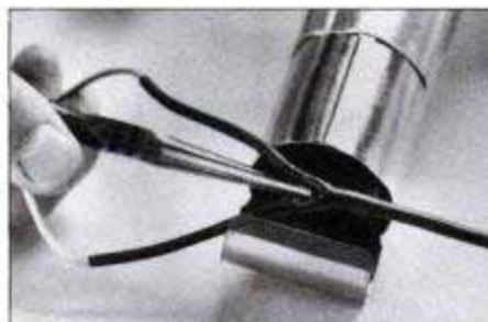
While the tubing is still soft from heat, spread the legs and crimp the tubing in the middle with needle-nose pliers.
