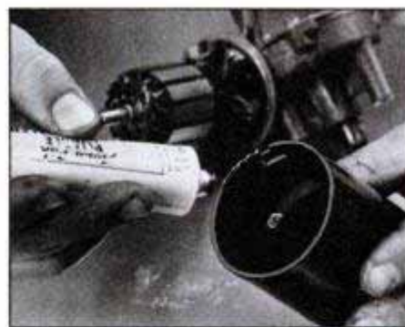
This electric motor housing didn't have a gasket. The poor seal let in dirt. A gasket was made with gasket material.
