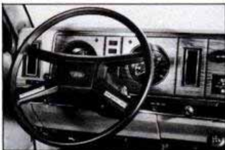
Placing horn switch at the end of turn-signal stalk brought some complaints.
