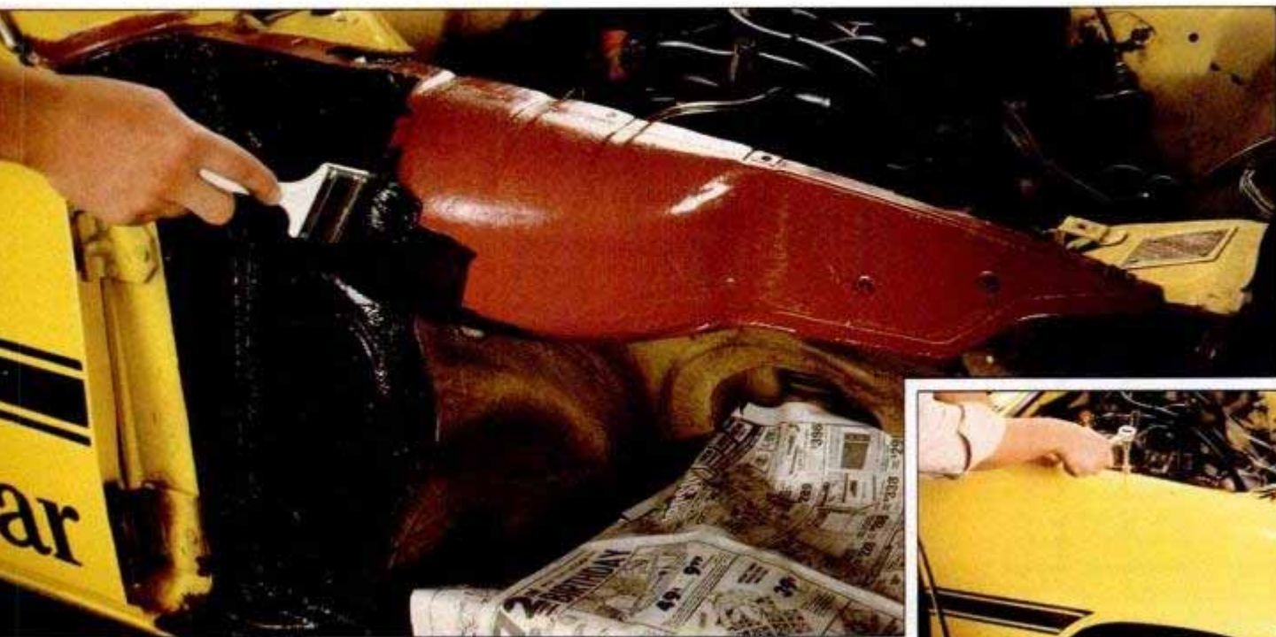
Total rustproofing can be a one-weekend home garage project. Metal primer and a rustproofing compound are all you will need. Removable fenders (right) make it easier.
