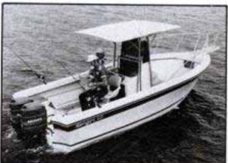
Ranger's 622, an offshore 22-footer with deep-V hull, high freeboard, pulpit and console, takes twin 115-hp Mercs.
