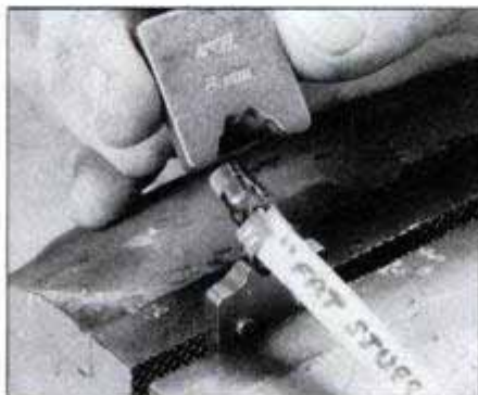
Start by placing the lower half of the crimping tool in a vise and then insert the connector carefully into the tool.
