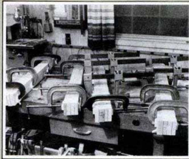
Chances are that you won't be able to buy 4x4 oak stock locally. Consequently, legs are made of glued-up 1-in. boards.
