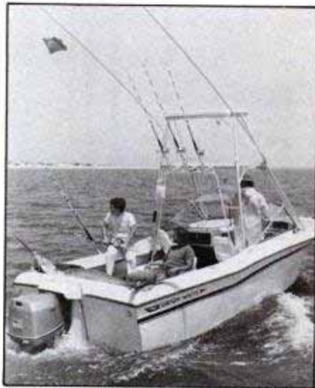
Rigged like a 40-footer, Grady-White's 22-foot Tournament Dual Console has a tuna tower, outriggers, Sea Drive.
