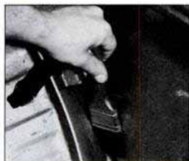
Water infiltration on this car was a direct result of a small leak in the vehicle's weatherstripping. The water settled in the hollows (above, left) and also directly below the leak on the wheel well (left). After cleaning off the rust, you should apply a metal primer and let it ooze into all of the car's cavities (above).
