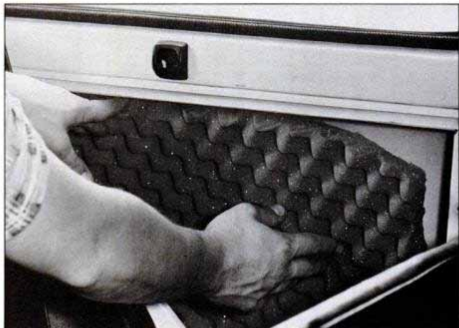
Dense foam rubber sheets that are glued to the bulkheads in your car will cut down on the noise level of the vehicle. The foam should resist heat up to at least 220° F. You may find it necessary to reroute speaker or harness wires.
