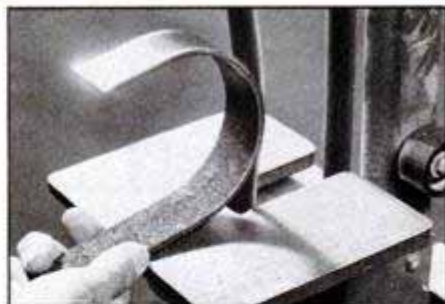
The brushing/cleaning belt—a nylon web impregnated with abrasives—can remove rust or clean plastics and glass.
