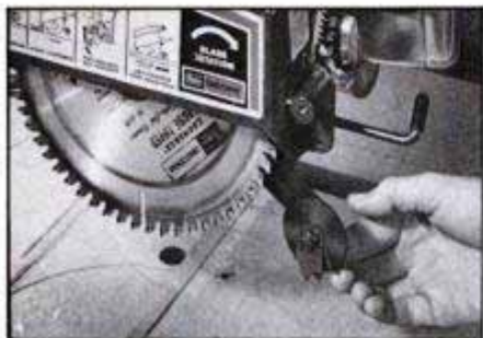
Keep pawls clean; points must be sharp.
