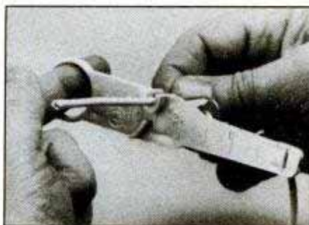
A wire stripper tool, available from the phone company, is a handy device. The tool, which has a built-in measuring scale, allows you to strip a multiconductor cable without damaging the wires. Afterward, you can use it for other jobs.
