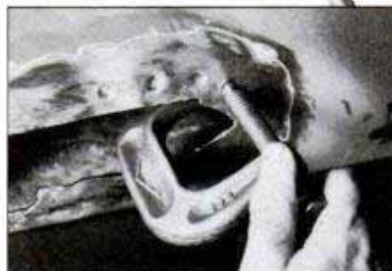
Make dimples around the perimeter of the hole with tool. Space them 2 inches apart and an inch in from the edge.
