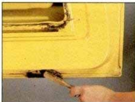
Drain holes in doors are prone to clogging. Use the spray-type rustproof coating with the extension nozzle for treating hollow, inaccessible body cavities.
