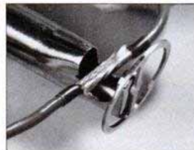
Solder-Sleeve comes in a variety of sizes that fits any automotive application. To install, strip the wires and insert them into the tube. Make sure the wires overlap and that the solder ring is located in the middle of the overlapped wires.
