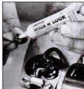
Use a locking compound on fasteners when reassembling unit. Vibration can cause fasteners to work loose.
