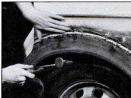
Braze the replacement panel in place with a gas welder and a bronze rod. Don't hold flame on one spot for too long or the metal may become warped.
