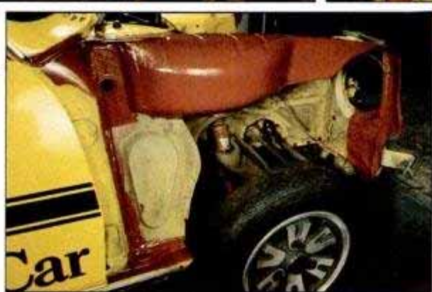
Degrease surface with good solvent (top). Once surface is dry and clean, apply two coats of red metal primer (above). When primer is dry (left), you apply top coat of thick rustproofing material.
