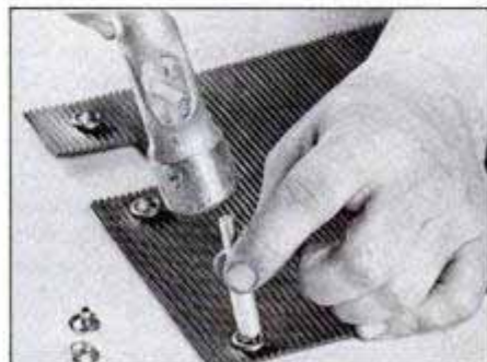
To make a boot, lay the coil on a sheet of foam, cut it to size and install snaps (above). Leave a notch in the boot to clear the coil-mounting bracket.
