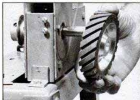
When you use Rockwell's contact wheel, position the machine to extreme right-hand side of bench for easy access.
