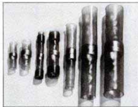
Solder-Sleeve comes in a variety of sizes that fits any automotive application. To install, strip the wires and insert them into the tube. Make sure the wires overlap and that the solder ring is located in the middle of the overlapped wires.
