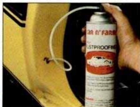
Drain holes in doors are prone to clogging. Use the spray-type rustproof coating with the extension nozzle for treating hollow, inaccessible body cavities.
