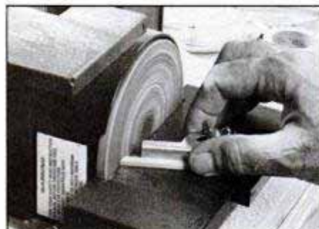
The disc sanders available on the Dremel and Craftsman models are useful for sanding particularly small workpieces.
