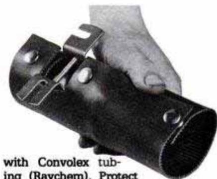
To make a boot, lay the coil on a sheet of foam, cut it to size and install snaps (above). Leave a notch in the boot to clear the coil-mounting bracket.
