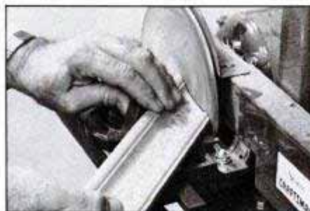
Obtaining precise angles is easily handled on the disc sander. The cast aluminum table with the miter gauge tilts to allow for bevel sanding and grinding.
