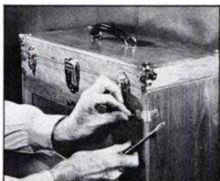
Corners conceal the screws which are used to hold the top compartment together.
