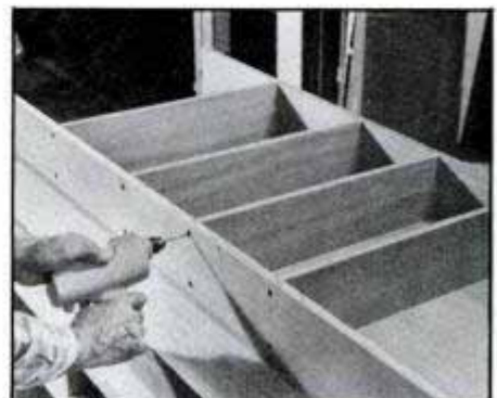
The pilot holes are bored into the shelf ends after the plug and pilot holes have been bored in the side pieces.
