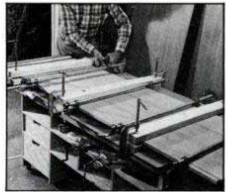
Light pressure on C-clamps holds the boards flat. Tighten up on the bar clamps to draw the edge-joints closed.
