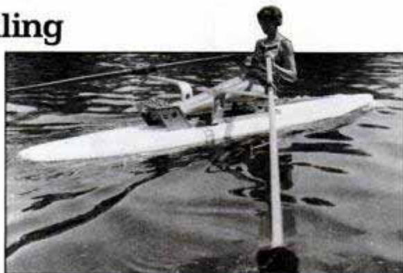
Any sailboard is turned into a rowing shell by adding a sliding-seat Oarmaster, a rig from Martin Marine.
