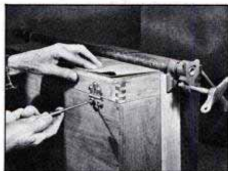
Install hinges with the lid clamped in position. Pipe clamps with wood blocks ensure proper alignment.
