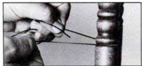
Round abrasive cords quickly smooth areas like the fine grooves in spindles.
