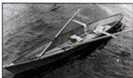
The Oarmaster can also be mounted in a Kittery Skiff. This Martin Marine kit boat has curved ends for a smooth ride.
