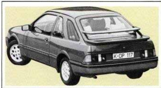
XR-4 has biplane rear spoiler, which lowers Cd from .34 to .32.
