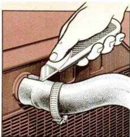
To remove a stubborn hose, slit it with a blade. Take care not to gouge connector.
