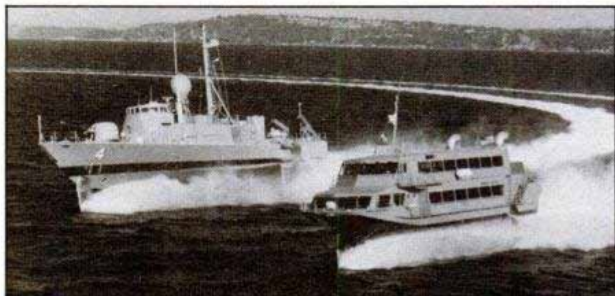
Hydrofoils for peace or war: Boeing's passenger-carrying civilian ferry (right) teams up with Navy's new missile-firing PHM version (left), both high-speed, foil-borne vessels.
