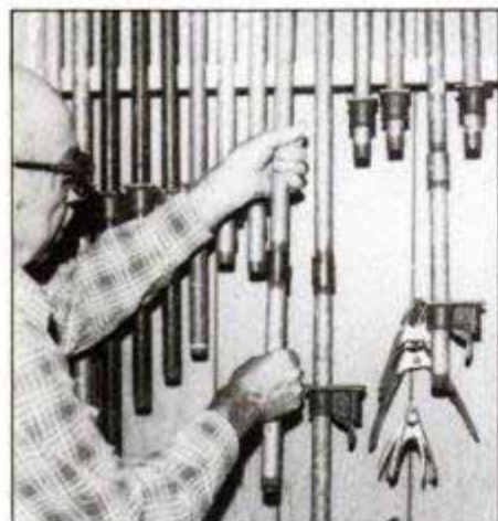
Lengthen your pipe clamps to suit any job. Add the desired length extension to clamp with a standard pipe coupling.
