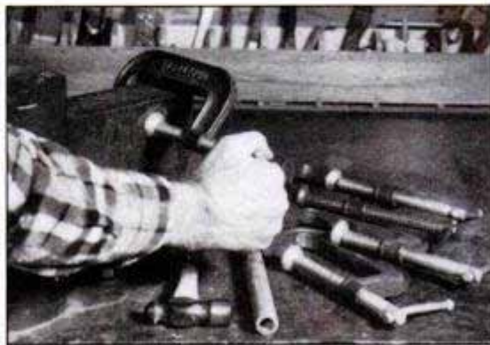
Strike the screw shaft to peen the end over (left). Hold the swivel pad in place and tighten the clamp to drive the peened shaft into the collar of the pad (right).
