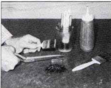
Make glue spreaders from nylon brushes (left). Cut bristles down to 1 in. long (right).
