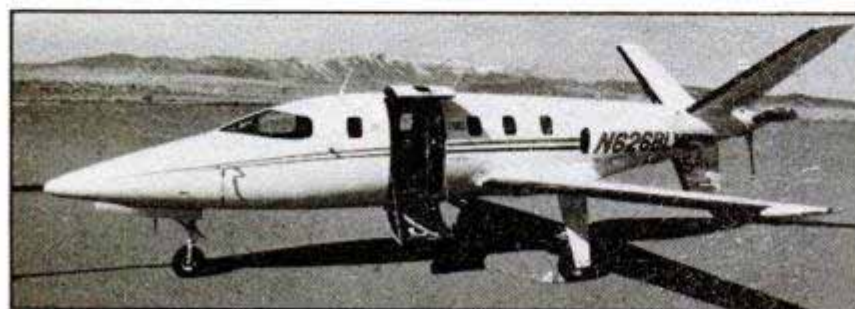
New high-speed, turboprop Lear Fan has unusual Y-tail, is undergoing flight tests.
