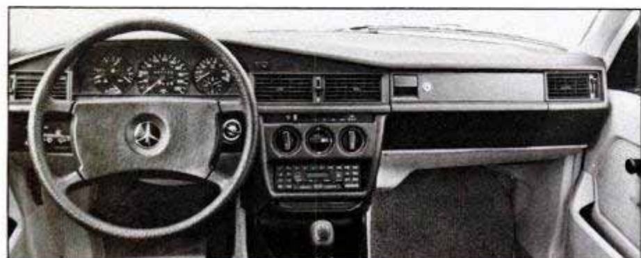
Instruments and controls are perfectly placed, right down to the glovebox latch, which is asymmetrically located in order to be as close as possible to the driver.
