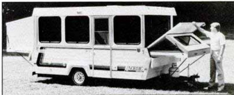
Hardwall Nordic camping trailer, new from Viking RV division of Coachmen, can sleep up to eight and opens from a 16½-foot road trailer to a 20-foot camper with a pushbutton electric lift system for quick setup.
