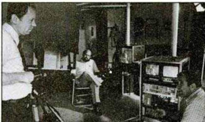
In recording, twin-screen monitor (right) shows two images before encoding. Combined, they appear as one on single monitor (rear).
