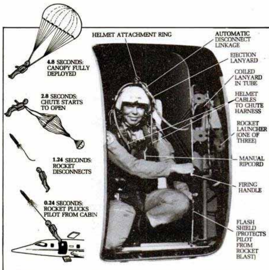
Pilot of disabled airliner crouches in doorway just before pulling emergency ejection handle. Sequence at left shows how rocket plucks him safely clear of craft so chute won't foul.
