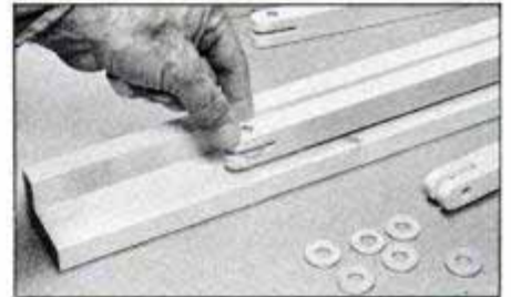
Fit end of connector over the pivot while slipping a washer into place in the slot.
