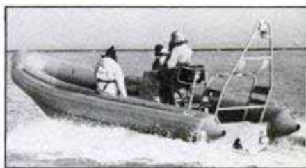
Avon's new Searider 7.4 is a combination hard-soft hull with advantages of both.
