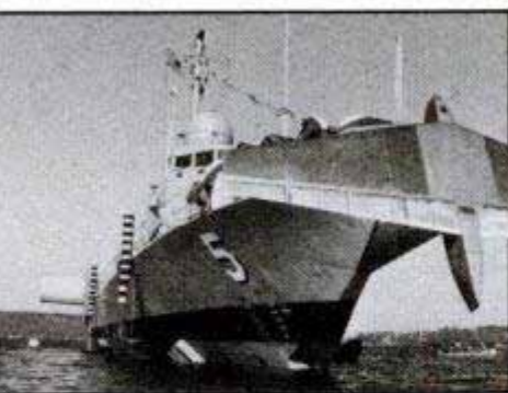
Large winglike bow foil, retracted above, swings up on pivoted strut for low-speed maneuvering, docking.
