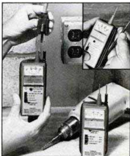
Snap-in probe and 3-ft. probe lead are convenient for various electrical tests.
