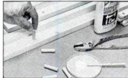
Crimp one end of dowel pivot pins with pliers and glue them in holes in plates.
