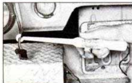
Hook at end of new tester makes it easy to grab wires when testing for continuity.
