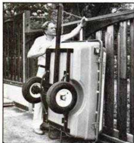
Coleman's compact utility trailer, named the Caboose, can stow on end in little space. Other mini-models include PackHorse II and multipurpose VersaTrailer.
