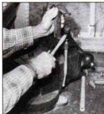
Strike the screw shaft to peen the end over (left). Hold the swivel pad in place and tighten the clamp to drive the peened shaft into the collar of the pad (right).
