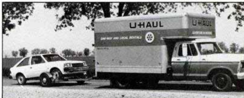
With 50 percent of new cars being made with front-wheel drive, U-Haul dealers are providing a rental tow-dolly for trailing a car behind your truck or motorhome. The dolly acts as a substitute front axle.
