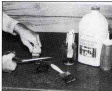
Make glue spreaders from nylon brushes (left). Cut bristles down to 1 in. long (right).
