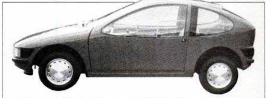
This tiny vehicle is a serious study of the possible transportation modules of the future. Lightweight materials and small motor will yield near-100-mpg efficiency.
