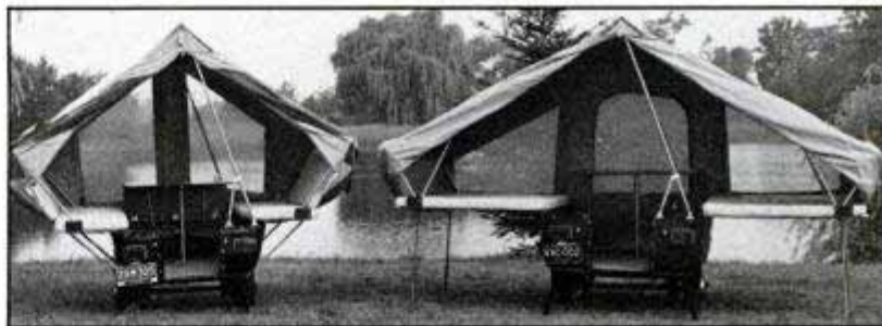
Even a motorcycle couple can tow a two-bunk trailer (left) from Continental Industries, Davison, Mich. The larger Travelite model (right) sleeps four and can be towed by compact cars. Both open for 6½-foot headroom.
