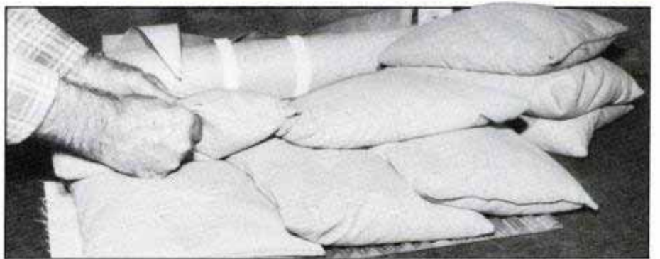
Gluing uneven projects, such as this tambour door, is easy with several sandbags.
