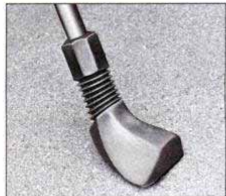
Plastic boot increases contact patch of a kickstand to keep bike from tipping.
