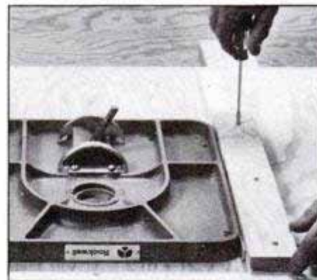
Saw table is removed to install hardwood track runners accurately. Rabbits cut in the runners allow some play, but shoudders fit snug against the track.
