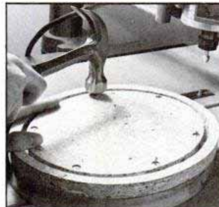
To work with a pin router, prepare a jig and nail it to the frame through six evenly spaced, counterbored pilot holes.
