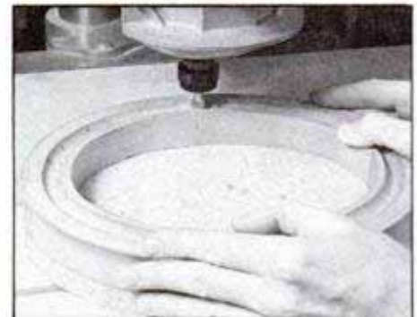
With the frame attached to the jig, flip the piece over and set the groove over the pin in the table. The router bit should be centered over the pin. Rotate the work, guiding it carefully with the pin in the groove to shape the frame face.
