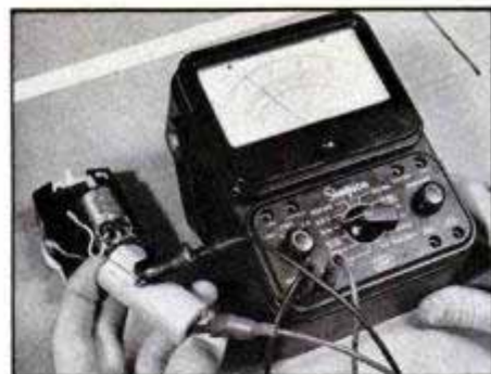
7 Remove the battery and test it with the voltmeter probes across its terminals.
