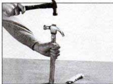
6 This type of replacement handle comes with two wedges. The wooden wedge is sliced to correct width, then tapped into the slit at handle's neck.
