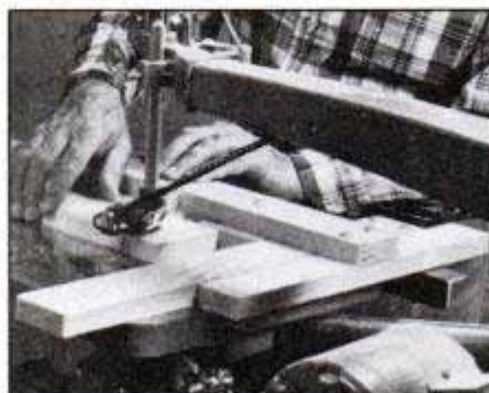
When cutting workpieces on saw table, cutoffs are limited to 3½-in. length.
