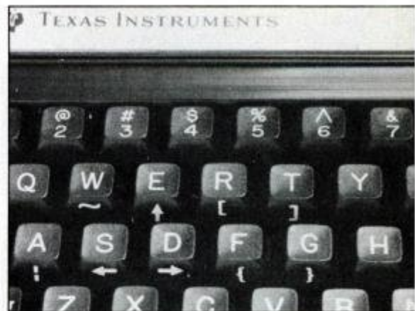
The Texas Instruments 99/4A (above) has a keyboard like a typewriter's; some of the keys control the direction of the entry cursor on the screen. A keyboard is very important—it's how a person "connects" to his computer. Be certain you'll be comfortable with your choice.
