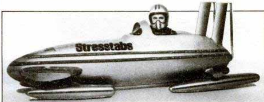
Kevlar bobsled, the first one to incorporate a roll bar, carries two in competition.
