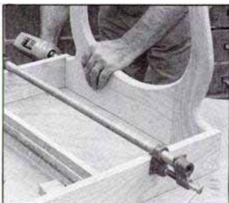
Hold the mirror yoke and side rails with clamps while boring pilot screw holes.
