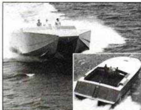
Cougar Marine's massive aluminum catamaran can top 55 mph with twin diesels.
