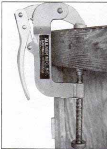
C-clamp with adjustable tension holds work firmly and maintains adjustment.
