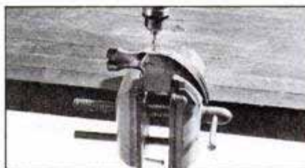
3 If portion of handle left in head's eye is difficult to remove, bore a series of 1/4-in.-dia. holes. Punch scrap out with sharp, narrow chisel and hammer.
