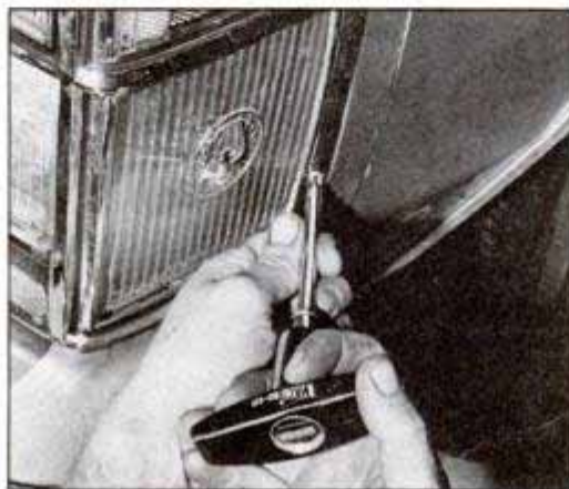
Heavy-duty ratchet screwdriver makes use of large assortment of shank types and sizes.
