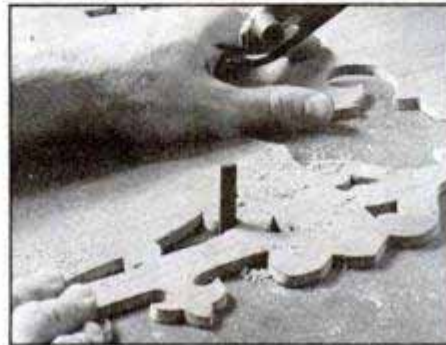
Use a fine jigsaw rasp to smooth the fretwork edges. For tight spots, use sandpaper glued to an ice cream stick.
