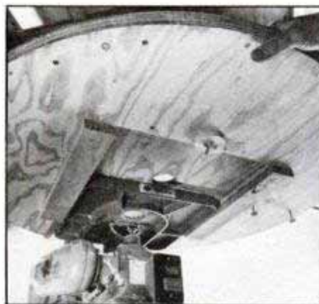
Underside view of the table as it slides into place. The eccentric cam is secured by a carriage bolt and wingnut.
