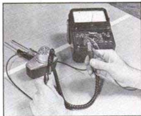
1 To test the line cord, place one probe of the continuity meter on the male prong, the other probe on the corresponding female end; test both wires.
