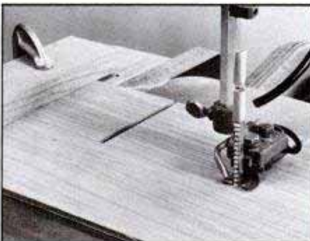
When workpieces extend beyond the table, clamp the guide block to the work so it rides against the angle-iron rail.
