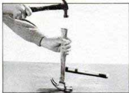
5 Tap in the replacement handle by putting old head upside down on a solid surface (workbench). Tap handle in until it is flush with hammerhead top.
