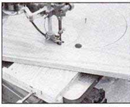
Cut a circle for the bowl with a scroll saw. Pivot the work on a nail driven into a board clamped to the table.
