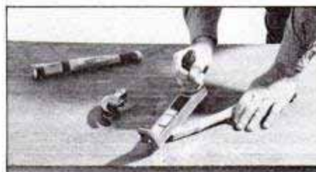
4 Replacement handle must be customized to fit hammerhead (handle is more or less universal size). Here, neck is planed both sides with a Surform rasp.
