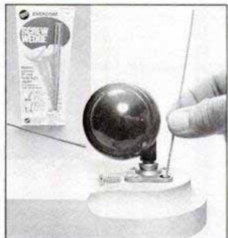
Screws once again fit tightly in enlarged holes when you use Screw Wedge (inset).
