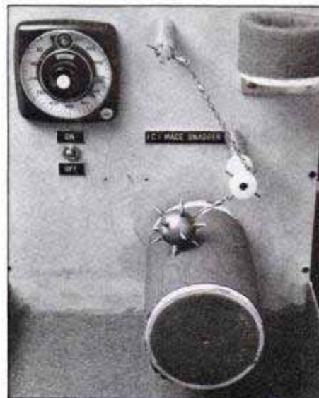
Mace snagger is used to test strength of space suits and other woven material.
