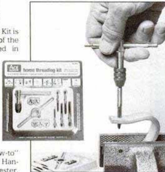
Chuck the desired size tap into wrench and cut bolt threads in prebored hole.
