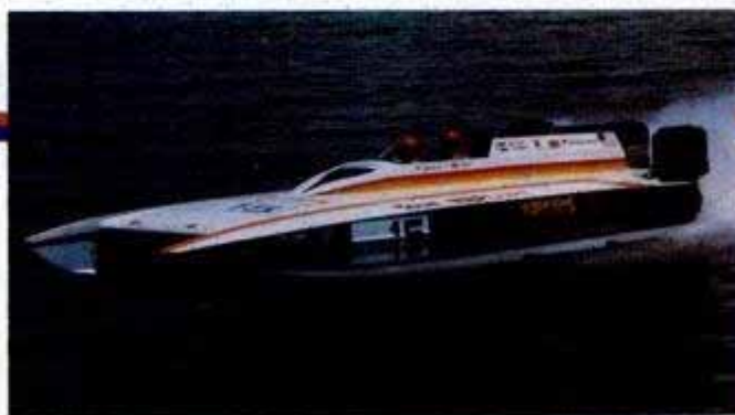
Catamaran-hulled "Popeyes" has been beating inboards in offshore racing with three of Mercury's 300 EFI outboards.
