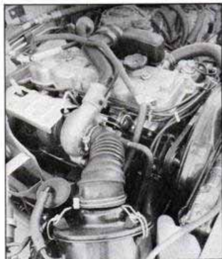
Starion (top) uses this 2.6-liter turbocharged Four, which delivers 145 hp.
