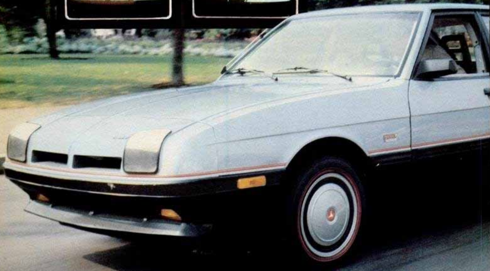
Government-sponsored Research Safety Vehicle has "friendly" fenders to protect pedestrians. It also has headlight covers which are recommended as a safety item by one branch of the DOT, but deemed illegal by another branch. Ford's CRT displays (inset, top) are in one of its experimental vehicles. Car functions are controlled by touching the screen. Map locator is hooked up to satellite. Arrow indicates your position.
