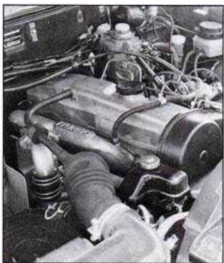
The 2.3-liter, turbocharged, four-cylinder oil-burner delivers an impressive 80 hp.
