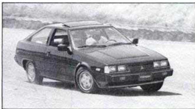
Fastback Cordia has a 1.8-liter motor which drives front wheels. The engine delivers a decent 82 hp and can be coupled to a manual four- or five-speed or to an automatic.
