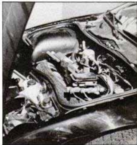
Spare tire, radiator and brakes live in the busy front compartment of the P-car.
