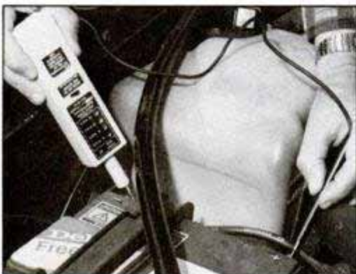
Smart Lite will perform efficient, quick voltage checks of your battery and charging system.
