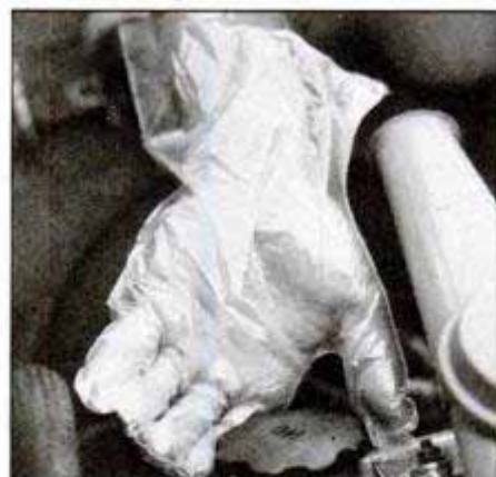
Thin plastic gloves keep hands clean, are cheap enough to throw out when used.
