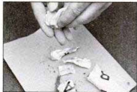
Two-part putty bonds to almost anything. It air cures or cures with heat gun.
