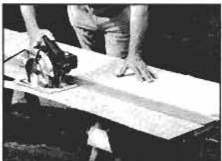
Guide saw against 3-in. strip to trim the base and set guide exactly for your saw.
