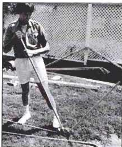
Shaping conduit into a custom curve is simple with standard pipe bender, gives rounded shapes that won't chafe cover.
