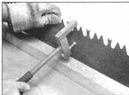
Stop screw on the setting tool lets you set the teeth uniformly and precisely.
