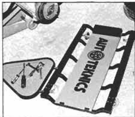
High-tech creeper has a metal frame, recessed wheels, removable tool tray.
