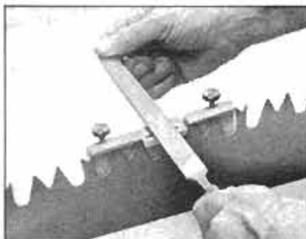
File raker projections flush with plate, then remove gauge and sharpen edges.
