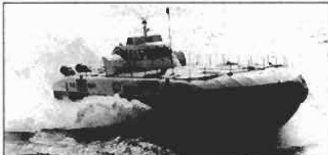
The U.S. Navy's air-cushion SES 100B skimming the waves at a blistering 105.7 mph—a record for military vessels.
