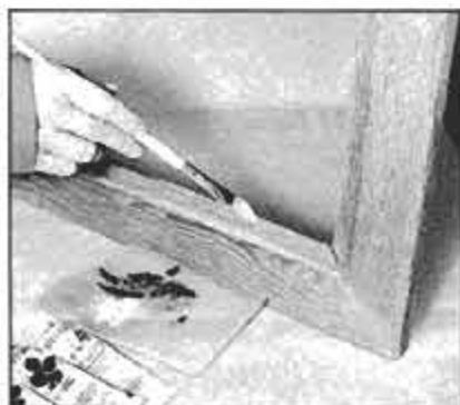
Paint newly cut edge to match frame's aged surface as closely as possible.
