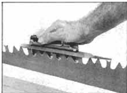
File cutting teeth to uniform arc by pushing tool opposite way from file tang.
