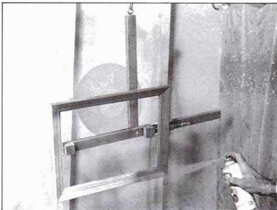
Fast and efficient way to spray-paint a frame is to impale it securely on the frame holder. The horizontal wood piece is then rotated vertically to paint the edges.
