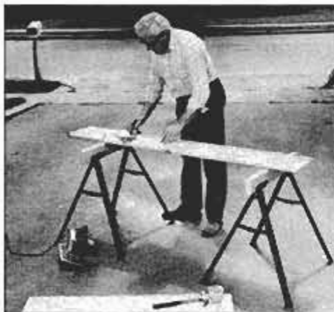
PM's tester, Rosario Capotosto, subjects Fas-Set's sawhorse legs to a stress test.
