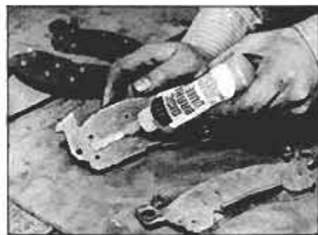
Compound applied to back of disc pads serves to quiet ear-piercing squealing.
