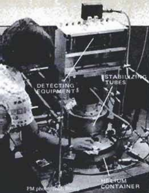
Stanford lab worker checks vacuum seal on the equipment that detected what is believed to be a monopole, a basic unit of magnetism. It took Stanford's Blas Cabrera months to locate one monopole.
