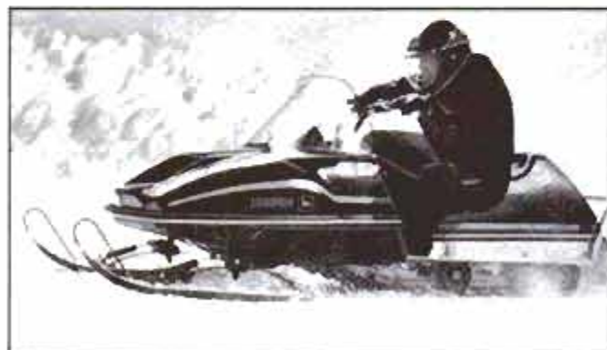
Liquifire, from John Deere, is a big, 436-cc-powered, liquid-cooled machine with both heat exchanger and a radiator.
