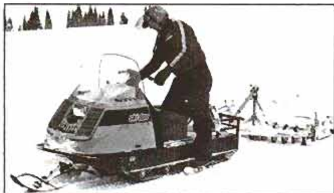
The single-ski, twin-track Ski-Doo Alpine, with its extra reverse gear, is a popular utility trail and ranch machine.
