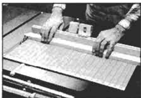
Swing the stop block up to square a ragged end without changing the setting.
