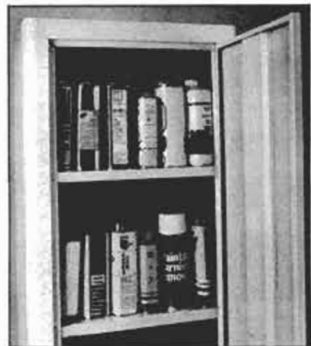
Store solvents in a lockable metal cabinet out of a child's reach. Flammable solvents, especially, should be kept in a metal cabinet, preferably out of the house.
