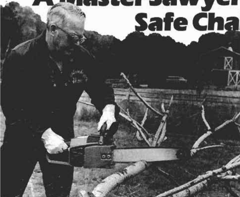
Dave Geer—a champion lumberjack—demonstrates safe techniques for limbing a tree. He's careful to cut in a spot that won't cause a sudden shift in the log's position.
