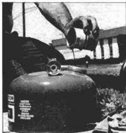
Oil and gas are blended to make chain-saw (two-cycle) mixture. Fuel should always be mixed in a separate safety container at least 10 feet from the spot where the saw will be used.
