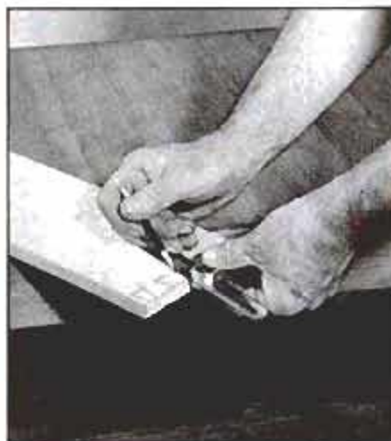
4 Use T-bevel to lay off duplicate lines at same angle, as when laying out sloped sides of dovetail joint.
