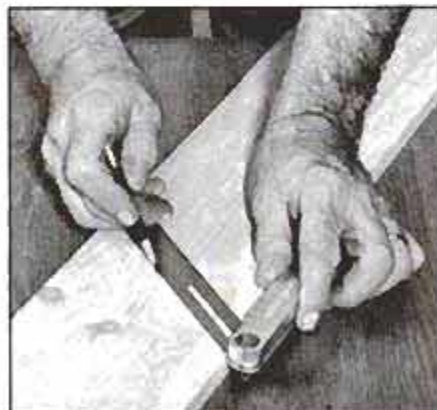
1 Typical use for a bevel square—laying off a miter. You can make a perfect match with an existing angle, too.
