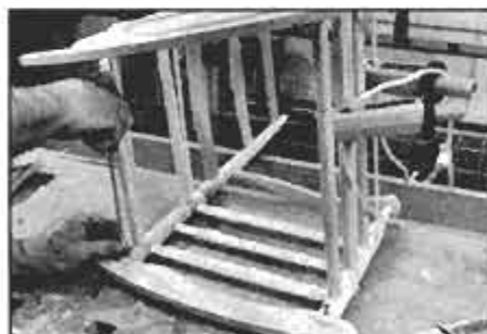
Rockers are installed using (provided) screws only, no glue, just as Shakers did.
