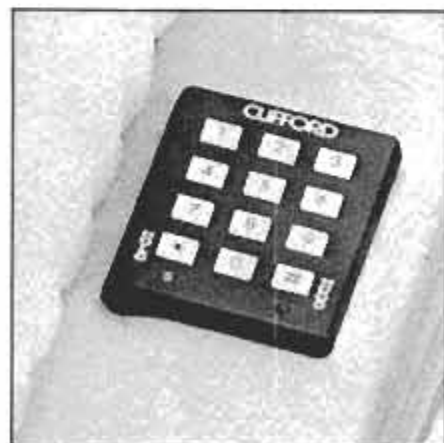
Keypad for Clifford alarm system was on driver's side armrest. System locks hood, kills ignition, blasts horns.
