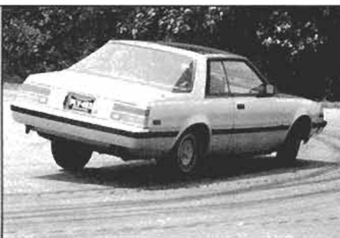
This production car is close to the point of terminal understeer. Note the weight transfer to the right front tire and the unloading of the left rear wheel.
