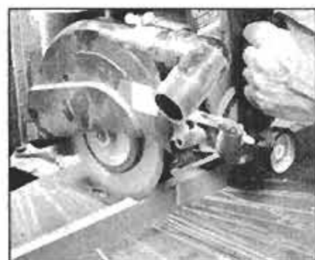
Cut a notch into a new fence to simplify alignment of cutting lines to blade path.
