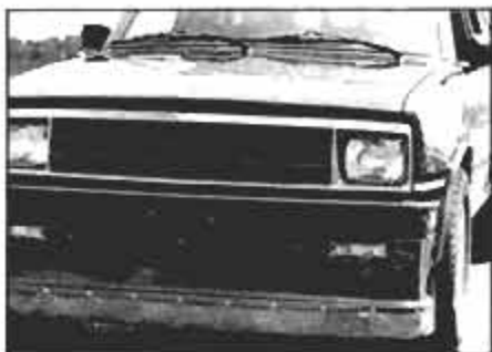
Headlight covers for Chevy (left) were handcut from clear plexiglass, painted with Cavalier logo. Aerodynamic spoiler for truck (above) has rubber extension.
