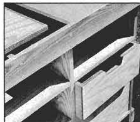
Close-up shows construction details: edge band around removable tabletop; screw-hole plugs; base-edge banding.
