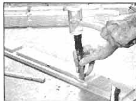
Use a sharp chisel to remove waste and to square the corner of the stopped rabbet.
