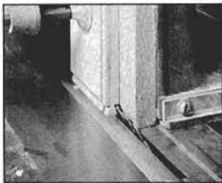
Cut sliding dovetails on drawer sides, using a tenoning jig, saw blade at 22°. Thicker stock is used as a spacer.
