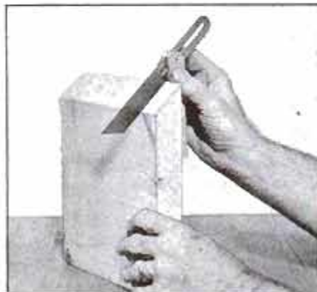
2 The T-bevel square is the tool to use when you have to check a beveled edge. Here stock fits tool angle tightly.
