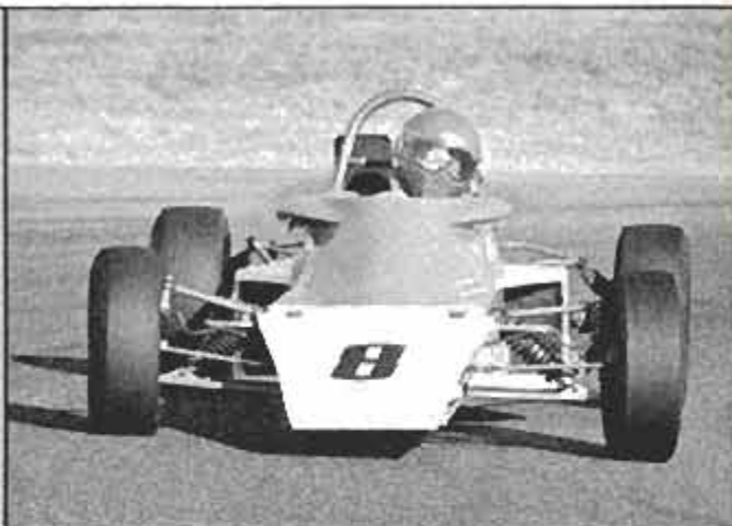
Slip angle is the difference between the direction of the tire and wheel, and the actual direction of the car. Note the tread distortion of the right front tire of the race car. It's in a tight left-hander at Laguna Seca Raceway.
