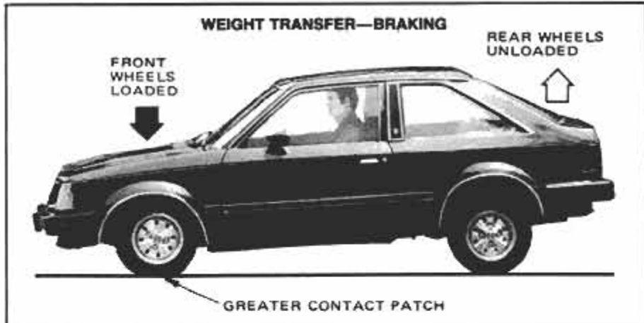
Forward weight transfer under braking can provide help in an emergency by increasing the contact patch and consequently enhancing the steering response.
