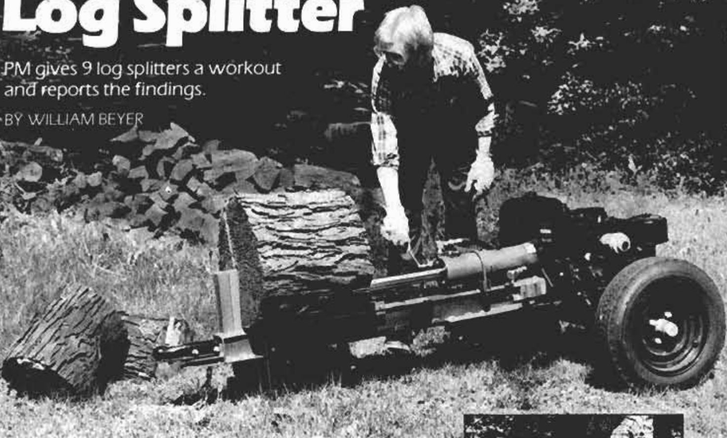
This 15-ton splitter is a Sears Craftsman. It's powered by an 8-hp gasoline engine.
