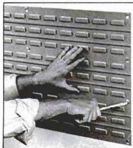
The metal bracket for the storage bins can be installed with screws or lagbolts.
