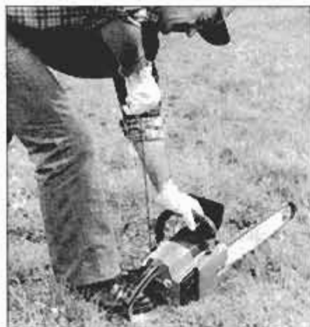
When you start a chain saw, hold down its back end with your foot or knee so that the chain and bar will be elevated clear of the ground. You should never lean over the bar past the chain line.
