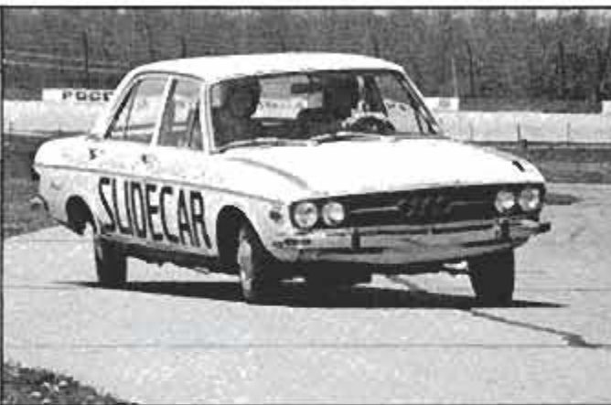
The Slidecar is made to oversteer. The driver here has dialed in enough opposite lock to catch the drifting rear end and is actually in quite good control of car.
