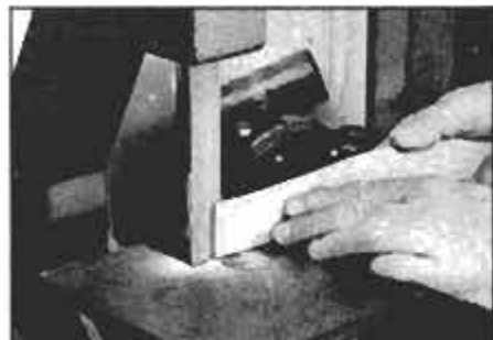
Last 1/2 in. or so at both ends of back slats were then sanded slightly before joining.
