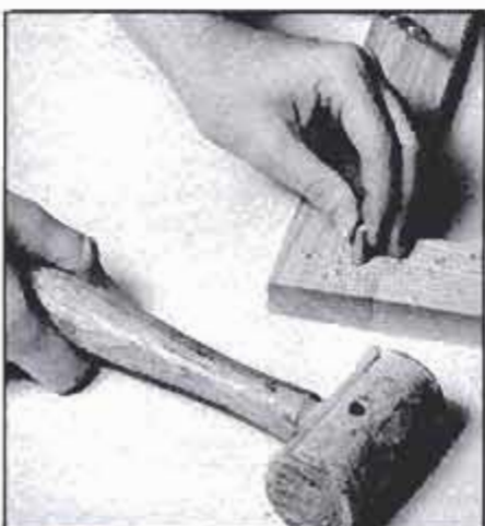
After facing has dried, bore 1/4-in.-dia. hole. Glue and pound in a 1/4 x 3/8-in. dowel. Sand dowel ends, stiles and rails.
