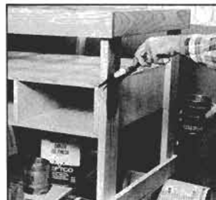
Deft's Danish Oil finish is very easy to apply; wood is simply saturated with it.
