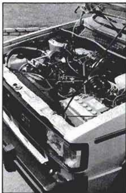
The 1.8-liter GTI motor pumps out 90 hp. Blackout exterior treatment is part of the standard GTI package. The interior gets well-bolstered sports seats.
