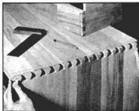
A practice dovetail joint was made as an exercise. The dovetails are cut first and used as a pattern for pins. Dots indicate the wood to be removed.
