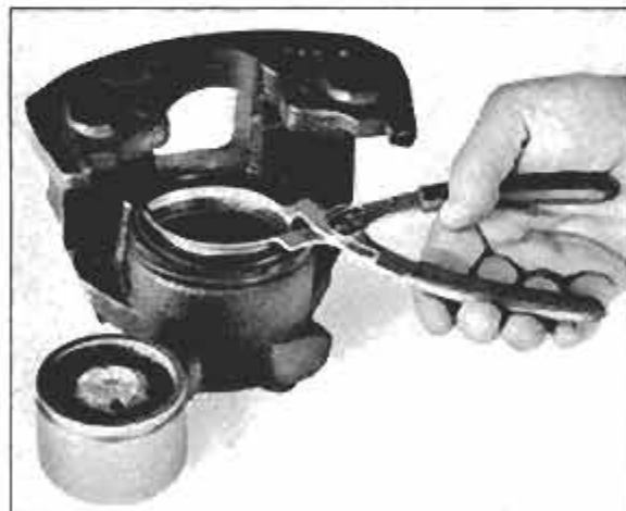
Disc brake dust-boot pliers spread dust boot for easy installation of brake piston. Pliers come in two sizes.
