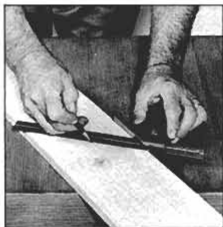
The combination square comes with an accurate 45° angle built into its head. Use it as shown to lay out this angle.
