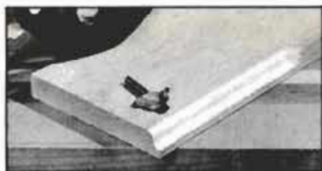
A Roman ogee is also a good bit to own; the shape gives an attractive edge to plaques and the like. By using the lower portion only, you can create a small cove.
