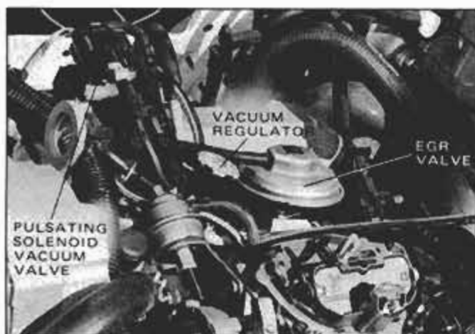
Computer-controlled pulsating solenoid valve (left) makes for tight EGR control. A new casting process eliminates porosity on the Pontiac 6000 STE wheel (right). Electronically controlled on-board air compressor on STE operates rear air shock to keep the car level. The compressor hose has a gauge (below) to inflate tires and toys.
