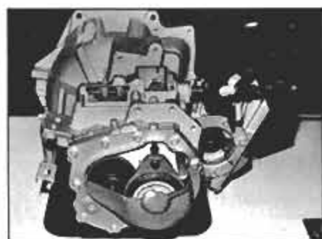
New five-speed transmission accommodates the fifth gear and synchro at the end of the gear housing.
