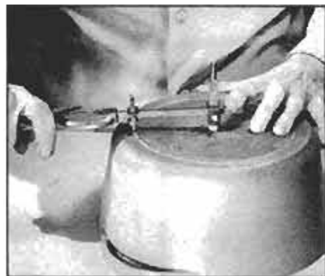
Circle cutter with extended cross bar removes heavy aluminum disc from bottom of discarded pot to form chuck faceplate.
