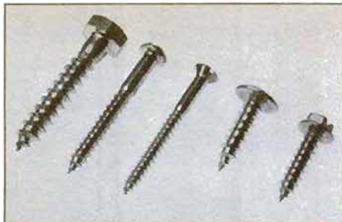
The lag screw (left) is used in heavy construction. It and the two adjacent screws are wood screws. The remaining two screws with coarser threads are intended for use in metal.
