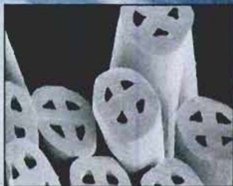
Enlarged even more, Du Pont's new Quallofil fibers reveal four air tubes per strand.
