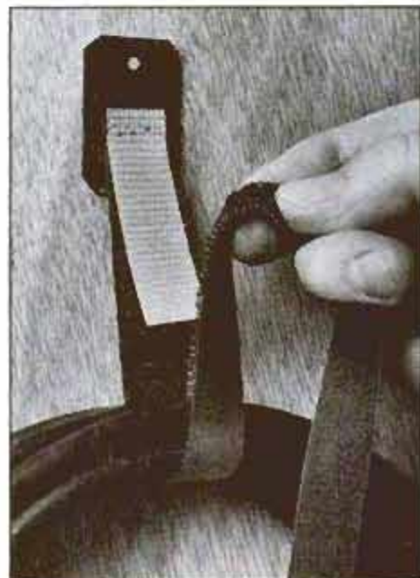
A Velcro strap is an ideal way to hang an often-used extension cord or other small objects. The strap tab is adhesive-backed. For heavier items, the tab has a hole for a nail, screw or other fastener.
