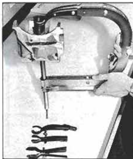
Adapter for valve spring compressor enables you to work on recessed valve springs with a minimum of fuss.
