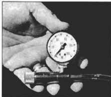
Computer-controlled pulsating solenoid valve (left) makes for tight EGR control. A new casting process eliminates porosity on the Pontiac 6000 STE wheel (right). Electronically controlled on-board air compressor on STE operates rear air shock to keep the car level. The compressor hose has a gauge (below) to inflate tires and toys.
