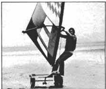
Dry-land sailing using the rig from a sailboard is possible with a Landsailer.
