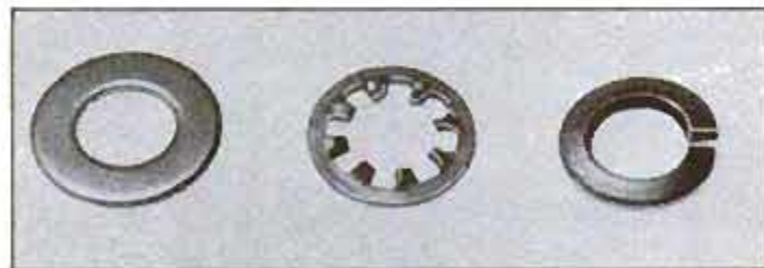
Three common washers used with nuts are (from the left): flat washer, internal-tooth lock washer and split lock washer. A flat washer tends to turn as the nut is turned, aiding loosening or tightening. The internal-tooth lock washer is often used with a wingnut to keep it tight. The split washer presses against the metal which also serves to hold a nut tight.
