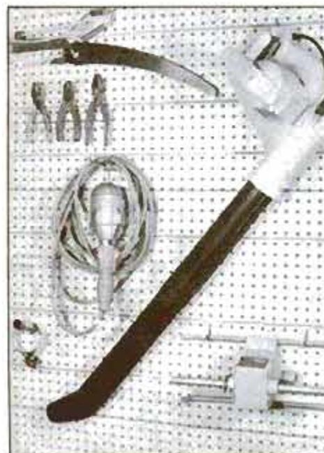
Adhesive-backed Velcro squares are used to fasten light items, such as a flashlight, within easy reach. Apply the hooked Velcro to the wall, the looped material to the item. Press the two together (inset) and the object remains in place until you need it.
