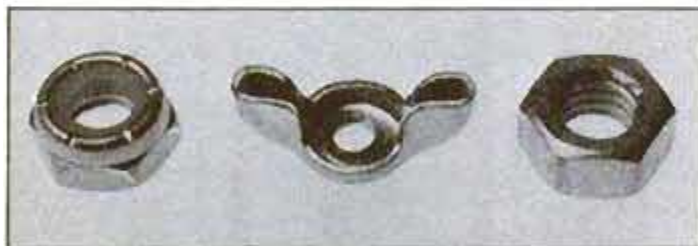
Three common nuts used with bolts are (from the left): locknut, wingnut and hexnut. The locknut, which is similar to the hexnut in its hexagonal shape, has a nylon insert which locks onto the threads of a bolt. The wingnut is used in situations where a nut must be loosened and tightened frequently by hand. Both the hexnut and locknut must be wrench-tightened.
