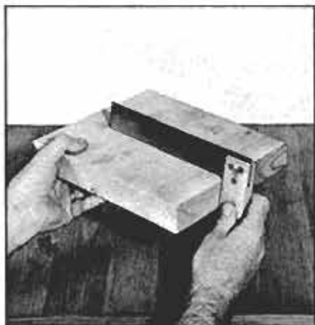
When board flatness is important, use a square to check as shown. If you find a crown or valley, plane the board flat.
