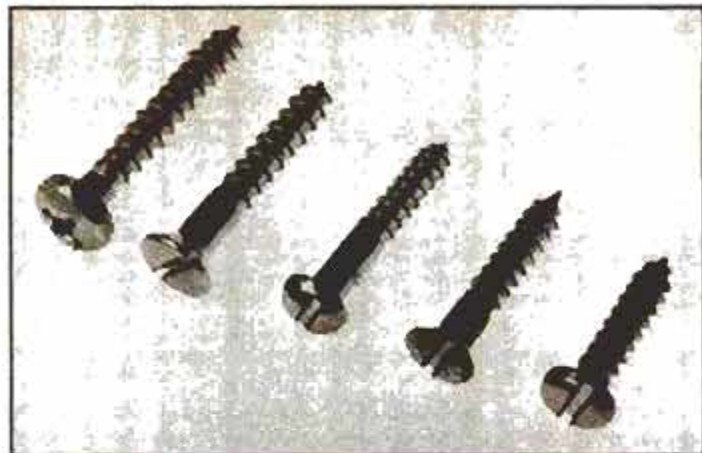
Heads of these screws are (from left): cross-slotted Phillips, oval, round, flat and panhead. Oval heads are partially countersunk into a surface; flatheads are driven flush (fully countersunk).
