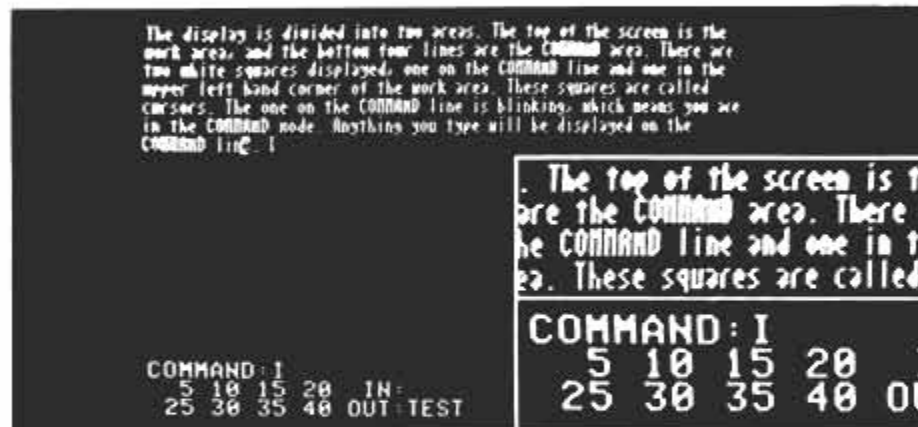
Screenwriter II 's display (above) features two type sizes. The large type is usual 40-column size. The smaller type is 80-column done without additional hardware.
