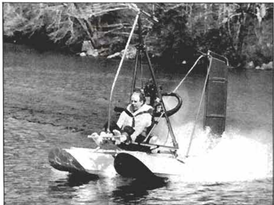
Remove the wing, add pontoons, and the Jet Wing becomes an exciting 40-mph airboat.
