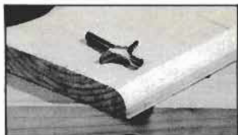
A rounding-over bit might well be the first one you will purchase. This shape is available in at least four radii.
