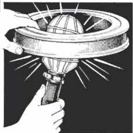
If the light from your droplight doesn't penetrate air filter, change the element.
