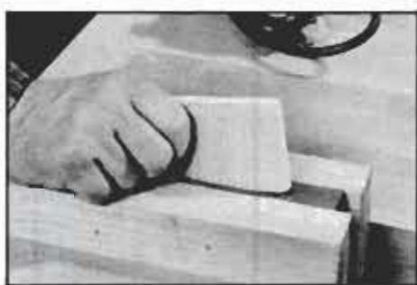
Cut spline mortises in both workpieces, then fashion the splines to suit openings they will fill. Here, in 1/4-in. stock, 1/2-in. splines will be glued into mortise.
