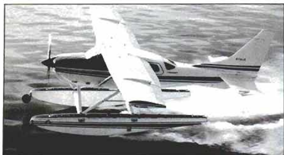
Watertight compartments, over 8,000 rivets, give integrity for tough water operations.
