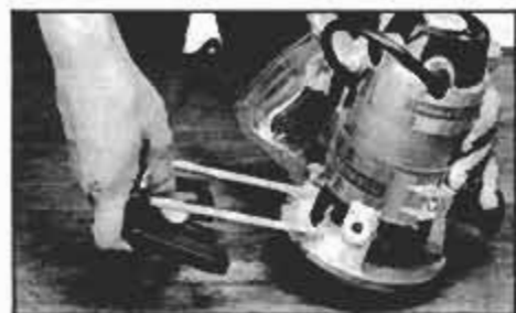
The edge guide on this router is installed into two holes built into the router base.
