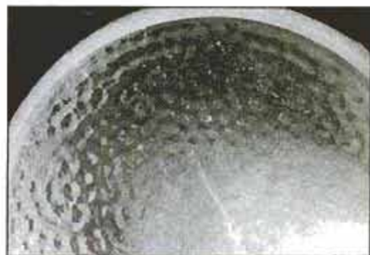
Inventor Mamo made a number of scale tests of bubble movement process. Photo shows pattern emerging around a block of ice, which moves to the right.
