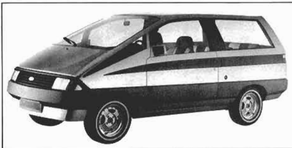
Future Ford van will be based on Escort platform. It will be 157 inches long, have a 94-inch wheelbase and carry six or seven passengers. A Chrysler minivan will beat it to market.
