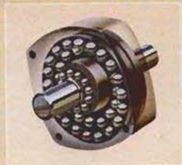
Precision: For critical assembly or processing jobs, conventional gearing doesn't supply consistently accurate robot positioning. Ball-bearing drive system could replace gears in future robots.
