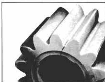
Crack in this gear is exposed within five minutes after developer is applied. Procedure exposes surface flaws only.
