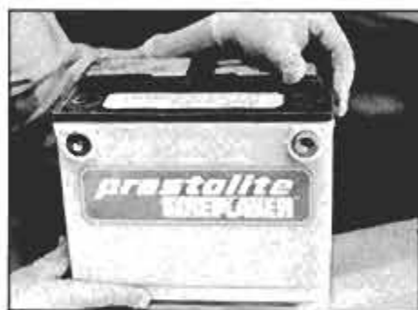
Prestolite FP800 battery features a cold-crank rating of 800 amps. at 0° F.
