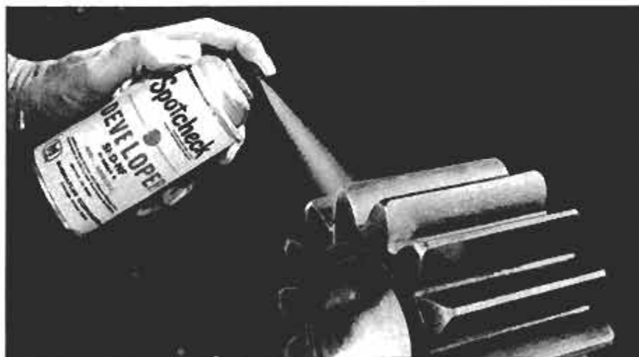
Spray on developer after surface has been cleaned and prepared with a dye penetrant.
