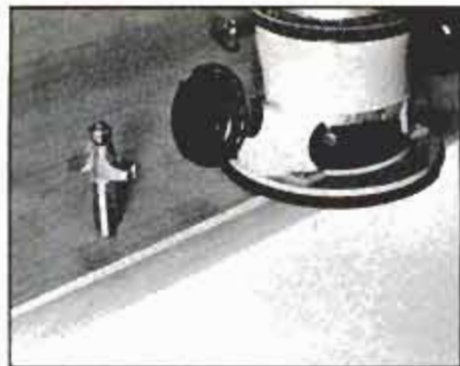
9 Using a router bit with a ball-bearing pilot greatly simplifies the task of cutting the rule joint on the tabletop.
