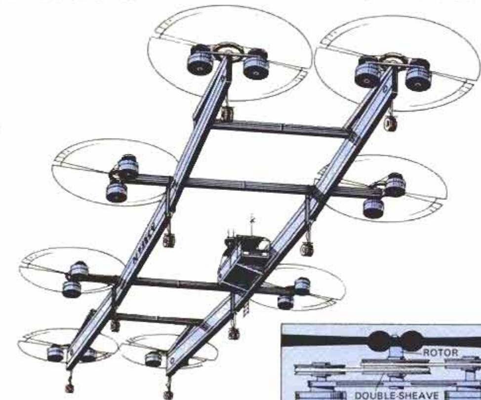
Proposed eight-rotor helicopter lifts 40 tons, has payload potential of 160 tons, world's largest. Simple, gridlike design keeps cost low. Inset shows how rotor is driven by two engines.
