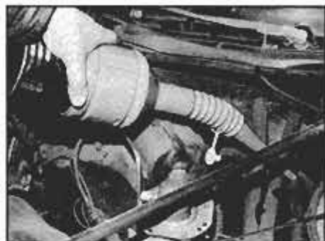
Flexible funnel pierces, holds and stores engine oil can. Cover cap seals out dirt.
