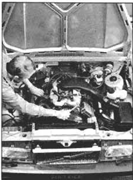
Hood opens 90° to the vertical position to allow for easy care of the 2.8-liter V6 (here) or the turbodiesel Four engine.
