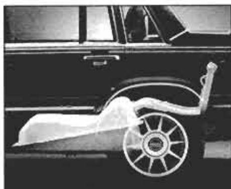
The 15.8-gal. fuel tank has unique built-in reservoir. It's mounted forward and has break-away-type filler pipe for safety.
