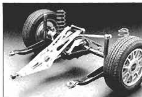
Wishbone-shaped subframe (light color) is centered over differential. It improves ride and handling of live rear axle.
