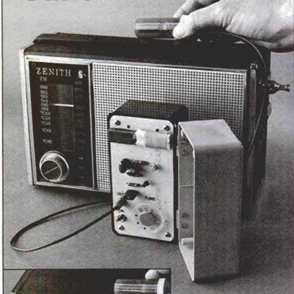
Antenna-Booster coil is held just above and parallel to the radio's own antenna (above). An AM radio antenna is usually a long, coil-wound rod that's easy to find (it's tinted in the photo at left).
