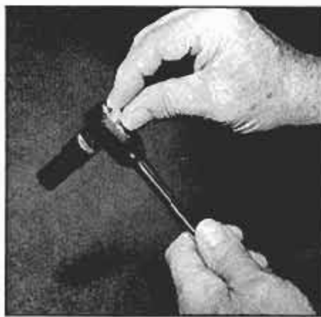
Sockets and extensions are locked onto ratchet and won't pop off until released.
