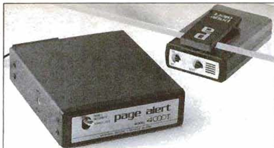
Page Alert 4000 is a silent radio alarm that activates a remote pager (beeper) in the event of a break-in. The unit has an effective range of up to five miles.
