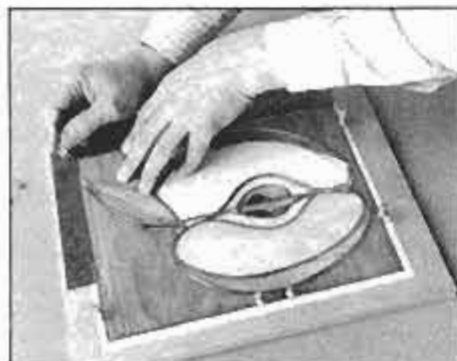
Place a pattern on scrap plywood and position the foiled glass on top of it. Check for square and size; secure with pushpins.
