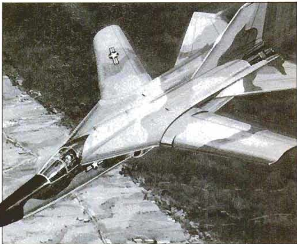
Artist's conception of an F-111 fitted with mission-adaptive wing. It's scheduled to fly in '83.
