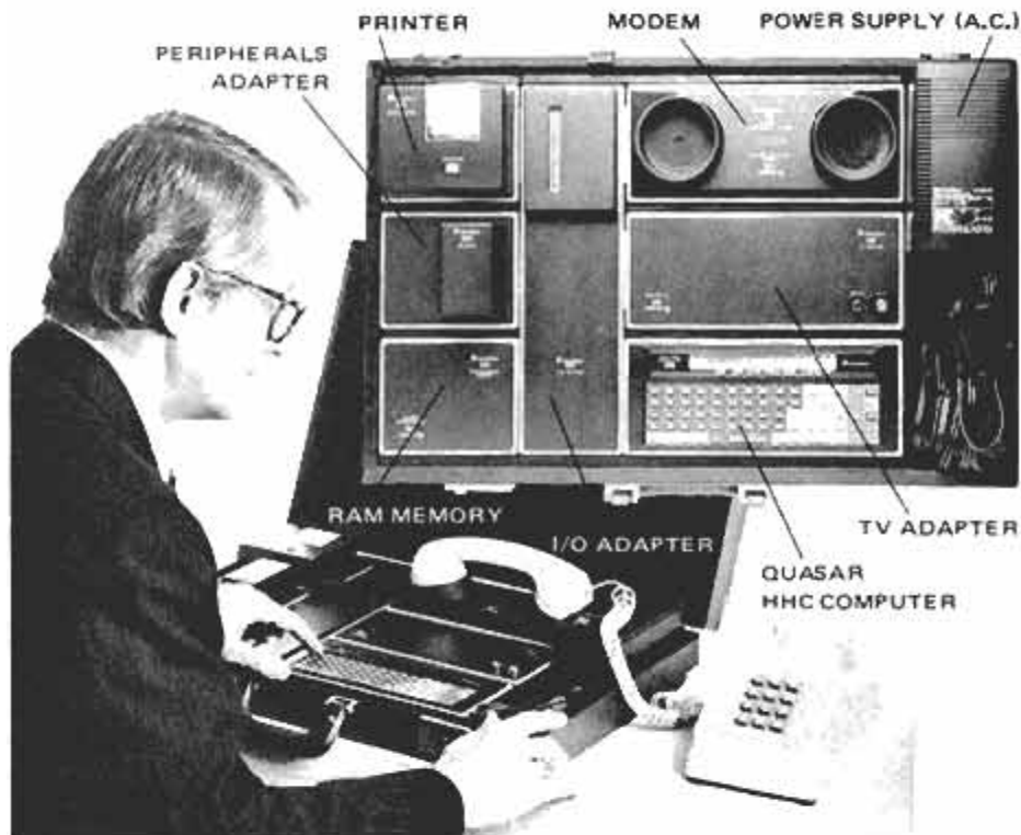
Plug-in attachments for the Quasar handheld computer (HHC) are shown in the inset. They will turn the HHC into a powerful computer system that will fit in your briefcase.
