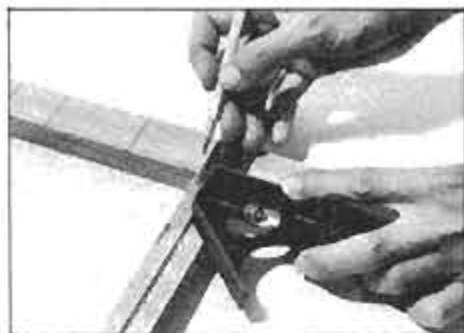
Mark the positions of the frets and nut carefully, using a combination square. This is most critical step in construction.
