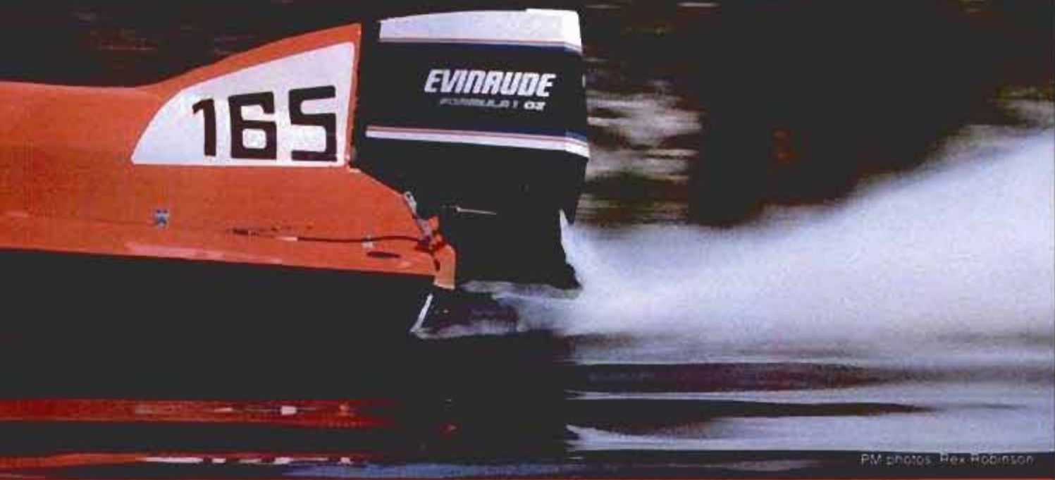
Cees van de Velden-enduro and Molinari-sprint tunnel hulls (above and below) handled smoothly at 100-plus mph. The potent new V8 powerplants are trimmed out with tilt and elevator-mount adjustments, which are controlled by steering wheel, foot and toggle switches in the cockpit.
