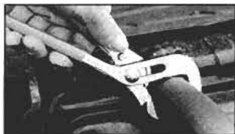
Adjustable-jaw-type pliers will hold a setting until you press the release button.
