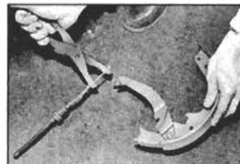
Special pliers will compress and hold the parking brake spring during installation.
