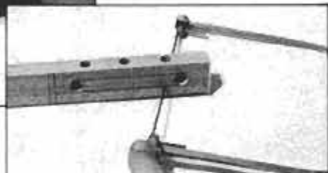
Tuning machines like the one shown here have a rigid metallic construction. The machines must fit firmly into the peg box.
