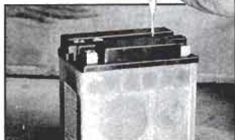
Tester is made especially for motorcycle batteries. Position of balls shows charge.
