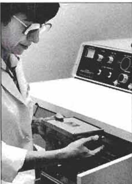
Janet Mouradian removes micrograph film from vacuum beneath the viewing screen.
