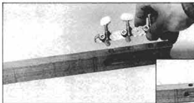
Tuning machines like the one shown here have a rigid metallic construction. The machines must fit firmly into the peg box.
