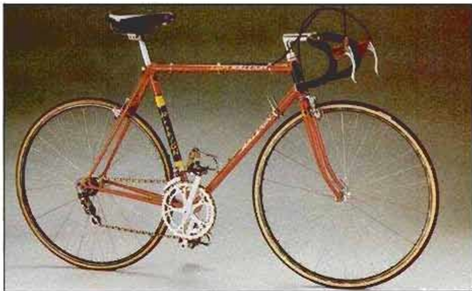
Raleigh Team Pro's 12-speed setup is based on top-line Campagnolo crank set and derailleurs; its tires are 260-gram Clements, which are mounted on Fiamme rims. This is the combo that took the 2,500-mile Tour de France—most prestigious road event in the world—two years ago.
