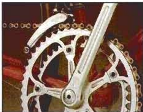
Raleigh Team Pro's 12-speed setup is based on top-line Campagnolo crank set and derailleurs; its tires are 260-gram Clements, which are mounted on Fiamme rims. This is the combo that took the 2,500-mile Tour de France—most prestigious road event in the world—two years ago.
