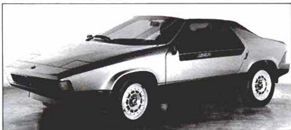
Exotically styled concept car, called Stealth, may be a preview of the Chrysler sports car currently under development. It's powered by a turbocharged 2.2-liter engine.
