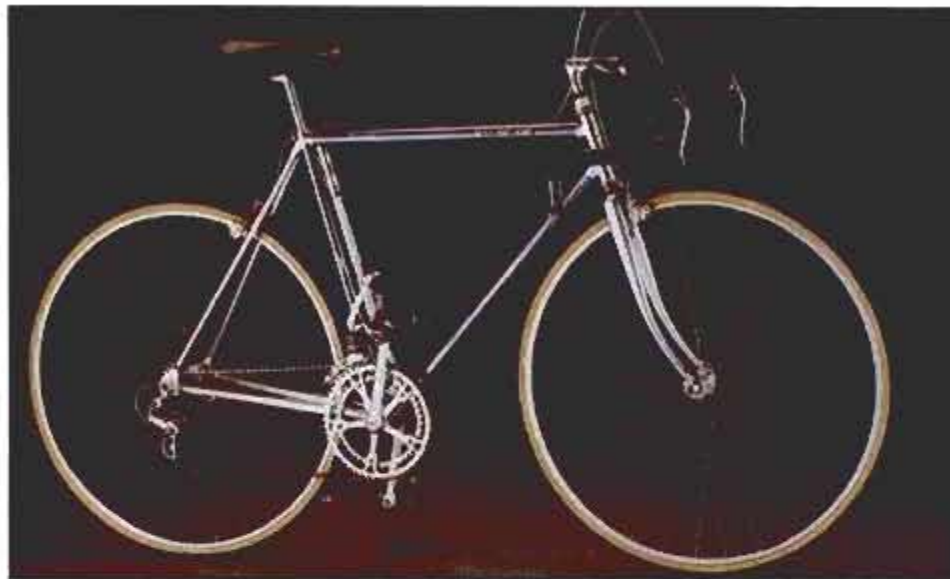
Motobecane's all-aluminum-alloy tubes (above) are expanded at the joints to provide greater area for aerospace cementing technique, which uses no lugs. Bike's lightness and finish are superior in its price range.
