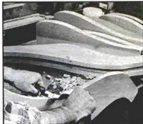
3 Use spoke shave to smooth saw marks. Always work with grain, not against it.
