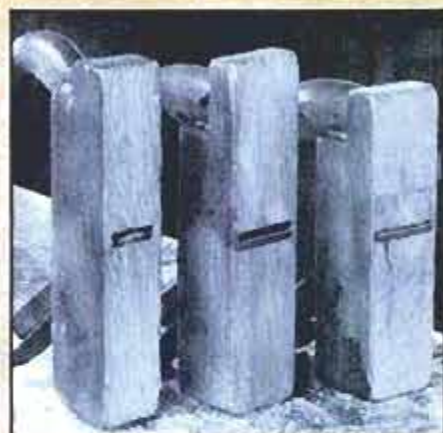
Scrub, jack and smoothing planes (left to right) are used for surfacing rough stock.
