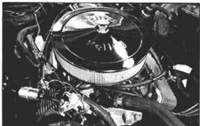
The free-flow, paper, air-cleaner element and housing is part of the kit. It lets the engine breathe more freely than stock unit.
