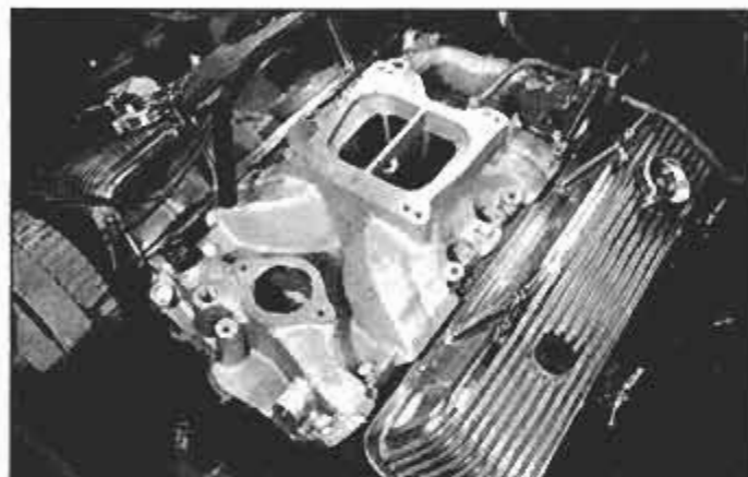
Holley Z Manifold has a divided plenum chamber for better fuel distribution and vacuum signal at low engine revolutions.
