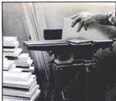
1 If stock is dressed on the sides only, joint one edge, then rip to proper width.
