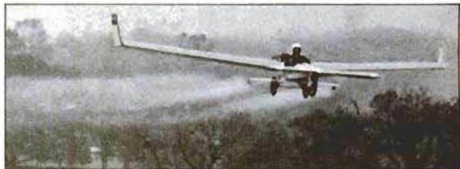
New role for an ultralight: Spewing twin streams of insecticide, 30-hp Gold Duster covers 40-foot swath at 60 mph, costs $8,500 as kit, is exempt from FAA licensing.
