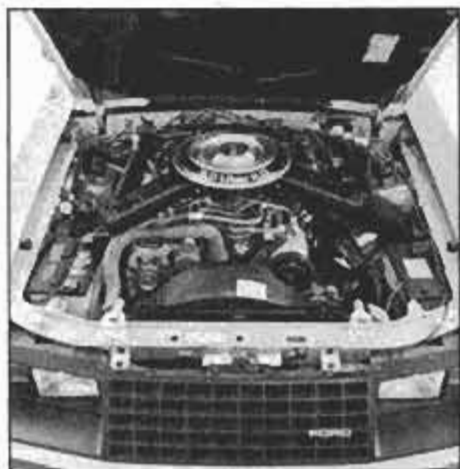
The optional 5.0-liter V8 engine makes the Mustang the quickest car on the market.
