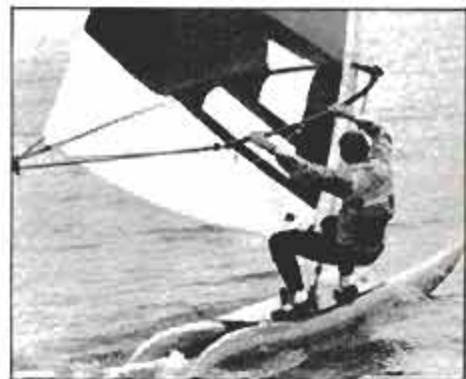
Twin inflated tubes are said to aid the stability of the British Twinsurfer sailboard.
