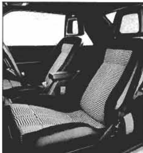
Recaro seat option gives support to enjoy handling of optional TRX suspension.
