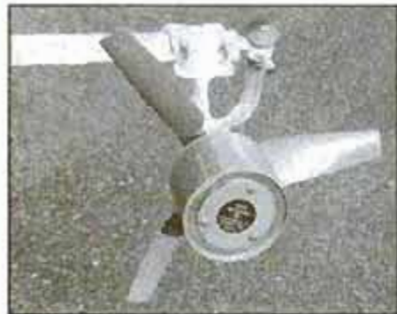
Prop-driven atomizer varies size of spray droplets to control bug-killing pattern.
