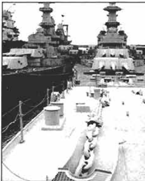
Foredeck of Iowa with Wisconsin lying alongside at Philadelphia Navy Yard. Dehumidifiers keep ships' interiors sound.
