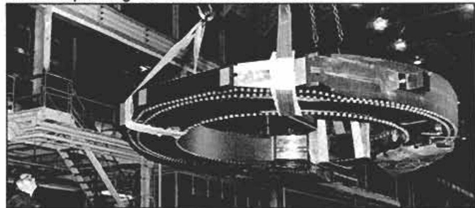
First of 22 big magnets is delivered to Princeton for the high-energy fusion reactor.
