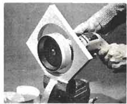
The large 4-3/8-in.-dia. sanding wheel runs cool and cuts at a fast rate.
