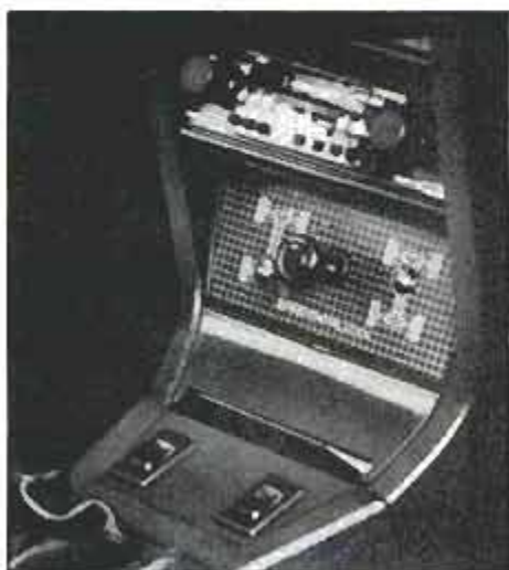
Differential locking knob is mounted on console; lights show system is activated.
