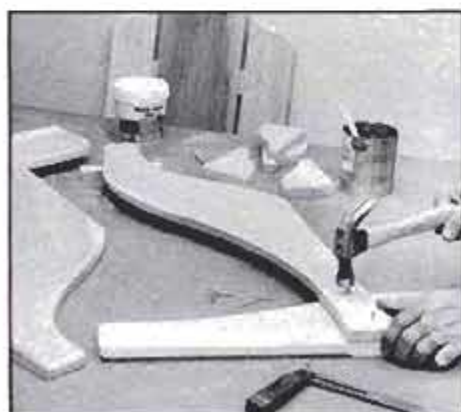
4 Start each assembly with legs. Use plastic resin glue throughout construction.
