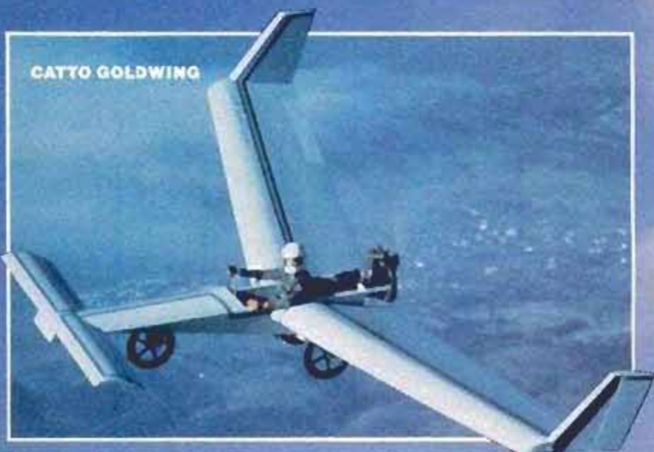
Endangered species? One of first "tail-first" canard designs, exotic Goldwing features sophisticated controls: elevator in canard, inter-linked ailerons and spoilers in wings, rudders in winglets. But at over 200 pounds, the 30-hp, 70-mph craft is one of many ultralights that may lose unlicensed status under new FAA rules. Kit is $4,295.
