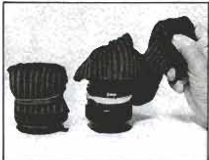
Replace only the element, not the whole filter.
