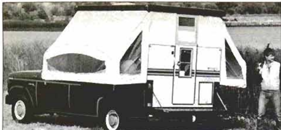
Coleman Wrangler slide-in tent camper fits standard pickups; Maverick model fits minis.
