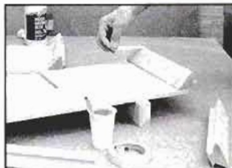
5 Masking tape must be used to hold glued joint together; clamps won't hold.
