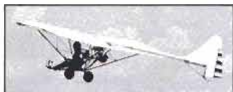
Twin 7-hp mills give Kolb Flyer speeds up to 45 mph. Craft has three-axis control.
