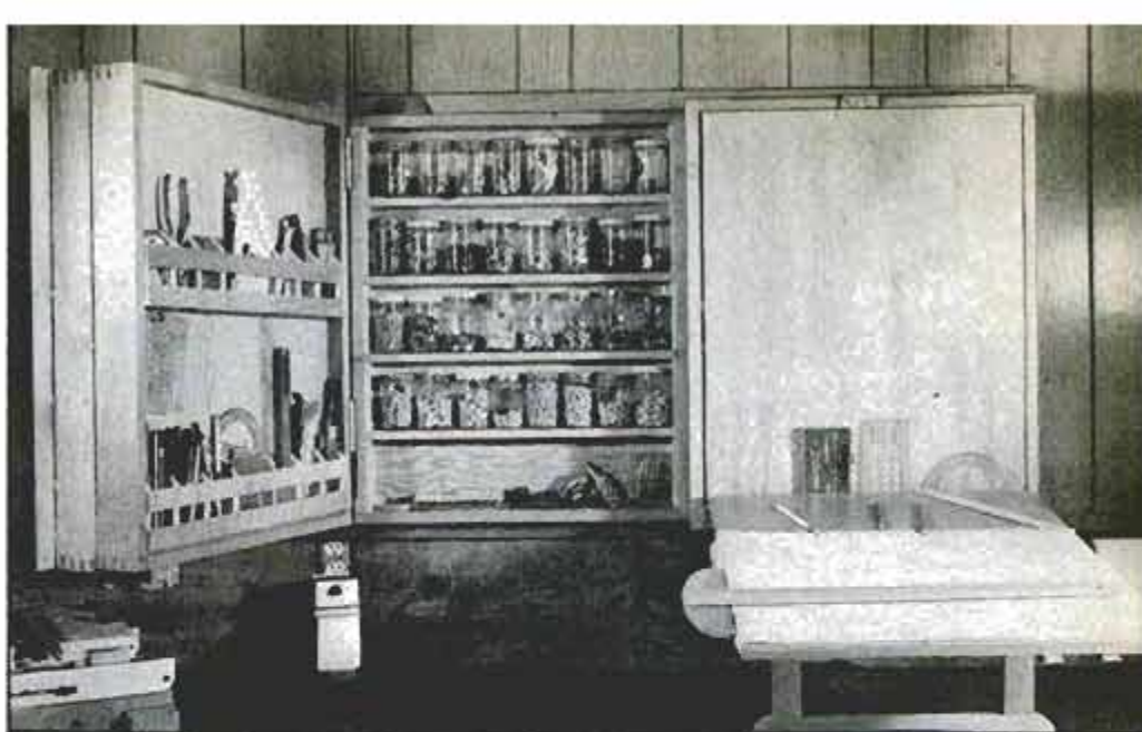
Drop-down drawing board is convenient. Store drawing materials on inner side of left inner cabinet. Drawing utensils in use are kept in a trough created when board is down.
