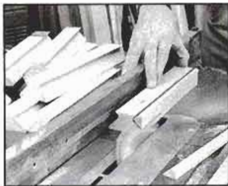
4 Fence is repositioned and the blade is elevated for the second series of cuts.
