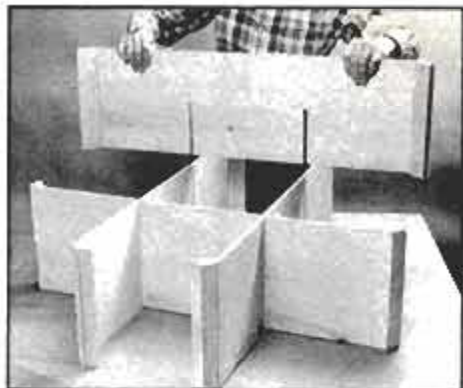
6 Test-fit panels together; do this work on a flat surface to ensure accuracy.
