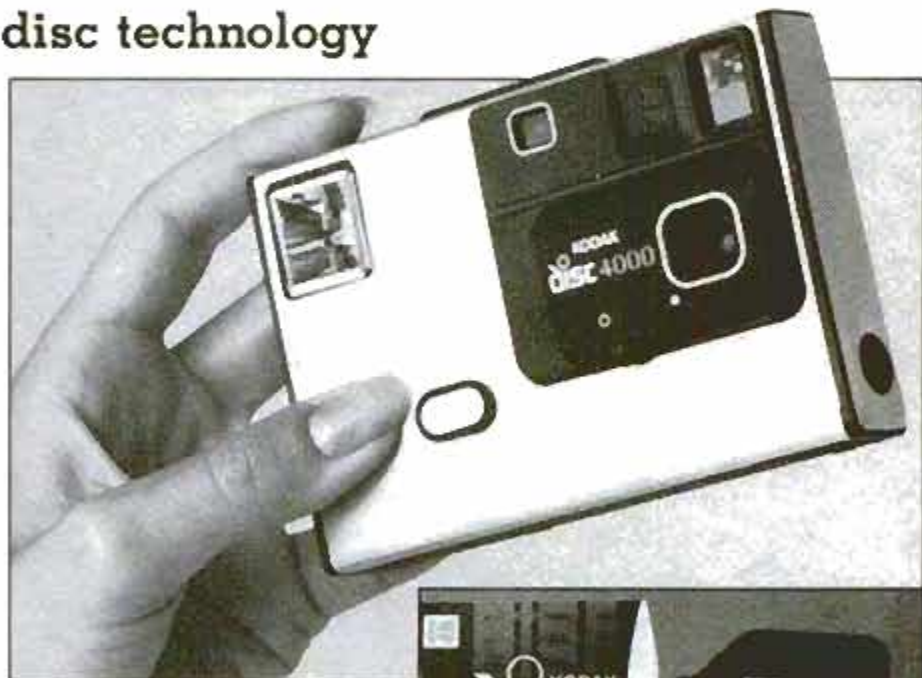
Kodak's new disc camera (above) uses cartridges (right) that hold 15 color-print negatives. Everything from flash to winding to new exposure is fully automatic.
