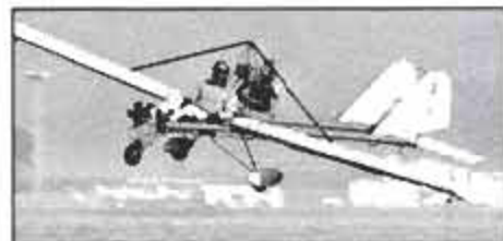
Jaunty twin-tailed P-38 Lightning, named after WWII fighter, does 55 mph on 30 hp.
