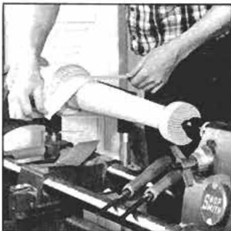
After shaping the post section, sand it smooth before removing it from the lathe.
