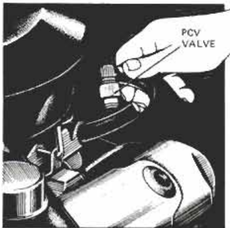
A PCV valve that won't rattle when you shake it is shot and should be replaced.
