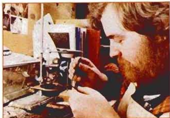
Steve Tofano, above, sculpts a figure using molten wax. The finished model is sold to a manufacturer, who makes a mold.
