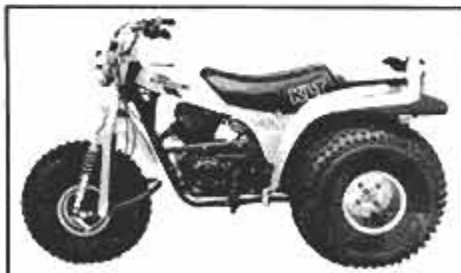
Grown-up tricycles are popular new rigs for off-road work and fun. Kawasaki KLT 250 has improved suspension, 246-cc mill.
