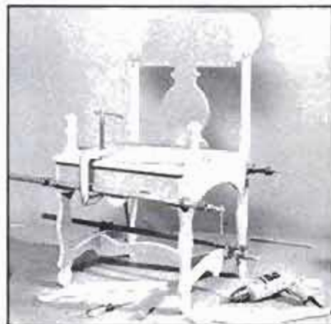
21 The chair is dry-assembled with clamps to bore the pilot holes for the screws in same way table was preassembled. Use drill press, then portable drill.
