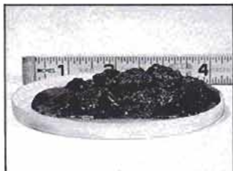
This much sediment was flushed from my tank in approximately 1½ hours using about 50 to 60 gallons of water. The amount of sediment varies with water hardness.
