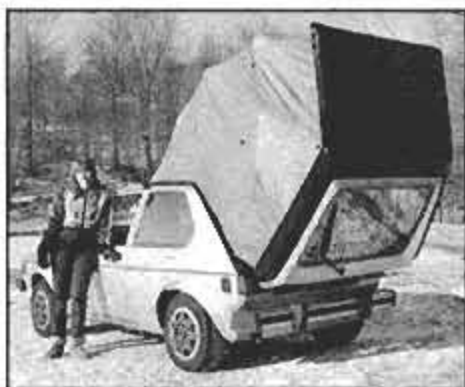
This VW Rabbit can hatch a hutch called a Hatchpack. Flip-up top opens out to cover a double bed for campground overnighting.
