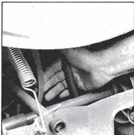
6 Make sure the mower's drive belt is properly tightened and not frayed or cracked. The drive belt may be partly inaccessible, but don't ignore this check. Turn the driveshaft by hand to inspect the full length of the belt. (Check your manual.)
