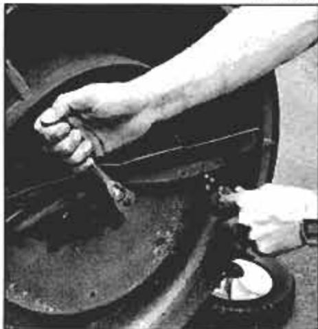
4 To remove or tighten cutter bar, hold in place with a screwdriver shaft inserted into a drain hole (left hand). Then use a wrench to turn cutter-bar mounting bolt. To tighten, turn clockwise as shown above.
