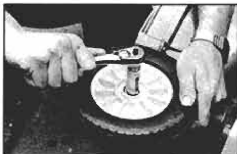
2 Turn the mower on its side to give the underside an overall inspection. Make sure each wheel nut is firmly tightened.
