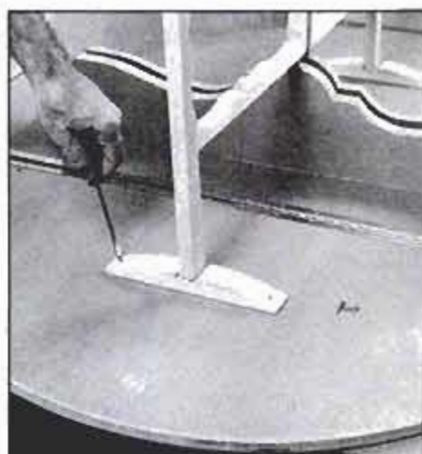
20 Here's how the stay secures the leg. Clearance at hinge allows leaf to be raised slightly, so the leg top clears the hump.
