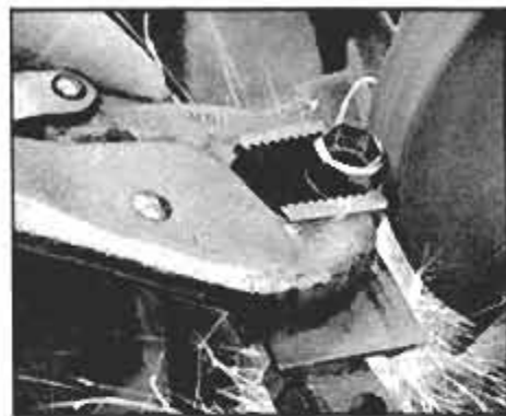
Use locking pliers to hold the socket head while grinding it to a hexagonal shape.
