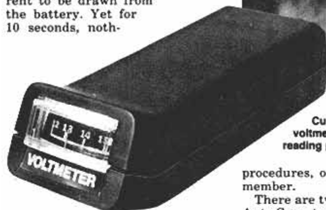
This project is more than a voltmeter (above); it's also a very sophisticated car burglar alarm. You can build it from kit or plans.
