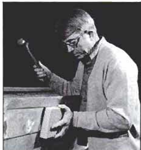
Dents in aluminum are smoothed out with careful peening and wooden backup block.
