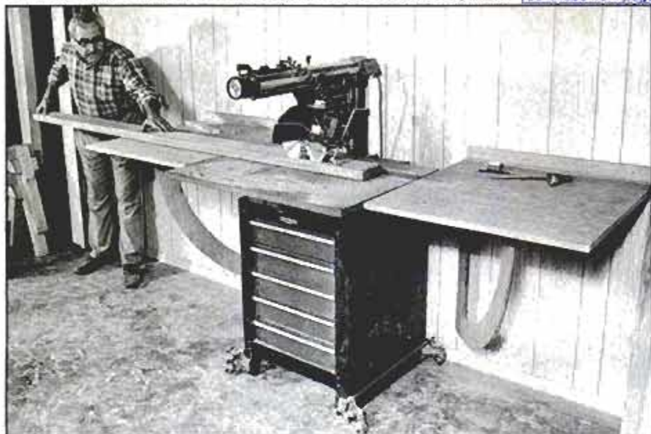
These drop-leaf tables keep work safely supported when sawing large boards alone.
