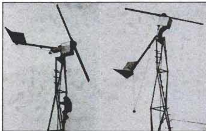
Windgen wind turbine in normal operating position (left) and tilted up in high wind: sliding weight damps the movement.
