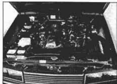
The 2.4-liter, fuel-injected Six is capable of pumping out 120 hp at 5,200 rpm.
