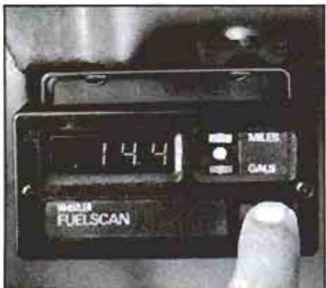
Compact Fuelscan monitors miles per gallon and distance, in miles, to an empty tank.
