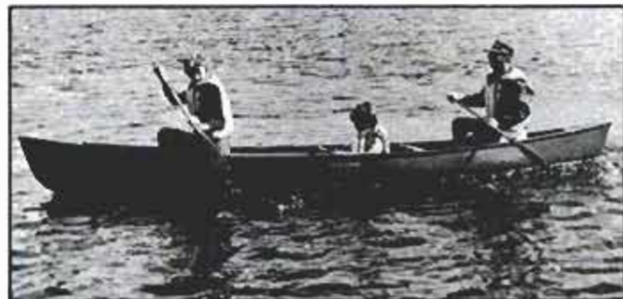
Old Town's Penobscot model is ABS plastic. Oldest of the canoe builders also uses fiberglass and Kevlar in addition to wood.
