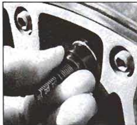
Pressure gauge mounts on valve stem and indicates tire pressure when it's pushed.
