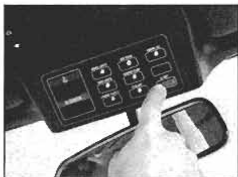
Warning lights set in the headliner alert the driver to a variety of malfunctions.
