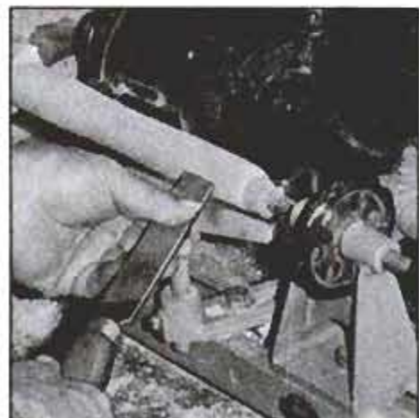
Shape handles with a skew chisel, leaving waste on headstock end. Cut tang end of handle to precise diameter for ferrule.
