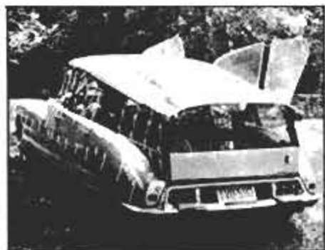
Reader Kamm's test car, a Citroen, sprouting tailfins for aerodynamic experiments.
