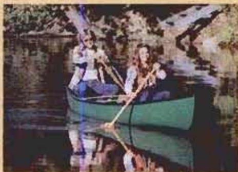
New Carleton from Old Town, a 78-pound 16-footer of Royalite, comes as a semi-kit.
