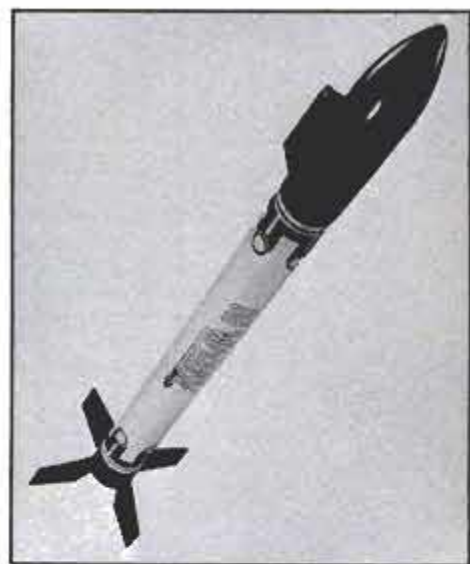
Astrocam 110 takes pictures from 300 to 500 feet high. The engine size sets altitude.
