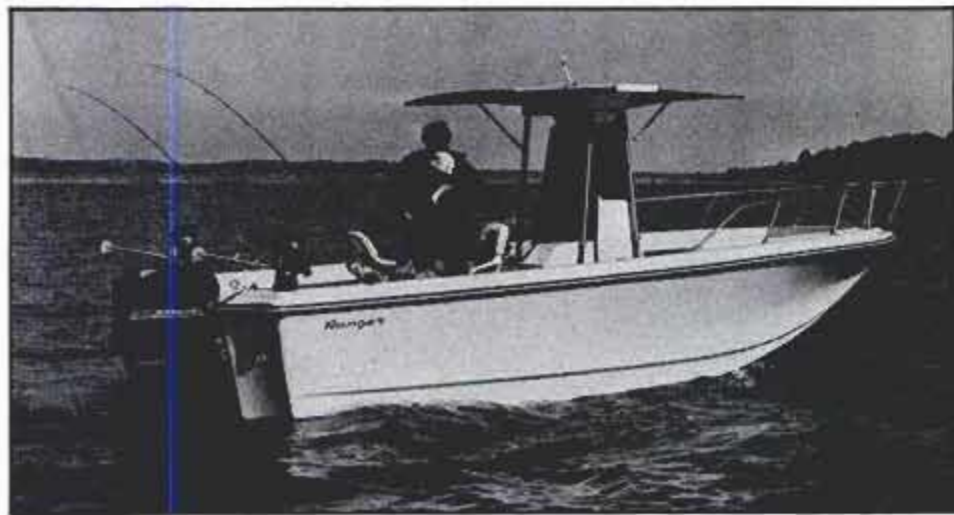
Ranger 622, a trailerable 22-foot, open-water, offshore fisherman with self-balling cockpit and high and safe freeboard, is new addition to a famous line of bass boats.
