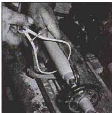
Once the first handle is turned, use it and outside callipers to ensure that following handles are turned to uniform shapes.
