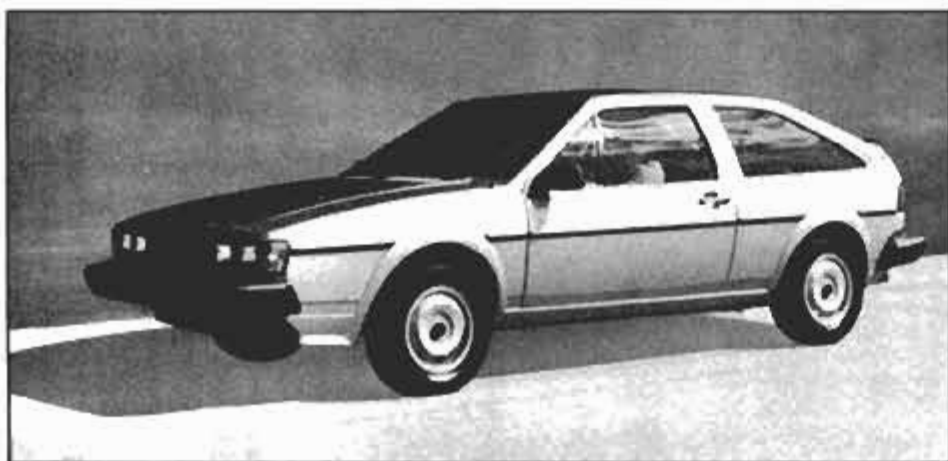
Restyled, but mechanically unchanged, the new Scirocco slices the air with a low .39 Cd.
