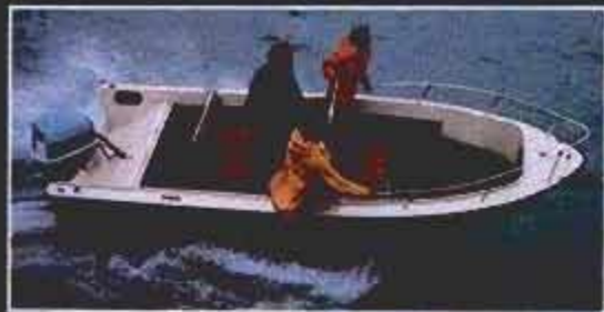
Grumman's aluminum 5.0, 17-footer, designed by Bill Shaw, gets a deeper V-bottom and provides a softer ride for fishermen cruising farther offshore.
