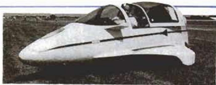
Sleek, aircraft-type styling is patterned after BD-5 fuselage.
