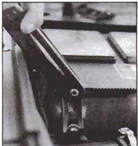
Clamps have fold-out adapters which you can clip onto side-mounted battery posts.
