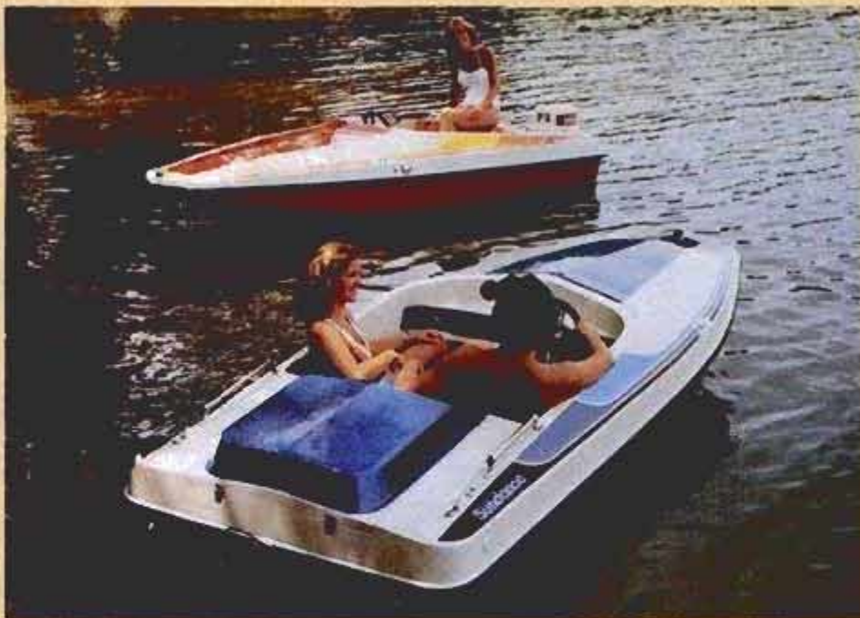
Some minis can mount inboard or outboard power options. Two-seater Sundance with 50-hp Arctic Power jet (foreground) or 35-hp outboard (background) can do 30-plus mph.
