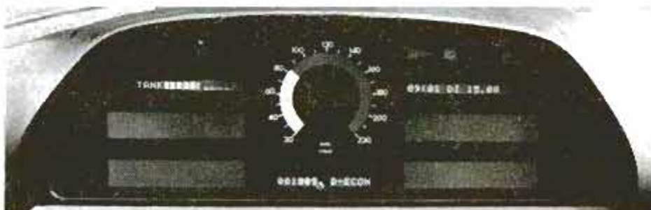
MB's new dashboard has four information panels operated through a keyboard on steering wheel. In addition to monitoring the engine, it supplies navigational data.
