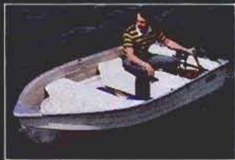
Aluminum is lightweight for portability. MirroCraft 10-foot Resort weighs only 120 pounds, but is rated to carry up to 500.
