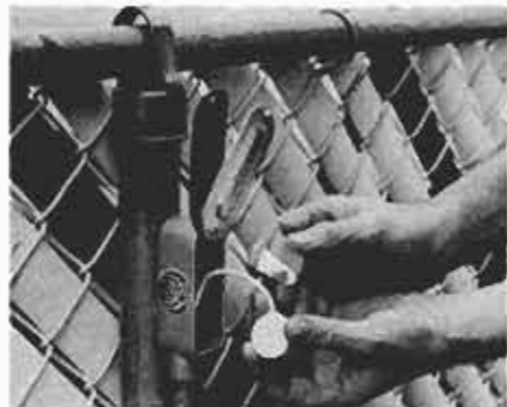
Fences are barriers to thieves. Napco makes a vibrator detector (about $9.50) to detect a thief climbing over a fence. For more information, see page 117.
