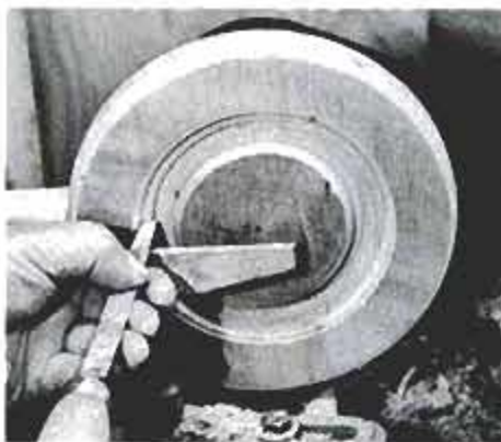
To make tops, cut a disc to size and complete detail work on lathe. Then cut disc in two and cut out centers to form arcs.
