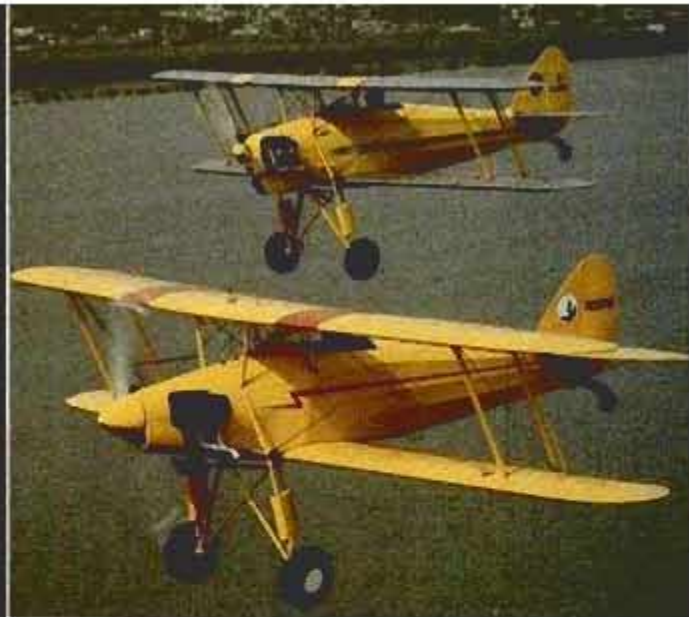
Looking like old-time barnstormers of the 30s, these nimble, single-seat Skyotes are actually high-performance biplanes designed for aerobatics. Stressed for +9 Gs and -6 Gs, they feature dual ailerons, can be built from plans and partial kits.
