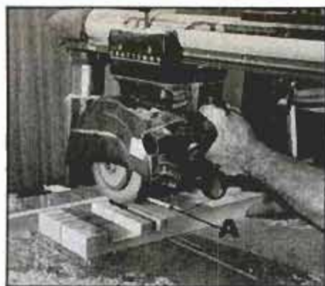
Uprights are cut in pairs with radial-arm saw to assure aligned dados. Use masking tape (A) to keep boards aligned.
