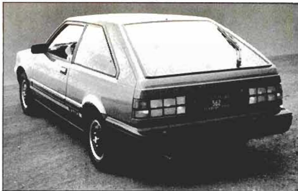
Sharply raked and chopped rear end of the Stanza is part of the reason for its very low coefficient of drag (Cd). Rear trunk volume with the seats up is 20 cu. ft.
