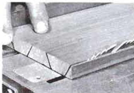
After 30° setting is made, cut beveled sides. Mark stock as shown: flip over after each cut for economical use of wood.
