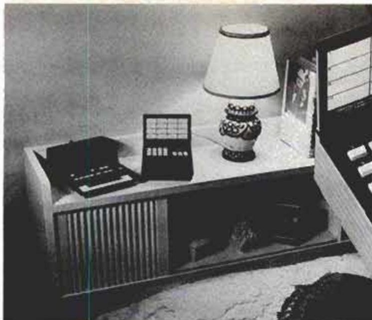
Automatic lighting-control systems use two control boxes (and modules detailed on following page) which may be placed at bedside or any convenient spot (BSR system shown). Main control box (top right) lets you manually control your lights and appliances. You need the programmer box (bottom right) for automatic control.
