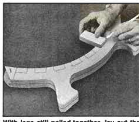
With legs still nailed together, lay out the arc for proper position of notches. Use a stepped block as marking template.
