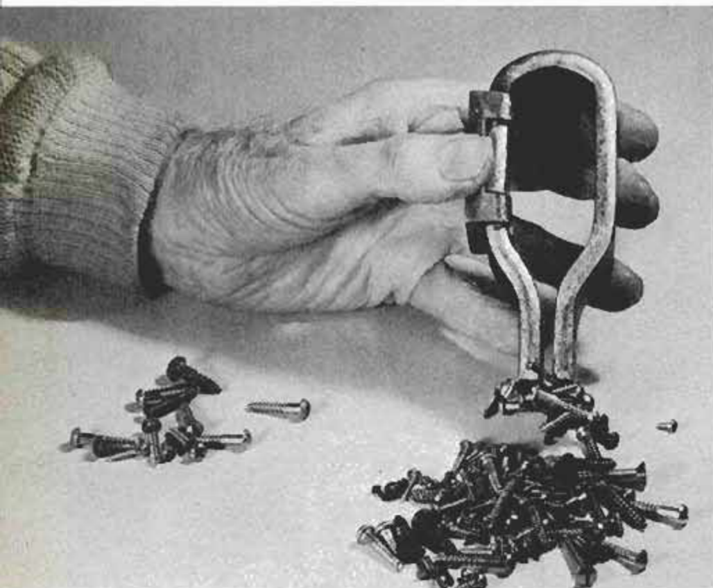
1 Use an old electric-meter magnet to separate steel screws from brass screws. These powerful magnets are easy to find and can handle many home and shop tasks.
