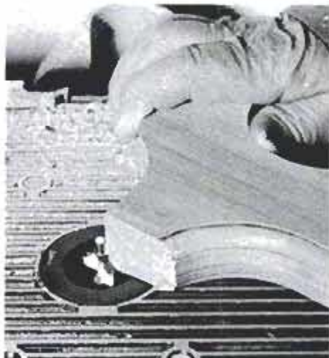
After sanding the sides and shaping the tops and the feet as shown here, the feet may be trimmed to their final size.
