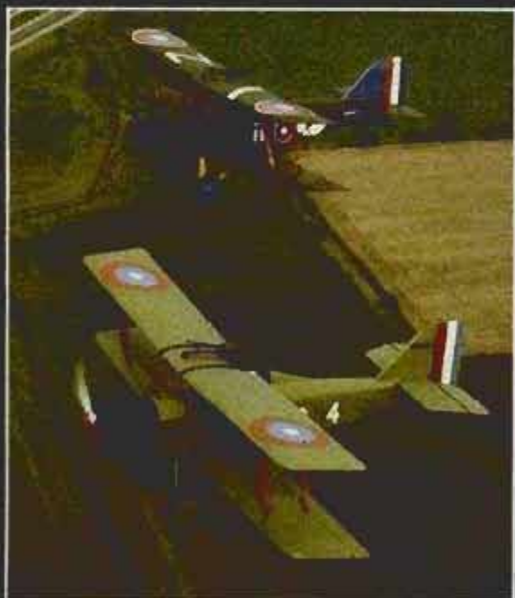
On dawn patrol, two British S.E.5a fighters hunt the Red Baron. The nostalgic WWI biwingers are 85-percent-scale, wood-and-fabric replicas with speeds up to 120 mph—just about what the originals managed.
