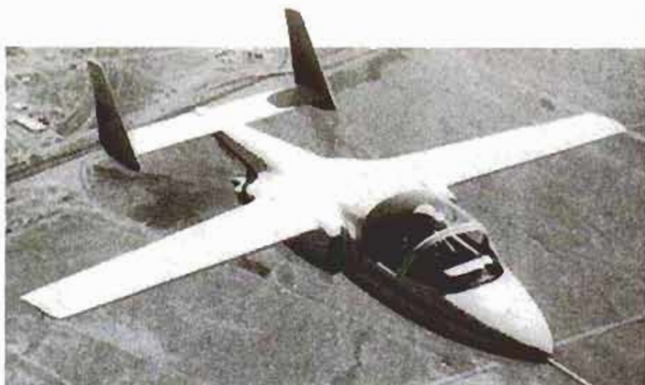
Proposed new Air Force trainer is designed like a homebuilt sports plane. Prototype above is a single-seater, but production version will have two seats side by side.
