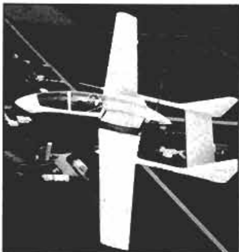
A pair of twin-prop Crickets, performing a "mirror-image" routine, show off their aerobatic skills. The tiny single-seaters are powered by two 12-hp chain-saw mills.
