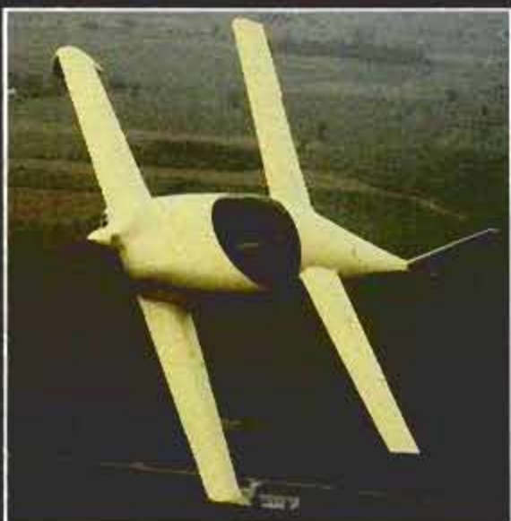
Sleek new Q2, two-place version of famed canard-wing Quickie, gets 180 mph and 60-mpg economy from small, 64-hp mill. The futuristic, all-composite craft has wheels and elevators in nose wing. Kit is $10,495.
