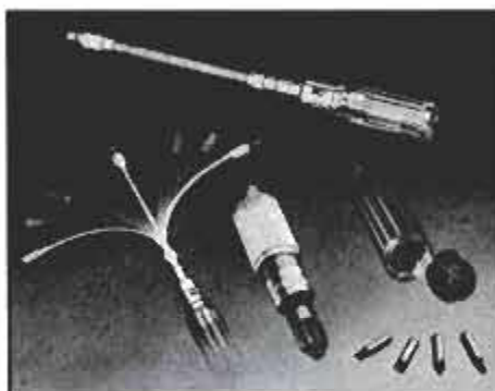
Unique flexible screwdriver will drive in or take out screws up to a 90° angle.
