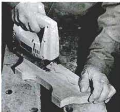
Using grid to scribe a pattern, cut out two slightly oversized feet with a sabre saw.
