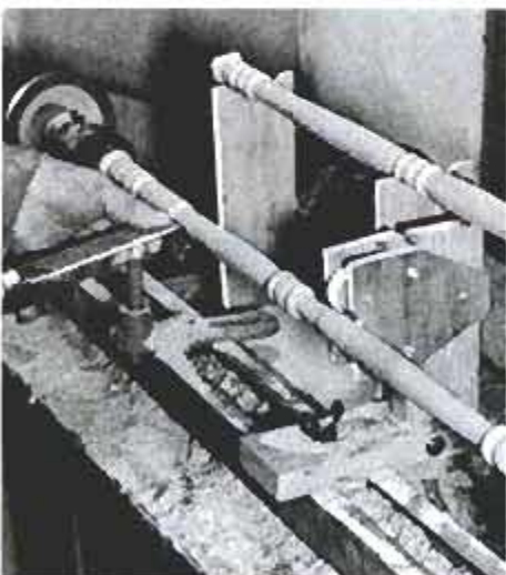
Shape the bars and uprights on your lathe according to a pattern of your own design.
