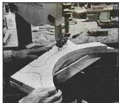
Gang-saw the legs. Nails driven on the waste side of outline hold pieces together.
