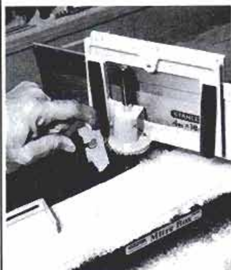
Spring-loaded wedge is pulled back to disengage the saw guide so it can be swung to new cutting position desired.
