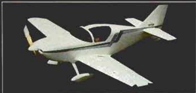
Award-winning Glasair is sporty, fixed-gear, side-by-side two-seater for engines up to 160 hp and speeds up to 230 mph. Rate of climb is a brisk 1,600 f.p.m. Kit, less engine, is $8,200.
