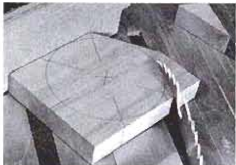
Use a miter gauge (not shown) to cut hexagonal top from ¾-in. stock. Saw blade should just touch the circle's perimeter.
