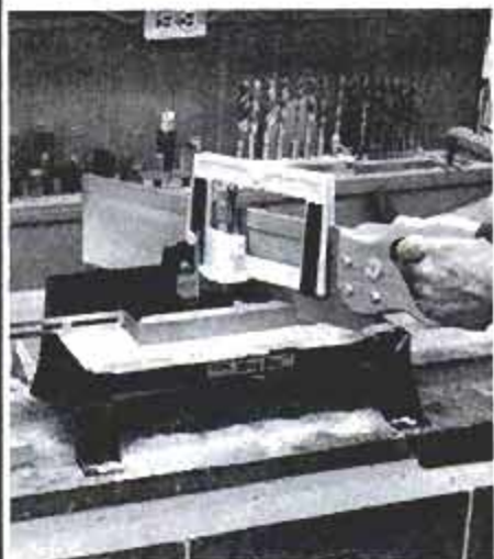
Tough, free-floating plastic guides hold saw in accurate alignment throughout while a five-sided figure is being cut.
