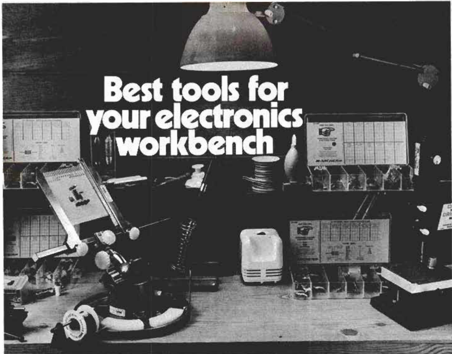
Well-equipped work center: Note the Pana-Vise (left) and small drill press (right). Cube-shaped table vacuum is in the center.
