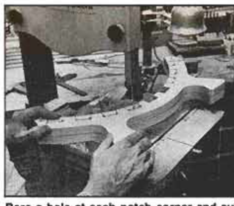
Bore a hole at each notch corner and cut out the waste. Holes simplify cutting and give completed notches a finished look.
