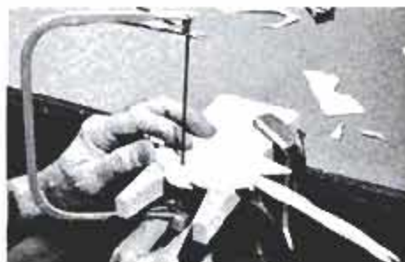
Coping saw does a quick, neat job on 1/8-in. plywood. Use a bench pin for support.
