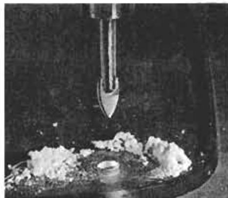
This ¼-in. tungsten-carbide bit mounted in a drill press can easily drill through ¼-in. plate glass in several minutes.
