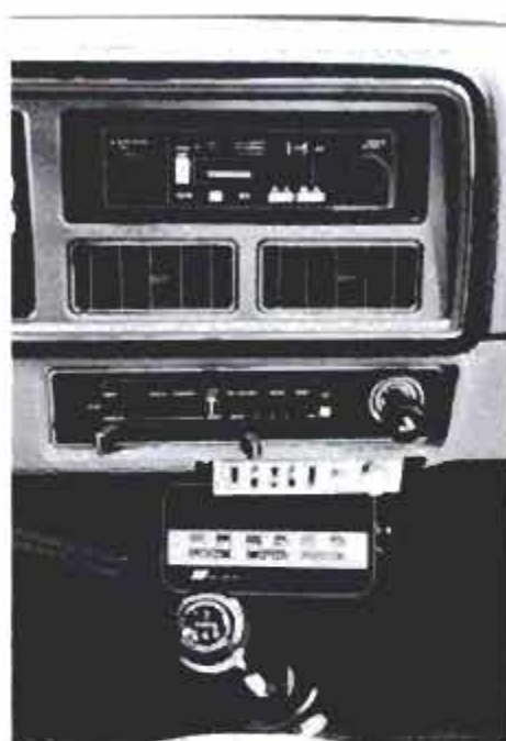
Zemco ZT-3 driving computer (mounted under the dash) monitors fuel consumption.
