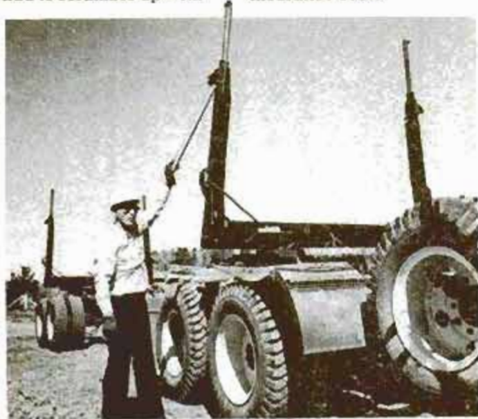
Simple jack—long overdue—keeps driver out of harm's way.
