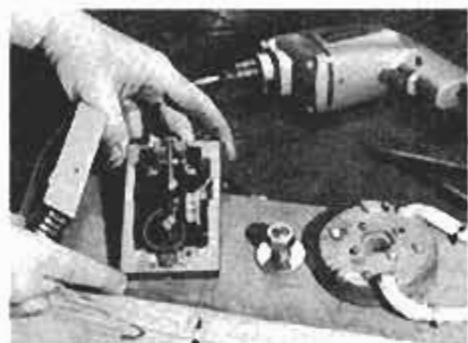
Contacts in line-voltage thermostat close with a rise in temperature. Set it 7° to 10° higher than house thermostat. It's about $25 in airconditioning-supply stores.
