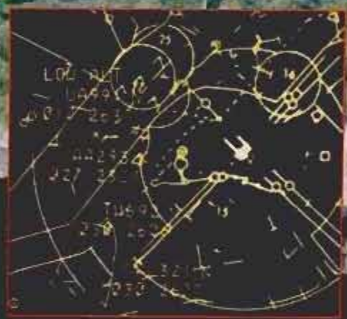
Simulated scene of an airliner flying too low and in danger of crashing into Manhattan skyline is shown pictorially and also (above) as it might look on a controller's scope. The "LOW ALT" warning would flash over the plane's flight number (represented by UA991) and a bell would ring—if the computer were working properly.
