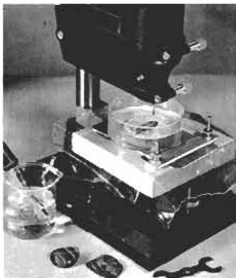
Drilling in stones is done with the Dremel variable-speed Moto-Tool and drill-press stand (No. 210), used by many jewelers.
