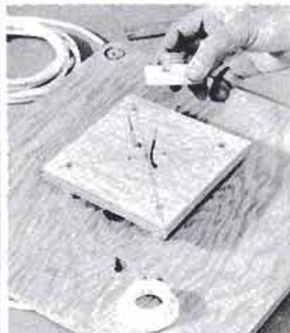
Components ready for test assembly (left): 1. spacer dowels, 2. spacer holding screws, 3. installed rod Teenuts, 4. lamp socket and mounting platform, 5. knotted lamp cord. Test assembly complete (right): Wire leads pass through platform into socket.
