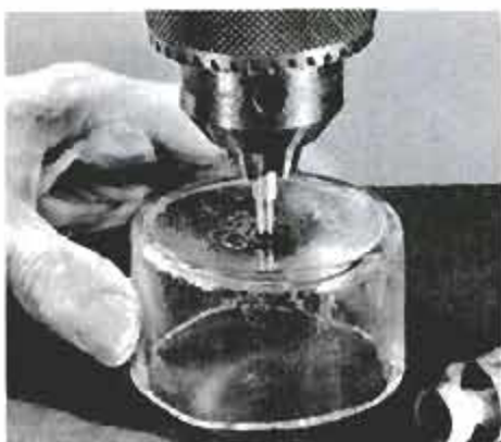
A ¼-in.-dia. hole is drilled in the bottom half of a glass jar, using a drill press with a brass bit and abrasive compound.
