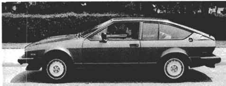
The GT V6 sits on a fairly trim 94.5-in. wheelbase, but weighs in at a chubby 2,800 lbs.
