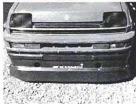
In order for a front air dam to be really effective, it must almost touch the ground.
