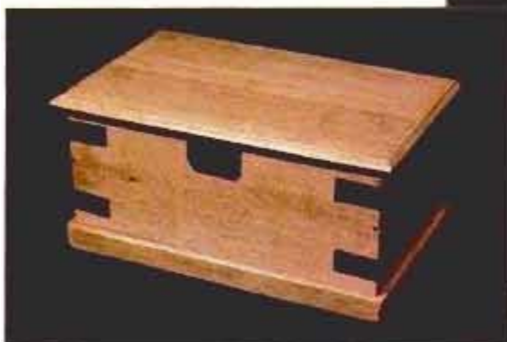
Our lidded reproduction is crafted of \frac{1}{2} - and \frac{3}{4} -in. cherry; we added a tray for chisels and such. With lid down, box can be used as a coffee table with storage.
