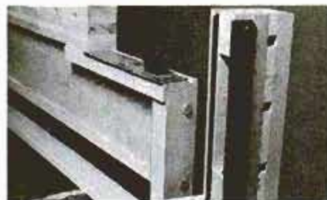
18 Back plate has been removed from test assembly of tail vise and attached to slab. Slot by which vise moves over large nut is now visible. Place vise, add lower guide plate and tighten the two nuts.
