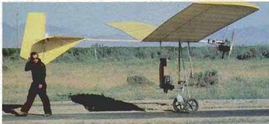
Woodhopper is so light and free-rolling, one person can walk it to and from the field. Hand-cranking prop to start engine is easier with a helper, but can be done by yourself.
