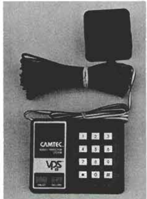
Camtec antitheft device keeps the ignition disabled until you punch in your code.
