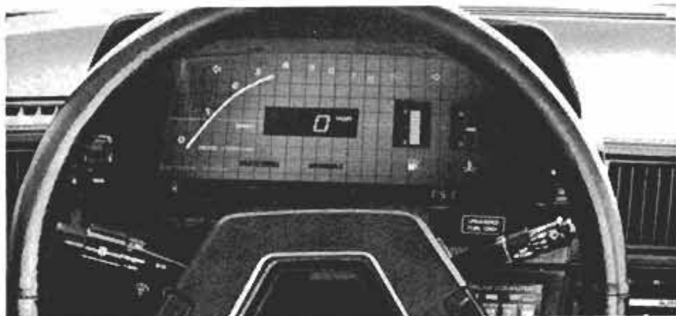
Digital dash with a tachometer that simulates a torque curve is rather gimmicky, but we liked it. Among the other features are a trip computer and eight-way adjustable seats.
