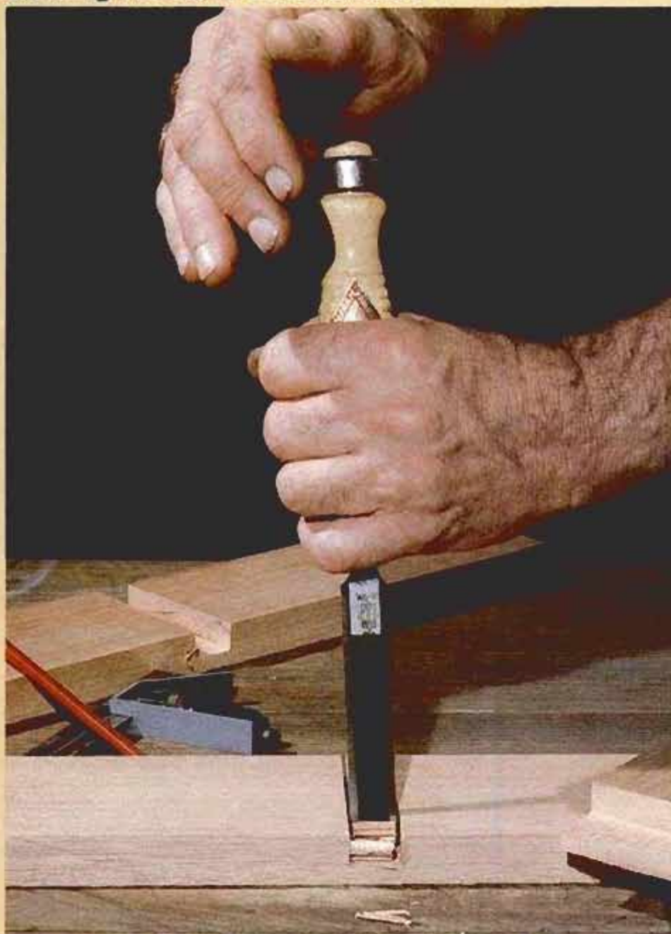
To make a dado with hand tools, you first cut the width lines to the desired depth with a fine backsaw. Then use a sharp chisel to clean out the interior portion.
