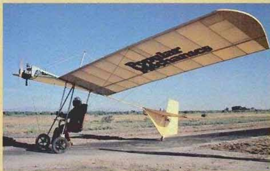
Classic taildragger configuration saves weight and simplifies construction. Bonus: Tail wheel turns with rudder, affording easy, one-control steering on the ground or in the air.
