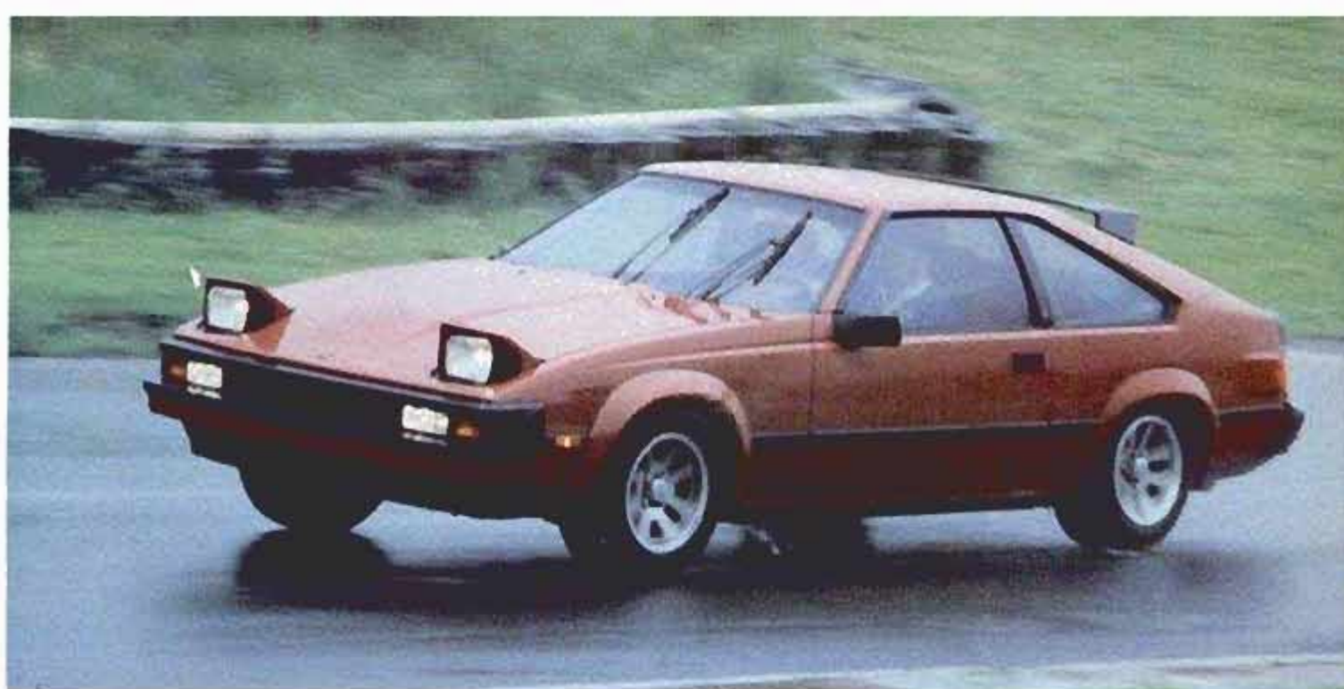
Celica Supra is powered by a dohc fuel-injected Six that produces 145 hp. Pop-up lights distinguish Supra from the other models.
