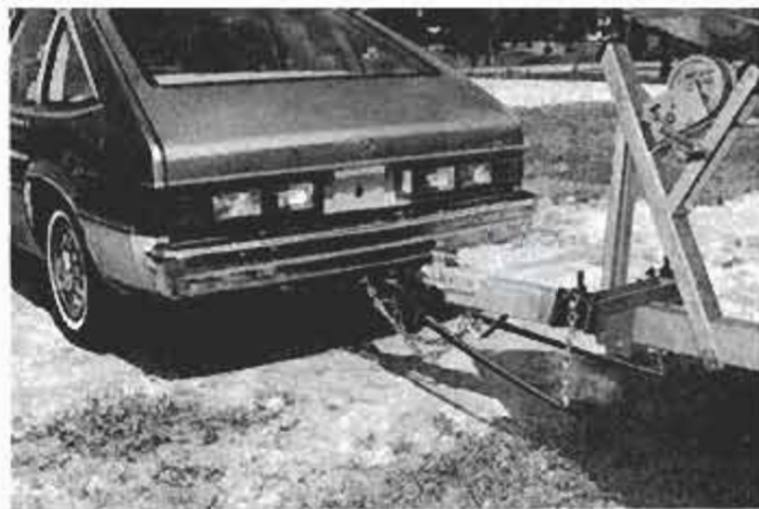
In addition to the load-leveling of the hitch, sway bars secured below the trailer tongue will prevent the rig from fishtailing.
