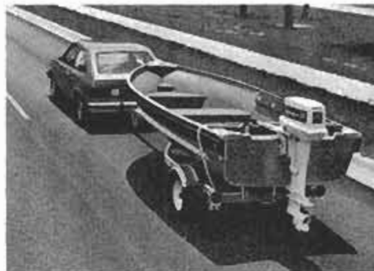
Small car towing a light aluminum boat needs Class I hitch (under 2,000 pounds).
