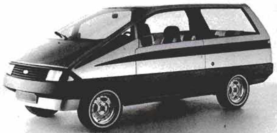
Experimental Aerovan has a small, 94-in. wheelbase but will hold seven passengers.
