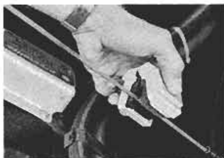
Dipstick wiper has adhesive back which allows it to be stored under your hood.
