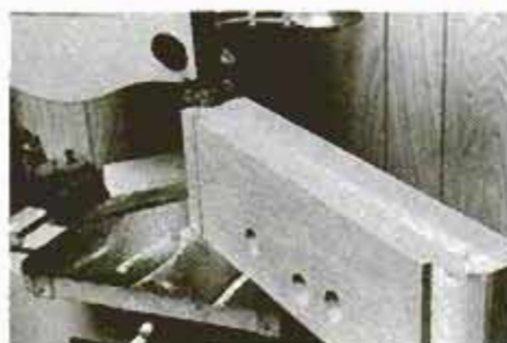
20 Front vise jaw is cut to size. Oversized through-holes have been bored.
