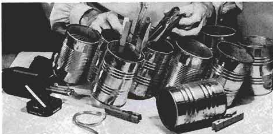
After center row is soldered, spring clamps or clothespins hold cans in place on sides.
