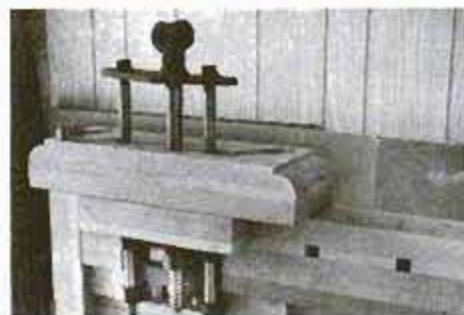
22 The final step in the front-vise assembly is attaching front plate to the vise jaw.
