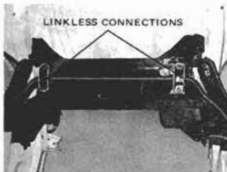
Linkless sway bar installed on the Super-Ks saves several pounds of weight and improves the handling over rough roads.
