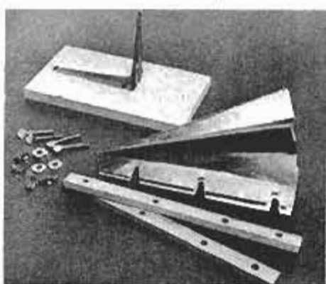
7 Clip openings in the flanges with tin snips. Thumbscrews, wingnuts and washers hold the flanges together.
