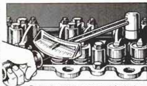
Beam-type torque wrench is the least expensive type you can buy. Reading is taken from the dial and the needle in handle.
