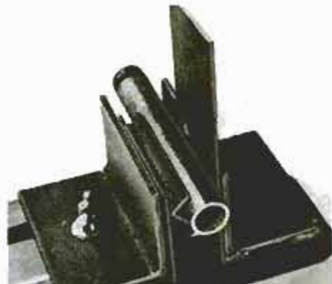
An angle-iron V-block is welded near one end of a \frac{1}{4} \times 3 \times 3 -in. steel plate to hold round stock. You can rotate the plate end for end or on its side as needed.
