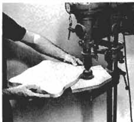
11 After cutting top to shape with band- or sabre saw, remove saw marks from edges with a 2- or 3-in.-dia. drum sander. Otherwise, router will follow ridges in next step.
