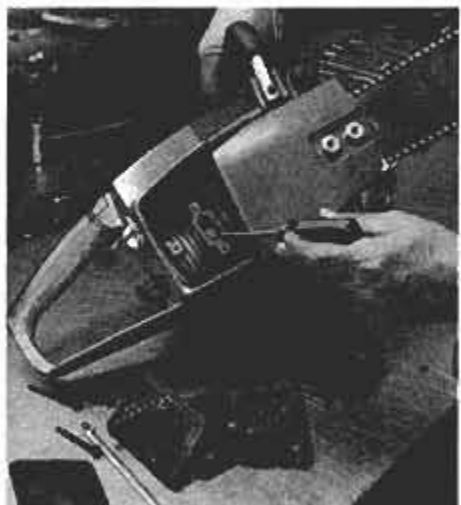
10 Screwdriver points to an area near combustion cylinder where carbon accumulation may occur. Remove muffler to expose area and clean away carbon.
