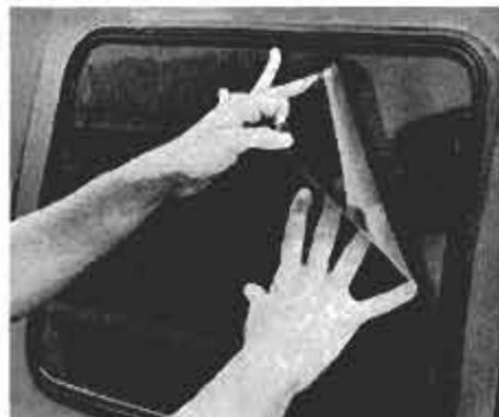
Window-tint film, which is illegal in some states, is applied on exterior of glass.
