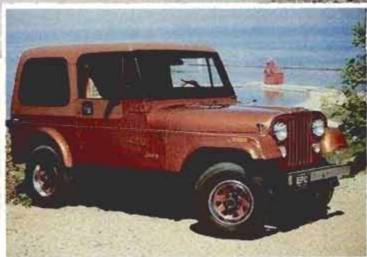
Jeep CJ-7 Limited offers a wider track than the standard CJ-7 for better stability on paved roads. It also has a bigger fuel tank.
