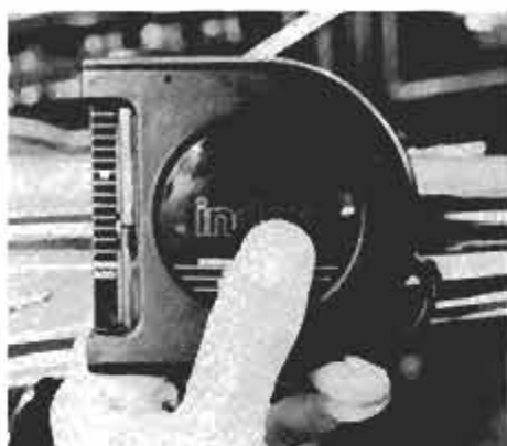
Oil-level indicator mounts inside the car and gives reading with the push of a button.
