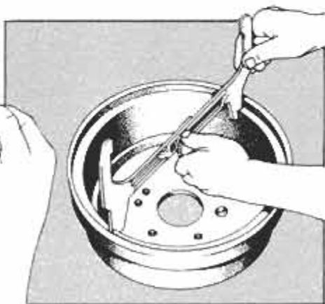
Brake-shoe adjusting gauge allows you to check installed tolerance between the brake drum (below) and brake linings (left). It also checks amount of metal removed if drums are cut on a lathe.
