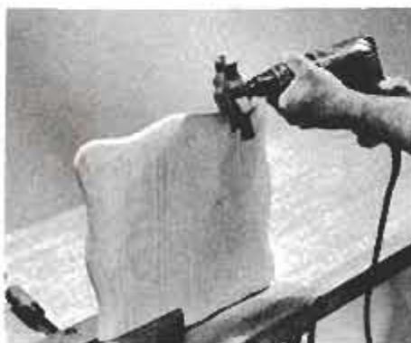
17 Flap-type sander, such as a Sand-O-Flex wheel, makes the final sanding easy.
