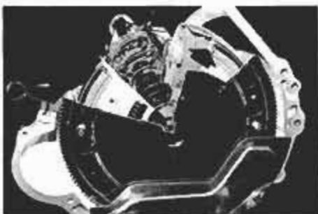
Spring-loaded friction shoes on C-5 automatic tranny offer smoother entry into overdrive mode, add 2 mpg on the highway.
