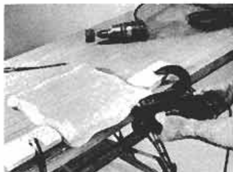
15 A small belt sander (the Sandcat here) and a fine-grit sandpaper help to complete this stage of the shaping operation.
