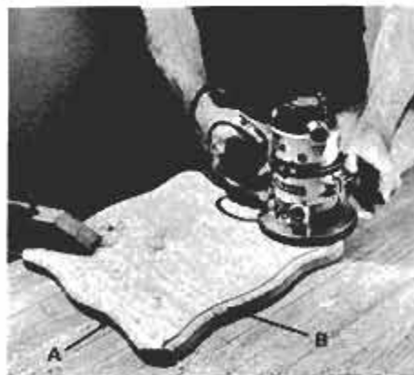
12 Top is cut to shape, then rounded with a 3/4-in. rounding-over bit and router. Avoid damage to wood by making two depth passes (A is after one pass; B after two).
