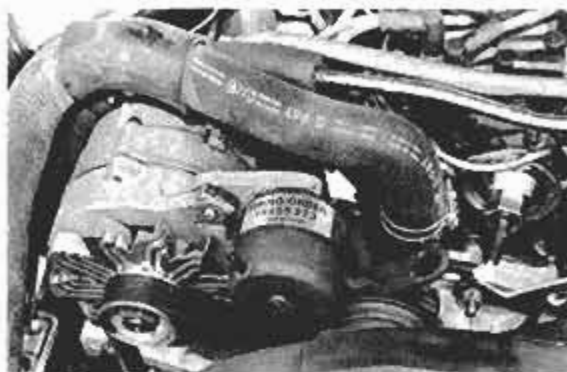
Twin-snorkel air cleaner is the tipoff that a high-performance, 5.0-liter V8 is in residence. The twin snorkel provides freer breathing, since the new radical cam profile needs extra oxygen. New cam also changed the firing order, which is now printed on a decal on the automatic belt-tensioner (arrow left).
