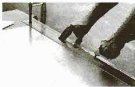
Aluminum sheet is easily cut with a utility knife in a couple of passes. Clamp a metal straightedge in place for use as a guide.
