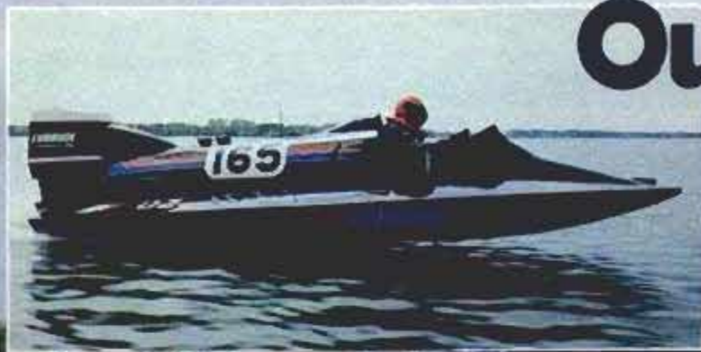
Evinrude's and Johnson's V8 racing machines with 3.5 liter (214-cu. in.) displacement will be making their debuts in speedboat races in Europe.
