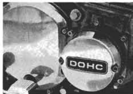
Chrome-molybdenum Allen screw set replaces Phillips screws on motorcycles.
