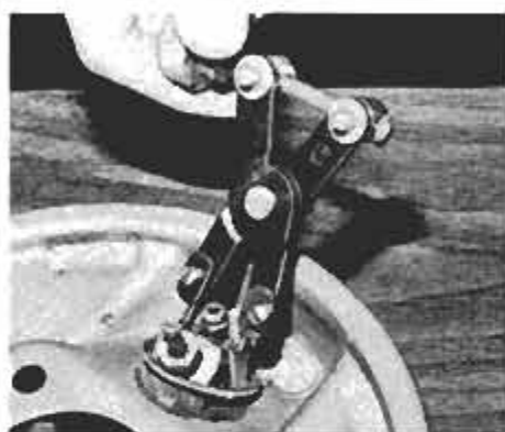
This clip remover makes fast work of taking off most rear cylinder retaining clips.
