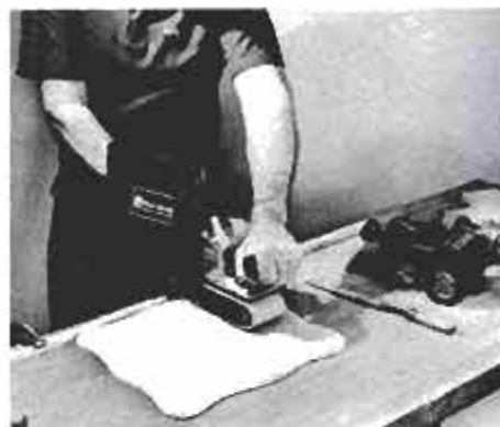
16 Switch to larger sander and smooth both flat surfaces of tabletop. Go with grain.
