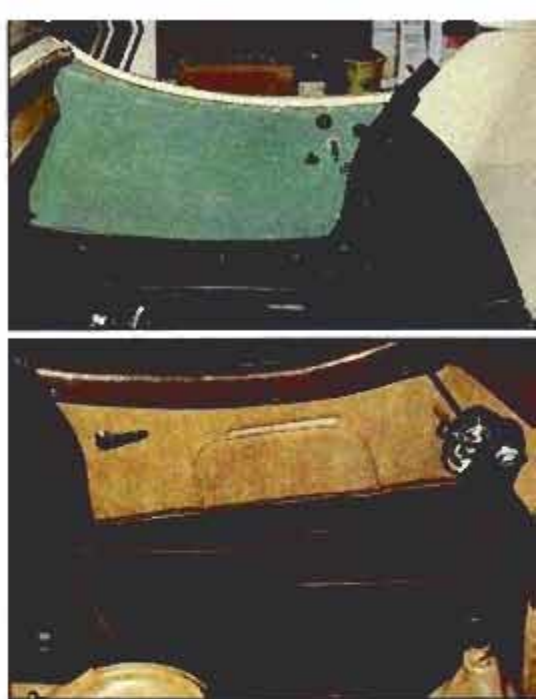
When shipped, the door is mounted, but bare (top). Door finished with upholstery supplied with the kit is shown above.
