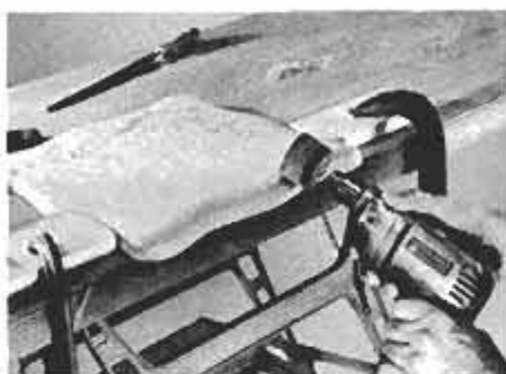
14 Now mount the drum sander in your portable drill and while the workpiece is still clamped between shop-made blocks, sand off all tool marks that are visible.
