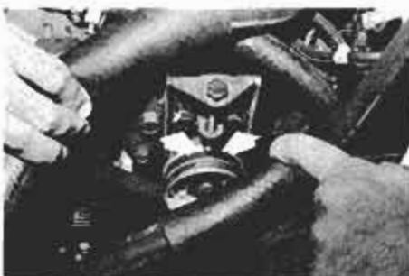
New V6 has no automatic belt tensioning. Tension is adjusted by loosening two bolts, and setting it with center bolt (arrows).
