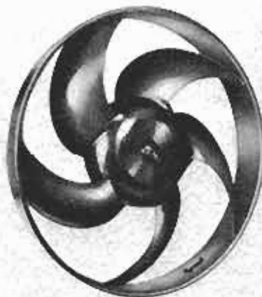
New cooling fan reduces the amount of power needed to pull air across the radiator. The blade design improves airflow.
