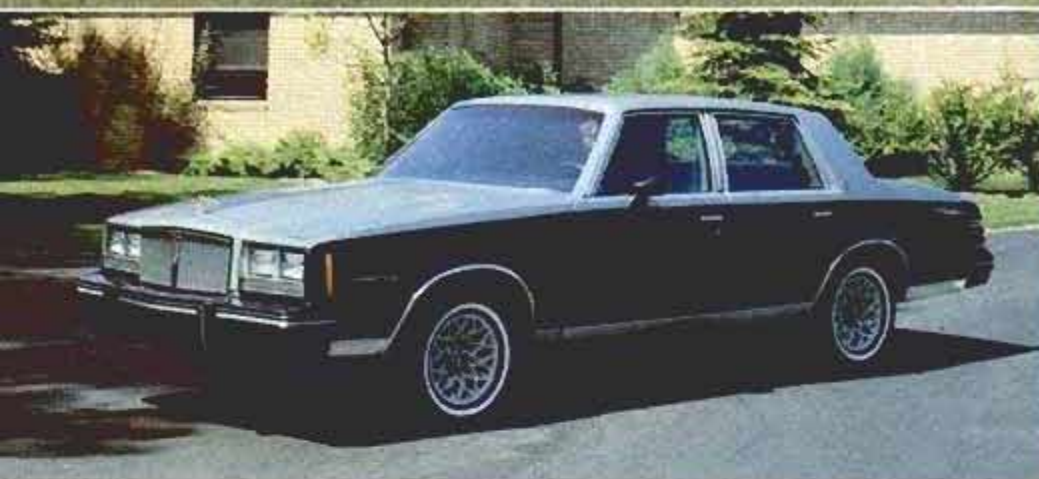
Pontiac's '82 Bonneville has 108.1-in. wheelbase. Standard engine is 3.8-liter V6; two gas V8s and diesel are optional.
