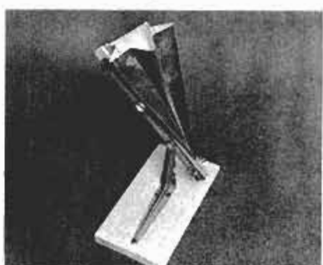
8 You can tilt the mold to achieve slanted patterns using wax of more than one color. The shelf bracket of the stand is notched to allow thumbscrew clearance.
