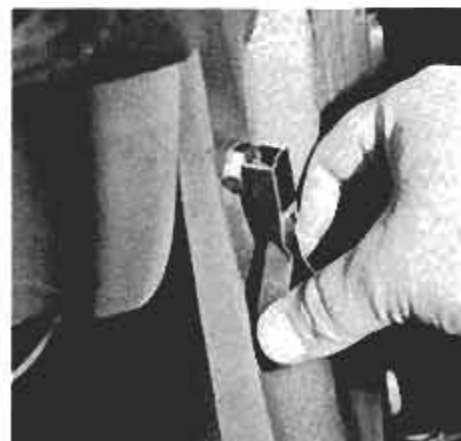
Spring clip holds in button, shuts buzzer when you need to leave car door open.
