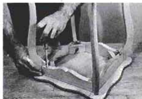
33 Table is assembled using match marks as reference. Glue, screw aprons to top.
