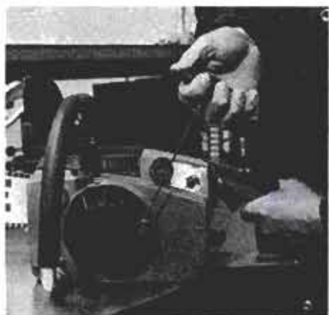
8 Pull starter rope to check for proper recoil-spring action. Spring adjusts easily if necessary. Keep the air intake louvers clean around the starter.
