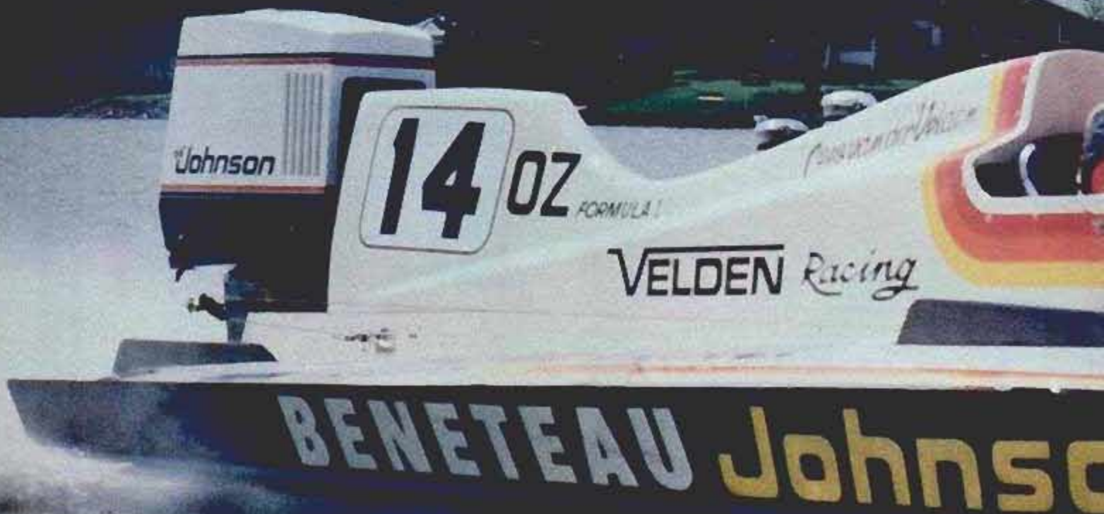
Evinrude's and Johnson's V8 racing machines with 3.5 liter (214-cu. in.) displacement will be making their debuts in speedboat races in Europe.
