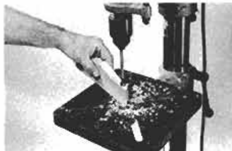
9 Aprons are cut to shape and locations for screws marked. Counterbored hole is made first with Power Bore Stanley bit.
