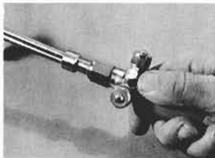
Torch is well balanced and has a comfortable grip. Oxygen is fed to work surface by pressing the button with your thumb.
