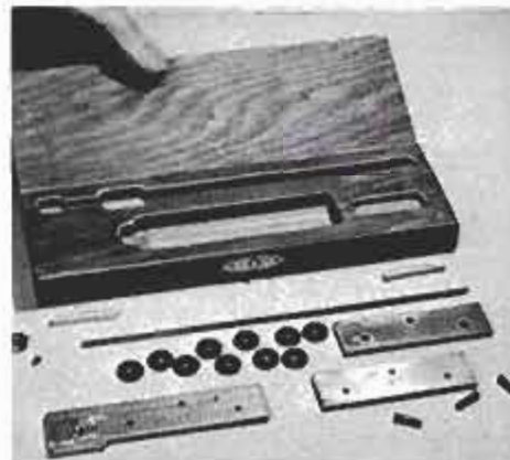
Parts of wiggle gauge, including safety caps for the points, are shown in front of handy storage box. Make box from \frac{1}{2} -in. plywood with \frac{1}{8} -in. plywood for top.
