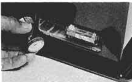
Two 1.5-v. batteries give ignition power to starter. These are housed at the rear.
