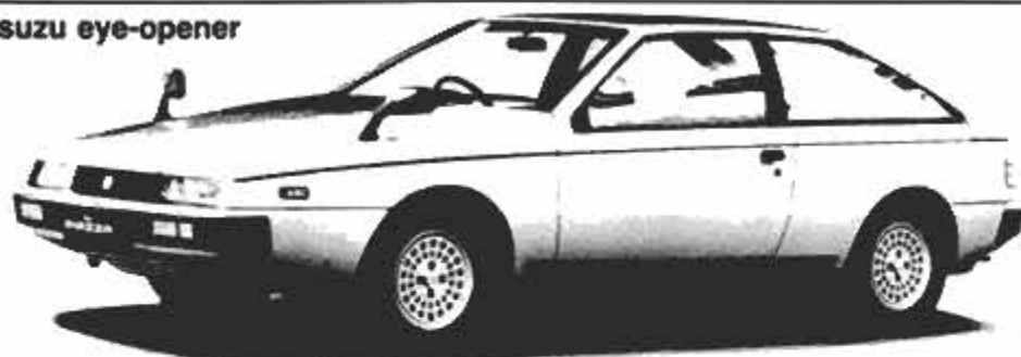
Isuzu Piazza with two-liter, single-overhead-cam Four gets 120 hp, with dohc, 135 hp.
