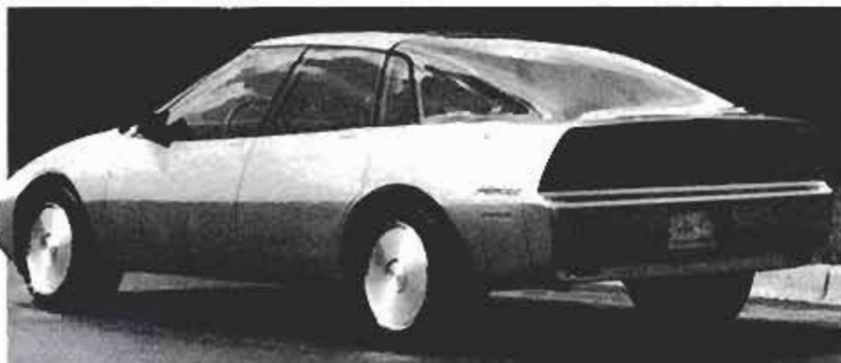
GM's experimental Aero-X car is based on Citation chassis, has room for four adults and has a Cd of just .295. Note the use of the Kamm tail and flush wheel covers.
