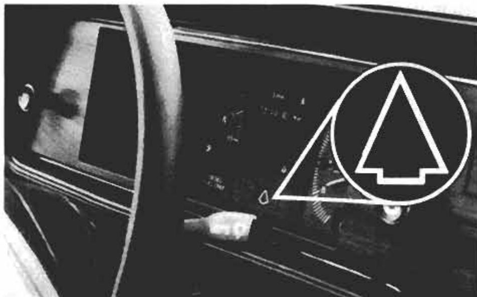
E (for efficiency) light on VW diesels blinks on to tell you when to upshift. According to Volkswagen, upshifting on cue from this light should improve mileage considerably.
