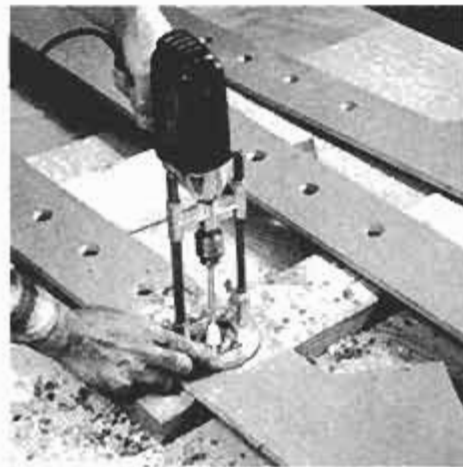
Use a drill press or portable drill guide to assure boring the holes straight. Place workpiece on scrap and bore through for a clean hole. Pilot holes make job easier.
