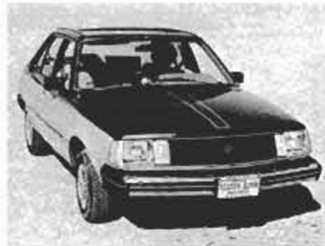
The 18i owes its fine handling to front-wheel drive, all-independent suspension.
