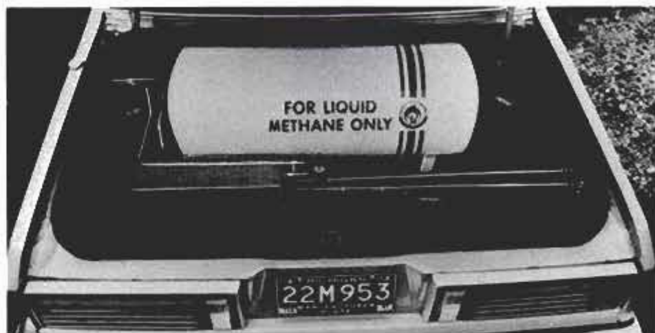
The fuel tank that holds liquid methane is fitted snugly into the trunk of the Fairmont.
