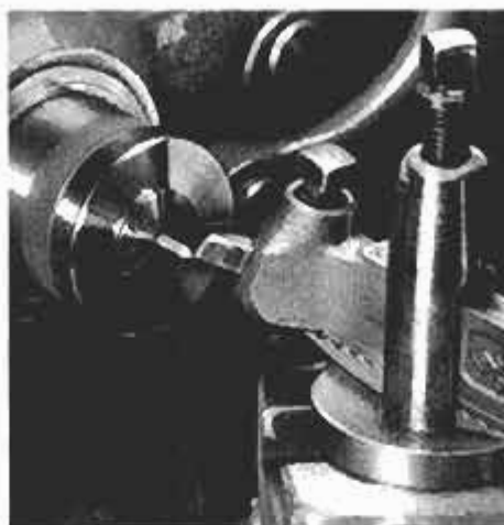
A 60^\circ point is machined on one end of the drill rod. Tool bit was inverted in holder and fed from the back for photo clarity.
