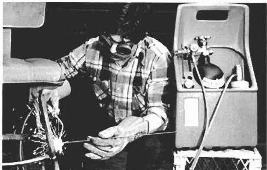
Repairing broken leg support of a chair is a job easily handled by the Tote-Weld. The complete kit, including gas cylinders, comes in a sturdy plastic carrying case.
