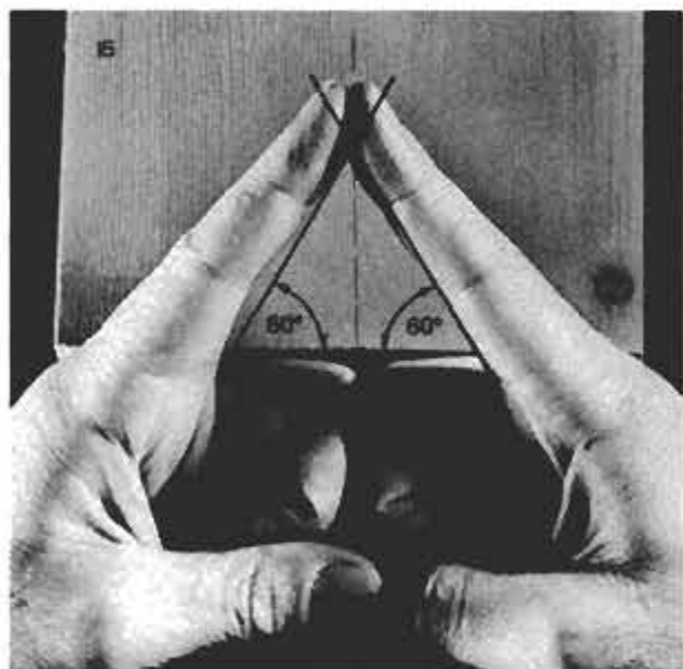
By placing fingers as shown you'll have a "protractor" with quick 60^\circ angle and perpendicular line references.
