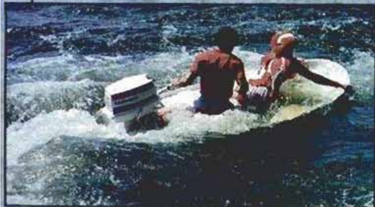
Even full of water, the Flying Flivver can power along with a high-mounted outboard, and bail itself out as the speed increases.
