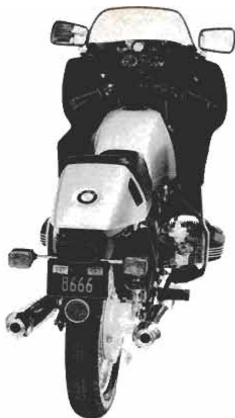
Full-frontal fairing, like this on BMW, provides best protection from the weather.
