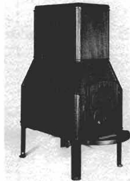
Jotul's cast-iron wood stove model No. 121 can put out 75,000 B.T.U./hr. with optional heat exchanger (uppermost section) or up to 49,000 B.T.U./hr. without an exchanger.
