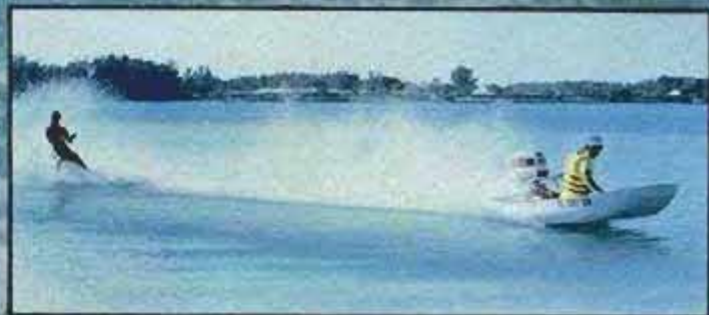
An experimental, lightweight model pulls a barefoot water skier; it can tow three or more on skis with a 25-horse outboard motor.
