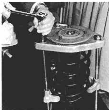
Heavy-duty MacPherson-strut spring compressor is for larger springs of GM X-cars.
