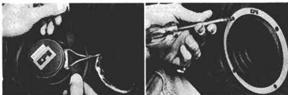
When installing front speakers in car doors, check that the wiring is of correct polarity, and make sure that speakers do not interfere with the window-cranking mechanism.
