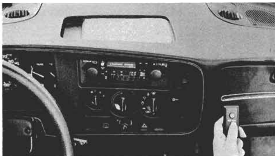
Remote-control scanning of AM/FM stations with handheld switch is one feature of 3001. Saab saves you job of installing front speakers: They're built into top of the dash.
