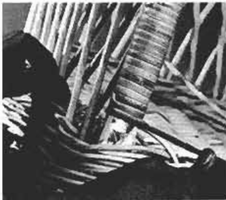
A leg is rewrapped with cane strands. A double wrapping goes around the V-shaped reed at the point where it abuts the leg.
