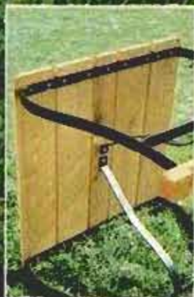
Furniture is built of oak and strips of mild steel. Countersunk nuts and bolts join the parts.
