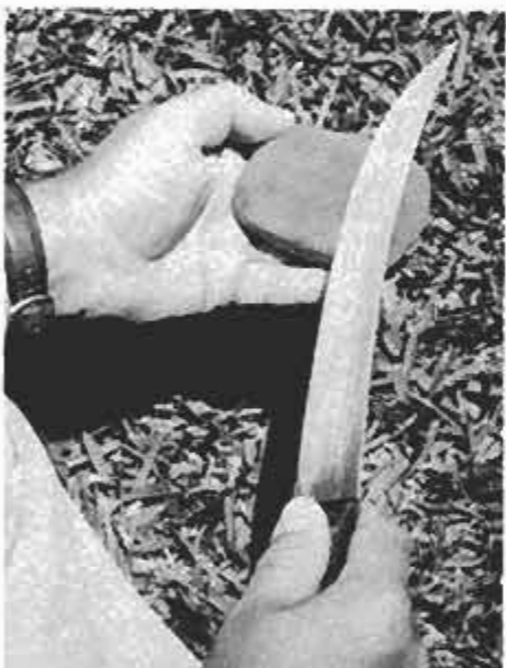
Even a rock will serve as a makeshift whetstone. Using a dull knife or ax requires extra pressure that may endanger the user.
