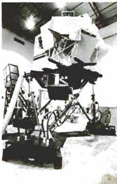
Cockpit, surrounded by a shell, permits visual effects, rides on six moving legs.
