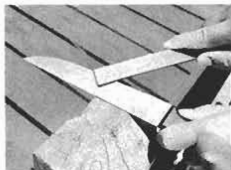
Versatile rectangular file, with short strokes to keep fingers away from blade, sharpens knife quickly. Oil against rust.
