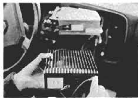
Remote-control scanning of AM/FM stations with handheld switch is one feature of 3001. Saab saves you job of installing front speakers: They're built into top of the dash.
