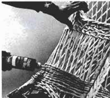
If you wait until repairs are completed before applying clear liquid hide glue, you can make corrections to rattan, if needed.
