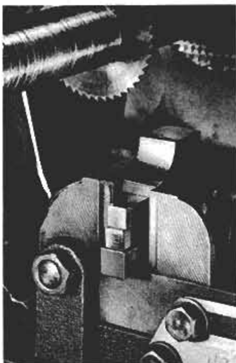
Three shims of different thicknesses produce combination needed to hold one or more workpieces square and in position.
