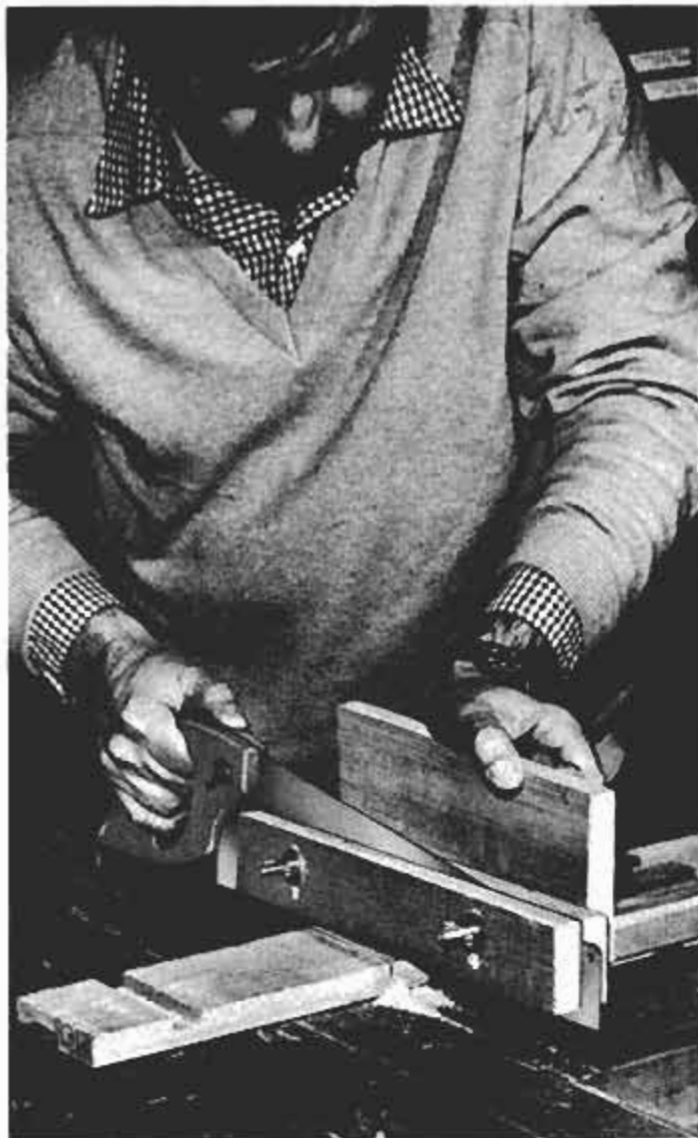
Saw with depth stop cutting a dado. In the left end of the board is a dado that was cut with this tool. Keep saw teeth sharp to make clean cuts. When using the saw guide, clamp board between the T-square head and guide jaw with a moderate grip.
