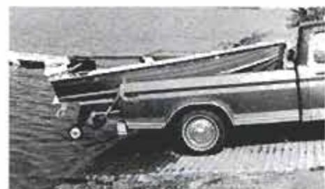
A pickup can replace a boat trailer for craft up to 14 feet with Winch-It System from Fluck Inventions, Perkasie, Pa. 18944.
