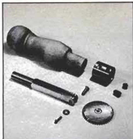
A disassembled wheel tool and its parts. Guard and its screws aren't shown, but one should be used in all cutting operations.
