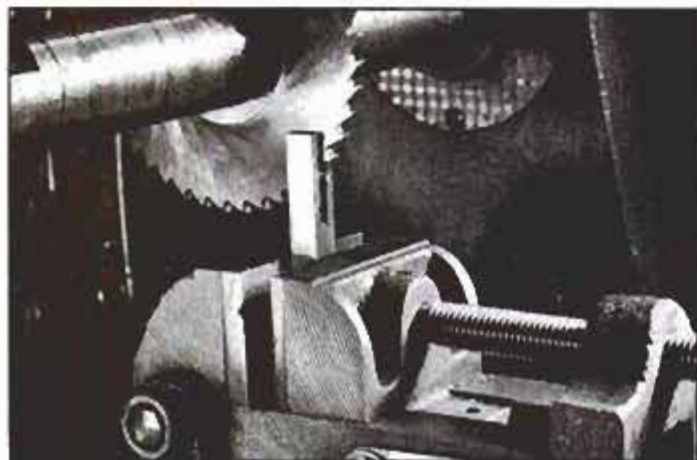
Wheel slot is cut in fork with a milling cutter. Axle hole, not shown in photograph, should be bored before you mill the slot.
