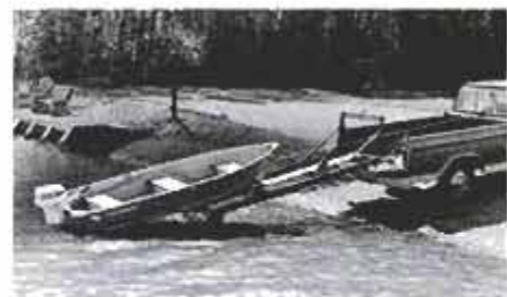
For launching or hauling out, Winch-It uses a rolling cradle, winch secured in truck's stake holes and tailgate cable supports.
