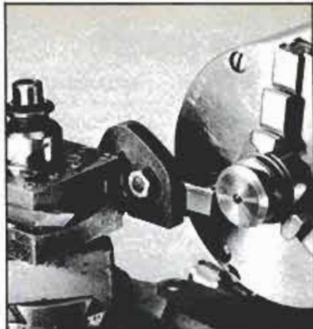
To form a creasing wheel, like No. 1 in the drawing, cut gear teeth completely off and machine the wheel to the desired shape.
