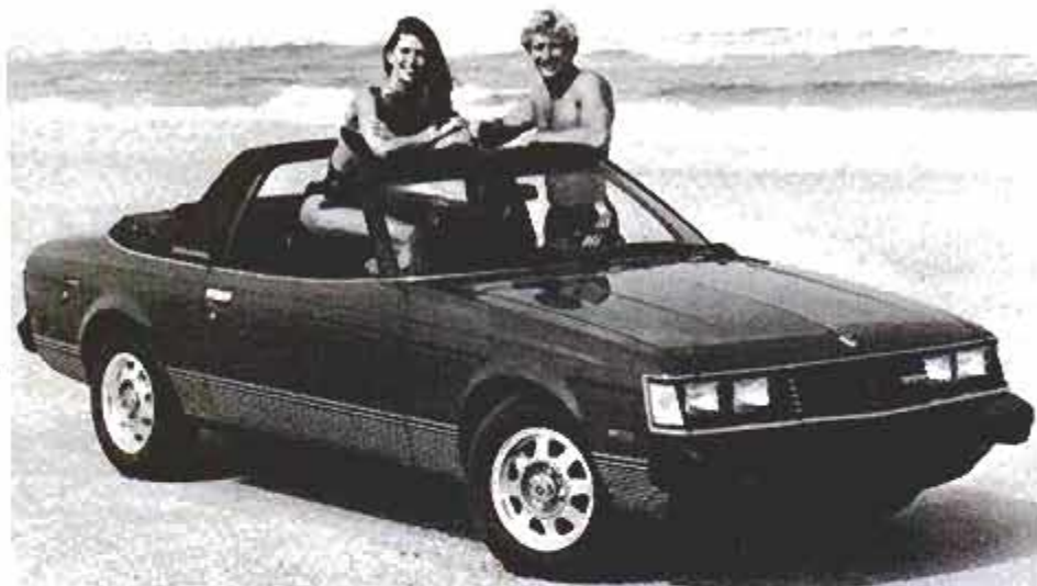
Sunchaser from the Griffith Company of Fort Lauderdale, Fla. has a Targa top with removable roof panels. The rear basket handle is a roll bar and body brace. Mustang convertible (below) is from Contec of Lake Geneva, Wis. that also converts Firebirds.
