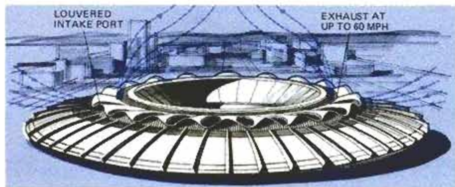
Air velocity in proposed dome system would vary depending on rain intensity, with a maximum speed of about 60 mph. Louvers restrict entry of moisture into the blowers.
