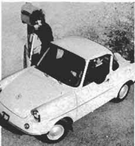
Mazda R-360 had a V-twin, air-cooled engine, which propelled it to 65 mph. This two-seater averaged over 60 mpg.
