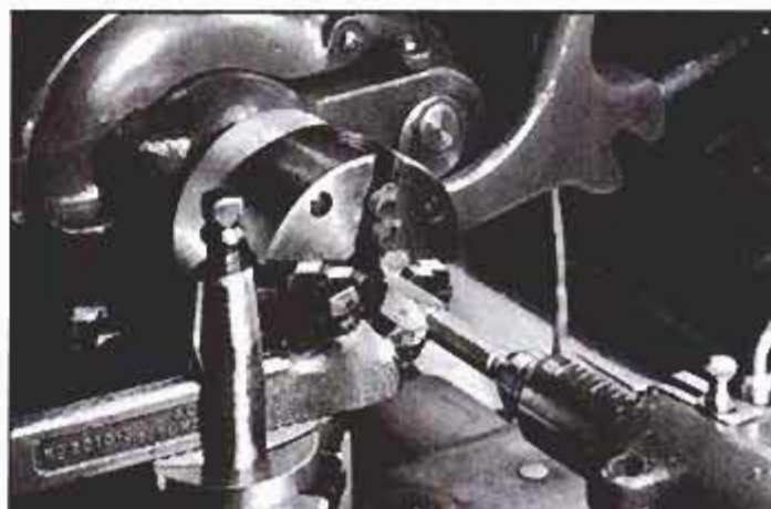
After the slot is milled, reverse the fork in the chuck and machine a 3/4-in.-dia. shank. Then insert fork in the handle.
