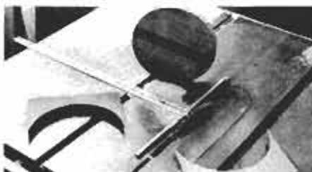
The finished disc requires only a small amount of sanding. Large work takes proportionately longer cutting time, but the results you obtain are equally good.
