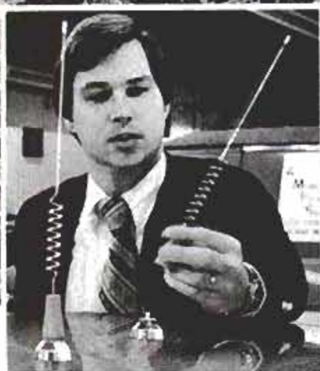
Rooftop antennas for cars have coiled segment, so they're small and easy to install.
