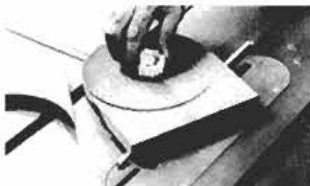
Small work like this is safely rotated with the knob. After each pass, the blade is raised 1/8 in. until cut is done.
