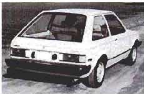
The GLC features a unique rear suspension in which rear tires toe-in under cornering.
