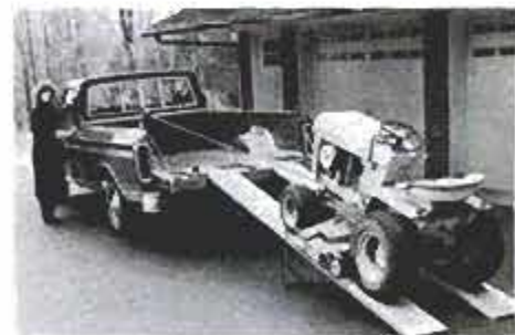
Garden tractors, snowmobiles, motorcycles can also be loaded with quickly installed, hand-winch Fluck system.
