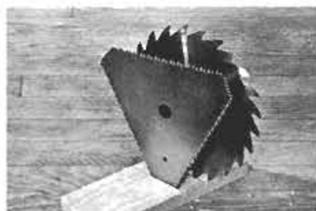
Triangular-shaped Crazy Saw is about the same size as a 7-in.-diameter blade.
