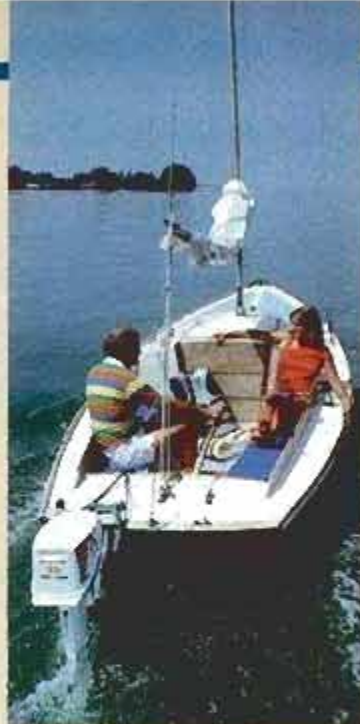
When the wind dies down, a transom bracket that hinges down and mounts a long-shaft outboard with top controls can power a sailboat home.
