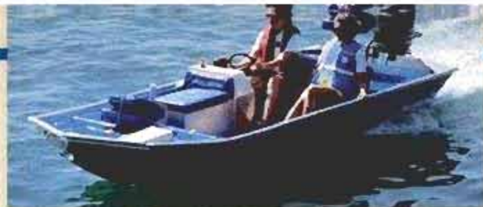
Fisher Marine's 16-foot aluminum Water Strider III-V, weighing 510 pounds, is rated to 60 hp, but with its Controlled-Vee hull, planes with 25-hp Mercury at economical two-thirds throttle.
