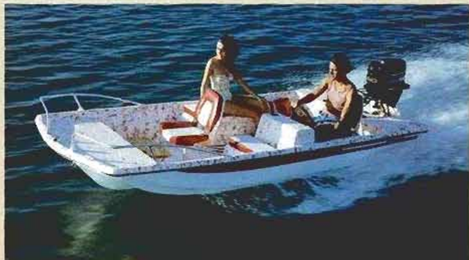
No longer ranked with the large engines, this 50-hp Mercury can pull several water skiers, tops 40 mph, but cuts fuel consumption almost in half at cruise throttle.
