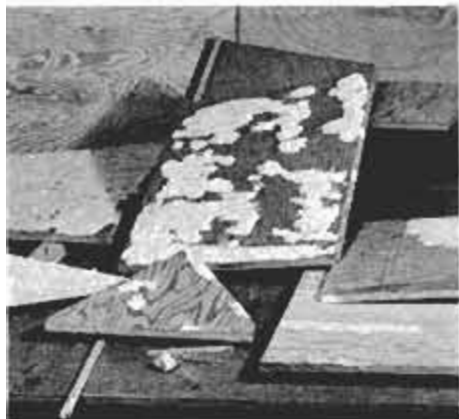
Use compound such as ZAR Wood Patch to fill voids and blemishes before assembly.
