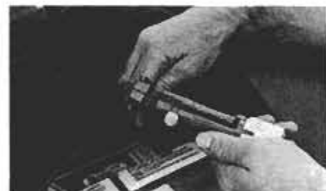
Battery-cleaning tool removes corrosion.
