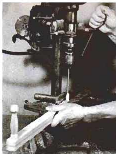
To bore holes, center-punch after clamping two strips together. Insert peg or dowel in finished holes and bore other end.
