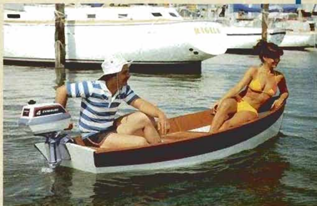
For yacht harbor dinghies, a smaller motor is safer on hulls with low freeboard and helps young skippers slow down to the tame, no-wake speeds that are required.
