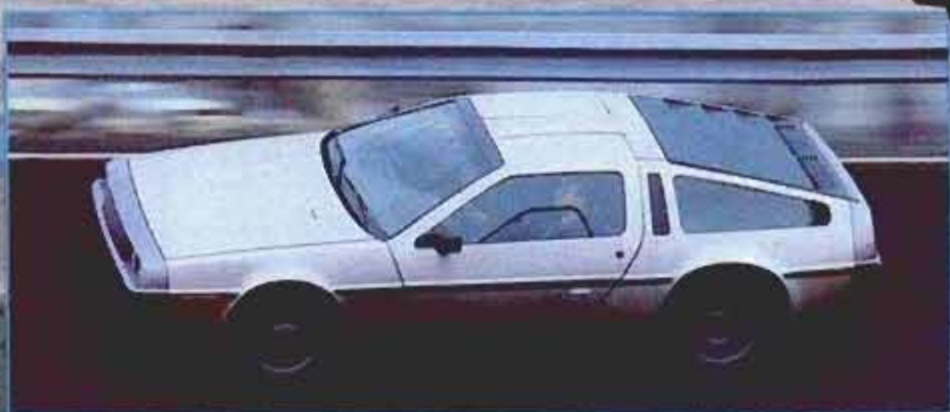
Short, 94.8-inch wheelbase and a low center of gravity give the car excellent handling characteristics and fast transient response.
