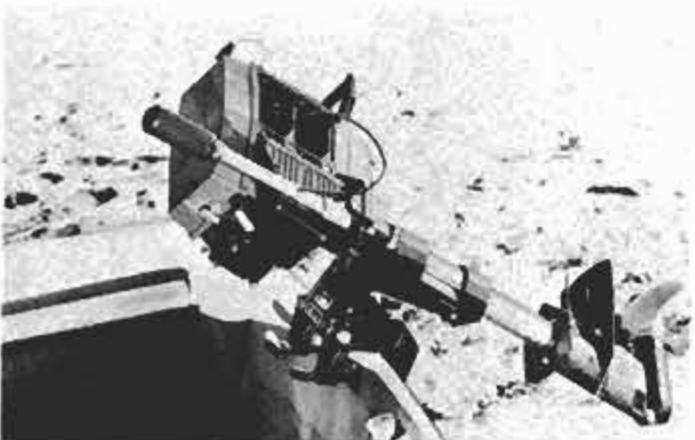
Among imported models is the Flat Nautica Whitehead, made in 8 and 14 hp, with adjustable shafts in lengths up to 34 inches.
