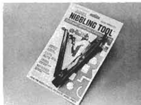
The tool's squeeze handle drives a spring-loaded punch that does the nibble cutting.
