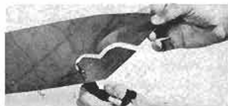
The Nibbler cuts 16-gauge copper sheet, and it can perform equally well on plastic.
