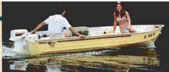
Even when rated for bigger motors, a light aluminum skiff like this one from Mirro Craft can be set up to get up on plane with a mill the size of a Johnson Sea-Horse 9.9-hp outboard.
