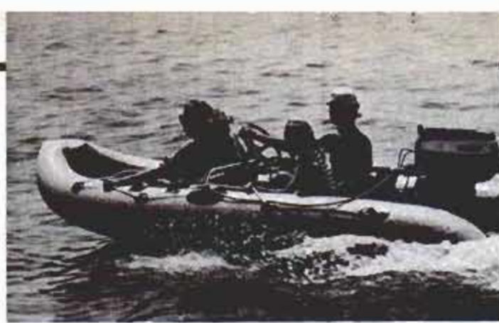
Using the remote steering recommended for safer control of big motors, Metzeler 12-foot inflatable mounts a 25-hp Yamaha.
