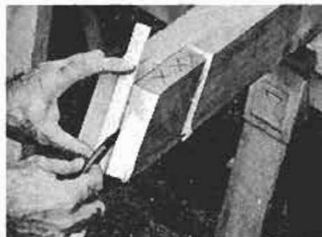
To avoid error, use a felt pen to mark a clear line; the Xs show which side is waste.
