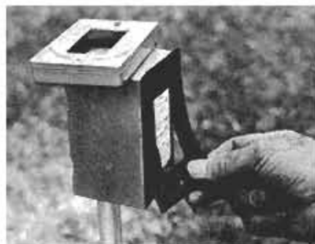
Waterproof gasket is inserted over the receptacle. The cover seats tightly against it.
