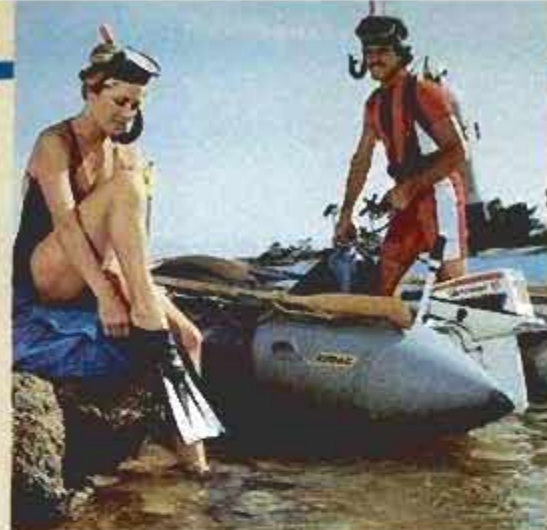
New design improvements, like Zodiac's inflatable keel, give vee shape to bottom and provide smoother ride while handling bigger, faster motors.
