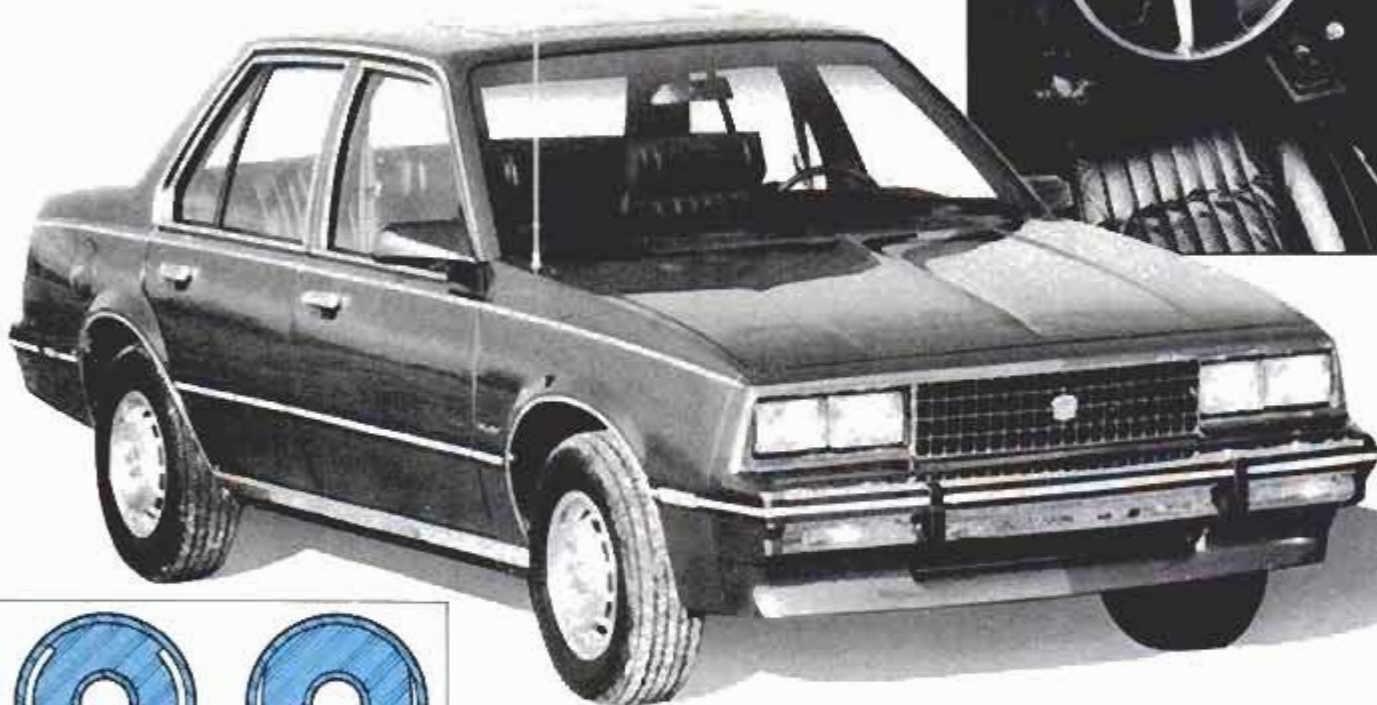
Cimarron is the smallest Caddy ever, but still features luxury interiors. Suspension differs from other J-cars: Smaller air gap in trailing arm bushing (below left) reduces oversteer.
