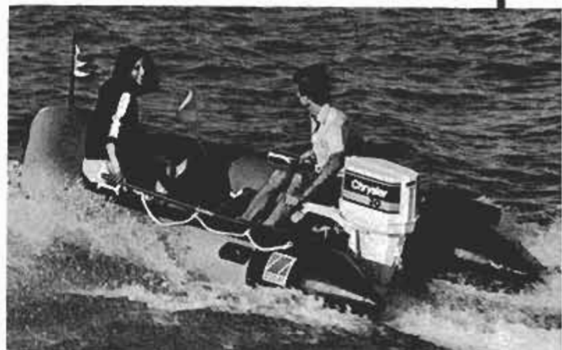
Small inflatables like this Zodiac can now handle powerful motors like the Chrysler 30. Zodiac 19-footer takes up to 115 hp.
