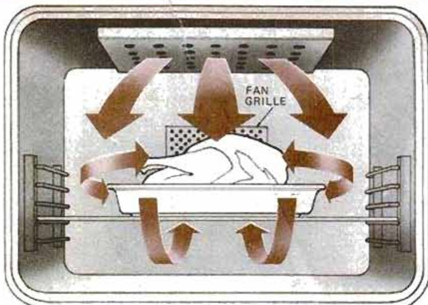
In a convection oven (above), the heated air is drawn across the top of the food, around the sides and under the bottom to cook evenly.
