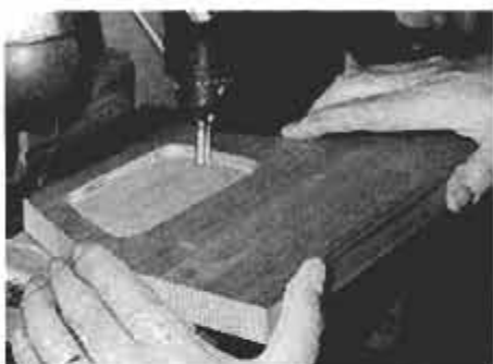
Recesses are routed in the truck sides to simulate authentic-looking cab windows.
