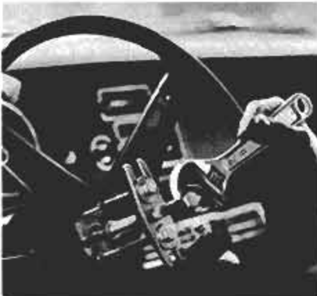
Special tools like the wheel puller won't be used often, but they're useful to have. When you really need them, nothing works better.
