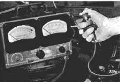
A limited-function dwell/tachometer will perform adequately for basic tuneups.
