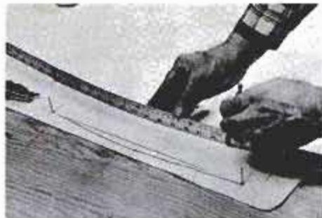
Flexible rule is used to draw the pattern for the curved cutouts. Rule is deflected \frac{1}{2} in. at center to obtain the required curvature.
