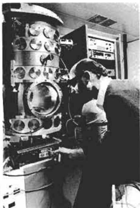
Mirrors are made in high-vacuum chamber.
