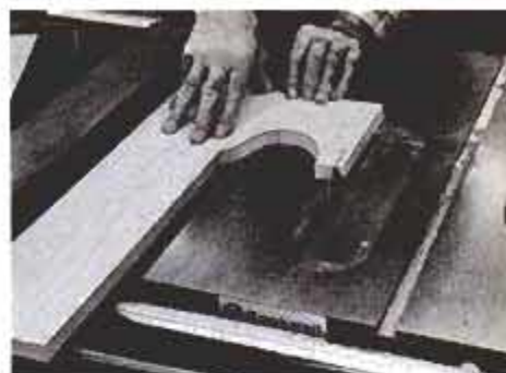
The 35° bevel on the top of the cradle sides is cut after pieces have been separated.
