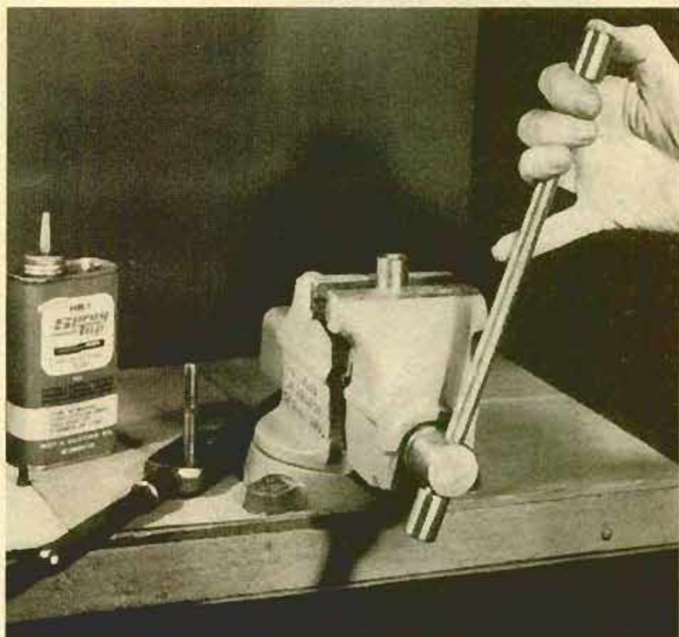
Apply greater pressure in vise jaw with a longer handle you can easily make yourself.
