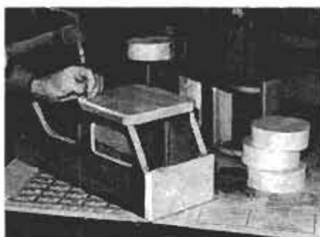
Because truck is for outdoors, assemble it with waterproof glue, finishing nails.
