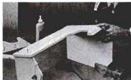
Hand-screw clamps are good for steadying project during assembly. Start the nails, then lift the section off and apply glue.
