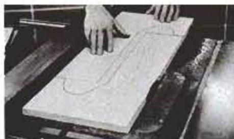
A 7° bevel is cut along both edges of the board. Note that, after you have cut one side, the board must be flopped before cutting the second edge to insure that the bevel angle is properly positioned.
