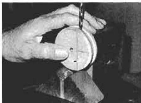
Through-holes in sheaves are bored parallel to diameter, but offset from axle holes.
