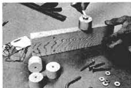
Sand wheels and check for fit. Accessories for car include U-bolt, plastic bubble.
