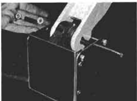
The bucket pivots on end of arm; the spacers on the rod keep the bucket centered.
