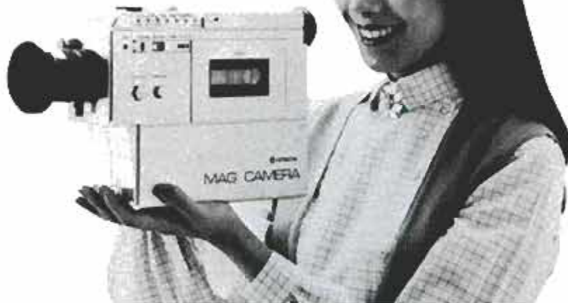
Video is challenging the home movie market, as demonstrated by this prototype from Hitachi. The portable combines a color videotape recorder with a color camera. It can be operated to play back as well as record.
