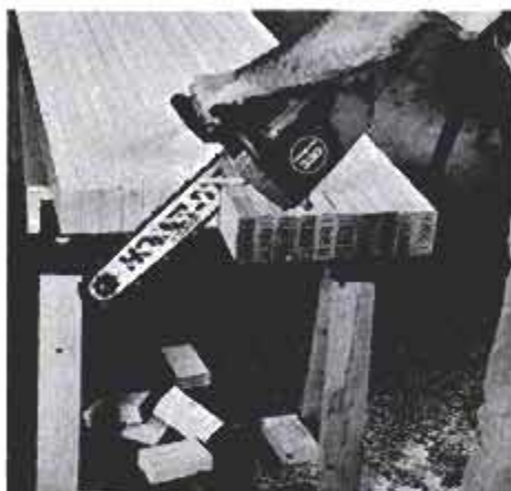
Hold the saw at a 45° angle to trim off the excess. Be sure to keep your body entirely to the left of the chain line.
