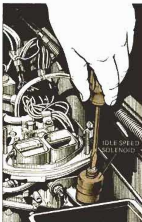
Crankcase emissions filter in Escort and X-body cars are replaced every 30,000 miles (left, Escort). K-car idle speed is adjusted by idle-speed solenoid (right).
