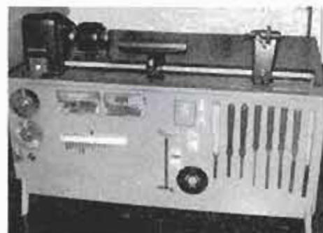
Plywood skirt on a salvaged dining-room table provides storage for lathe tools. Area beneath the table stores large items.
