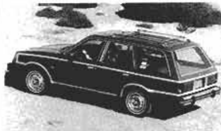
With rear seats folded, five-door wagon can carry as much as 61 cu. ft. of luggage.
