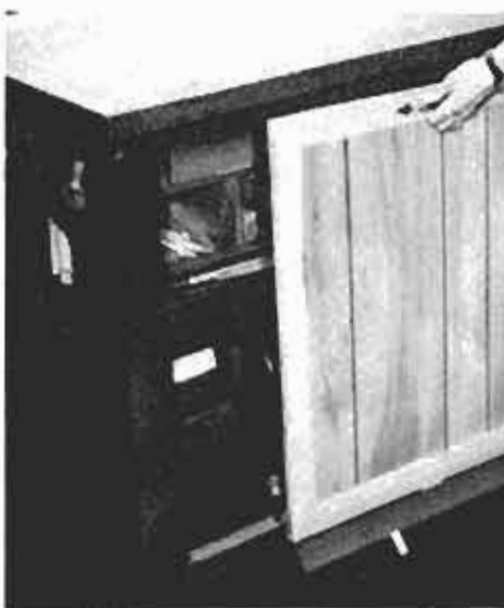
Pull top of door out slightly and lift evenly on door handles to disengage dowels. Lightweight door can be set aside for full access to storage under the bench.
