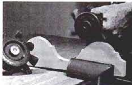
A second version of the flap-type sander features slashed strips, which can be used to sand both the inside and outside cuts of a scroll. The two shown (from Sand-O-Flex) permit you to snip off the worn sandpaper and advance fresh abrasive. The refills keep down the cost of sanding.
