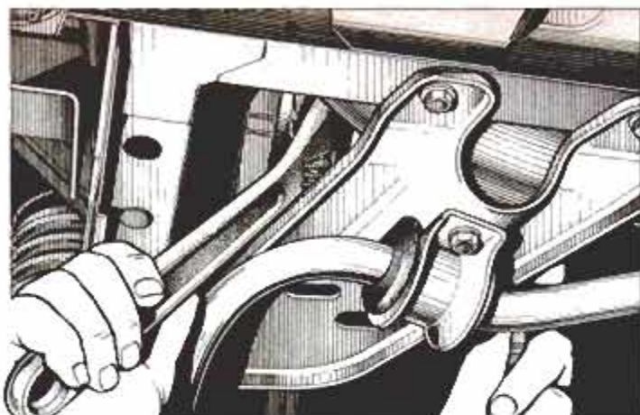
The only way you can adjust drive belts of the Escort is to get beneath the car. This is a very awkward and annoying task.
