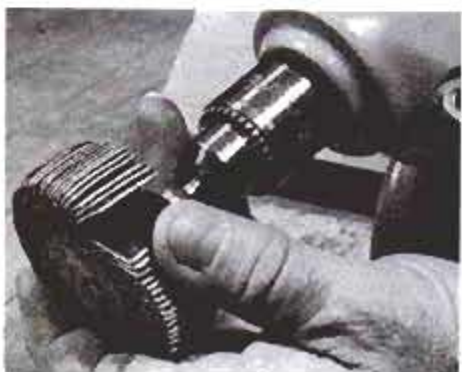
Rugged flap-type sander sports strips of sandpaper around a wheel. This type is excellent for sanding particularly rough scrollwork and other irregular shapes.
