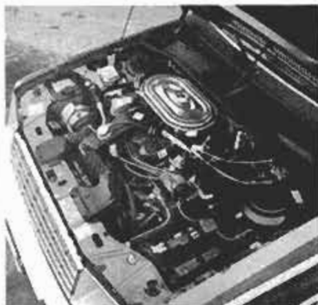
Escort's 1.6-liter ohc Four delivers 65 hp, gets 28/36 mpg according to its owners.
