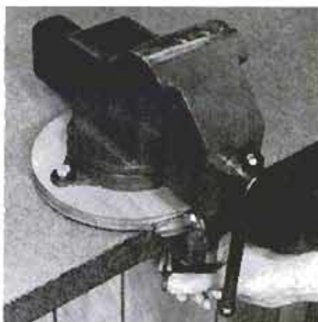
Roaming vise uses clamp that came from dough mixer. It's an easy-to-make clamp.
