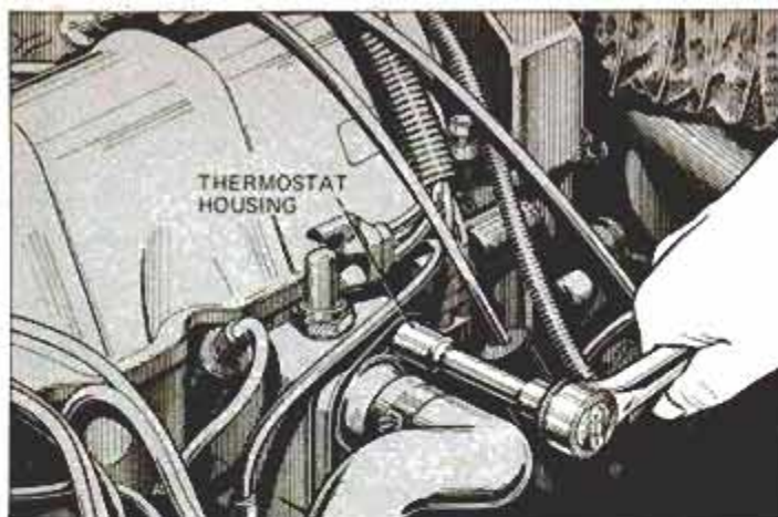
The thermostat housing of the K-car is located at the side of the block. It's a snap to remove and install a new thermostat.
