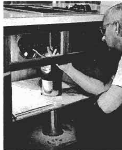
Grease trap below the grill is a glass jar that can be easily removed for cleaning.
