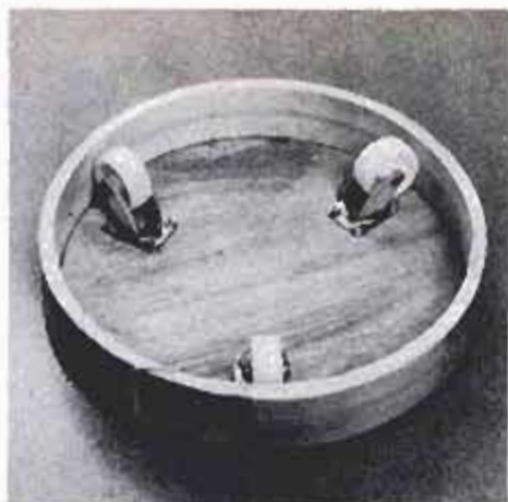
View from bottom: Three plate-type casters make it a snap to move a heavy planter.
