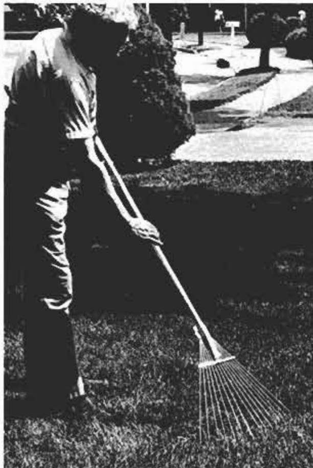
Rake's tines are fully expanded to comb the lawn (photo, left). Adjusting tine expansion (right) is similar to operating an umbrella; here the rake is closed.
