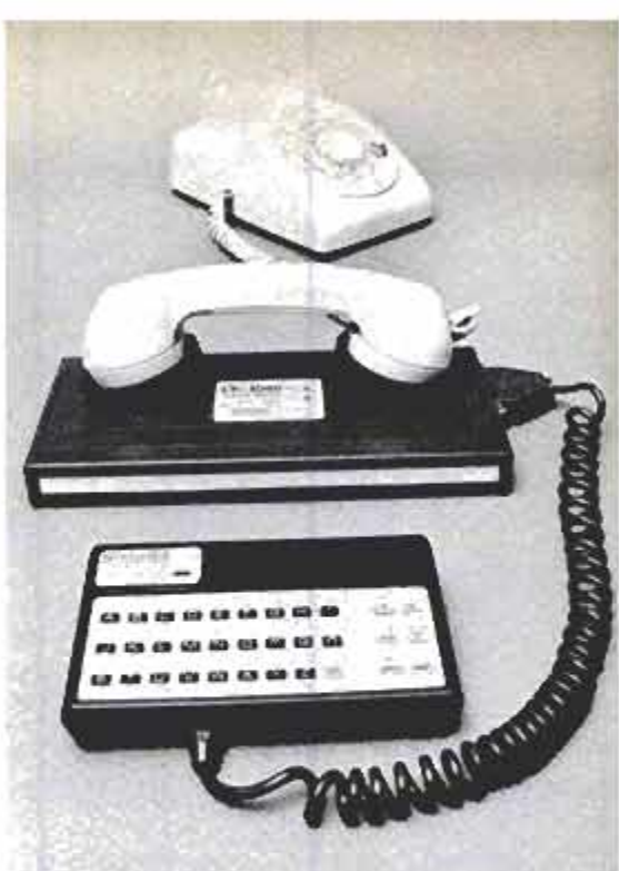
You can even "access" full-size computers with tiny, handheld units like this Nixdorf. However, it lacks multiline display and other functions, such as ability to make sense of lower-case letters.
