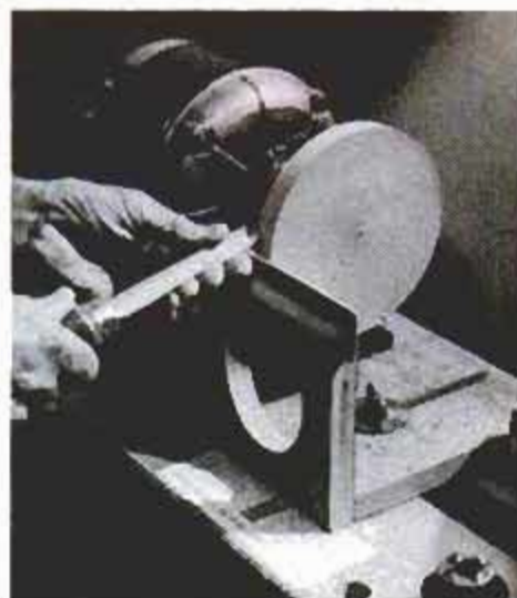
Using a pulley wheel as a mount, low-cost lathe can be used for faceplate turning.
