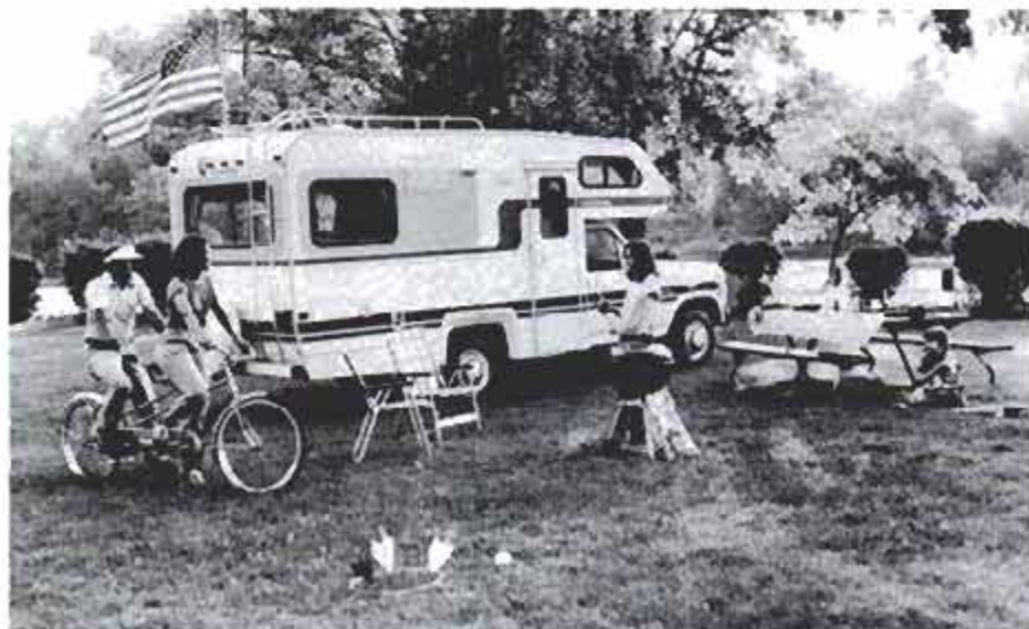
Laminated construction lightens body of the Coachmen Caper XL mini-motor home. Built on a Ford chassis, the 20-footer has six-cylinder power, rear dinette plan.
