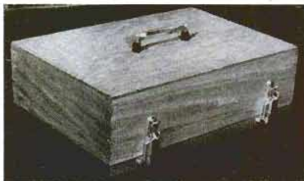
Finished box has luggage latches and drawer pull for a handle. The cover frame is red oak, and the top is \frac{1}{4} -in. plywood. Photograph shows a base of \frac{1}{4} -in. alder.
