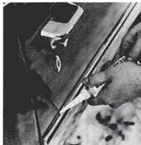
A thin bead of Dow Corning silicone rubber sealant helps "rustproof" auto trim. The bead seals out moisture, dirt and salt and protects the trim's fasteners.
