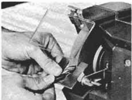
Sharpen worn twist drill bit while holding it in the toolrest groove for guidance.
