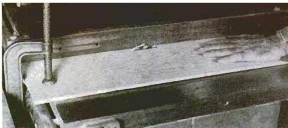
Clamp board securely to table, then elevate saw blade a bit beyond desired height.
