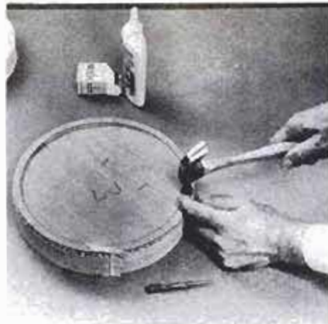
Glue and nail the platform first, then add fillers and finish with the retaining ring.
