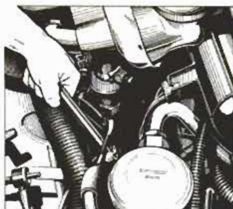
Sparkplugs on rear bank of V6 X-cars are a chore to remove. They're also hard to see.
