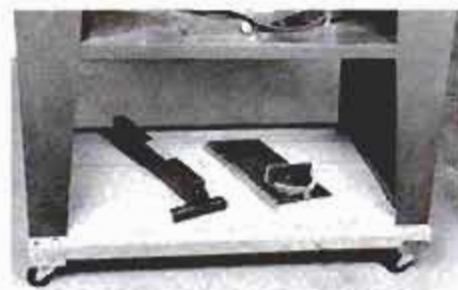
Shop-made saw dolly improves stability by widening base and also provides shelf.
