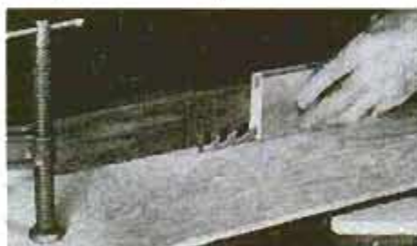
Now, stock fed into blade is supported on both sides of blade by accessory tool.
