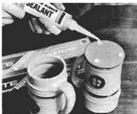
Silicone feet on mugs protect wood tabletops from scratches. Apply small dabs of sealant (left). Next, use three coins to support the mug over a piece of wax paper, but keep the coins out of the sealant (right). Allow 24 hours for curing, then peel wax paper.
