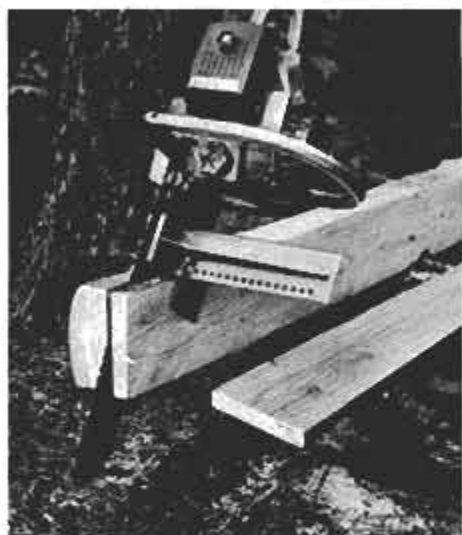
The adjustable guide bracket helps you to saw boards to the thickness you desire.
