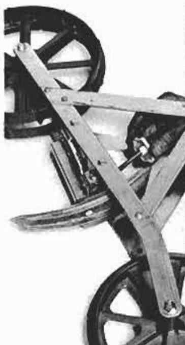
Unlike other cultivators, the working part of this one is located between the wheels (above, right). Set desired cutting depth by turning adjustment handle (left).
