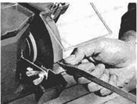
Square screwdriver tip after reshaping blade by holding on rest, touching wheel.
