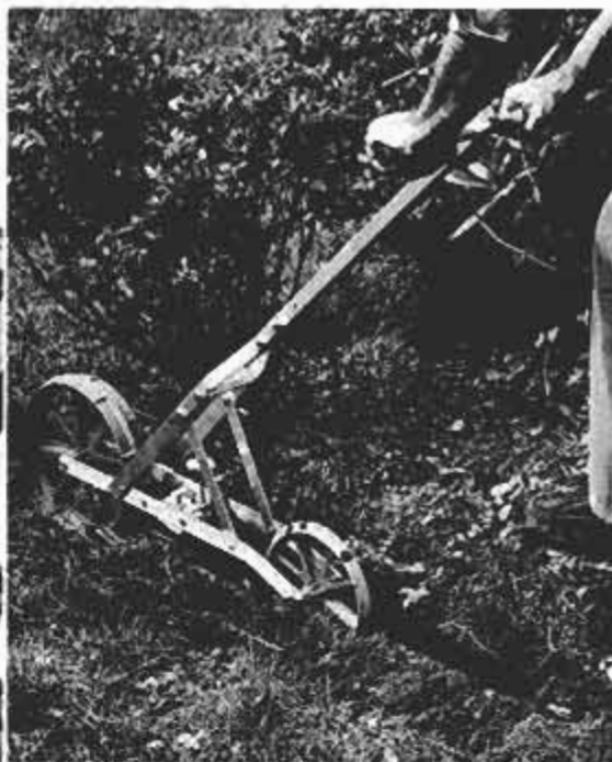
Unlike other cultivators, the working part of this one is located between the wheels (above, right). Set desired cutting depth by turning adjustment handle (left).
