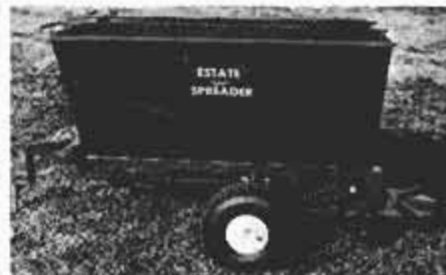
Mini Spreader has a 12-bushel capacity.
