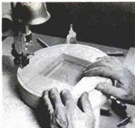
To cut circles from block, shift the pivot point after tangent cut is made to get blade to inside. Cut forms ring and skirt.
