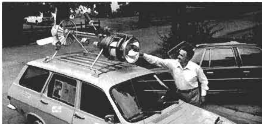
Tamosiunas recharges battery, using roof-mounted air turbine and propeller.
