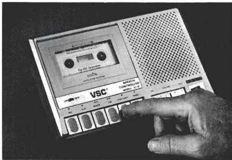
Prototype Variable Speech recorder speeds up tape without losing clarity.
