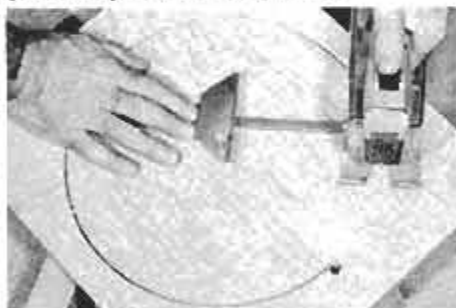
Stop the saw periodically when cutting circle so workpiece can be shifted on its support (a pair of 2x3s here). Saw blade should cut only the work, not the supports.
