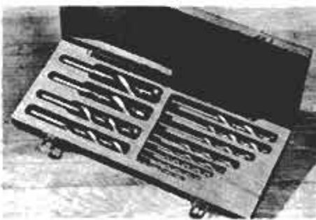
The 12 bits range from 1/8- to 1-in. dia.
