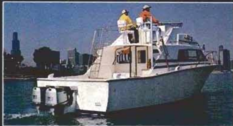
OMC Sea Drive prototype powers 33-foot Bertram. Waterproofed units are lighter than inboards, take less space, can go faster on less fuel.
