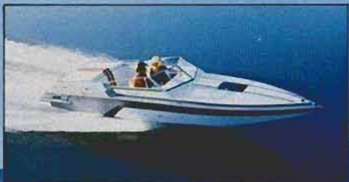
Hammond V-2150 Challenger MK II has clocked 60 mph with a 260-hp MerCruiser, and has an outboard version rated for 250 hp.
