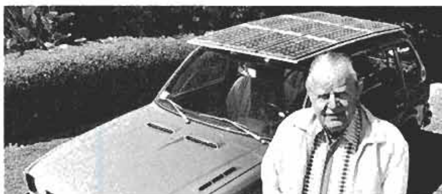
Panels on Moore's car contain 396 photovoltaic cells feeding six batteries.
