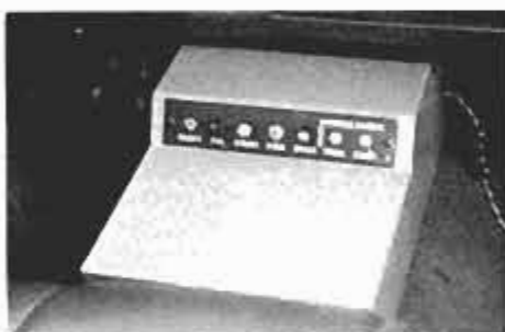
Control panel next to driver can activate the entire system or selected functions.
