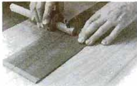
Cut strips with sharp cutting gauge. We chose 1 1/2-in. widths for the prototype, but this can be changed to suit pieces.
