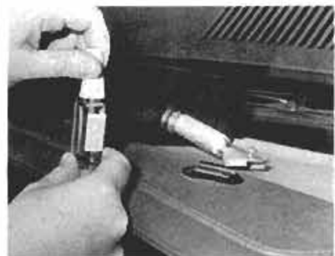
New adhesive kit enables you to attach rear-view mirror to windshield instantly.
