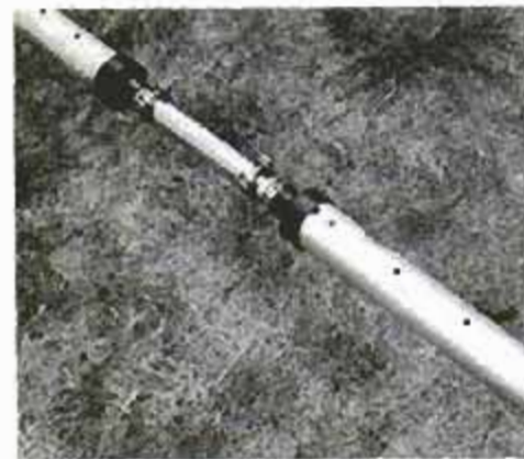
The traps contain drain holes so that rain will run out. Keep them pointed downward.
