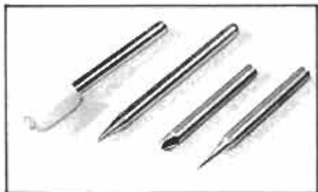
Basic set of styluses and cutters. Both ends of second stylus are used to trace.
