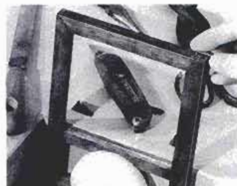
Pin hinges for door are reproduced from thin, polished brass. See text and drawing on facing page for installation details.
