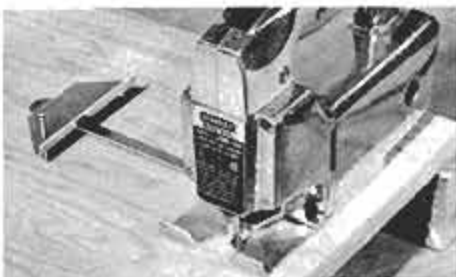
When blade is fully into work, with saw shoe flat on the work, cut toward one of the cutout lines (1) and then cut straight into the corner. With blade moving, back the saw up (2) and turn the corner (3). Step 4 simply repeats step 1 and so on.
