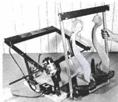
Typical setup for carving with the spindle accessory. Note the speed control here.
