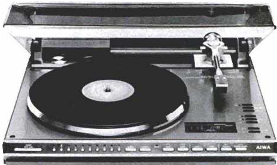
The most unusual feature of Aiwa LP-3000 is that the tone arm is powered by two separate motors—one drives the arm across the record and other lifts and cues it. Photodiodes are also in the Yamaha PX-2 table (below) and they continually adjust to correct angle.
