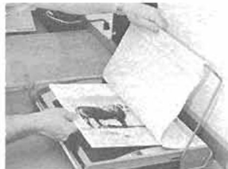
Sandwich of mounting board, tissue and print is held snugly to the dryer by canvas.
