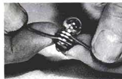
To form the lamp socket, wind copper wire around threads of a lamp base as shown.
