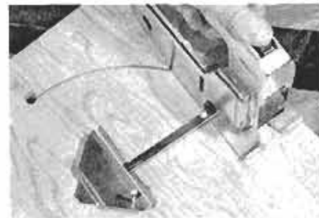
For best results when cutting a circle, use a rough blade with a heavy set (the tooth set assures blade-turning clearance). Push the saw with a slow feed rate and, if your saw has variable speed, set it to the fastest cutting speed to obtain maximum strokes per inch as you make the cut.
