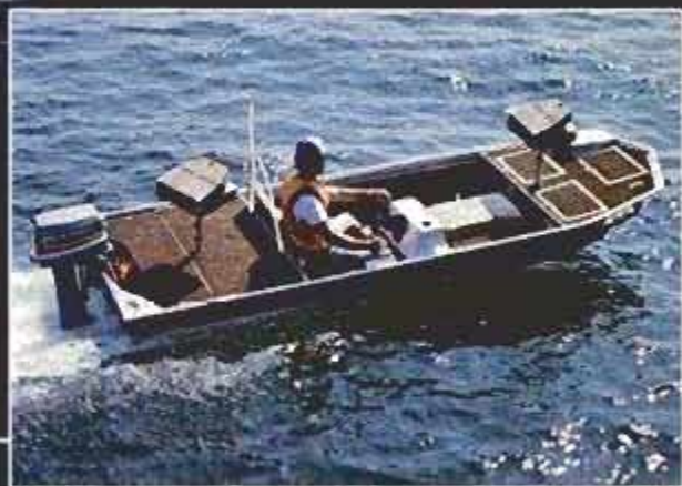
An aluminum bass boat with a new full-length V-hull, Rover III V-20, by Fisher Marine, West Point, Miss., is 20 feet long, takes a 40-hp outboard, weighs 420 pounds.
