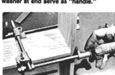
Unlike pipe clamp, which must be longer than the workpiece, Maxi-Clamps can be attached as shown to close a butt joint.
