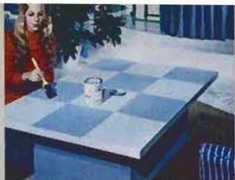
Cube tabletop is painted with conventional latex paint, then covered with 1/4-in. glass.
