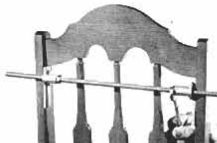
A simple "spreader" arrangement such as this pops a chair's glue joints apart safely when doing restoration work.
