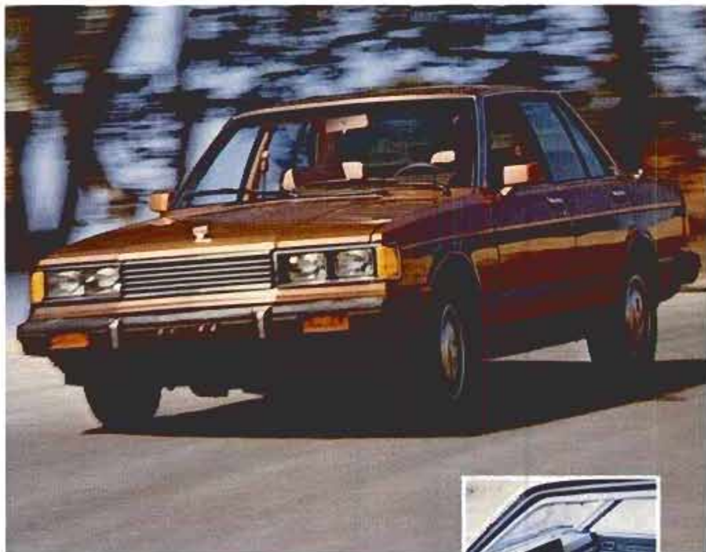
The Datsun 810 sedan uses a modified version of the 280ZX sports car's suspension which furnishes good handling.
