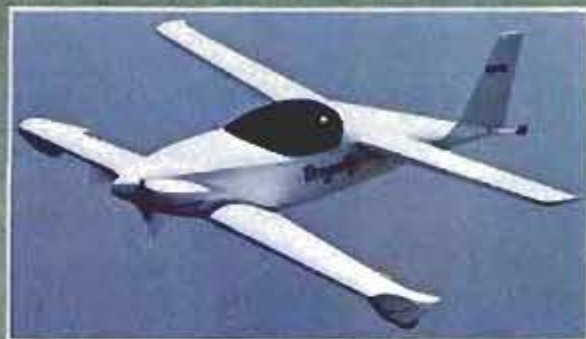
It looks like a Quickie, but isn't. The all-new, futuristic Dragonfly features a tandem-wing design, two-place, side-by-side seating, dual side-stick controls.
