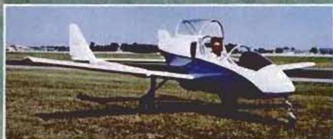
Twin tail booms give BD-5 fuselage a dashing new look in this 300-mph Acapella. It has folding wings, retractable tri-gear.
