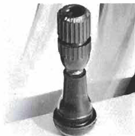
Air-pressure monitor tells you at a glance when the tire air pressure is getting low.
