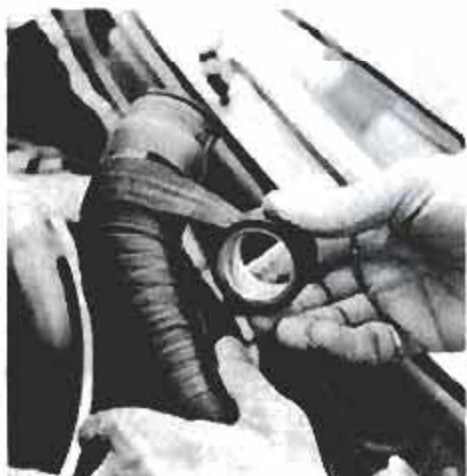
Self-vulcanizing tape bonds to itself for repairing hoses and other pipes or tubes.
