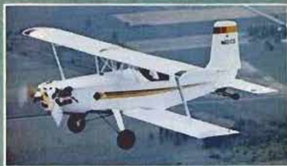
A little single-seater in classic biplane style, Der Cricket is aimed at economical flying. Taking VW engines from 45 to 60 hp, it cruises at 95 to 110 mph.
