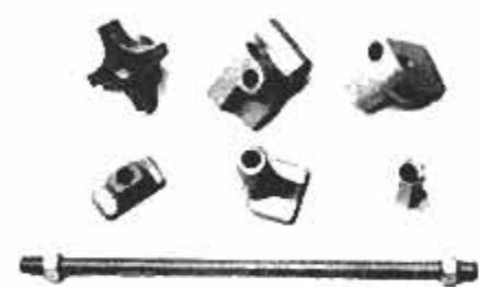
Close-up of major parts: knob, three- and two-hole junction blocks, pressure foot, clamping jaw, coupler, rod, nuts.
