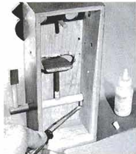
Retainer pegs are pushed into holes with a screwdriver blade. Use glue sparingly.
