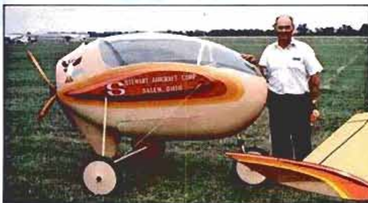
Reminiscent of early "flying bathtubs," Gypsy sports stubby fuselage, full aircraft-type controls, is foot-launchable.
