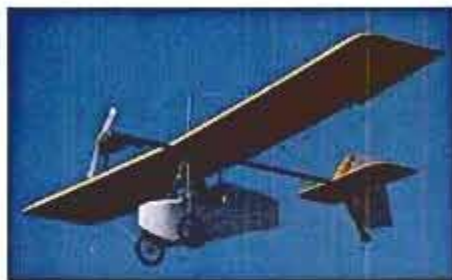
Reminiscent of early "flying bathtubs," Gypsy sports stubby fuselage, full aircraft-type controls, is foot-launchable.
