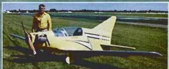
Reincarnation of the BD-5: In Scorchy, it gets a new name and a nose-mounted engine in place of original pusher-prop drive.
