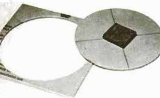
To avoid scratches when cutting acrylic, glue wood pad to protective paper to take the trammel point, then peel off the pad.
