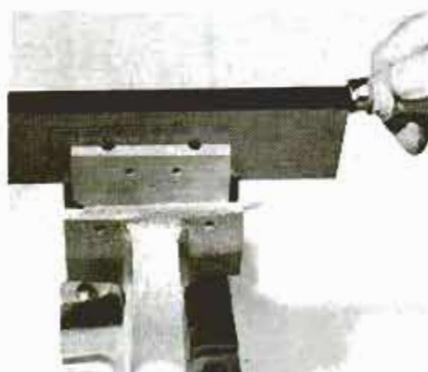
Edge silt is sawed in the trammel block, so block can be clamped securely on the router-base rails. Backsaw is best for this.
