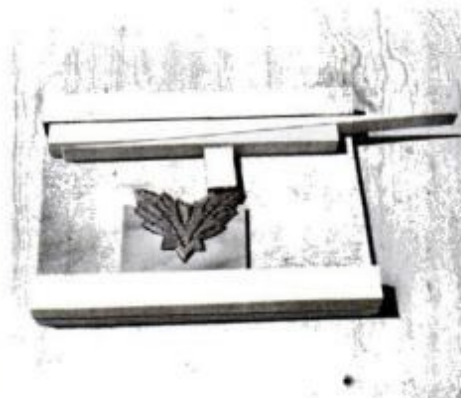
18 Odd jobs often need a shop-made clamp. Get clamping action with this jig by pushing in long wedge with your hand.
