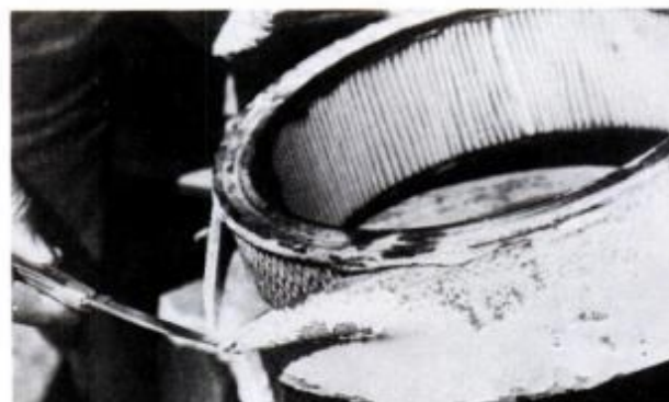
Dodge van kept going, even though two-stage filter's outer element was completely caked with volcanic ash.
