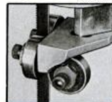
Blade guide arm adjusts for size of work; gives maximum rigidity to blade for squareness and accuracy.
