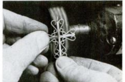
12 Polish the cross on the buffing wheel without rounding away its square edges.
