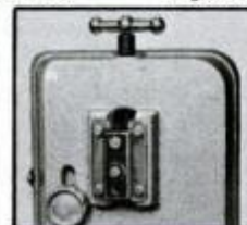
Idler bandwheel mounted on gibbs for alignment adjustment, accuracy and proper blade travel.
