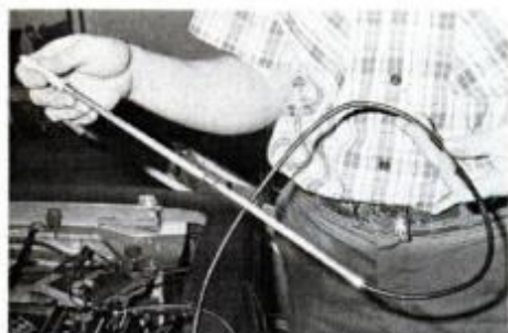
Stiff probe holder will give you remote timing-mark readings for timing checks.
