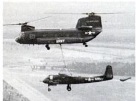
One form of sky hook: Chinook chopper airlifts a Mohawk—a portent of the future?
