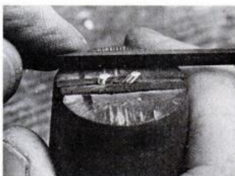
3 Bend and cut a second half-heart; then file the ends of both half-hearts flat.
