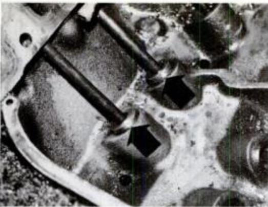
Replacement lifters (arrow) of CVCS system allow intake valves to open .200 inch.
