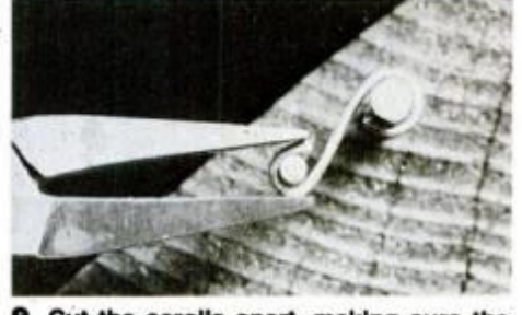
9 Cut the scrolls apart, making sure the cuts are aligned. Place scrolls individually on nails to make final closing bend with needle-nose pliers. If needed, tap flat before positioning scroll next to the cross.
