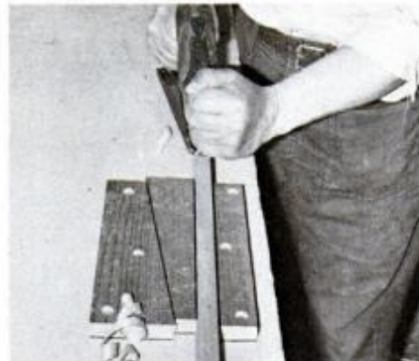
17 Make this clamp for holding wood while planing. Provide opposite bevels on angled edges to keep wedges flat on the bench.
