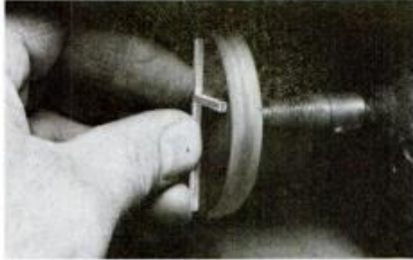
7 Polish the cross on a wheel with tripoli then jeweler's rouge, taking care not to round the edges. Substitute polisher is a leather-covered wood scrap.
