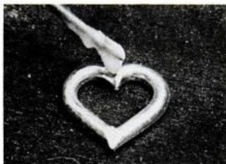
4 Position both halves on a soldering block; then apply flux to the two joints.
