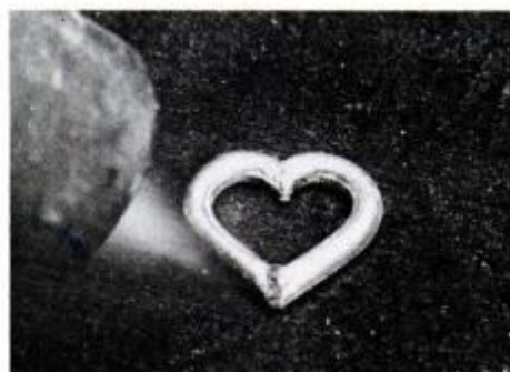
5 Heat the silver enough to both dry out the flux and melt it to a glasslike state.
