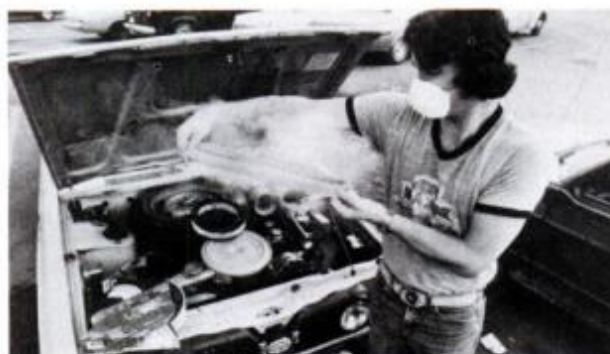
Snap-cleaning the outer foam element on a two-stage Maxi-Air filter in Yakima, Wash., near Mt. St. Helens.
