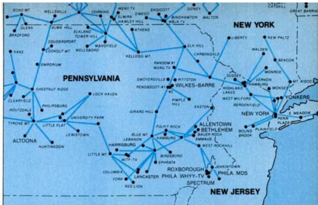
Section of the East Coast microwave relay network shows signal routing from tower to tower. Before satellites, networks such as this were the only way to relay signals.
