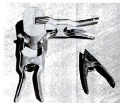
10 Commercial spring clamps come in many styles. Model at left has pivoting jaws for irregular shapes, opens 3 1/2 in. wide.
