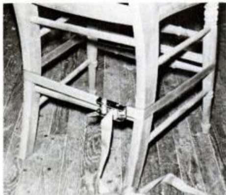
19 Use screwdriver or wrench to tighten rugged Pony web clamp. Self-locking cam holds tight, yet permits quick release.
