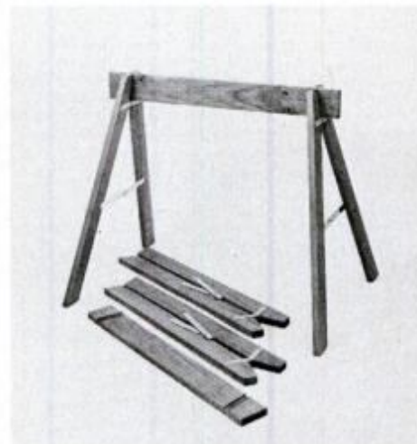
Sawhorse disassembles for easy storage.
