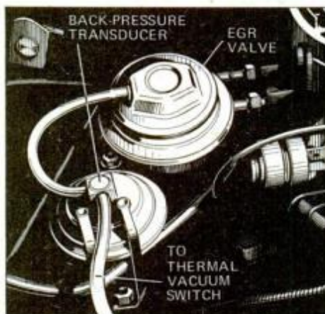
Some GM cars have Back Pressure Transducer (BPT) separate from EGR valve. To test BPT disconnect hose, check vacuum.
