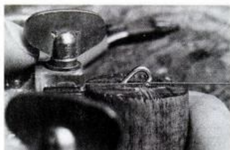
2 Secure the excess wire in a wooden jeweler's hand vise, or a vise that has leather-padded jaws. Cut off the half-heart shape with a jeweler's saw.
