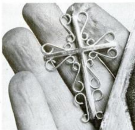
13 Do a final polishing with a stick faced on both sides with leather. Use one side for tripoli, the other for jeweler's rouge. Wash the cross in soapy water.
