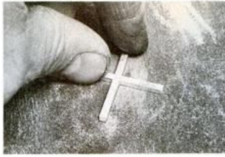
5 To smooth cross, rub it in a circular motion on 400-grit paper on a flat surface.
