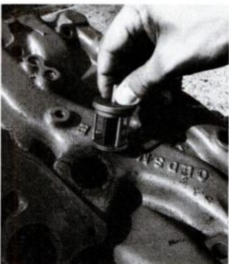
Barrel-shaped valve fits into a machined hole on top of intake-manifold plenum.
