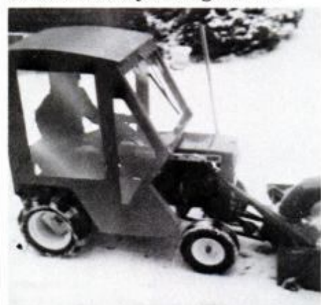
Warm and cozy in PM's homebuilt tractor cab. Note added exhaust riser on engine.
