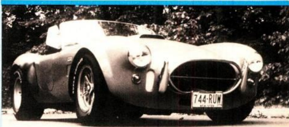
The Shelby Cobra was a British roadster stuffed with a 427-cu.-in., 500-hp V8 engine. For $7000, it offered drivers performance remarkably similar to a full-blown race car.
