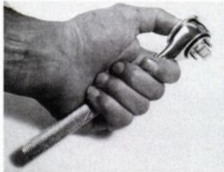
A positive release ejects wrench sockets.
