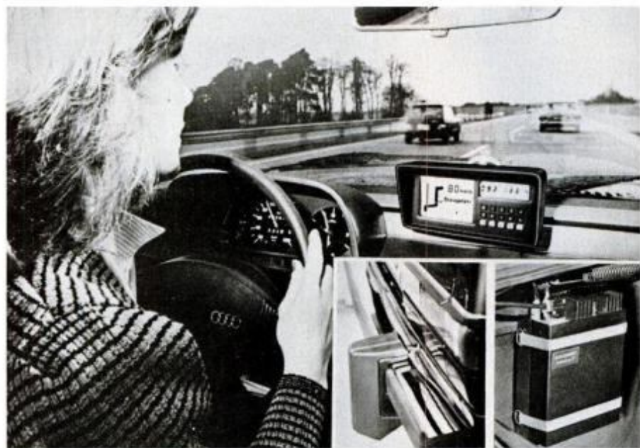
On-board Ali components include transceiver and antenna in bumper (inset photos, left). Dashboard displays indicate upcoming turns.
