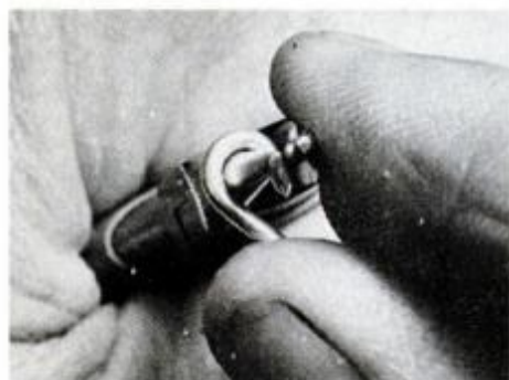
1 With roundnose pliers, bend a \frac{1}{8} -in. half-heart in .060-in.-dia. silver wire.
