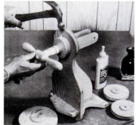
Fork is held on trike by tapping a 3/8-in. dowel through collar and into the fork.
