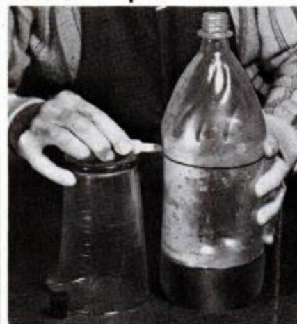
A felt-tip pen makes a heavy, highly visible cut line around soft-drink bottle.
