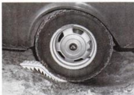
Plastic ramps provide a safe, sure grip for tires that are in snow, mud or ice.
