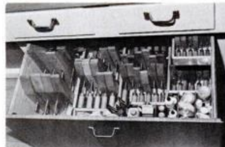
Deep drawer in same bench contains assortment of hand screws, glue, web clamps. Because of weight, drawer is on slides.
