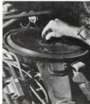
Unwind the thumb screw at the top center of the air cleaner. Lift the air cleaner to expose the top of the carburetor.
