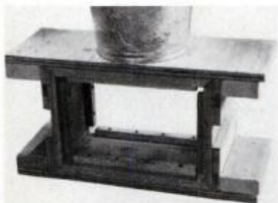
Clamping jig (above) must be sized to project, unlike adjustable jig.
