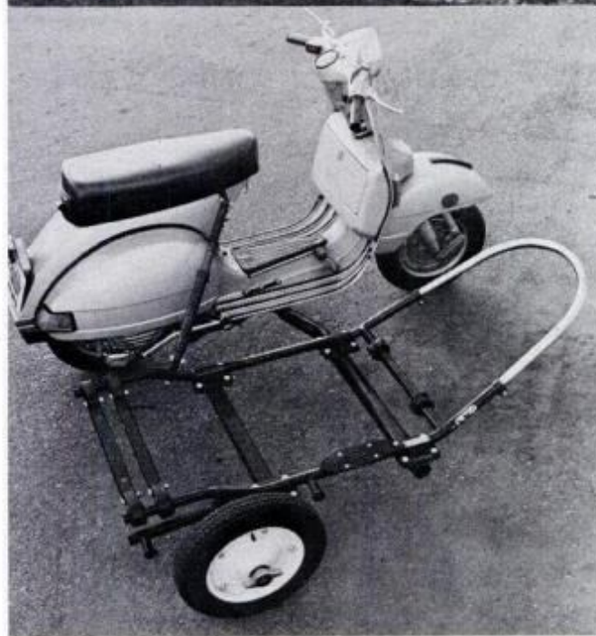
Off-road racing with a sidecar is not for the faint-hearted (above). It takes muscle and strong kidneys. Subframe for a Vespa sidecar is bolted, not welded, to the scooter (left). The sidecar is then bolted to the frame. Note the steel loop in front. It's there for crash protection. The heart of the flexi sidecar mechanism is the spring-loaded slider tube (right). It allows the sidecar to lean with the cycle.
