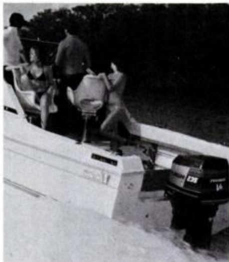
For cruisers, a big bolt-on like Evinrude's 235 gives planing speeds even with throttle set at the economy-cruise position.
