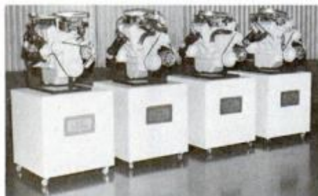
The new family of GM automobile engines includes a Three, a Four, a Five and a Six.
