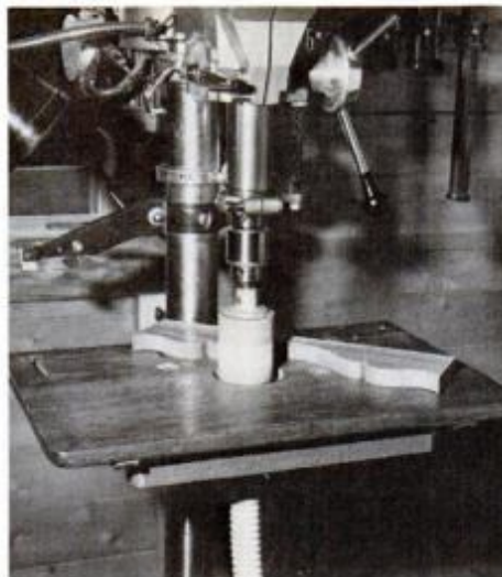
A great shop jig—a sanding board for your drill-press table. This one makes it a snap to use the drum sander. Plywood is installed on table with four thumbscrews.
