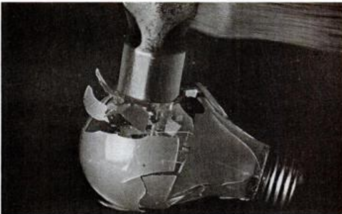
No sense taking this photo until you've got a dead bulb. By varying trigger gap, different stages of breakage can be caught.
