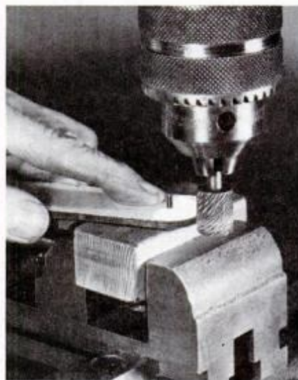
Milling table allows work to be fed into the rotary file at \frac{1}{16} in. per pass.
