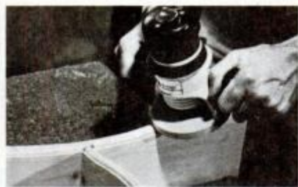
Convex router base lets you shape curved edge, is guided by piloted bit.
