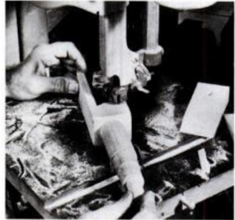
After turning the fork on the lathe, slot for the wheel is cut out on the bandsaw.
