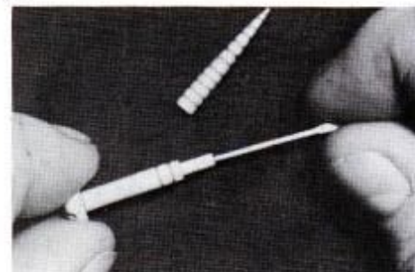
The surprise is this full-size needle—inside the wooden screw. Yep! Opfer turned the wooden needle on the lathe, too.
