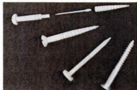
His lathe runs so true owner can make miniature turnings like these. Screw at far right is a commercial 1½-in. screw.
