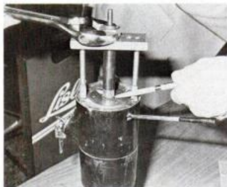
This lock-plate compressor allows fast and easy access to turn-signal switches.
