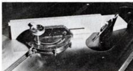
Author particularly liked miter gauge addition. It eliminates cutting through backup board. Drawing shows how it's made.
