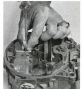
With a screwdriver, remove the single screw that holds down the "Y" shaped stamping on the "butterfly" valve.
