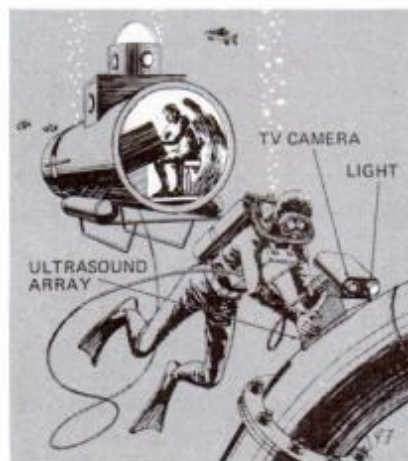
Diver probes pipe for hidden flaws.
