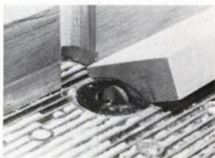
Use core box bit to rough-shape molding. Adjust the bit and fence for each pass.
