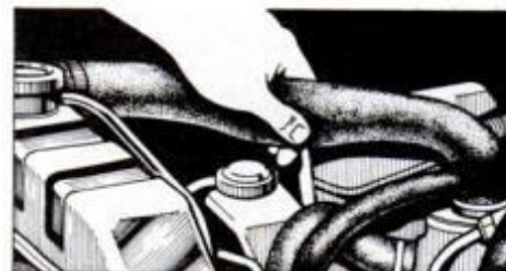
Inspect hoses for fatigue by squeezing them with your hand. They should be firm and free of cracks when squeezed.
