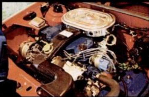
The Escort/Lynx 1.3-liter engine (1.6-liter optional) is transversely mounted and features an overhead cam, hemispherical cylinder head and hydraulic lash adjusters. The dash layout (right) is excellent and readable. All vital controls are handy.
