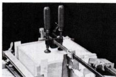
Here, clamp held by bar clamp gripping box is used to hold the drawer bottom in.
