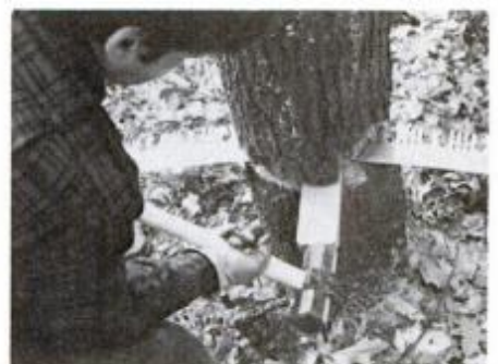
If saw binds while cutting, drive wedges as needed to free blade and continue sawing. Plastic wedges won't damage saw.
