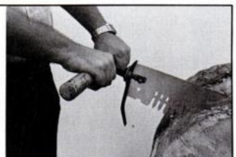
Another desirable feature is adjustable handles that let the grip rotate 90°. This is handy for avoiding obstacles.
