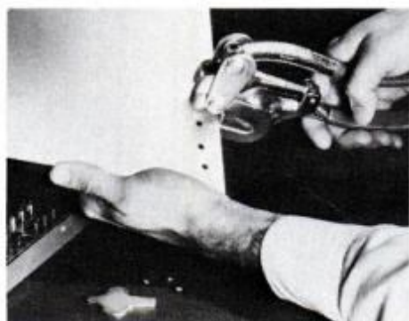
Punch is well balanced and can be used with one hand by most do-it-yourselfers.
