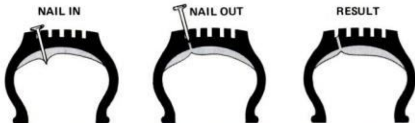
Self-sealing tires are coated with a rubber-based material which instantly seals a hole after a puncture. These tires will soon eliminate the need for you to carry a spare.
