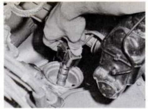
Removing the automatic transaxle's governor is a one-minute job. You can reach it easily from the top of the transaxle.
