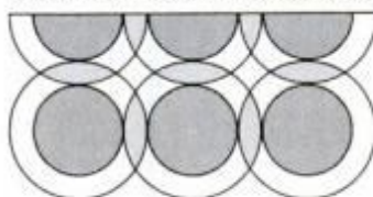
IMPROPER SPACING (7-1/2"-RADIUS SPRAY SPACED 12')
