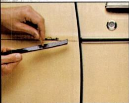
1. Spread activator on loose trim, bumper moldings, emblems, etc.
