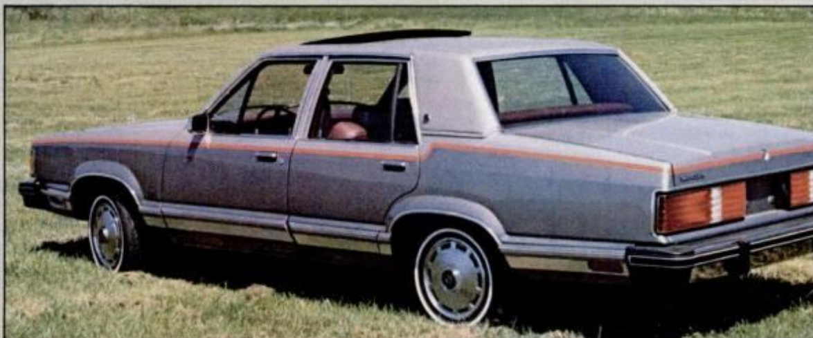
The standard engine for this year's restyled Granada is the 2.3-liter Four. Overall, the lines have been rounded to improve the aerodynamics and reduce fuel consumption.
