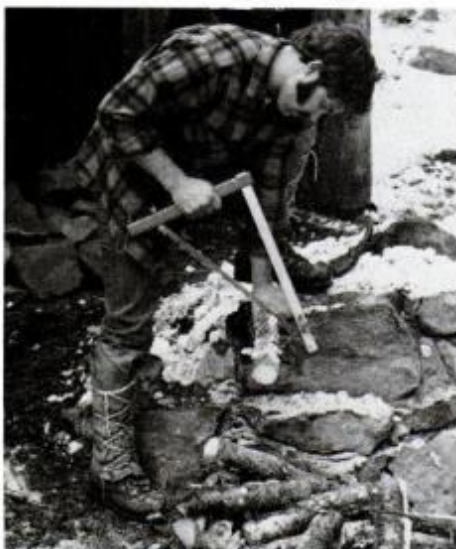
Small-size crosscut saws (above), which are handy for the cutting of small-diameter logs, are equipped with replaceable blades. The folding types are especially handy for the use of backpackers (below).
