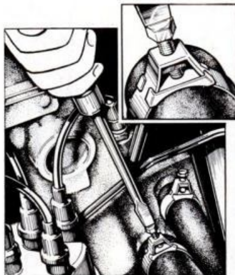
Old-style tower clamps should be checked more frequently than the new worm clamps. Position them 1/4 inch from end of hose.
