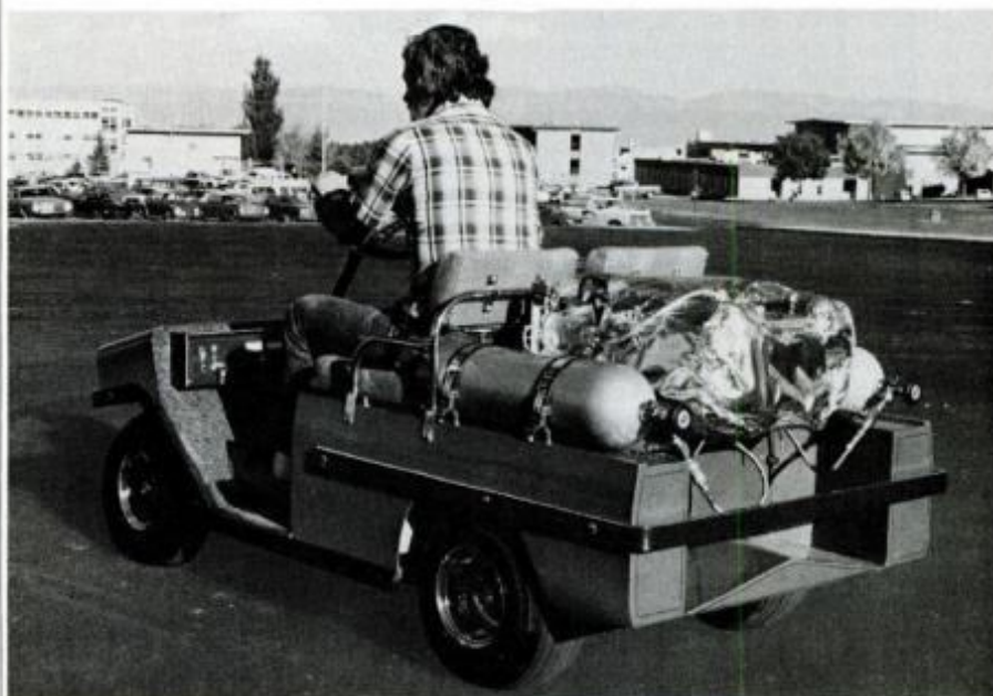
Fuel cell on a golf cart test-bed has shown great promise for use in cars.
