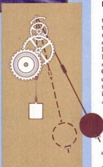
The drive mechanism relied on a "grasshopper" armature to translate pendulum action to gears.
