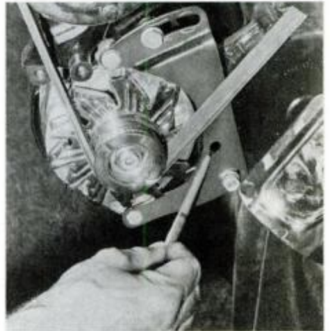
To set alternator-belt tension, a small hole in the bracket for a screwdriver is used for making the final adjustment.
