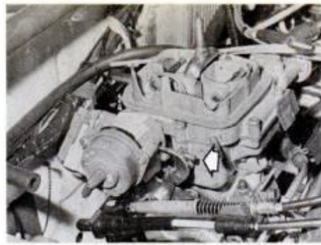
Idle-speed screw is not sealed in the new Four and is readily accessible from the passenger's side of the engine.
