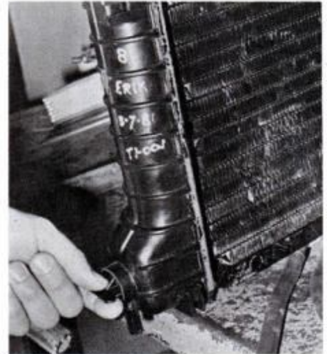
The Escort's radiator tank is made of plastic, and so is the drain cock. It can never rust and "freeze" closed.
