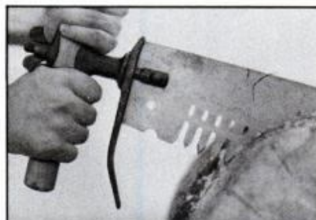
Old-style saw handles, often seen at auctions and flea markets, have rugged finger guards to prevent jammed fingers.
