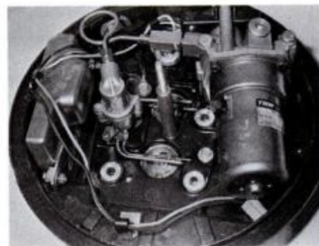
The fuel-injection system is under the air-cleaner cover. Spray bars over the throttle plates inject fuel into the manifold.
