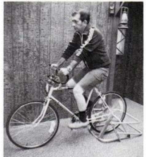
Bike exercise stand uses aluminum chair frame partially folded with back on floor.
