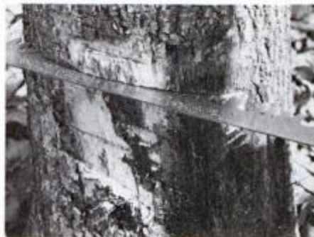
Prior to making either cut, chip away bark with a hatchet. Dirt and bark itself, might otherwise dull saw quickly.
