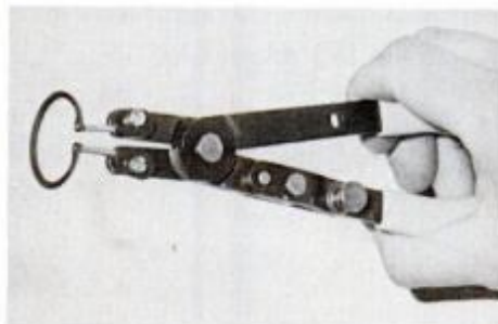
In its first position, the snap-ring pliers can disengage internal-type snap rings.
