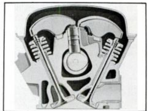
In designing its new overhead-cam Four, Ford discovered the hemi-head (right) would yield most power, fuel economy.
