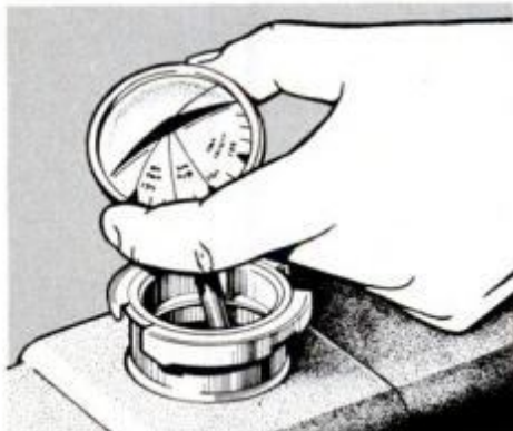
A quick check of thermostat operation can be done with a thermometer. Check to see at what temperature water begins to flow.
