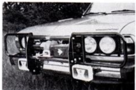
Compacts and full-size pickups and 4wds can be fitted with combination brush and grille guard with winch kits by Warn.
