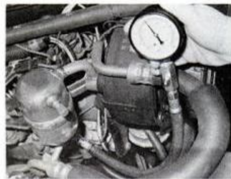
Thexton gauge has adapters for all makes of diesel engines; reads up to 1000 p.s.i.
