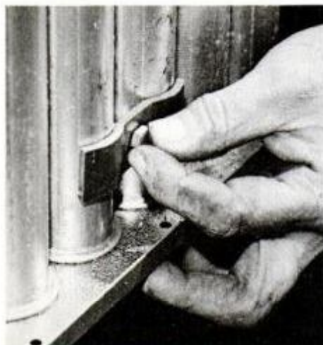
Pivot installation is quick and easy; a single nut holds each one securely in place.
