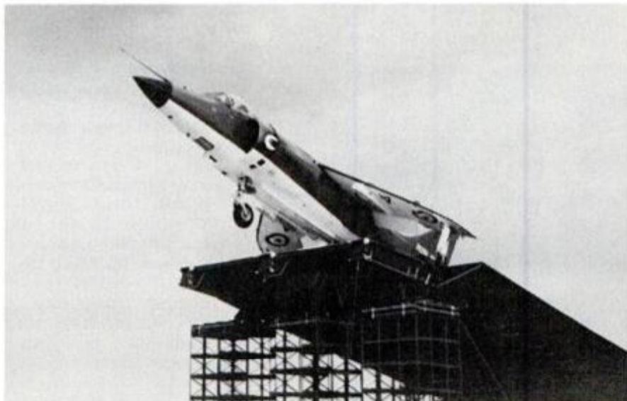
Ski-jump gets plane up where it flies, momentarily, without lift—like a rock.
