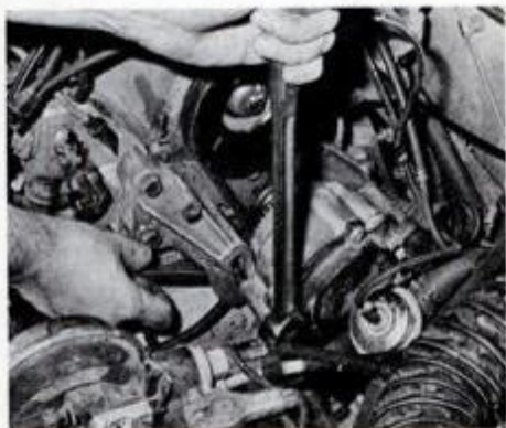
To take up the slack on the fan belt, the air-pump retaining bolts must be loosened; they are short but are easy to reach.
