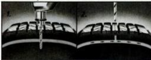
When the tread is punctured, Uniroyal's special sealant automatically surrounds the puncturing object. As the object is withdrawn, the sealant fills the gap, preventing the air's escape.
