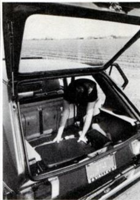
Huge luggage area holds 15 cu. ft. with the rear seat up, 22.6 cu. ft. with it down.
