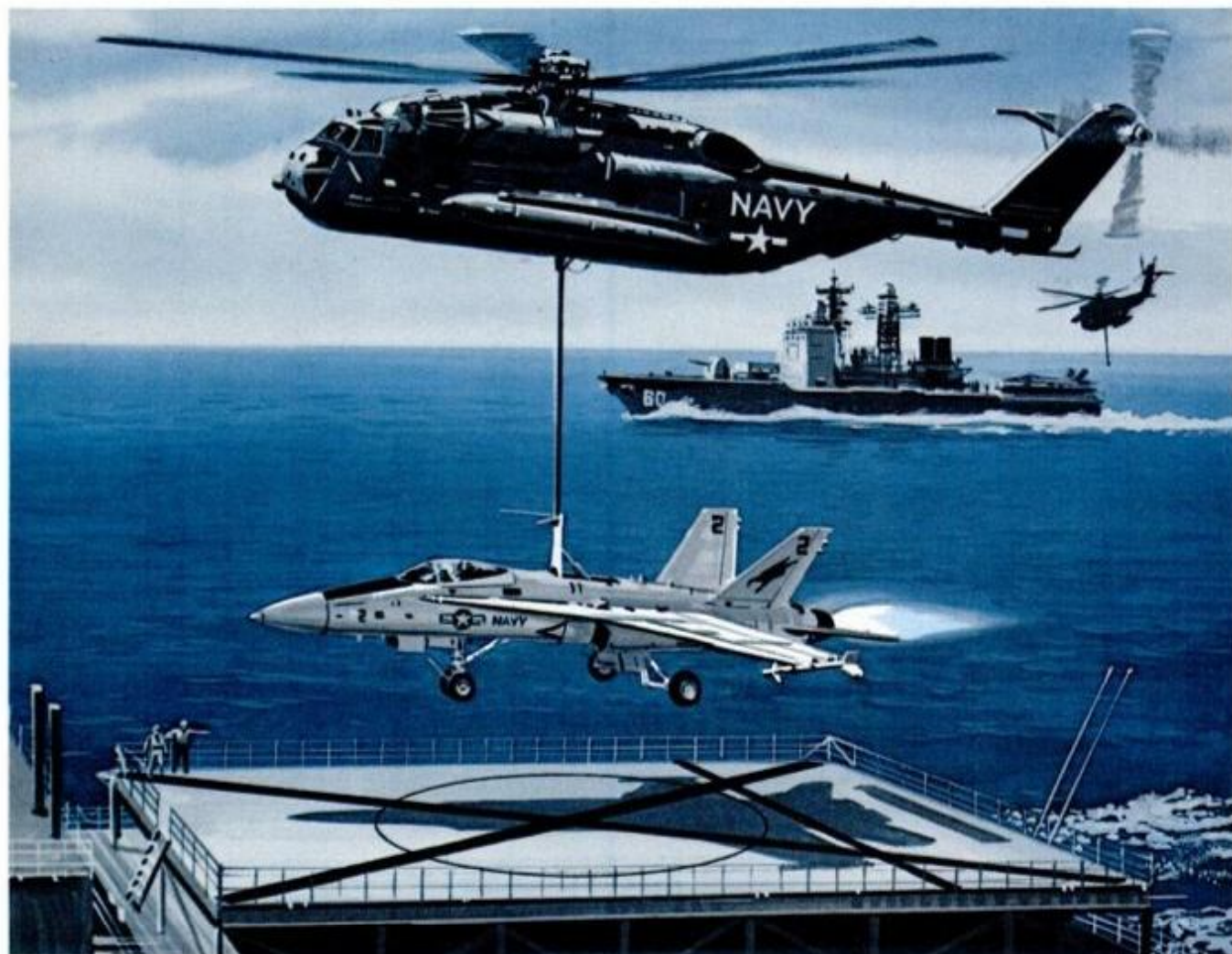
"Flying catapult" concept would use helicopter's lift as the vertical component for a VTOL-capable supersonic
