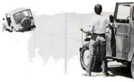
With a winch, the off-roader can pull his rig or a friend out of trouble. This Warn winch mounts a handy remote-control switch.
