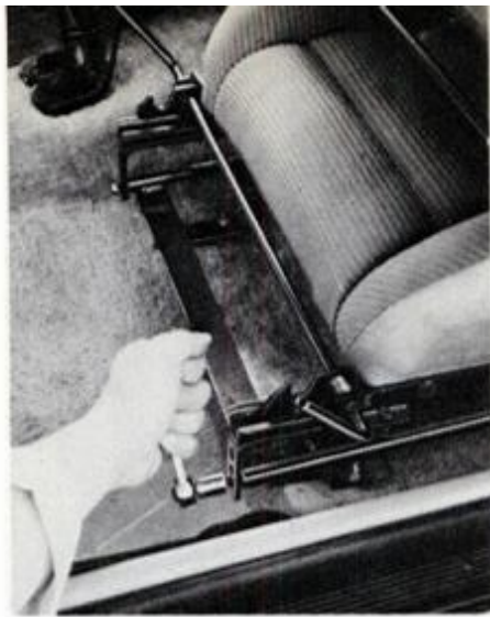
Subframe for replacement seats uses same studs as stock seats (right). New seat is then bolted to the subframe (left). It takes less than an hour to do the whole job.
