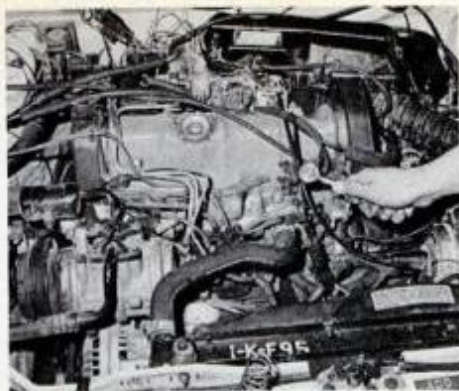
The sparkplugs face toward the front of the car, making their removal very easy. They are not obstructed by any plumbing.
