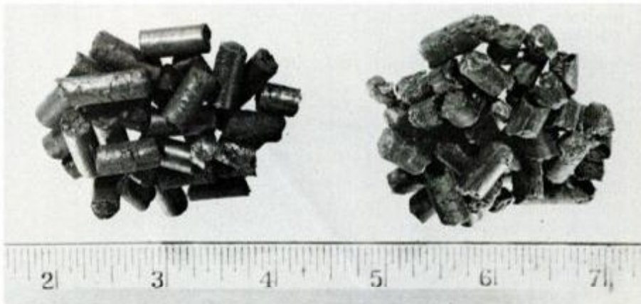
Coalex (black) pellets at left, and Woodex (brown) pellets at right, are used by industrial plants, hospitals, schools and facilities that have commercial-size boilers.
