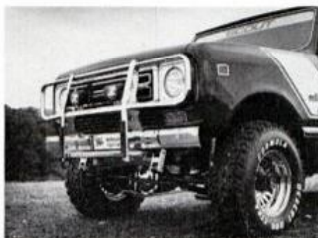
Front-end improvements with lights, grille guard and truss rod under the transfer case to prevent axle bend dress up Scout.
