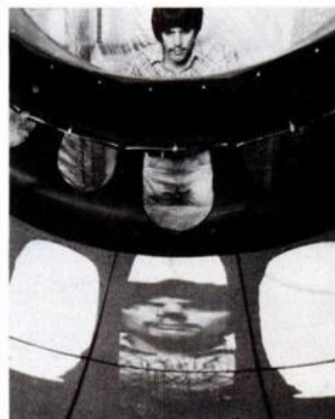
Mirrors in one PEP device, used in quark studies, deflect light from fast-moving particles onto phototube for measurement.
