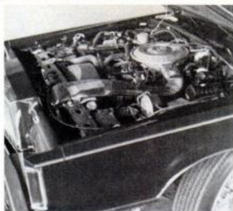
Most owners chose 5.8-liter V8 engine. They found it yielded 18.1 mpg on highway.
