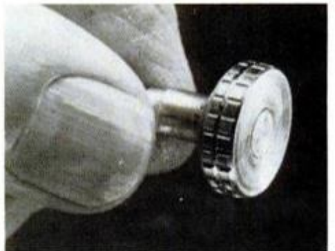
Longitudinal grooves on the rim of thumbscrew were spaced with indexer at left.
