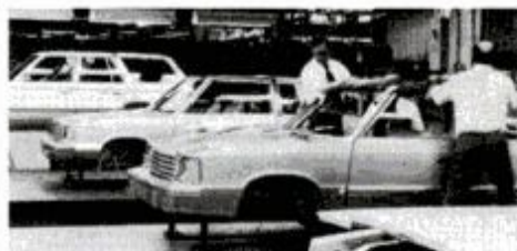
The 1981 Plymouth Reliant is being tested for the final-tooling and assembly fits.
