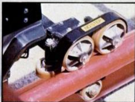
Small rollers keep coaster on the tracks.
