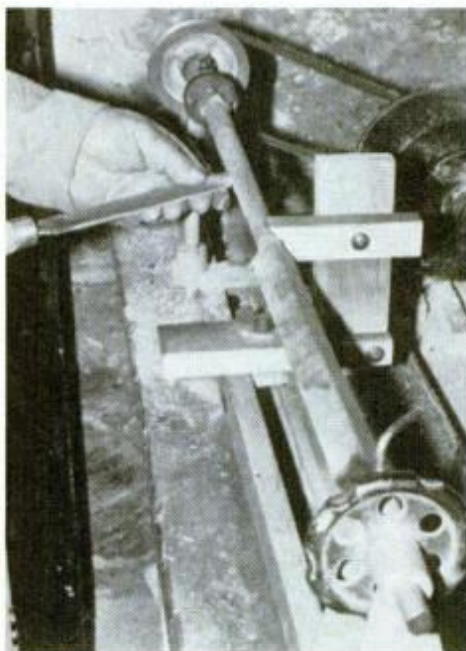
Simple-to-make lathe accessory supports a long spindle having a V-shaped notch.
