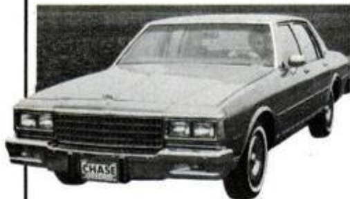
Caprice hood slopes more for '80. This, plus other modifications, adds 3 mpg.
