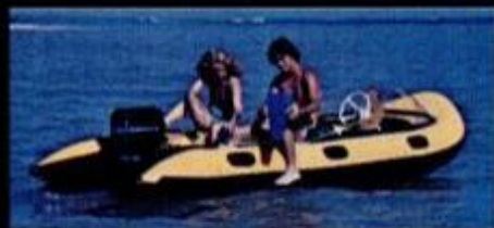
New blow-up boats are being fitted with forward steering for motors 20 hp and up.
