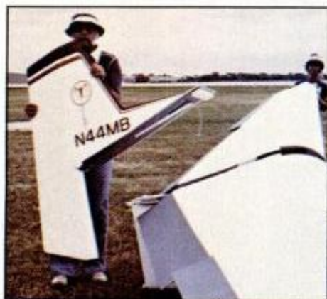
Minibat is a flying-wing sailplane powered by a 3-hp "sustainer" chain-saw motor buried in its fuselage (the prop measures 19 in., rotates in slot between fuselage and rudder), following a bungee-cord launch. The kit offers premolded parts.
