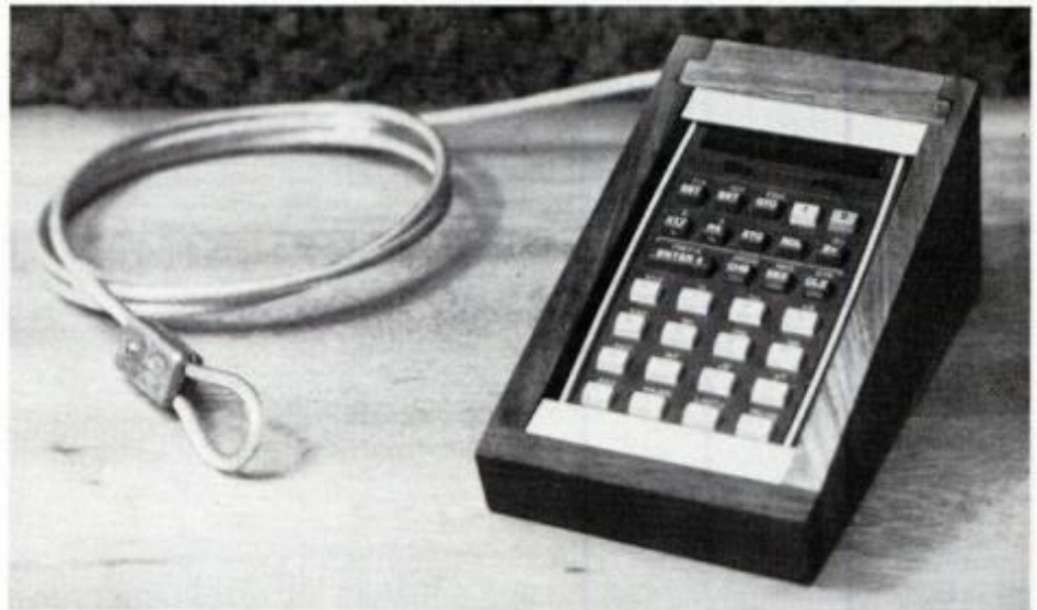
Stand makes calculator easier to read. Its cable can lock to the desk to stop theft.
