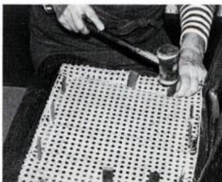
Stretch new cane seat into position using opposing wedges. Then use wedge and mallet to tap cane into remaining groove.
