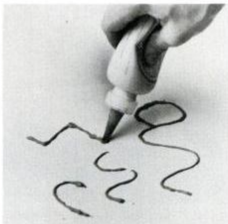
Practice on scrap material until you can apply the liquid lead in a uniform line.
