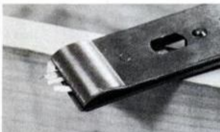
To assemble, place cap on the flat side of the iron with its screw in the slot.
