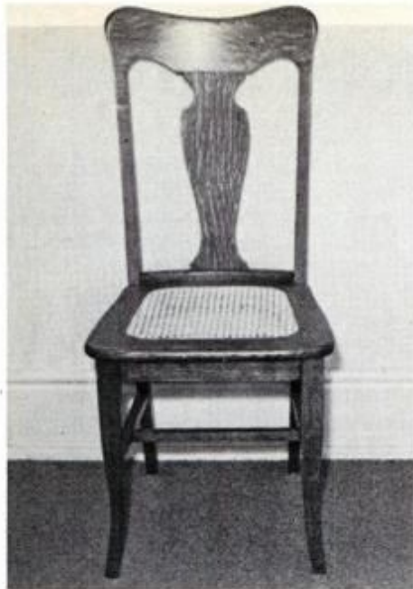
New seat in this chair is made of low-cost, machine-woven cane. Text tells how to replace split cane seats quickly and easily.
