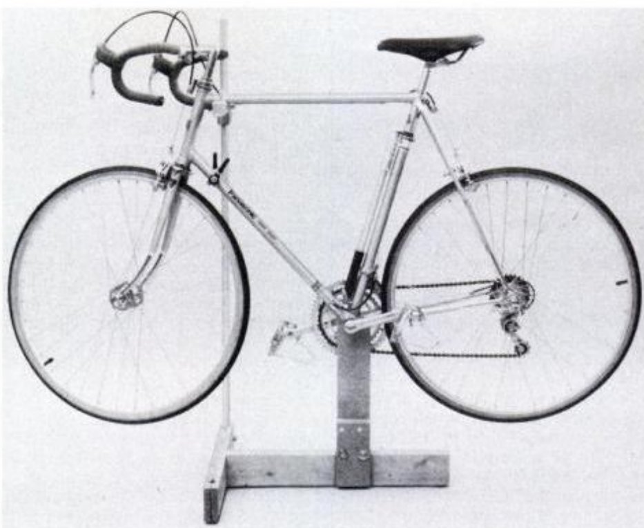
The top support bracket of the bike stand holds the 10-speed touring bike by its top bar. The stand's top support bracket can hold a woman's bike by its handlebar stem.
