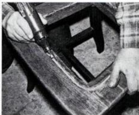
A high-speed rotary tool is also effective when you're cleaning the old caning material and the glue out of the spline groove.
