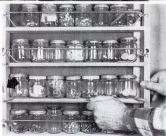
Storing all your miscellaneous hardware in one place will save you time that might otherwise be spent searching. Baby-food-size jars on shelves built into doors are held in place with wire retainers and turnbuttons (arrow).
