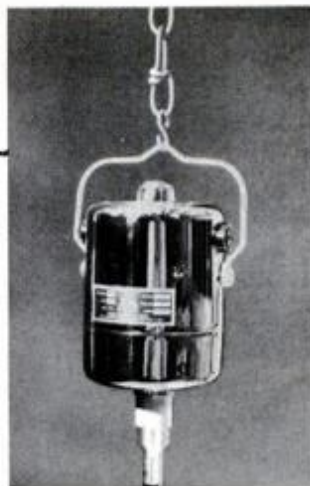
Grinder motor can be suspended from ceiling to eliminate back pressure on the handpiece while carving.
