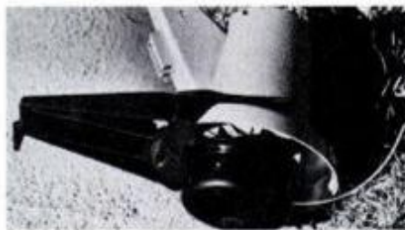
Dome cap at base of cutting head houses the automatic line-feeding mechanism.
