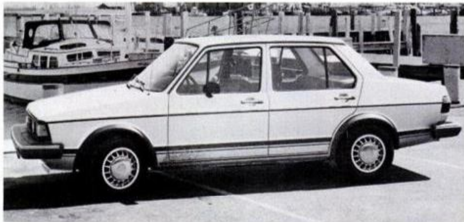
Racy version of the Jetta (there's a no-frills "stripper" model, too) features blacked-out window molding, urethane fender flares and a fully integrated front spoiler.
