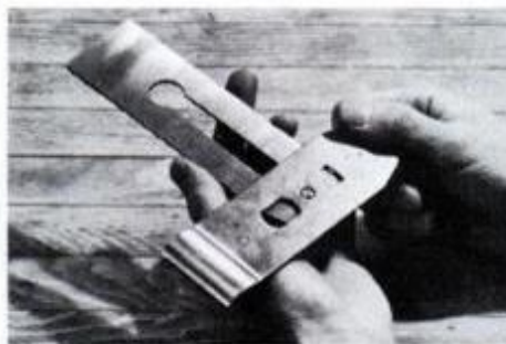
Draw the iron back (above); then align it with plane iron as shown at right.
