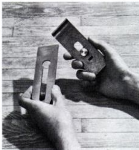
Plane iron (left) and its cap must be put together properly for efficient cutting.
