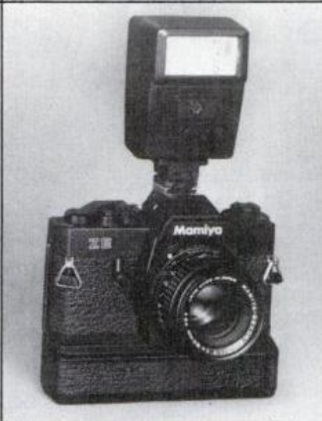
wind. Fujica AX-5 (lower left) features dual-mode automation, two-head flash option. Mamiya ZE (lower right) couples lens to auto system electrically.
