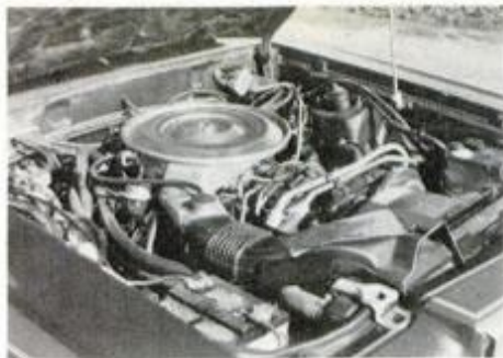
Larger 302 V8 delivers slightly better mpg than the 255, thanks to o.d. automatic.
