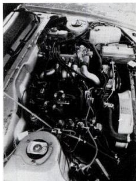
The two-liter gasoline engine produces 96 hp; the 2.3-liter diesel yields 71 hp.
