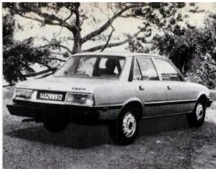
Large glass area and slim pillars give good visibility. Rear suspension is independent, with coil springs, rear trailing arms.
