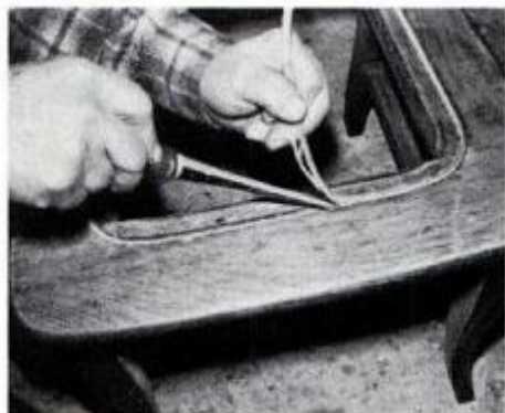
Remove the old spline and cane with a narrow wood chisel and clean the groove, being careful not to chip the seat boards.
