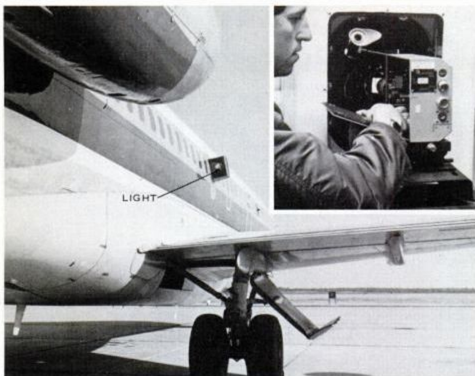
Extra landing light on FAA plane illuminates rear engine during flights in rain. Camera (above, right) inside the plane photographs the buildup of water near the jet intake.
