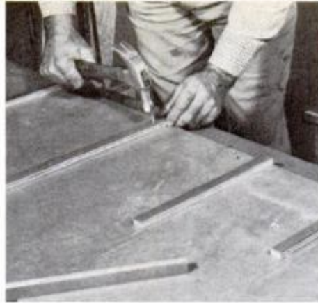
Glued-and-nailed cleats help to support the shelves and simplify assembly. Use galvanized nails for good holding power.
