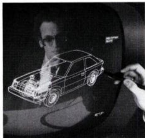
Computer-graphics model of Ford's Escort/Lynx is used to test its body rigidity.
