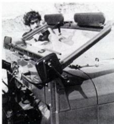
For serious off-roading, the windshield is able to fold down flat right over the hood.
