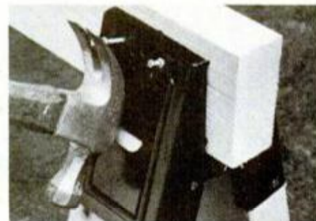
Assemble temporary structures with double-head (scaffold) nails. Used on this sawhorse cross member, they are easily pulled to permit folding and flat storage.
