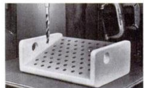
Photo above shows the setup for boring perpendicular crayon holes in the holder's angled surface. The drill bit is the brad point type—perfect for this purpose.
