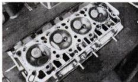
Valves are clean and show little wear. Black deposit on combustion chamber is merely soot. Note wipe mark on No. 2 chamber.
