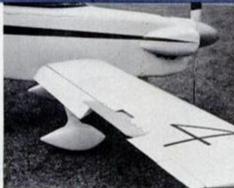
Ailerons are tiny—only 24 inches long—but are mass-balanced, highly effective. Numeral 4 on wing is plane's race number.
