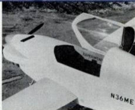
Side-hinged canopy opens out of way for easy entry. Slot in nose cowl is exhaust port for novel forced-air cooling system.
