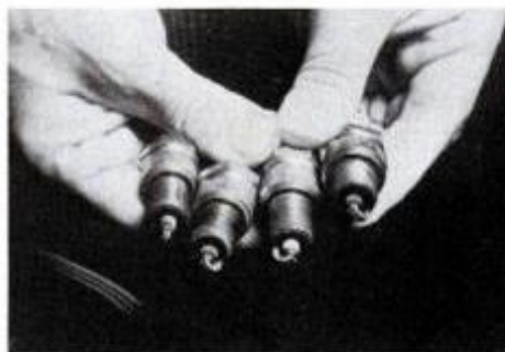
Changed every 15,000 miles on gasohol, the sparkplugs are free of carbon deposits.
