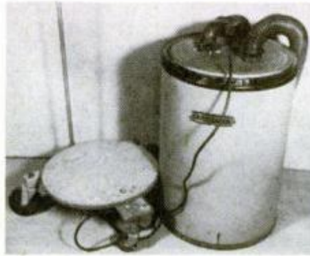
Use the three-wheel dolly for shop vacuums up to 15-gal. models. Use the four-wheel version for the larger units.
