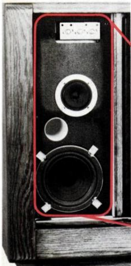
Large, well-placed speakers and improved audio amplifiers characterize new sound-conscious TV, such as Sylvania's Super Sound series models.
