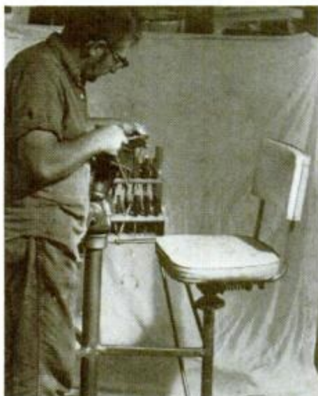
Filing stand combines universally adjustable table for vise, a handy tool station and a seat that rotates for desired comfort and mobility, all combined into a single, useful unit.
