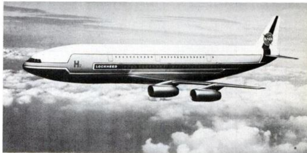
Four-engine subsonic hydrogen plane could carry 400 passengers seated on two decks.
