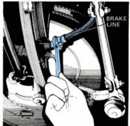
Replace brake hoses that are soft, weak, bulging, collapsed or otherwise damaged.
