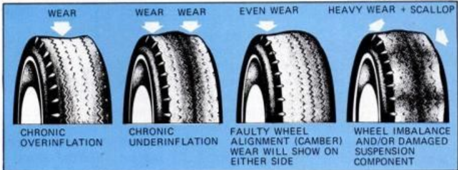
Tread wear can indicate suspension problems. Faulty wheel alignment will show up as a biased tread pattern. An out-of-balance tire will show as scallops or cupping.
