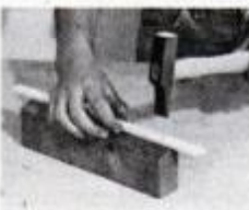
Hammer's square face makes it easy to drive brads and nails—even in a corner. Other end starts tacks (left).
