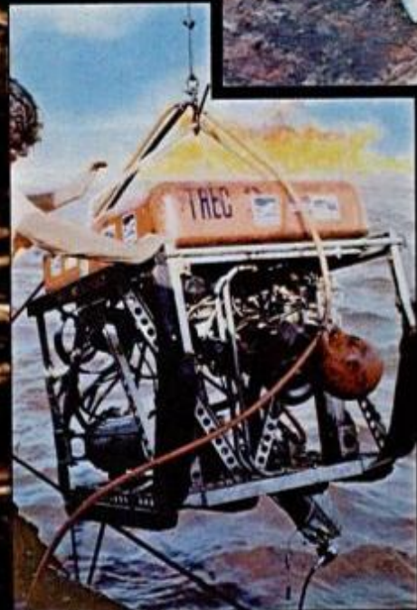
Blunt bow of flattop work barge, Able Turtle , nosed into edge of the flames (top). Divers attempting to locate leak (above) required hosing down as deck temperatures rose to 145° F. The remotely piloted underwater vehicle (left) finally found the source of oil plume, then got caught in its upward vortex. The turbulent ride to the surface banged up electronic components.
