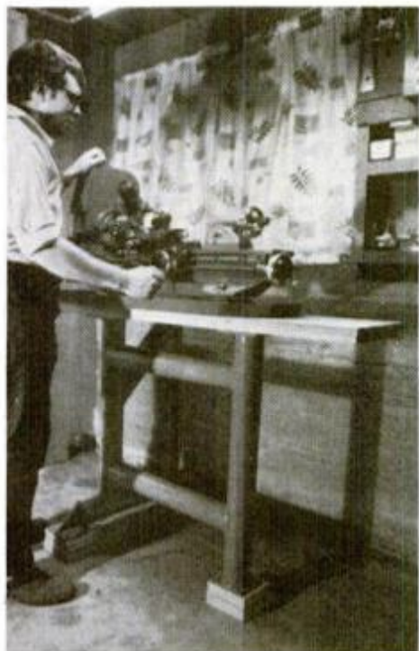
Lathe stand is raised to preferred work height (50 in. to center) with wood blocks and leveled with 1½-in., sheet-lead shims.
