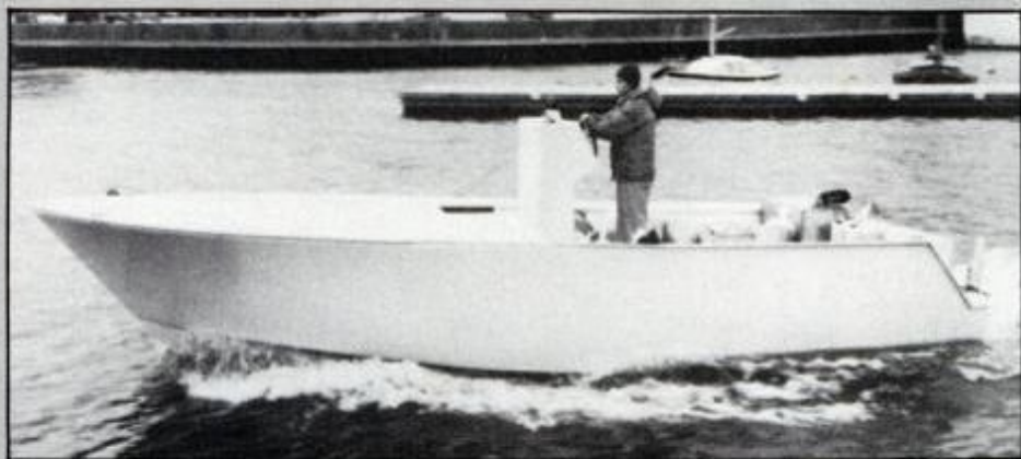
Testing a development model of Swedish Albin 7.5-meter hull with Wynne Marine "Propeller Pocket" and "Double Deadrise" deep vee, author runs ballasted hull in trials.
