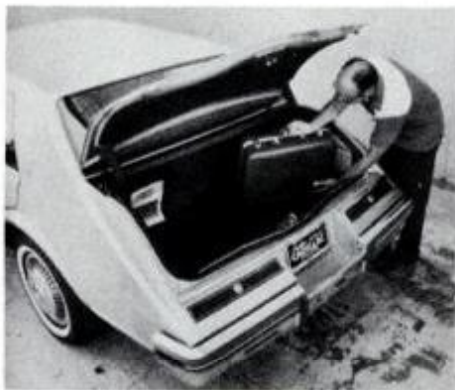
Without a differential, trunk is deeper, accepts large suitcases upright or on side.
