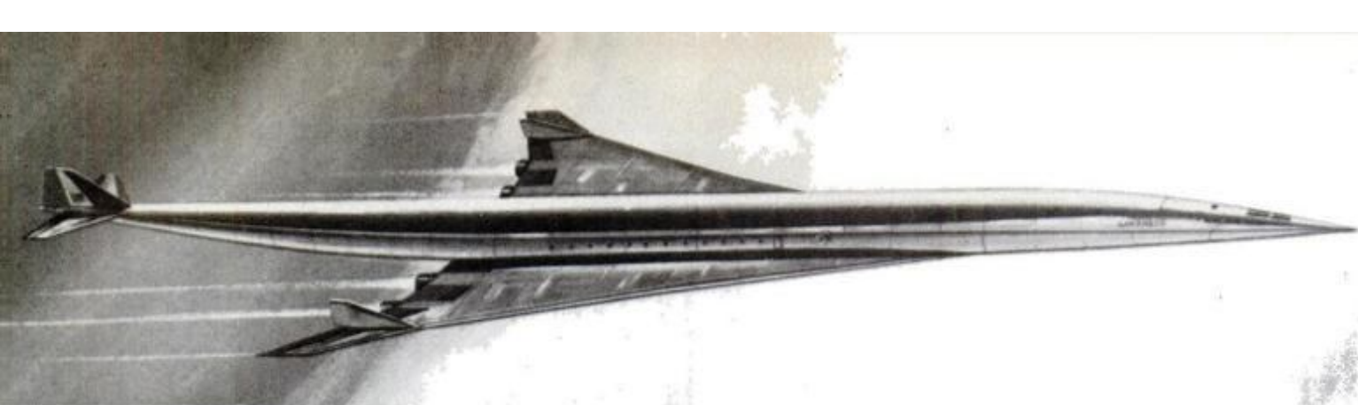
Theoretically, hydrogen-powered passenger plane could carry 234 at cruising speeds around 2000 mph. Range: 4200 miles.
