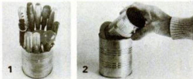
The modular tool and supply organizers (1) that make up this caddy are cleverly made from coffee- and soup-size cans. First glue a hardboard disc to the smaller can's bottom (2) to keep it centered
