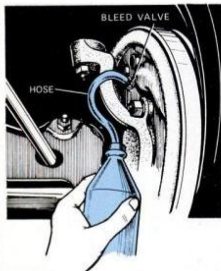
On drum brakes, bleed valves are located on the back of each wheel. On disc brakes they're found on top of caliper.
