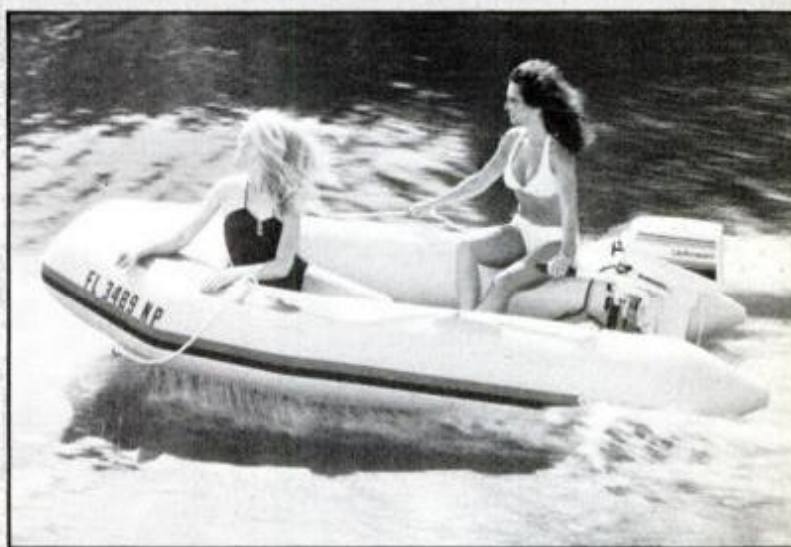
Even the push from a 4.5-hp Johnson is enough to plane a Boston Whaler inflatable. More muscle could provide ski speeds.
