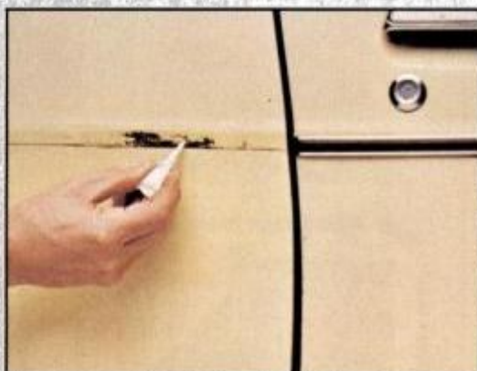
2. Apply adhesive to other surface. No measuring, no mixing, no waste or mess. Cure begins only after parts are put together.
