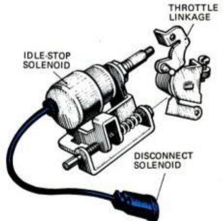
Disconnect the wire lead of idle-stop solenoid before testing engine vacuum.
