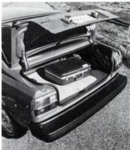
Sedan's trunk is 9.3 cu. ft. With seats folded, Liftback gets 34-cu.-ft. capacity.
