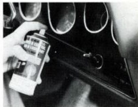
Aerosol spray eliminates radio crackle.
