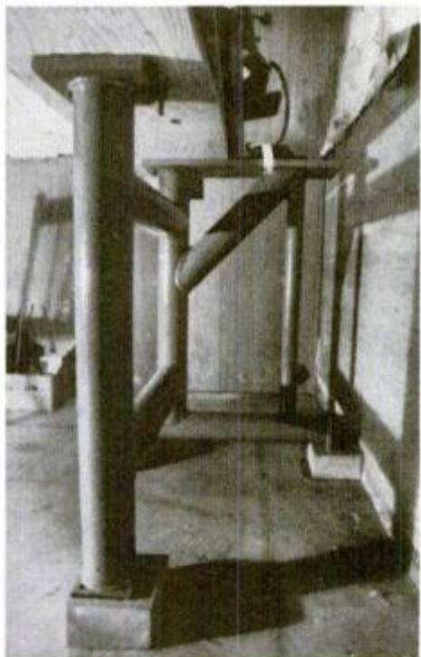
Lathe stand is raised to preferred work height (50 in. to center) with wood blocks and leveled with 1½-in., sheet-lead shims.
