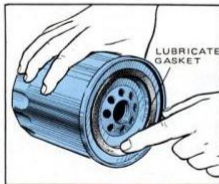
Apply oil to the gasket of a new filter to secure a tight fit with the engine.
