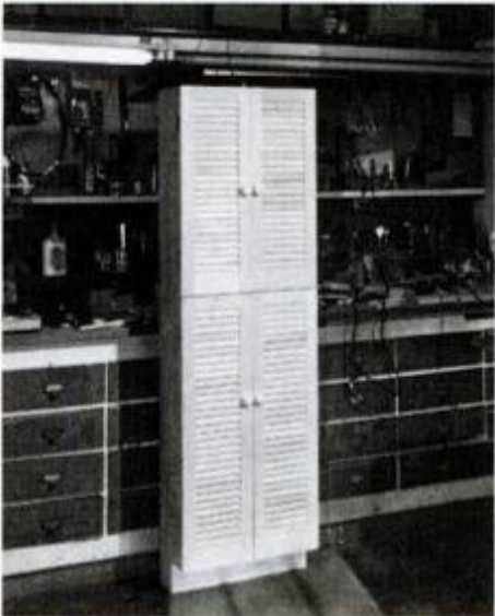
Temporarily assemble the complete unit in shop with the box set up plumb and level. When the fit proves satisfactory, remove hardware and doors to paint the center.
