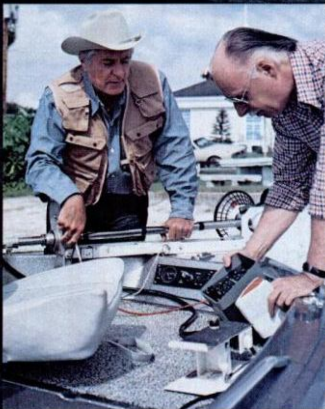
New fishing-boat refinement, an extra instrument panel in bow lets angler there tilt rear engine, check battery strength.
