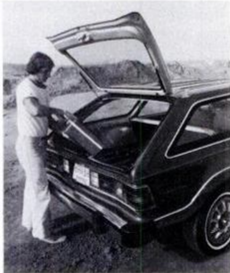
Wagon's hatch tends to drip when opened in rain; liftover sill is higher than most.
