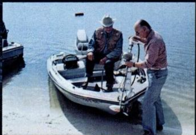
Electric trolling motor should swing down easily, stow securely while underway with stern engine. Prop weed guard is a plus.
