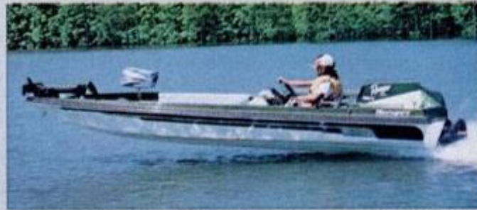
Like outboards, sterndrive inboards place weight aft for best planing angle. Forest Wood's Ranger 1980-V uses a MerCruiser.
