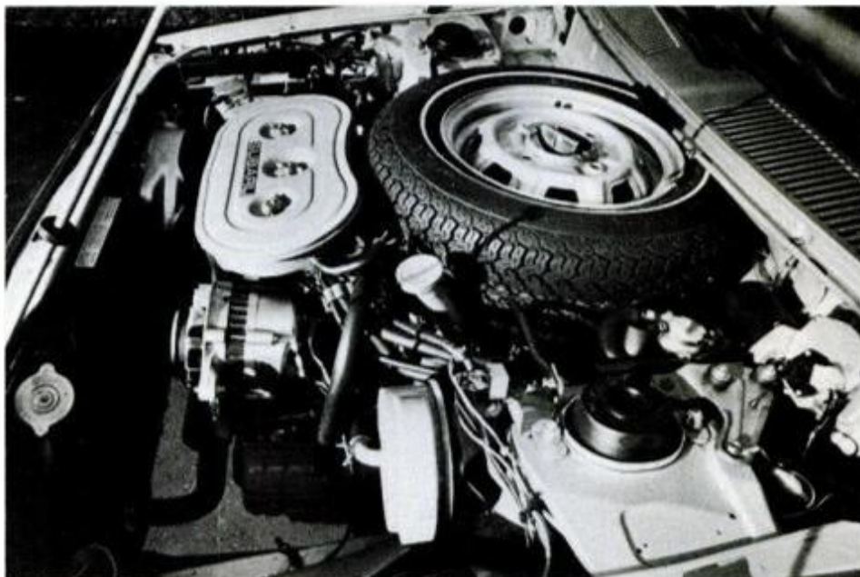
Aluminum-alloy, 1.6-liter engine produces 67 hp at 5200 rpm. Flat, four-cylinder configuration runs smoother than in-line, provides room in engine compartment for spare.
