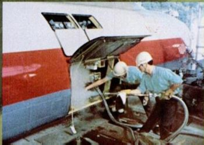
JNR technicians pump liquid helium in prototype's four chambers. Supercooled coils inside hold strong magnetic force during run.
