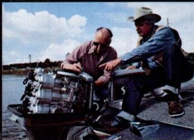
Automatic metered oil injection is a feature of Spirit's new 85-hp outboard. Lube is squirted into the engine as required.
