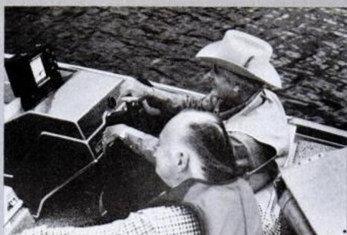
New graph depth-and-fish-finder recorders on well-equipped boats pinpoint drop-offs and lunkers while craft is planing.
