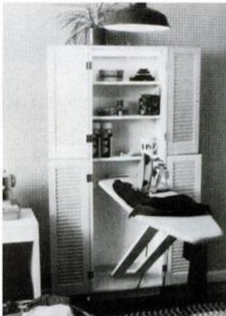
Temporarily assemble the complete unit in shop with the box set up plumb and level. When the fit proves satisfactory, remove hardware and doors to paint the center.
