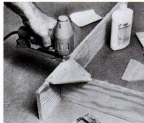
Staples simplify gluing reinforcing gussets in light assemblies. Use long-leg \frac{9}{16} -in. staples for \frac{1}{4} -in.-thick gusset.
