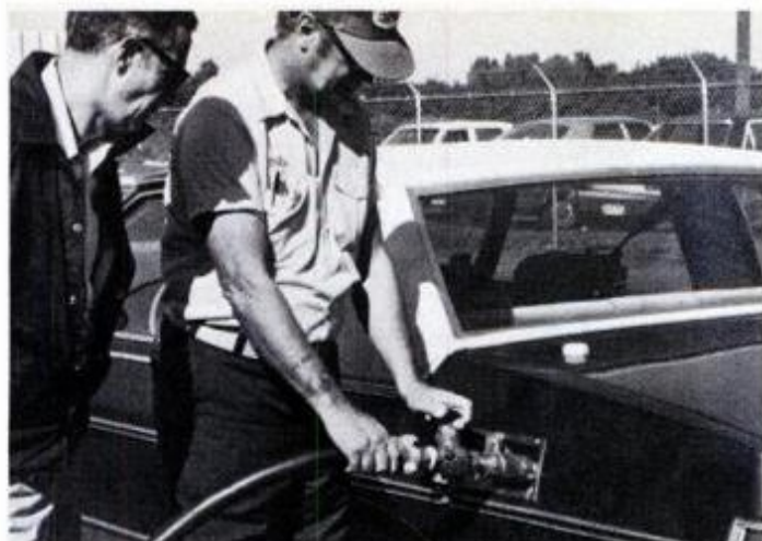
Filling a propane tank takes several minutes and requires special equipment that is not available at all propane dealers. Dealers are few and far between.
