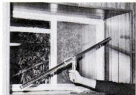
With padlock undone, tension can be released and the bar lock easily removed.
