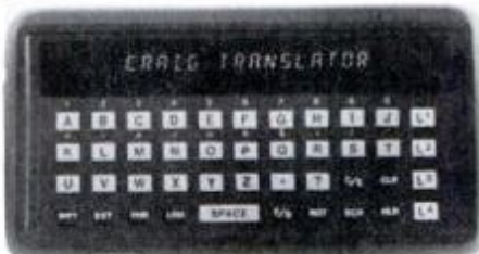
Translator from Craig Corp. is able to accept up to four language cartridges.
