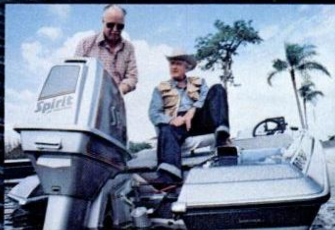
Economical operation is influenced by engine trim that can be controlled from helm. Full electric tilt allows easy beaching.
