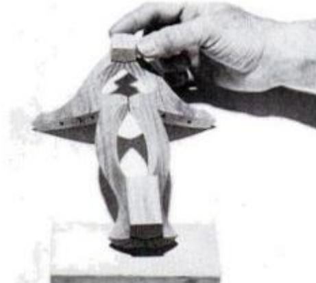
Glue face-beveled reinforcing blocks to back. They also serve as standoffs.
