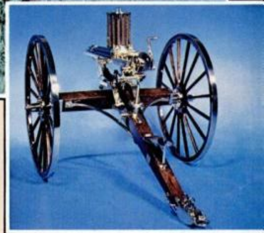
Karl Furr fires his 1/2-scale replica of 10-barrel Model 1874 Gatling gun. Miniature shoots .22 shorts at 800 rounds per minute—five shots at each turn of the crank. Feed drum holds 222 cartridges.
