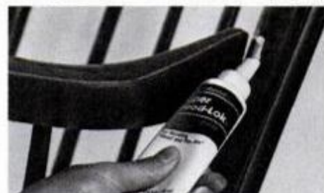
Adhesive's firm, nonrunning consistency makes it good for vertical applications.
