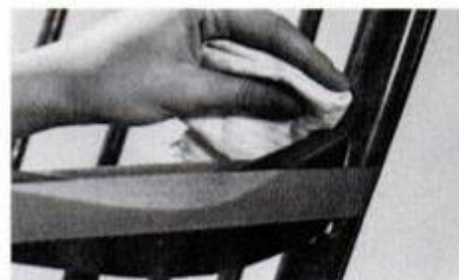
All glue squeeze-out is immediately wiped off using a slightly dampened cloth.
