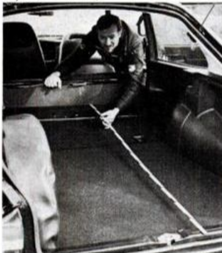
Six-foot rule stretches from folded-up back seat to tailgate in author's 900 EMS. Additional storage space is under floor.
