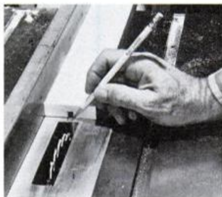
For precision, set dado to groove width wanted, test on scrap, mark cut on insert.
