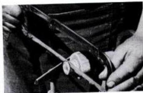
With the lathe running, carefully saw off the first escutcheon with a hacksaw.
