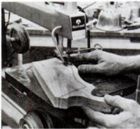
Cut curves for scroll sconce after creating bevels on inside edges. Cut both pieces at one time on a band- or other saw.
