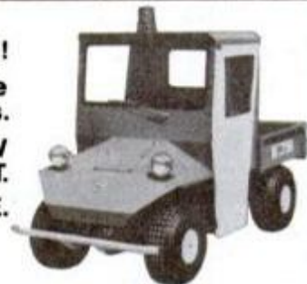
Hauler Mark 4 Model HH-411 shown with optional cab, lights, emergency amber flasher, windshield wiper and wiper. Optional bolt-on steel cab with vinyl canvas doors protect driver and rider from foul weather. Optional windshield wiper and washer for clear view.
