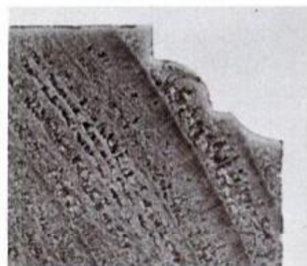
A shallower classic profile was made with the No. 1 cutter on page 59.
