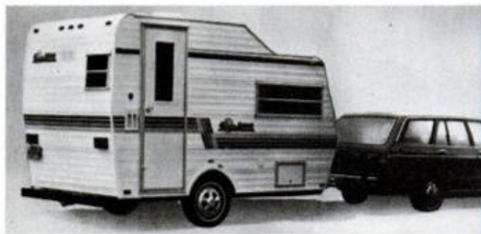
For sub-compact towing to sleep four in 13½ feet, Sunline's self-contained trailer has a hitch weight of only 125 pounds.
