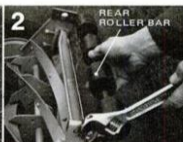
Yard-Man's model 15515 hand mower weighs 42 pounds, cuts an 18-in. swath and has a six-blade cutting reel. You can adjust the cutting height from 1/2 to 1 1/4 in. The mower is ticketed at $125.
