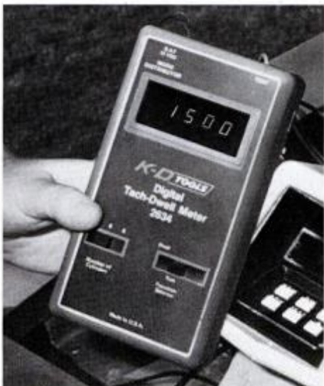
K-D Tools' digital dwell-tachometer has bright LED readout, 10-rpm resolution
