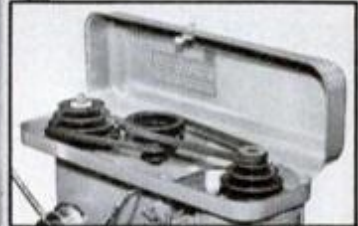
VARIABLE 12 SPEEDS! Change speeds easily with V-belt drive. Select from 12 speeds: 230 to 3890 RPM. Uses standard size V-belts.
