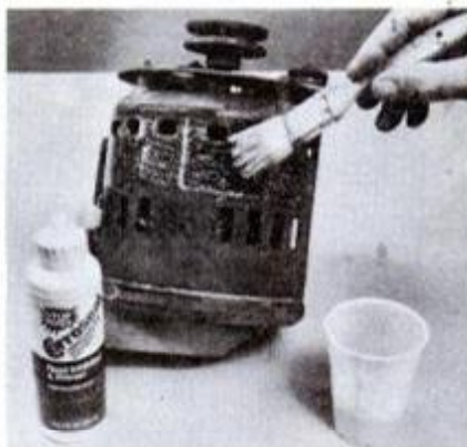
Rusted washing-machine motor housing was revived; coating is good primer for all types of topcoats.
