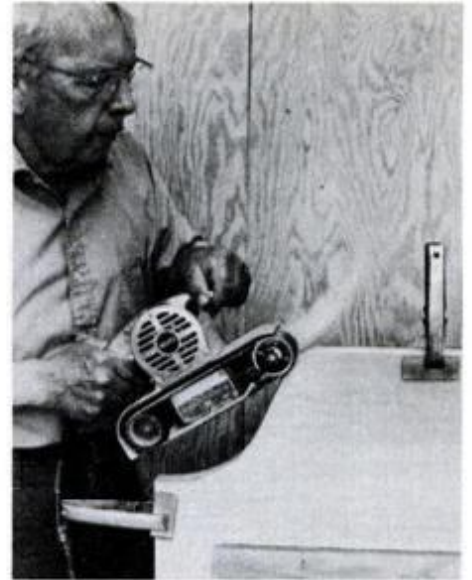
Good clamping technique on wide pieces: C-clamps and boards prevent warping.
