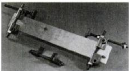
Larger of these two bar clamps is made up by using a length of scrap lumber.
