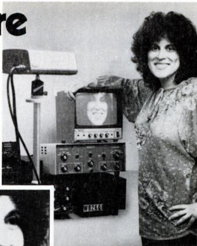
Images from a slow-scan TV monitor aren't as sharp as broadcast TV. Note how image (left) is made from 16 shades, ranging from white to black and divided into small, mosaic-like blocks. Each block's shade of gray is controlled by one of 16 different musical tones.
