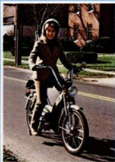
Two-speed MK II cruises at 28 mph.
