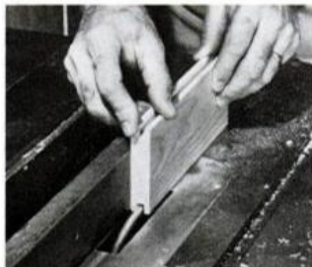
When grooving short pieces (D, E), apply pressure at front and back . . .
