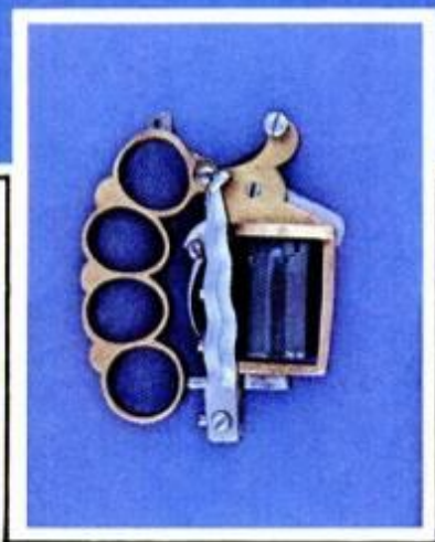
Folded for use as knuckle-duster, the triple-threat firearm had dagger, brass knuckles. Shown actual size.
