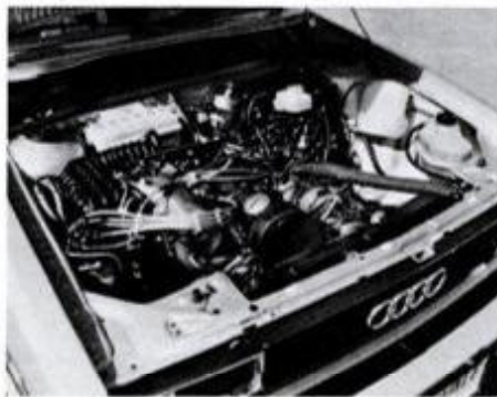
Four-cylinder engine tilts 20°, has 1588 cc, fuel injection and delivers 78 hp.
