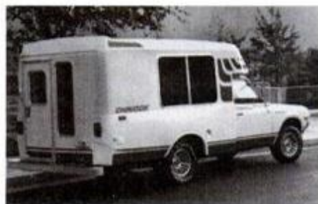
A Ford courier, Datsun or Toyota body can sit under Chinook's 17-foot Eagle to give low gas use for RV vacation travel.
