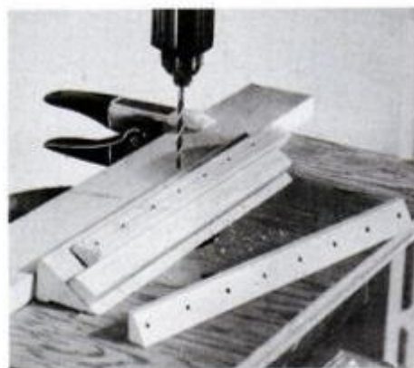
Jig helps you bore holes perpendicular to face of spool bar accurately and safely.
