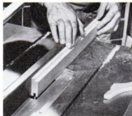
When grooving rabbeted stiles (B, C), have push stick ready for use near end of cut.
