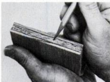
Rigid core (pencil point) consists of wood flakes, not usual laminated veneers.
