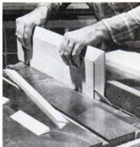
You can cut side bevels without blocks. Stand behind the fence for good control.
