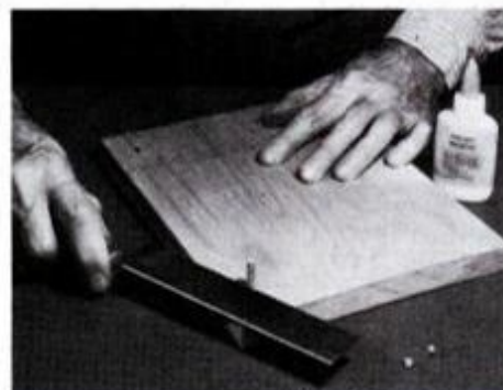
Screw hole can be filled by driving in splinter and sawing flush, or by using dowel plug and glue or plastic wood to fill.
