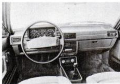
Rocker switches on sides of instrument cluster let driver keep hands on wheel.
