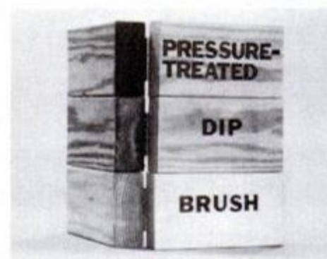
Darkened areas of 2 x 4 sections, formed by applying preservative-sensitive reagent (test solution), show extent of preservative penetration for three methods.
