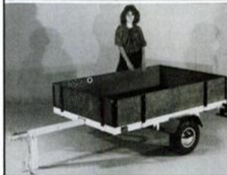
Unfolded from narrow two-foot width, the Fold'N Fun trailer can open to a 4x8-foot platform for cargo, a pair of motorcycles or snowmobiles, or a camping tent or boat. It's available in three models from Innovative Products, Appleton, Wis. 54913.
