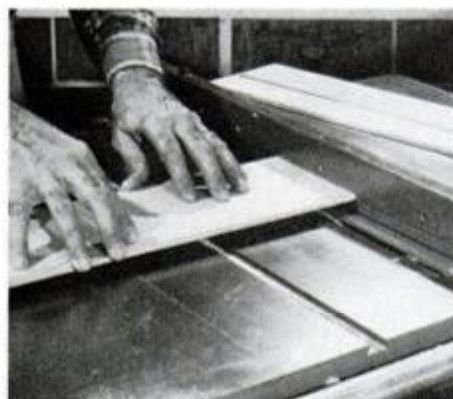
Adjust fence and blade to square off panel shoulders. First make test cuts on scrap.
