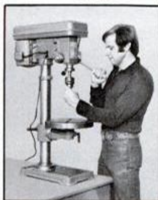
Precision ground quill has milled rear rack
