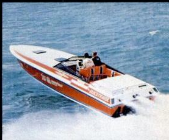
Excalibur Executioner, a limited edition 32-footer from racer Reggie Fountain, has turbocharged 475-hp Mercruisers, 87 mph.
