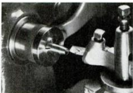
For outside bevels, invert tool bit, set slide at 80° and feed against blank.
