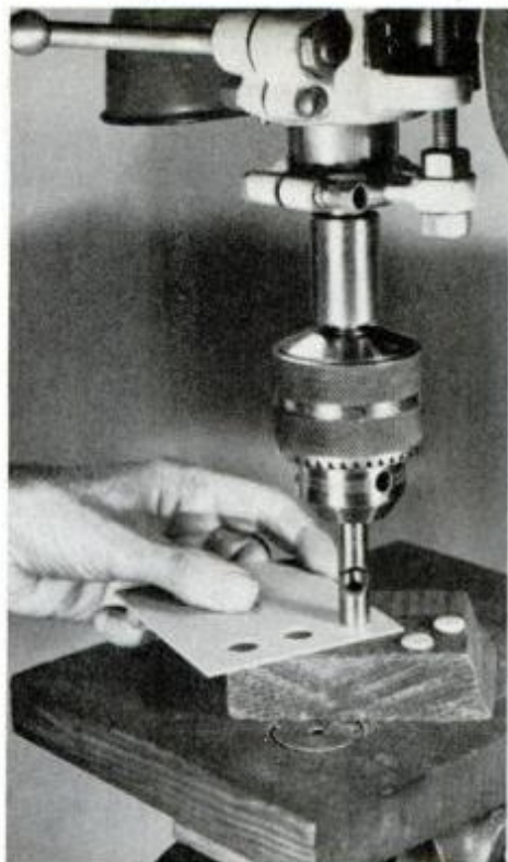
Rotary punches can be used to cut 1/2-in. holes in cardboard with a drill press (left), or 1/4-in. holes in leather by twisting punch held in tap wrench (above).
