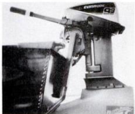
Running shoal water up to six inches thin without tearing up the prop is possible by raising the outboard and attaching a Riffle Runner by Water World, Roseburg, Ore.
