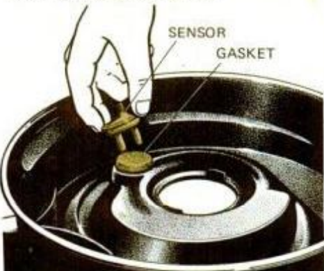
If damper door on air-cleaner housing doesn't open between 95° and 135° F., sensor must be replaced. To remove, pry off retaining clips with screwdriver. Be certain that the gasket (below) is in good condition before replacing the sensor.
