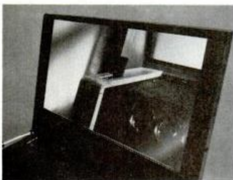
Lenses in picture tubes of a projection TV are one-piece units (as shown above and at right). The best systems available use three picture tube/lens arrangements. One assembly projects red, the next blue and the third green. The three projected images are reflected from a mirror (left) and are combined visually on the large projection screen.
