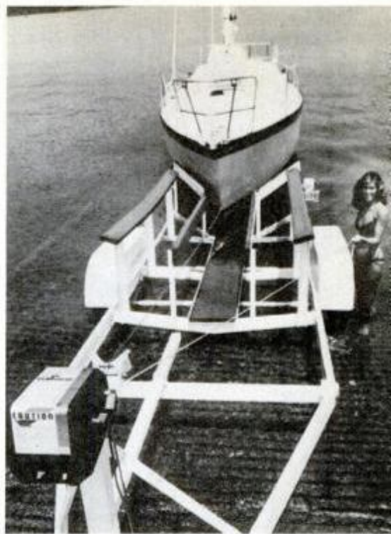
With craft up to 30 feet now being hauled on a trailer, Dutton-Lainson, Hastings, Neb., has a StrongArm electric winch to power or hand crank boats up to six tons.
