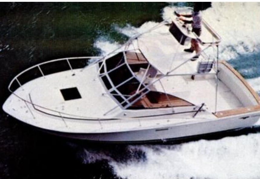
Phoenix Marine of Hialeah, Fla., offers latest Jim Wynne double-deckrise performance hull with "propeller pockets" (visible in the transom above) that require only a 22-inch draft with twin gas or diesel engines.
