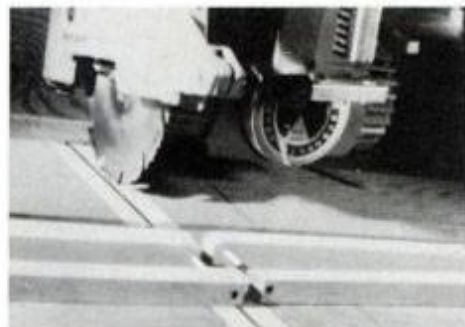
Hardwood fence has dowel hinges which allow it to pivot for cutting angles.
