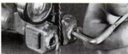
The guide pins are adjusted so they are close enough to blade to prevent it from twisting as work is fed in. Guides should not rub the blade sides. With pins as close as possible, they are adjusted forward or back to ride behind gullets of saw teeth.
