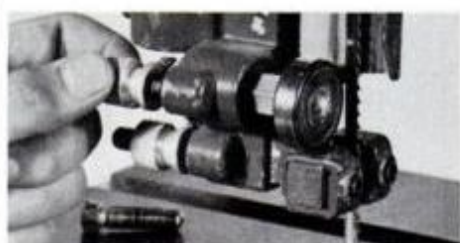
Next, blade support wheel is positioned about 1/64 in. behind blade spine. Finally, bottom guides—located below the table—are adjusted in similar fashion.
