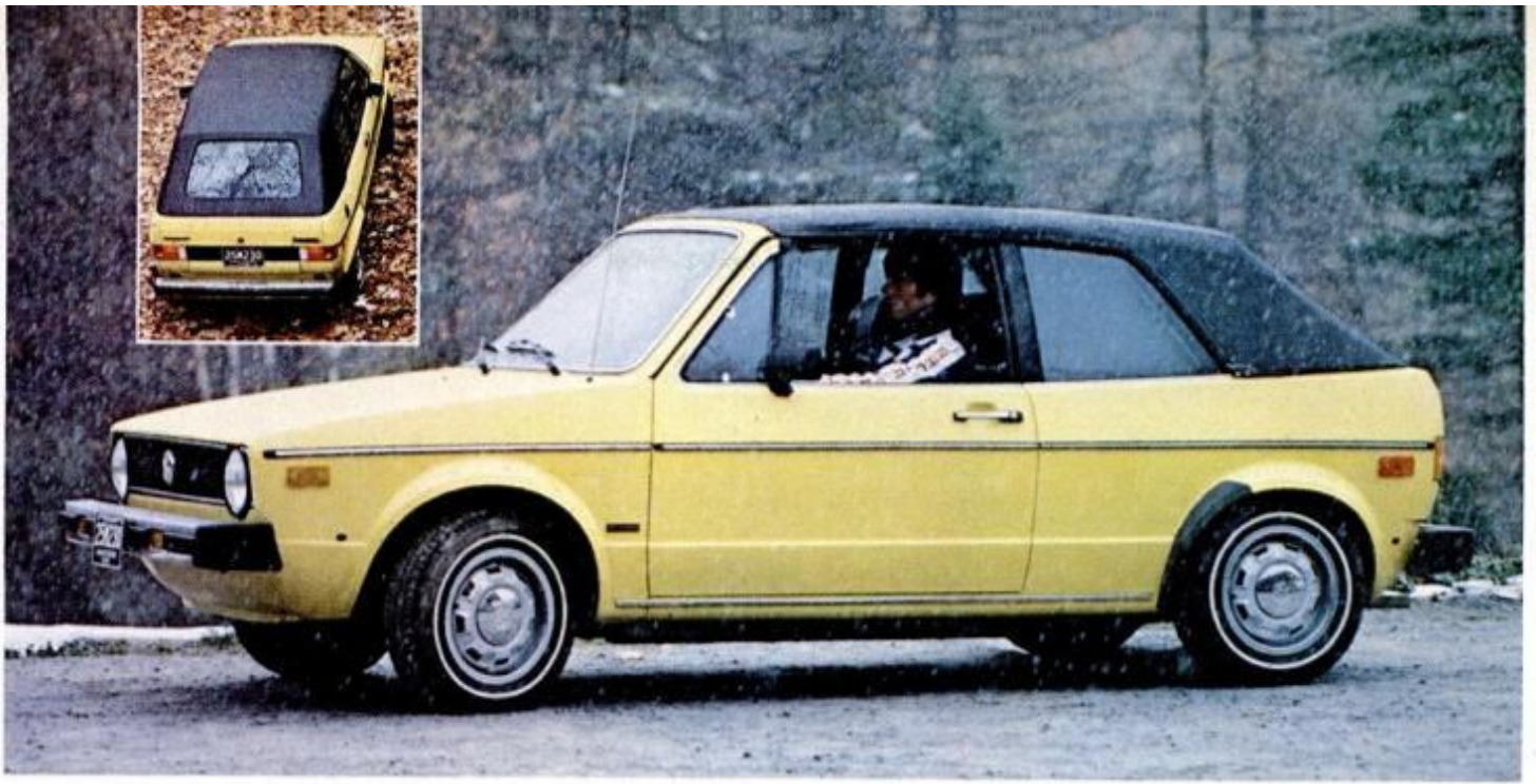
Convertible has glass rear window (inset) with electric defogger. Padded top folds down easily, doesn't take up cargo space.
