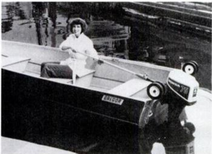
Handi-Mate is made by Bush Products in Lynnwood, Wash. The device clamps on an outboard motor tiller and extends both throttle and steering all the way up to center seat.
