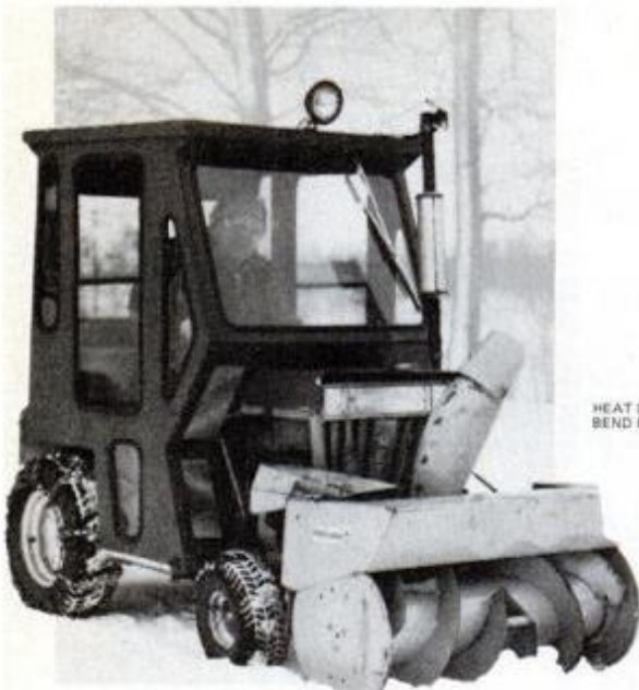
Easy-to-make plywood tractor cab keeps driver warm in severest Midwest winters.
