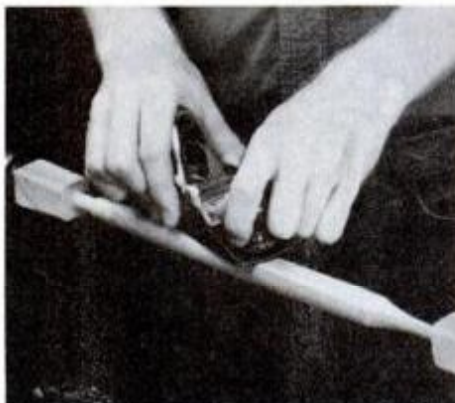
Before you remove stay from the lathe, plane two flats on opposite sides of the workpiece as indicated in the plans.
