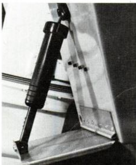
Shown in maximum "up" position, Bennett tab is remotely controlled from the helm.
