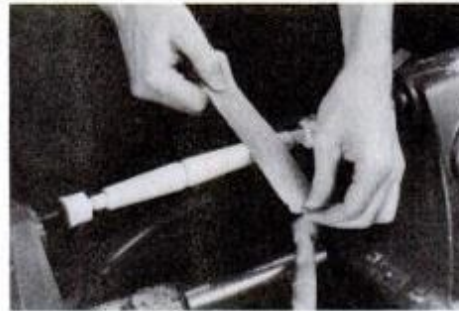
After stay has been turned and coves have been cut, sand smooth with 220-grit paper while workpiece turns in the lathe.
