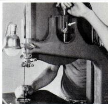
Blade must be tensioned by turning star wheel as shown. Some saws have a tension scale (arrow) that permits quick tensioning—you simply line up fiber washer with the correct tension on indicator. If your saw lacks a scale, tension blade so it has a 1/4-in. flex in a 6-in. span.
