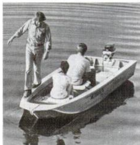
Good, quick stability test for small hull (if you're a good swimmer) is to stand on one gunwale. Grumman's 3.8 passes easily.
