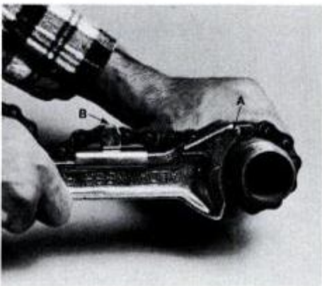
To use, wrap chain around pipe, feed end of chain under anchor pin (A), and hook to notch on spring-loaded pressure clip (B). Use like any ratchet-operated wrench.
