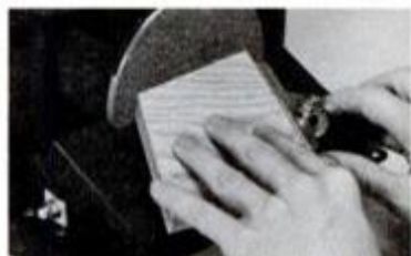
Large tilting table, adjustable miter gauge for sanding accurate angles.
