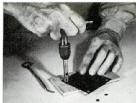
Rotary punches can be used to cut 1/2-in. holes in cardboard with a drill press (left), or 1/4-in. holes in leather by twisting punch held in tap wrench (above).
