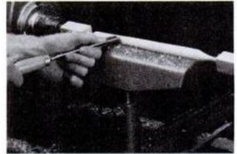
Turn 20 arrow-shaped back stays, using a cardboard template to check contour and to assure uniformity during the turning.
