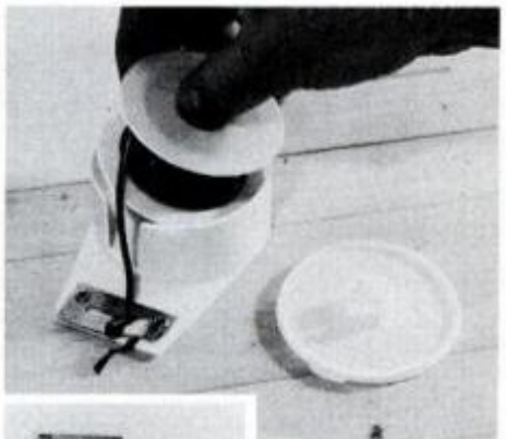
To install refill (left), cover is removed and reel is inserted (above). The spring-steel piece at bottom is used to sever the tie at desired length.
