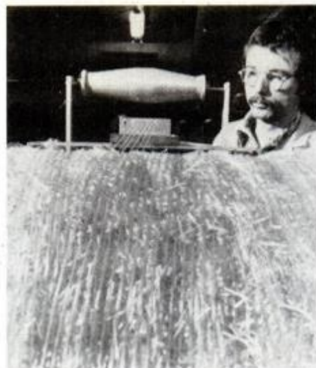
Fiberglass strands, from PPG Industries, will combine with resin and chopped fibers to make tough, moldable composite.
