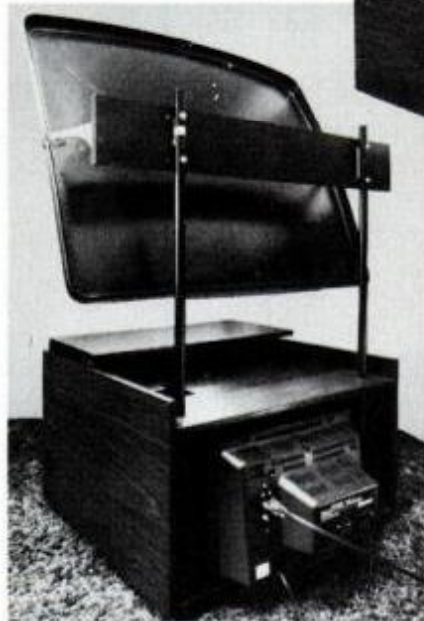
TV must be set exactly within cabinet or you'll see distorted picture.
