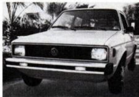
Rabbit Diesel got 38.7 mpg on 2950-mile trip from New York to San Diego.
