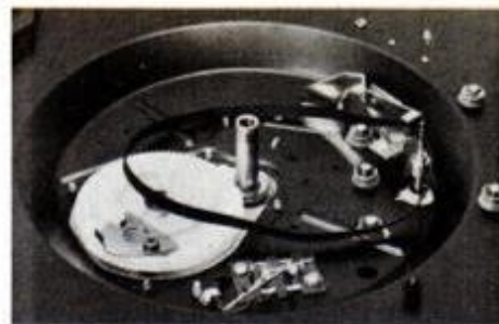
In the belt-drive turntables, moving the belt from one diameter of the pulley to another changes its speed.
