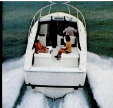
Phoenix Marine of Hialeah, Fla., offers latest Jim Wynne double-deckrise performance hull with "propeller pockets" (visible in the transom above) that require only a 22-inch draft with twin gas or diesel engines.
