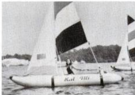
The Kat 416, an inflatable catamaran from Semperit/Steyr-Daimler-Puch, is 13 feet long, weighs 125 pounds, can carry 1000.
