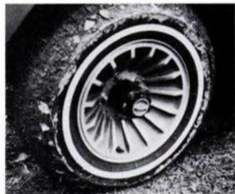
Automatic wheel hubs are $97 option: They enable 4wd to be engaged from driver's seat. Hubs can be locked manually for engine braking on front wheels. Test car had Goodyear Tiempo P225/75 R15 tires on styled alloy wheels ($440 for set of five).
