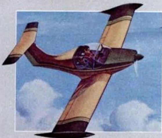
Trim little single-seat Adventure is only 13 feet long, with a 20-foot wingspan. Of composite glass-foam-epoxy construction, it has both flaps and ailerons, takes engines from 60 to 85 hp, hits speeds up to 180 mph. Plans and partial kits will be available.
