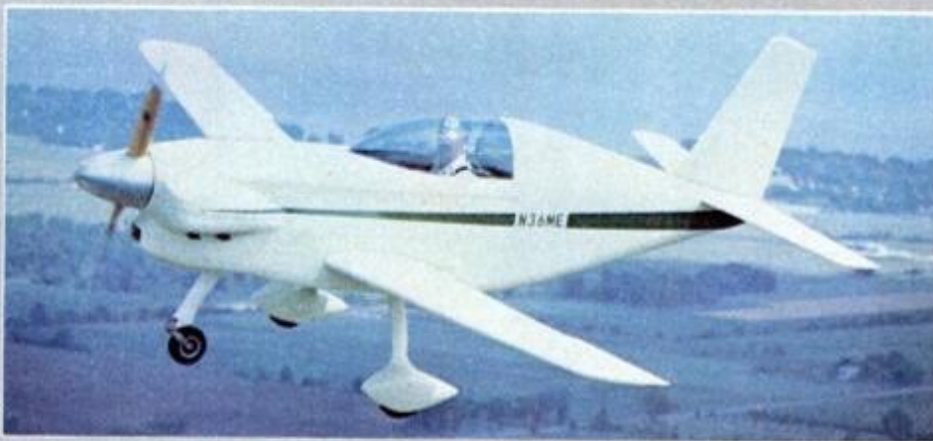
Trim little single-seat Adventure is only 13 feet long, with a 20-foot wingspan. Of composite glass-foam-epoxy construction, it has both flaps and ailerons, takes engines from 60 to 85 hp, hits speeds up to 180 mph. Plans and partial kits will be available.
