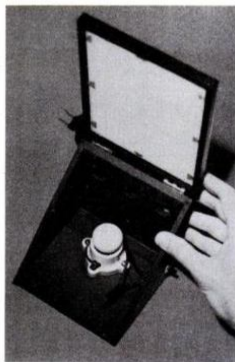
Hinged frame provides ready access to bulb. Cleat-type porcelain socket is wired in series with rotary on/off switch.
