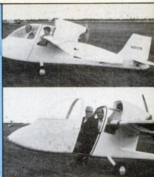
Superb visibility is keynote of mid-wing, pusher-prop Taylor Bird. Rear-mounted 65-hp Subaru engine puts two-place, tandem cabin ahead of wings, free of obstruction. Entire nose section slides forward for entry (above). T-tail shown in drawing will replace conventional tail used in prototype. Plans and parts will be available.
