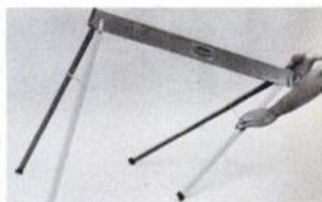
The lightweight sawhorse sets up quickly (as shown above). With an auxiliary support clamped in place (below), the sawhorse also serves as a table-saw aid.
