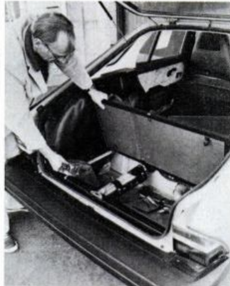
Extra space for tools and valuables is under trunk floor; volume is 1.1 cu. ft.
