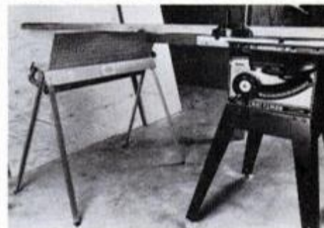
The lightweight sawhorse sets up quickly (as shown above). With an auxiliary support clamped in place (below), the sawhorse also serves as a table-saw aid.
