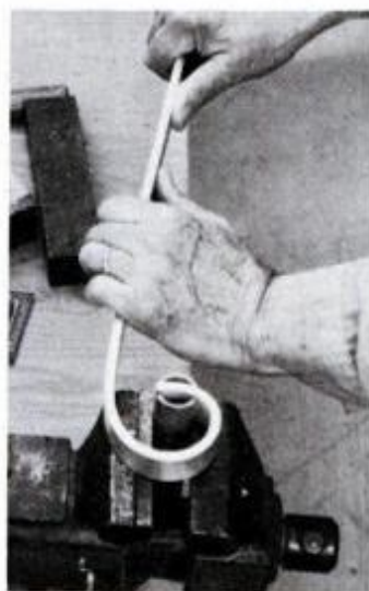
To make jig for bending scrolls in bar aluminum, cut slots in one end of 3/4-in.-dia. pipe; clamp pipe in vise. Reposition bar as needed to shape. Test on scrap to see how bend occurs.
