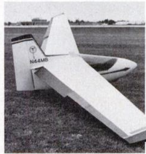
Fully aerobatic, little kit-built Minibat motor glider flies on 3-hp engine, can be assembled in a week from premolded parts.
