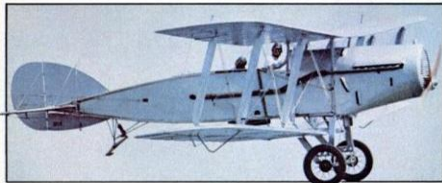
Huge biplane is full-scale replica of World War I Bristol F.2B, a two-seat British fighter with 40-foot wingspan. Six are being built for movie High Road to China .
