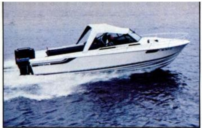
Testing on a 24-foot Regal, we found the rig handled easily over 50 mph, could be trimmed for no-torque steering resistance.
