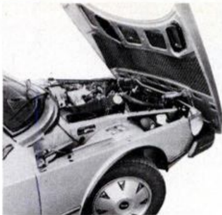
Two-liter, overhead-cam, fuel-injected Four puts out 115 hp; with turbo, 135 hp.
