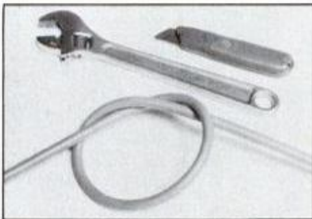
Polybutylene tube (foreground) is bent to 10 times its diameter without kinking. For example, a 1/2- to 3/8-in.-dia. tube can be turned in a 5- to 6-in. radius. Wrench and knife are used on Qest system.
