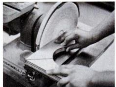
To even straight edges, use stationary sander fitted with coarse grade abrasive.
