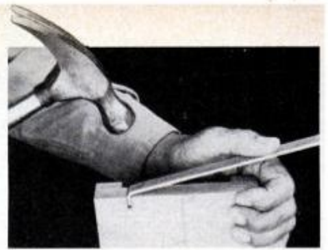
Use edge slot to make first bend in guide. Strike aluminum strip close to the bend.
