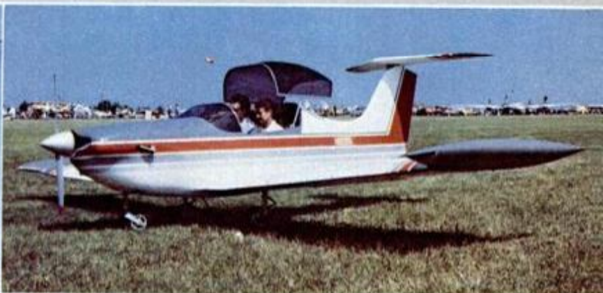
Trim little single-seat Adventure is only 13 feet long, with a 20-foot wingspan. Of composite glass-foam-epoxy construction, it has both flaps and ailerons, takes engines from 60 to 85 hp, hits speeds up to 180 mph. Plans and partial kits will be available.
