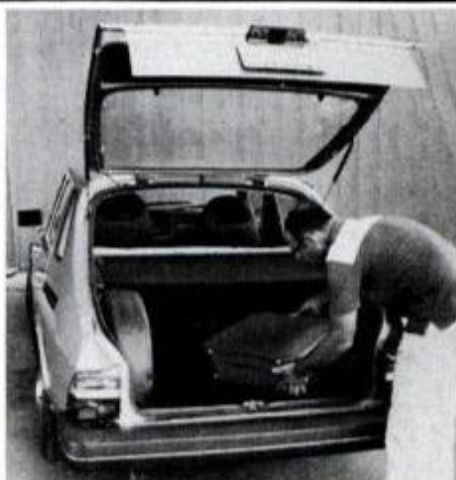
Extraordinary cargo volume and versatile arrangement are praised by owners. With the rear seat folded (left), the luggage compartment length is 71.7 inches; volume, 53 cu. ft. Trunk is formed when the back seat is upright and the parcel shelf is in place (right).
