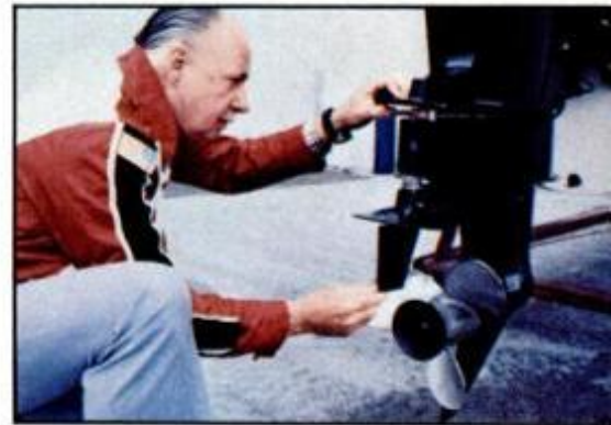
New, larger powerhead and this refined lower unit make possible higher speeds without vacuum "blowout" around prop.
