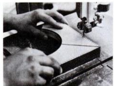
Use bandsaw to cut notches for fishing line. (See the notching diagram above.)
