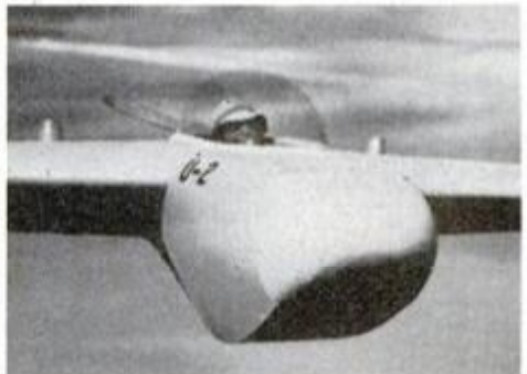
cockpit pod, retractable tri-gear. Top speed is 80 mph; wingspan, 34 feet; weight, 140 pounds. Kits will be available.
