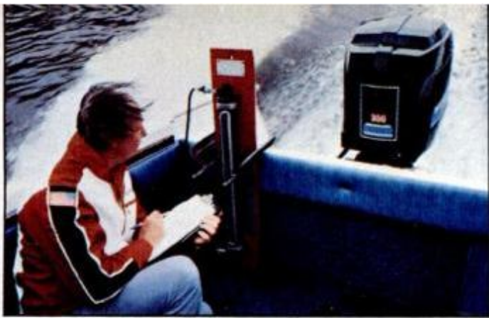
Fuel-flow meter readings indicate the new mill will not gulp extra gas to deliver bonus performance on large, heavy hulls.
