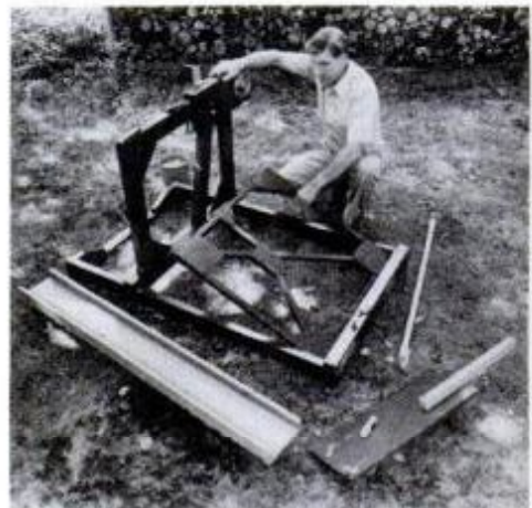
Assembling the chain-saw table takes only about five minutes. The unit folds up for easy carrying and storage.
