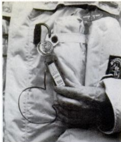
D-ring of built-in safety harness anchors water-activated Rescuelite, another aircraft item that lights on immersion.
