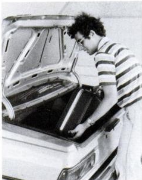
Mazda's 14.2-cu.-ft. trunk grows 11.8 cu. ft. when rear seatbacks are tilted forward.
