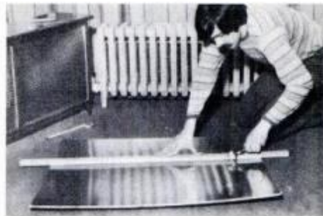
Panel is cut to size, then creased with a pie crust edger for a bend at the top.
