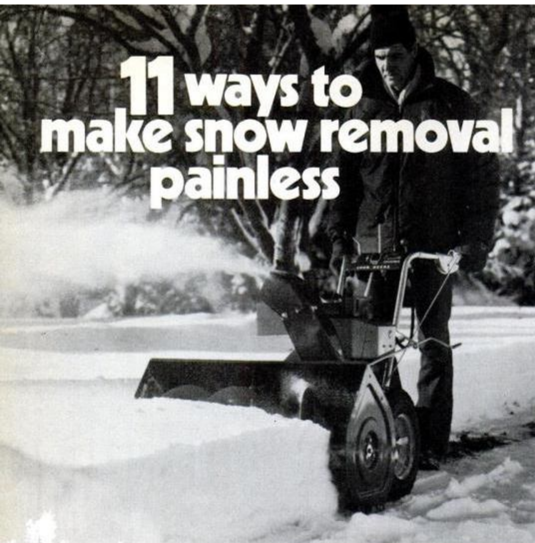
Powerful two-stage blowers have 5- to 10-hp engines, clear 24 to 32-inch widths.
