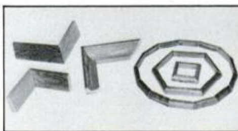
Jig makes fast work of standard 45° miters, as well as handling 15° and 30° cuts.
