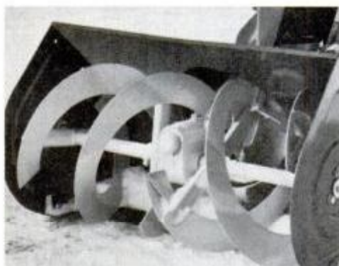
Apply coat of paste wax on inside of auger shell to help keep snow from sticking and accumulating on surfaces.
