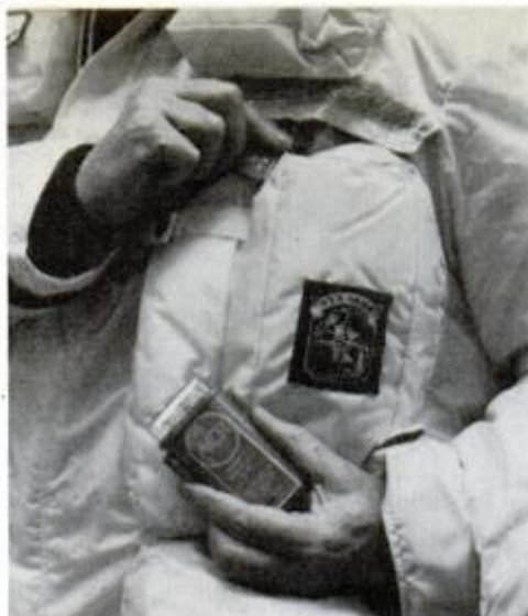
Secured below pull tab for flotation inflation cartridge, is an ACR Firefly Rescue Lite, a nine-hour flasher strobe light.
