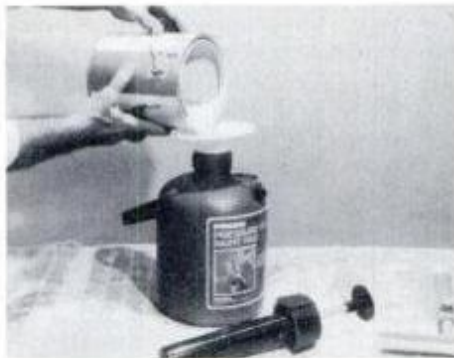
Remove the pump assembly to fill the 1-gal. tank with paint. Don't try to use extremely thick, driplless paint or oil paint.
