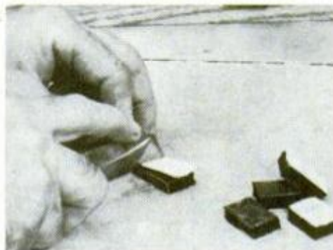
Use a utility knife to cut 16 small squares of weatherstripping from the roll.
