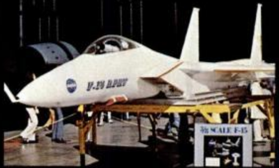
Stall characteristics of Air Force F-15 fighter were tested in a remotely piloted, 3/8-scale model of the plane, launched from a B-52.
