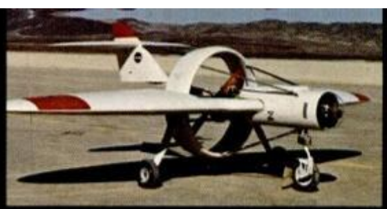
To test oblique wing flight concepts, NASA contracted for rotating-wing RPRV powered by 4-cylinder, 90-hp engine driving shrouded prop.
