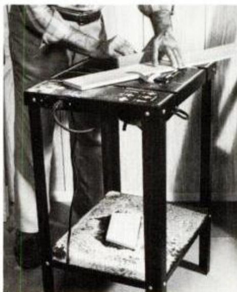
Steel saw table can be used with router, portable circular saw or sabre saw.
