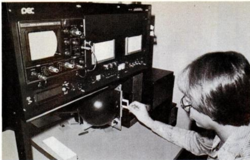
Technician puts slide in laser printer. Scanning process takes less than 20 seconds.
