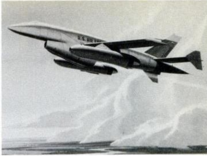
Air Force's Firebee II is a tactical RPRV system including models for high and low altitude reconnaissance plus ordnance delivery.
