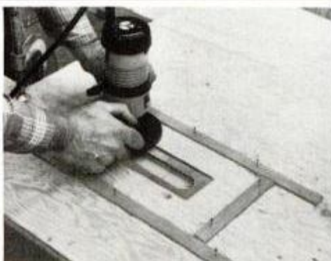
Cut table insert recess using router and mortising bit. Wood strips act as guide.
