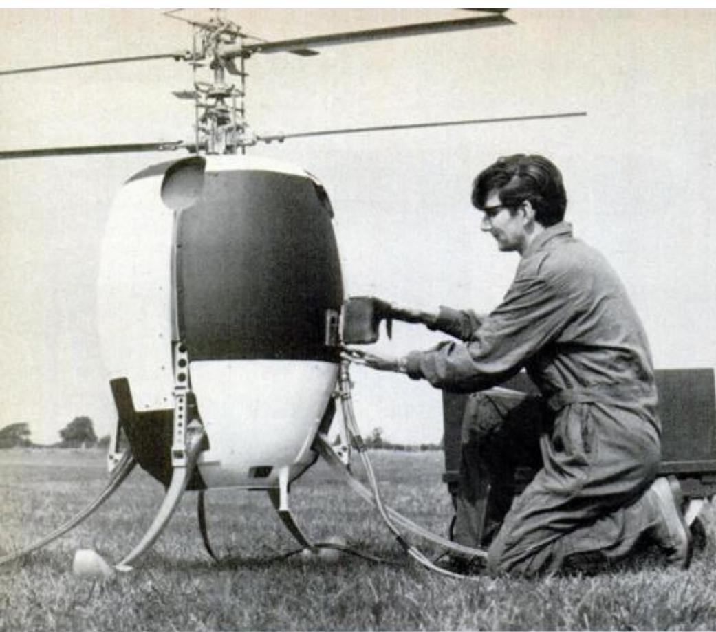
Mini-RPV built by Westland Helicopters Ltd. in England could also be called a remotely powered helicopter (RPH). Designed to provide battlefield surveillance (both visual and electronic), the RPH uses a coaxial rotor system. Of prime interest to military users is its resistance to detection by radar, sonar or infrared equipment.
