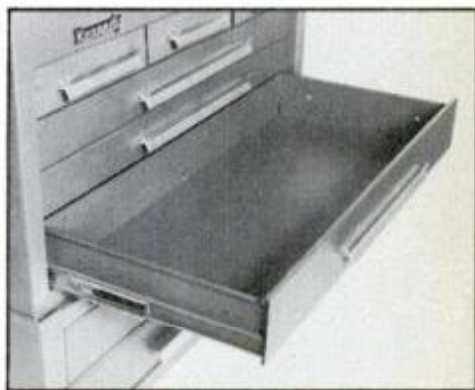
Full-extension drawers are a plus. They allow easy access to all tools. Sturdy drawer slides are a must.
