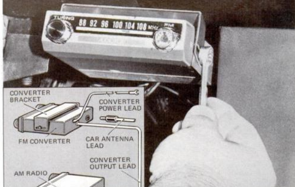
Diagram (left) shows how FM converter attaches between your car radio and car antenna. Photo (above) shows how easily under-dash installation is accomplished.
