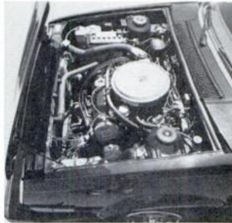
Crosswise Four delivers 90 hp with 5-speed or 85 hp with Hondamatic, burns regular.
