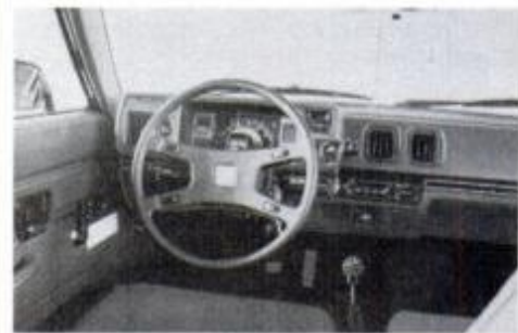
Speedo, tach needles share central dial. Owners object to awkward radio controls.
