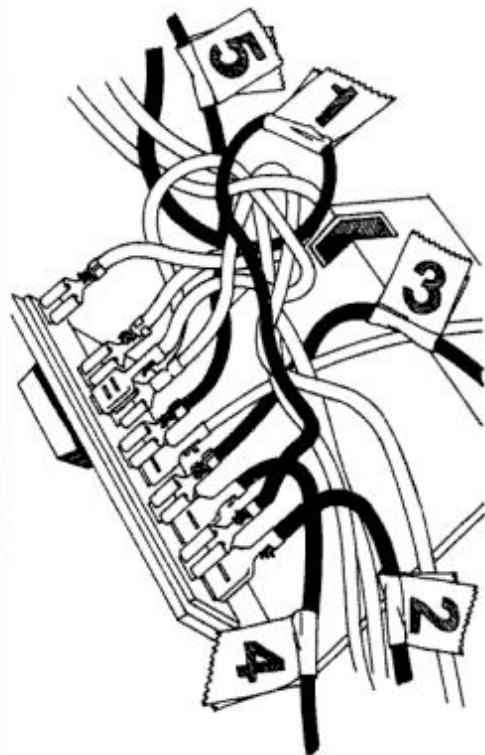
Numbers identify wires for reinstallation.
