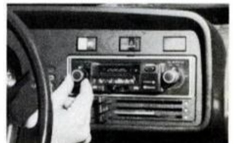
Once again, the final installation. Note how mounting plate Clarion supplied fits dash perfectly. It's little touches like this that make for good styling.
