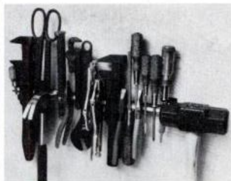
Toolholder is claimed to hold up to 480 lbs., will grip round-shank tools.
