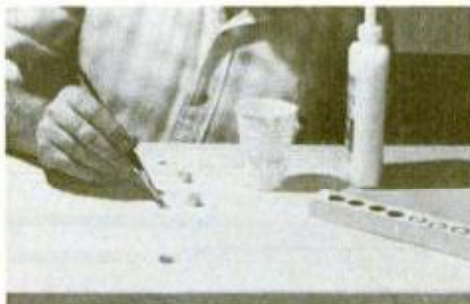
Use brush to apply small amount of white glue in holes for plugs; tap into place.
