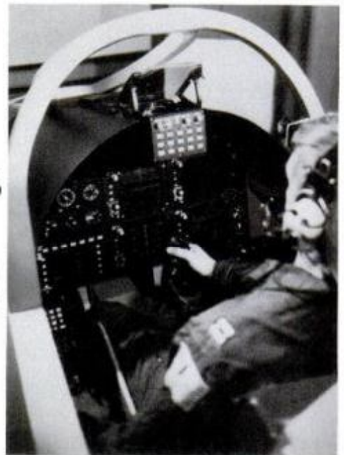
Cockpit of the future? Simulator tests will reveal practicality of experimental instrument system relying on digital computers. Cathode-ray tubes guide pilots to targets and back, with electronic maps.
