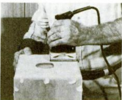
Set nailheads, fill the holes and sand all surfaces smooth before making the saw cuts that separate the doors.
