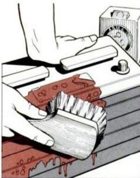
Scrub the battery top, sides and bottom with a mixture of baking soda and water.
