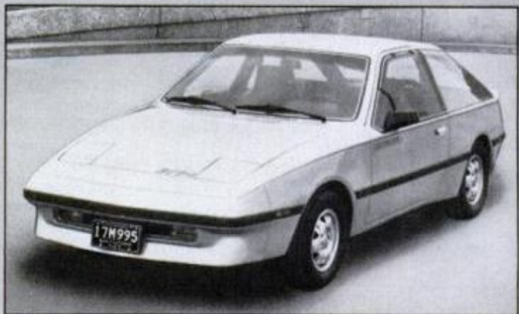
Experimental ETV-1 by Chrysler and General Electric is four-seater with 75- to 100-mile range. It may be available in mid '80s.
