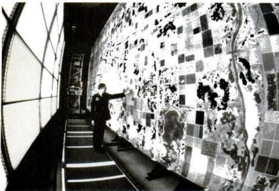
Tiny TV camera on a boom "flies" over model board at Wright Patterson, sending realistic images, including lights, farms, bridges, rivers and cities, to display system in cockpit simulators. Covering TV lens with a filter simulates fog.
