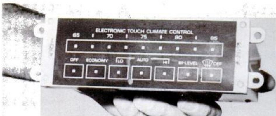
Temperature controls optional on Buick Electra use all-electronic, touch-switch panel, computer and motors (not vacuum switches, diaphragms) to work flap doors, ducts.
