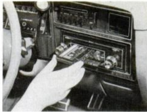
Once radio is in, check out each function—even those you won't use very often. The completed installation should look just like a factory job—only better!
