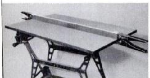
Use glue and clamps to hold 1x2 in place on bottom of the Vulcanfibre panel.
