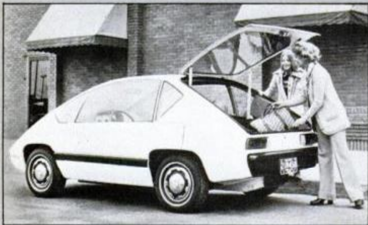
Experimental car by Copper Development Associates is 3000 pounds with 1200-pound battery pack, goes 120 miles at 40 mph.
