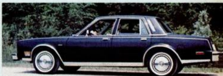
Chrysler LeBaron four-door is on a 112.7-inch wheelbase, but new coupe model is 108.7 inches between the wheels.
