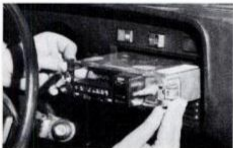
Note the clips on the side of this Clarion PE-662C unit—you need them for Rabbits and Audis. Clarion radios have mounting kits for most imported cars.
