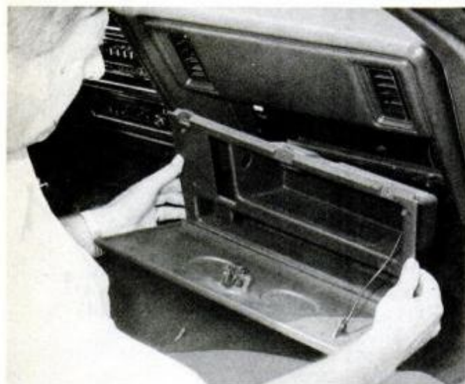
Mirada and Cordoba glovebox (left) removes easily, leaving a huge opening for access to heater and air conditioner ductwork, some vacuum controls and electrical connectors. On the slant Six and 318 engines, you'll find the coil more accessible (above, left). Periodic checks of the NOx sensor (above, right) are quick because of its easy-to-reach position.
