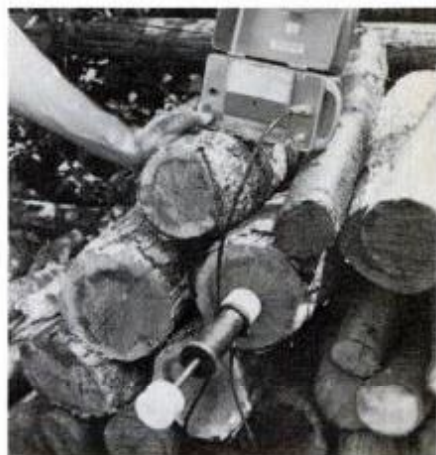
Meter reads 23-percent moisture content in logs seasoned for 10 months—slightly high for clean burning.
