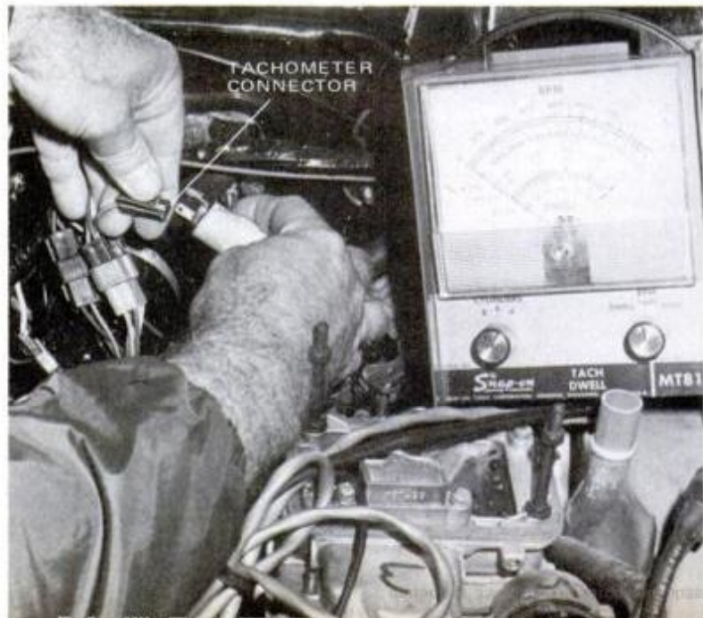
Tachometer connector on the Pontiac-built four-cylinder engine (above) is viewed from underneath the car. It's a nightmare to reach, so AMC designed in a wiring harness with protective connectors that places a tachometer connector in a more convenient location. It's now inside at the top of the engine compartment, as shown at right.
