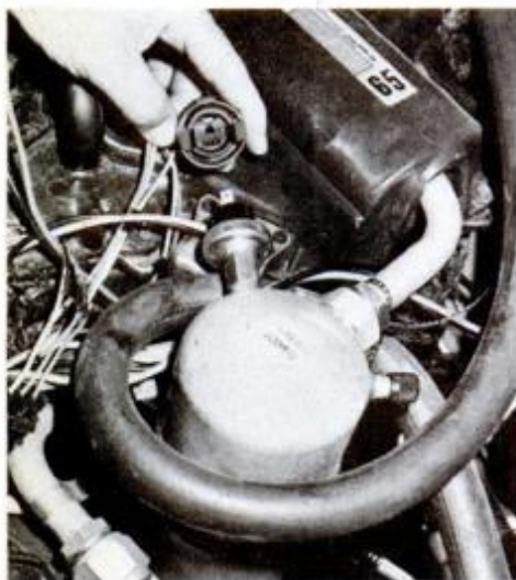
Easier servicing of GM airconditioning systems is the advantage of a new pressure switch. It's found on the accumulator.
