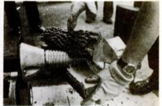
Bark Buster 50 , a self-contained, screw-type splitter, is $400 from F.W. and Associates. It's compact enough to fit most car trunks and weighs 125 pounds. The handle, used to wheel unit, doubles as a log-support bar when repositioned beside screw. Screw tip is removable for sharpening.
