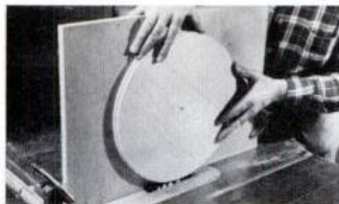
To cut edge groove, lower dado head and clamp jig to fence. Turn on saw, elevate cutter slowly, rotate wheel into cutter.
