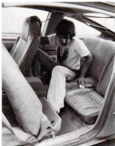
Tall driveshaft tunnel splits rear seats, which, at best, have room for children.
