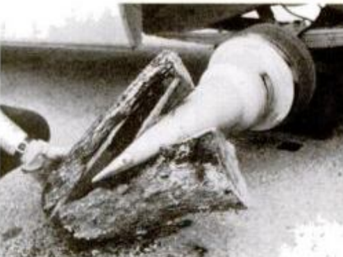
Hub-mounted screw lets you do two-month wood supply with same amount of gasoline you'd use to mow your lawn. It splits 30-inch-diameter logs up to 24 inches long.
