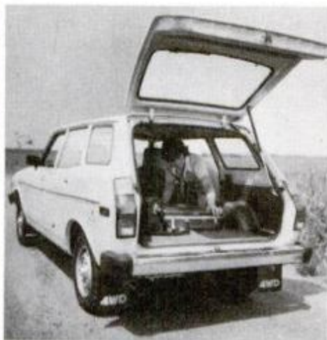
Rear-seat bottom tucks against front back rest, gives large cargo deck with low sill.
