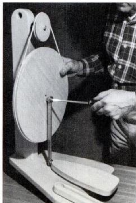
Screw offcenter bolt (N) into pretapped hole in axle hub. Note: Attach drive belt before installing the footman.
