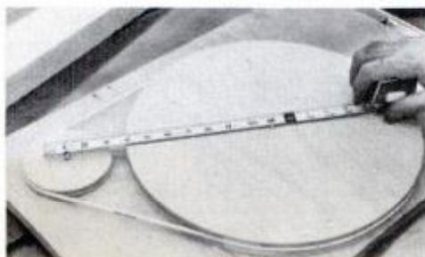
The center-to-center spacing for bearings can be double-checked by test assembling wheels and belt before drilling.
