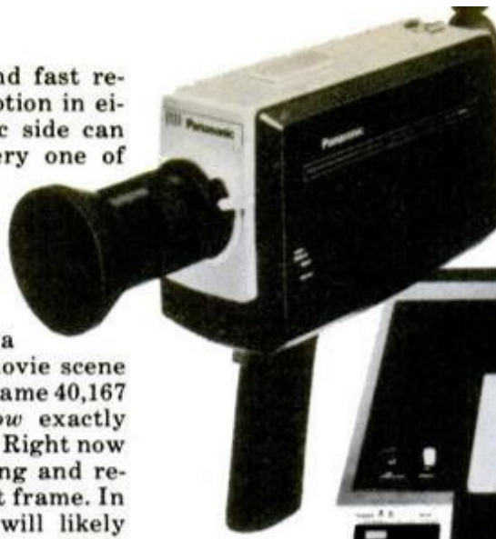
Video cassettes, such as this PV-1600 from Panasonic, point up differences between disc and cassette. As shown, this deck can use different video cameras to record home video "movies." It can also record off the air. Discs are play only.
