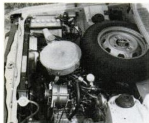
Oil dipstick hides under spare, but engine access is good otherwise, say owners.
