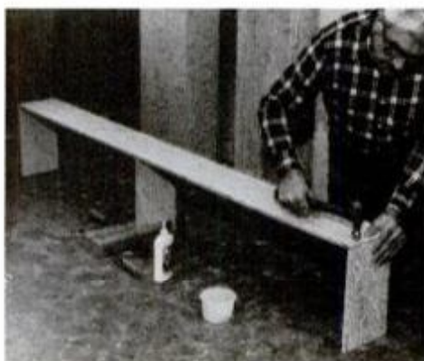
Platforms are made up as individual units, then secured to the bed frame with nails or screws at final assembly in the bedroom.
