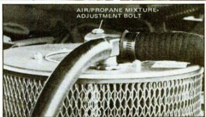
New components under the hood allow V8 to be switched between existing gasoline system and added propane system.
