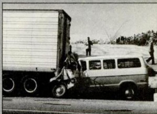
When a lighter vehicle—even a van—hits a heavy truck, the results can be gruesome. Slow moving, improperly lighted truck can cause fatal rear-enders.
