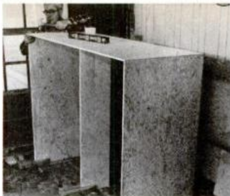
Clamps are handy for holding boards in place while nailing. A temporary center-piece permits lifting ends to apply glue.
